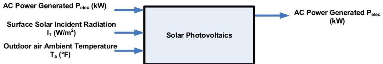
Figure 3.8. Input/output diagram for solar photovoltaics monitoring algorithms.
