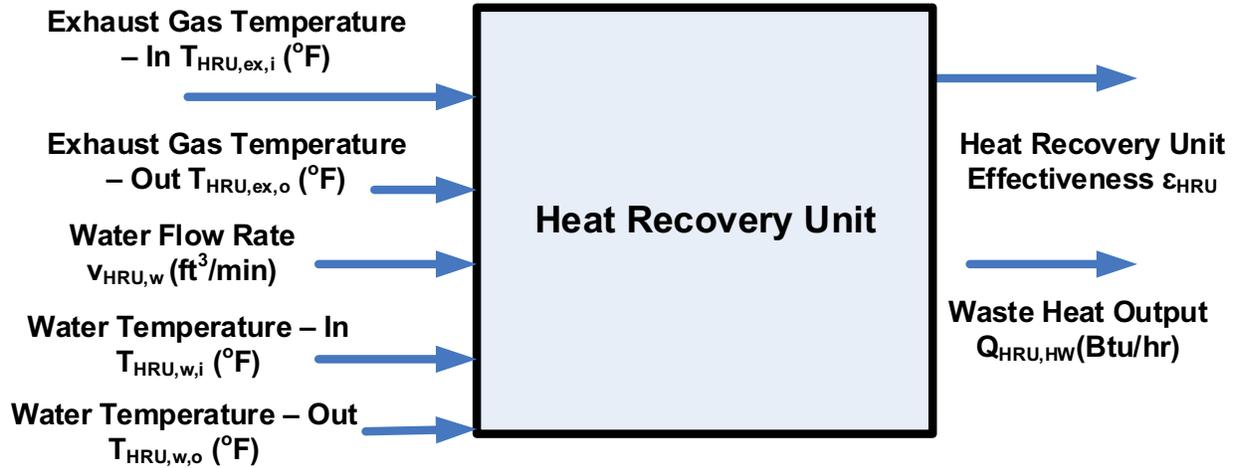
Figure 3.3. Input/output diagram for heat recovery unit monitoring algorithms.
