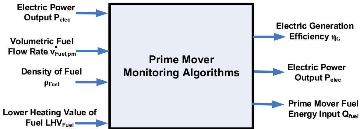
Figure 3.1. Input/output diagram for prime mover performance monitoring algorithms.
