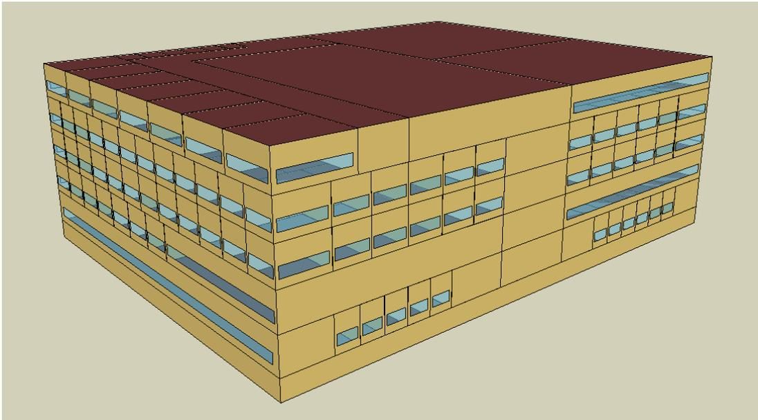
Figure 2.1. Axonometric projection of the geometry of the DOE hospital prototype.
