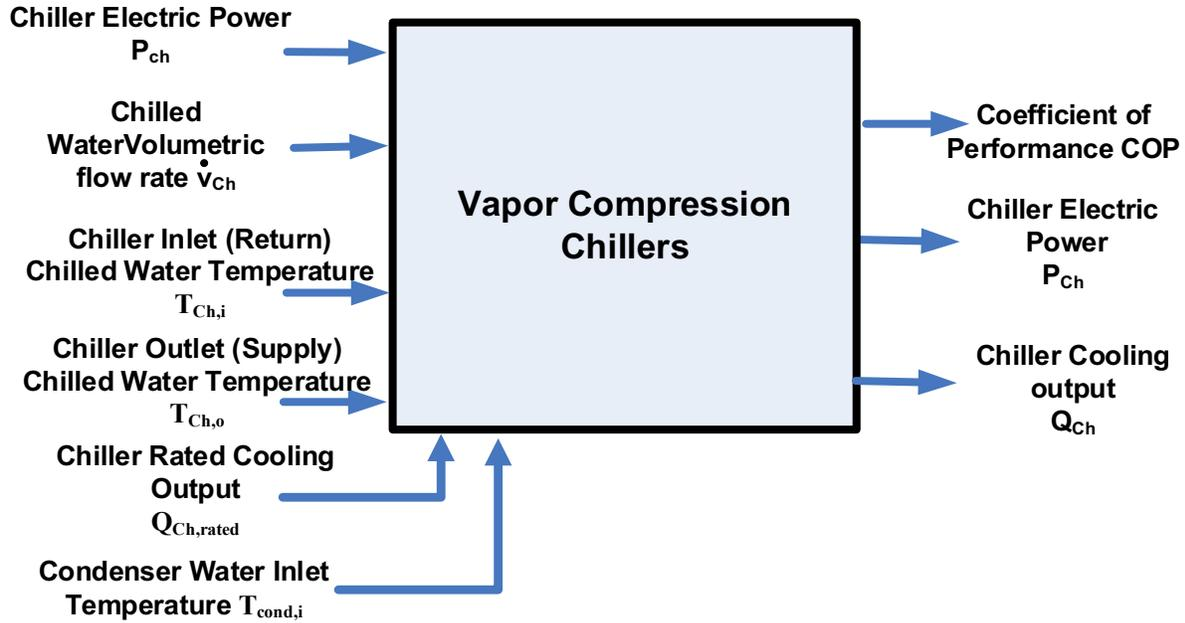
Figure 3.2. Input/output diagram for vapor compression chiller monitoring algorithms
