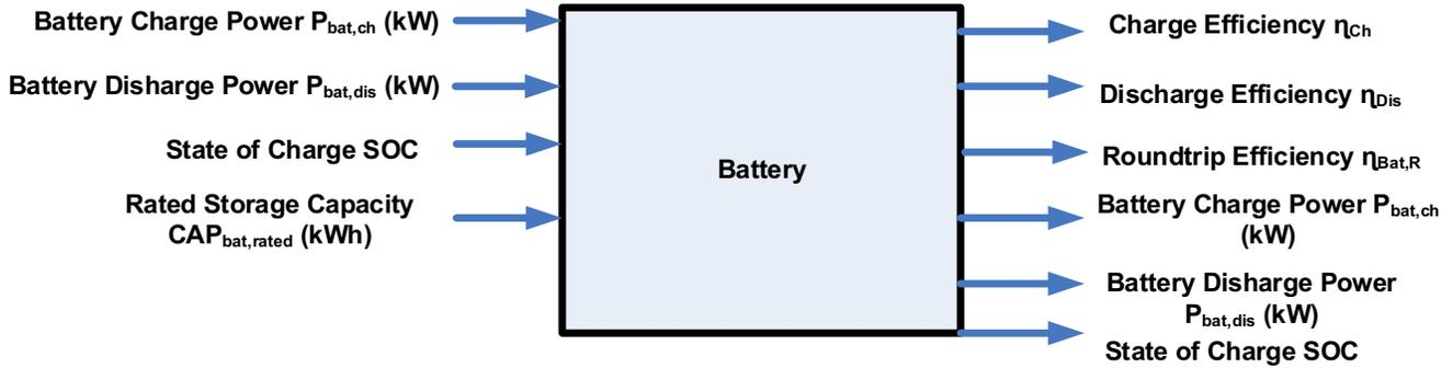
Figure 3.6. Input/output diagram for battery monitoring algorithms.
