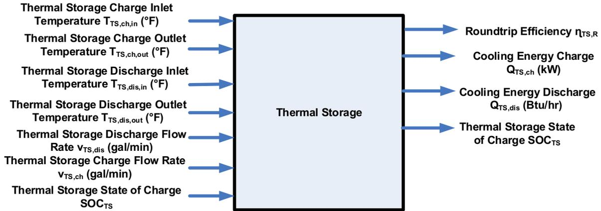
Figure 3.7. Input/output diagram for thermal storage monitoring algorithms.
