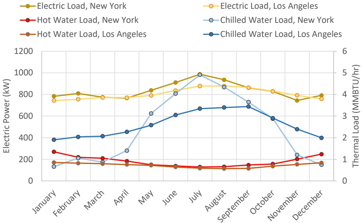
Figure 2.4. Variation of average electric, chilled water, and hot water building loads on a monthly basis (Los Angeles and New York).
