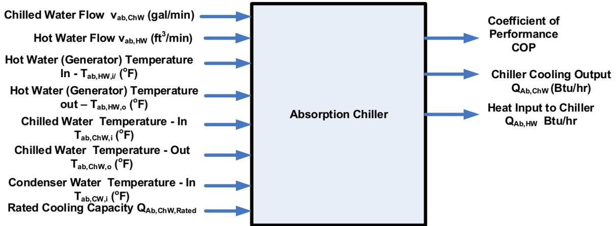
Figure 3.4. Input/output diagram for absorption chiller monitoring algorithms.
