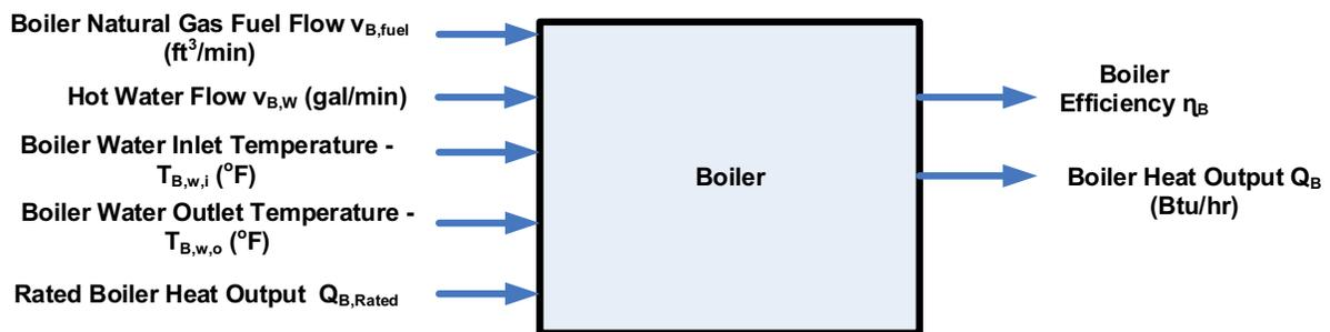
Figure 3.5. Input/output diagram for boiler monitoring algorithms.
