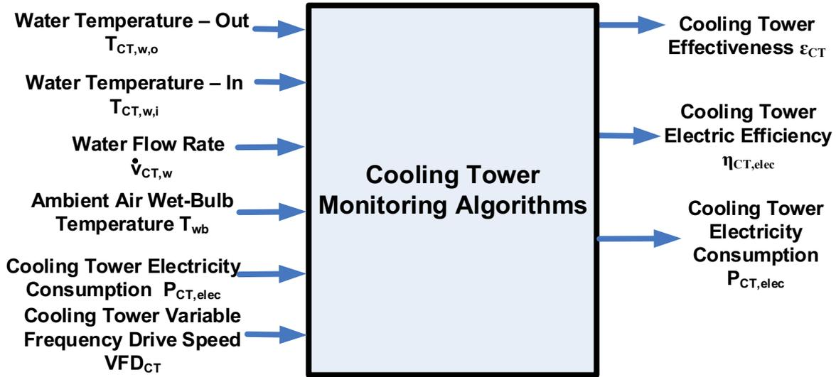
Figure 3.9. Input/output diagram for cooling tower monitoring algorithms.
