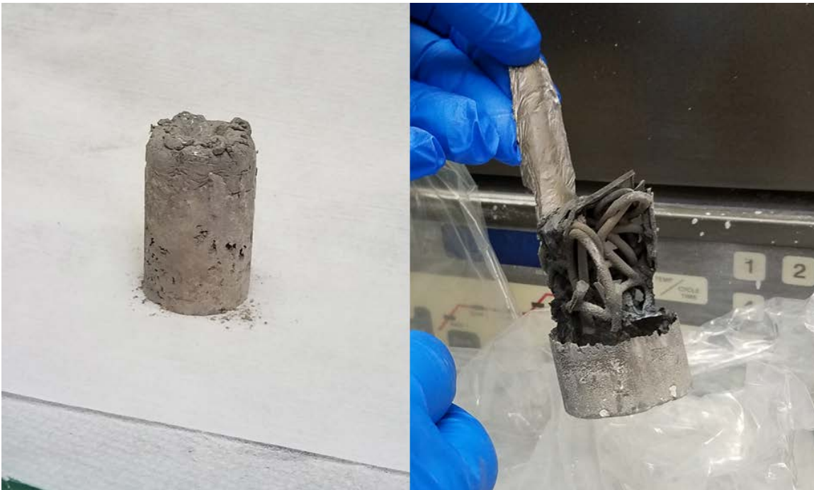
Figure 2.2. U10Zr Casting #2 (VIM-Only) ( left : Billet; right : Crucible Dross)
