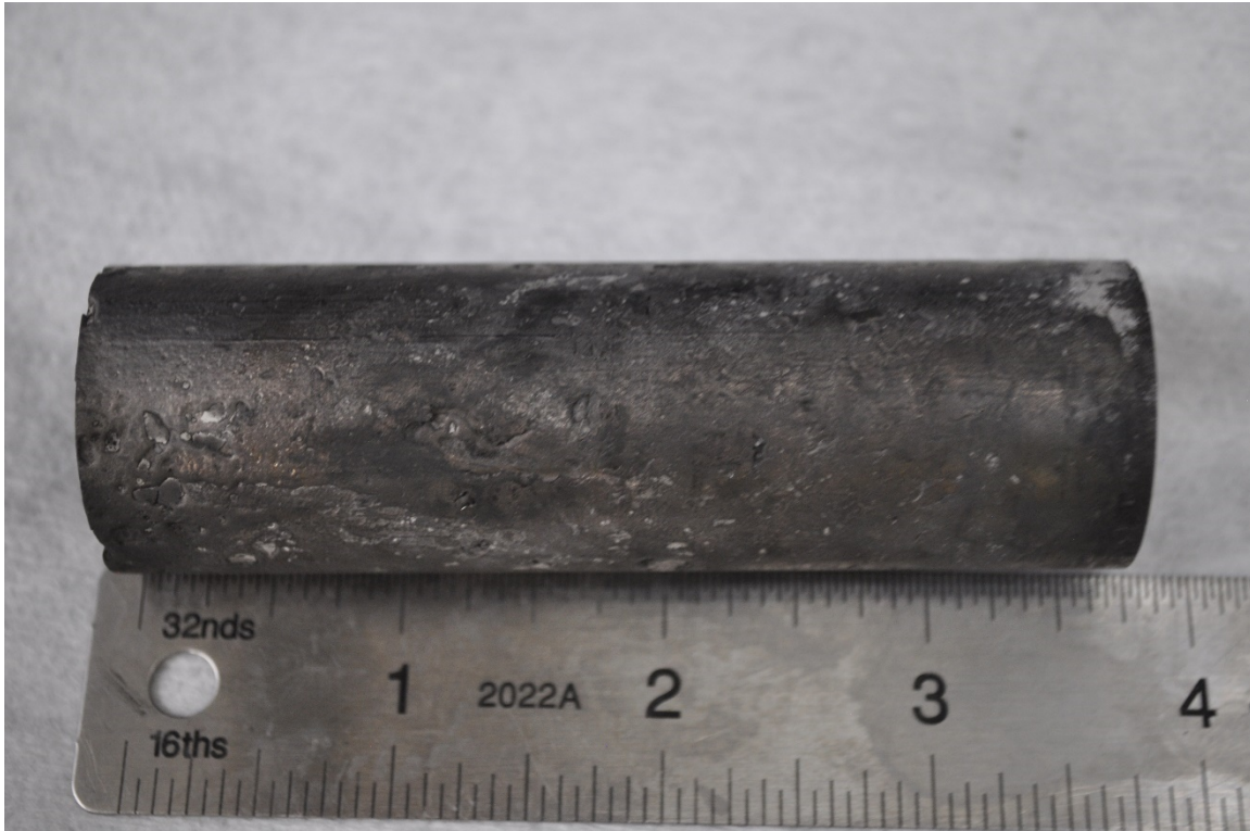
Figure 2.4. U50Zr Casting #4 (Master Alloy Feedstock)
