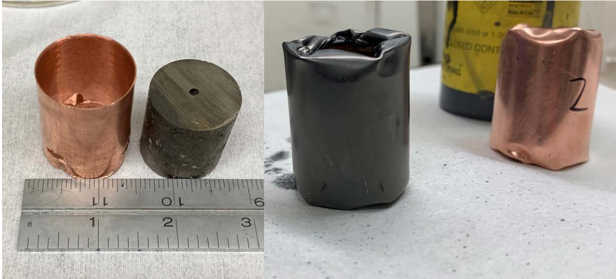
Figure 3.1 U50Zr 630°C Extrusion Billet and Cu Can (left); 680°C and 630°C Canned Billets with 630°C Billet Lubed (right)
