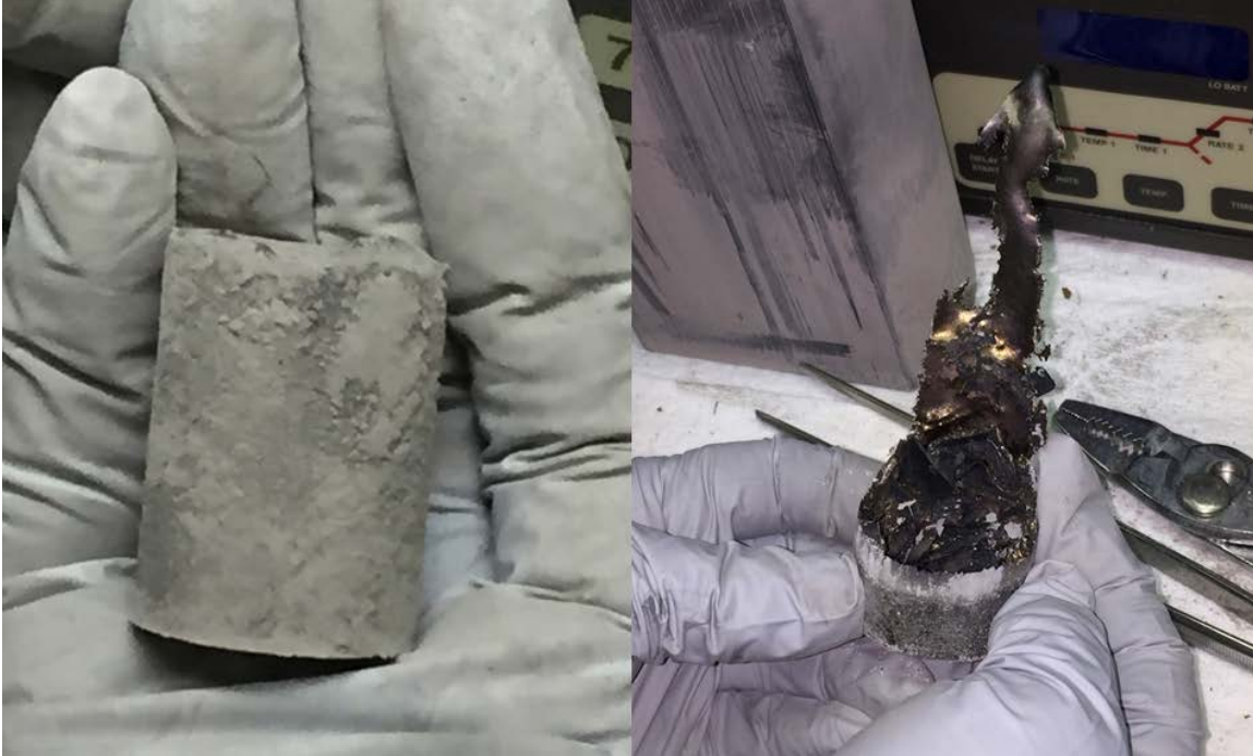
Figure 2.1. U10Zr Casting #1 (VIM-Only) (left: Billet; right: Crucible Dross)
