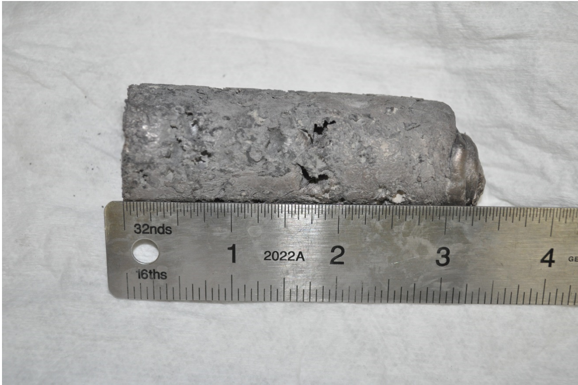
Figure 2.3. U10Zr Casting #3 (Master Alloy Feedstock)
