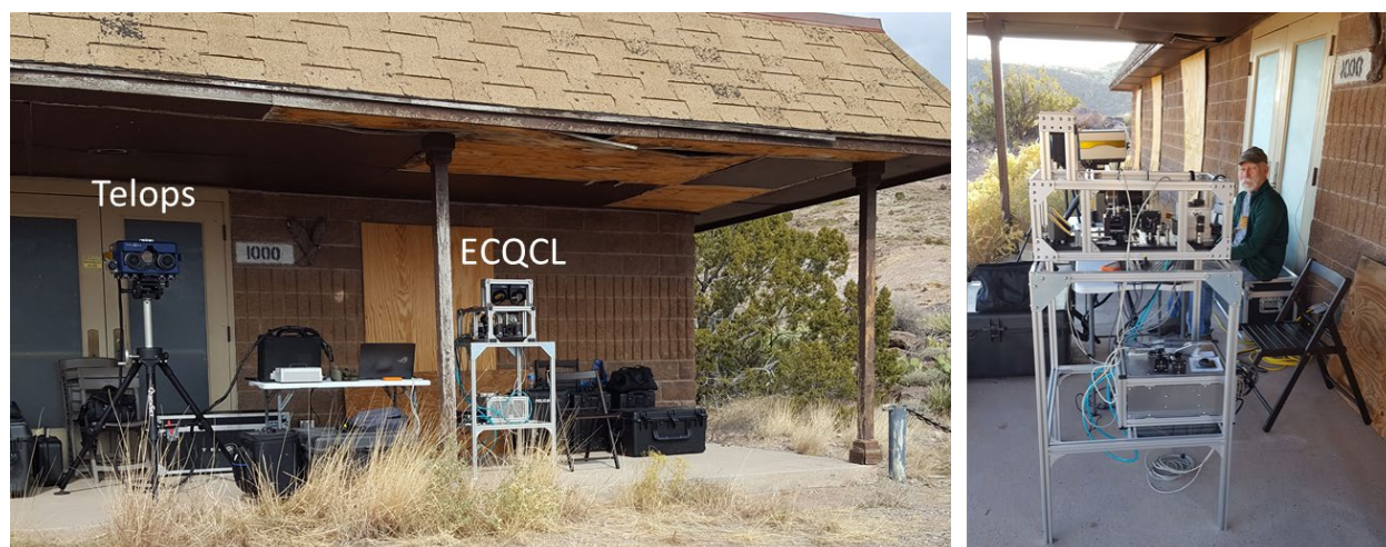
Figure 3: (left) Photograph of swept-ECQCL system and Telops hyperspectral imaging instrument at Little Eagle site. (Right) Dr. Bruce Bernacki (PNNL) operated the Telops system.
