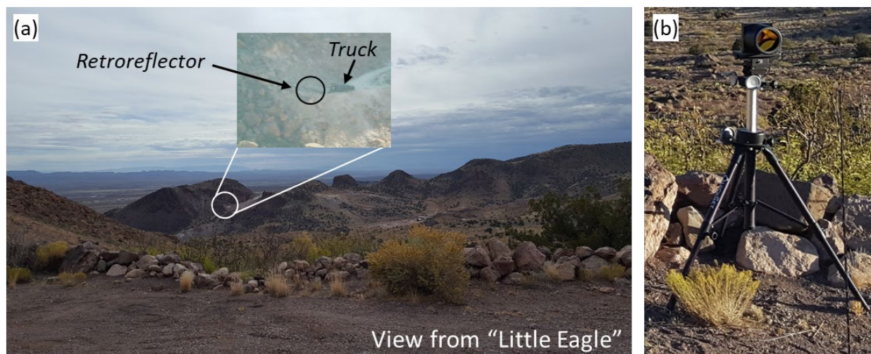
Figure 4: (a) Photograph of valley from swept-ECQCL located at Little Eagle site. The inset shows an image obtained using the visible alignment camera coaligned with the ECQCL beam. The approximate location of the retro-reflector is circled. (b) Photograph of retro-reflector mounted on tripod.
