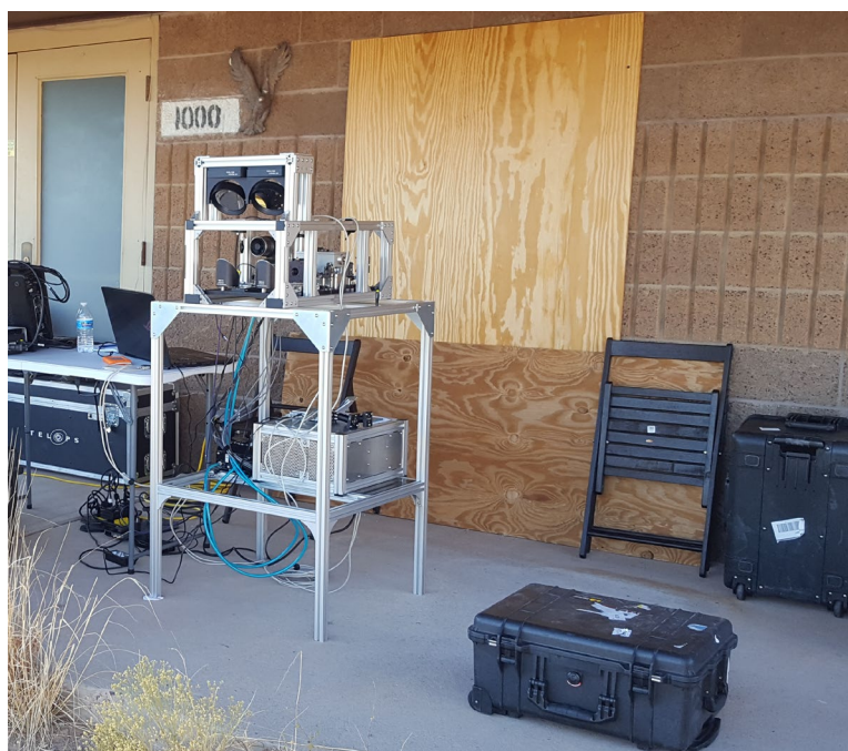
Figure 2: Photograph of swept-ECQCL remote detection system located at EMRTC “Little Eagle” site.
