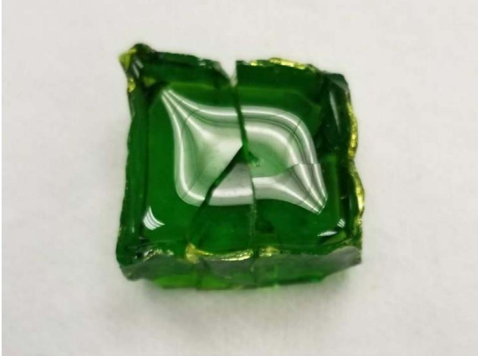
Figure F.2(b). Photograph of glass LAWPh3-02 after CCC heat treatment (top).
