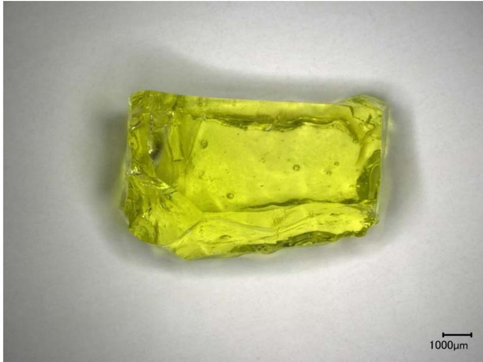
Figure F.13(a). Optical micrograph of glass LAWPh3-14 after isothermal treatment at 950°C for 24 h magnified 20X.
