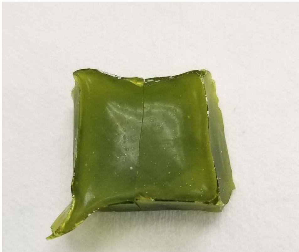
Figure F.3(b). Photograph of glass LAWPh3-03 after CCC heat treatment (top).
