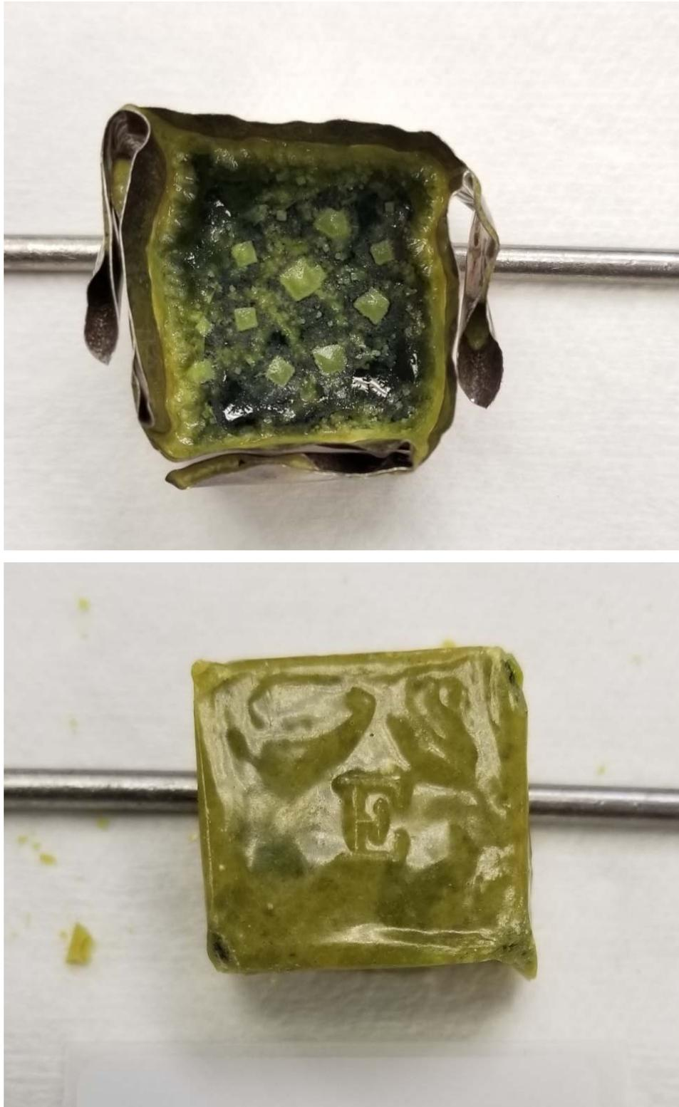
Figure F.16(b). Photograph of glass LAWPh3-17 after CCC heat treatment in crucible (top) and bottom out of crucible (bottom).
