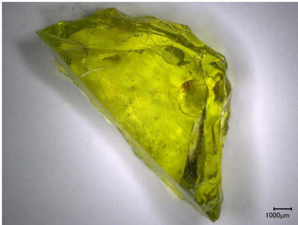
Figure F.1(a). Optical micrograph of glass LAWPh3-01 after isothermal treatment at 950°C for 24 h magnified 20X.
