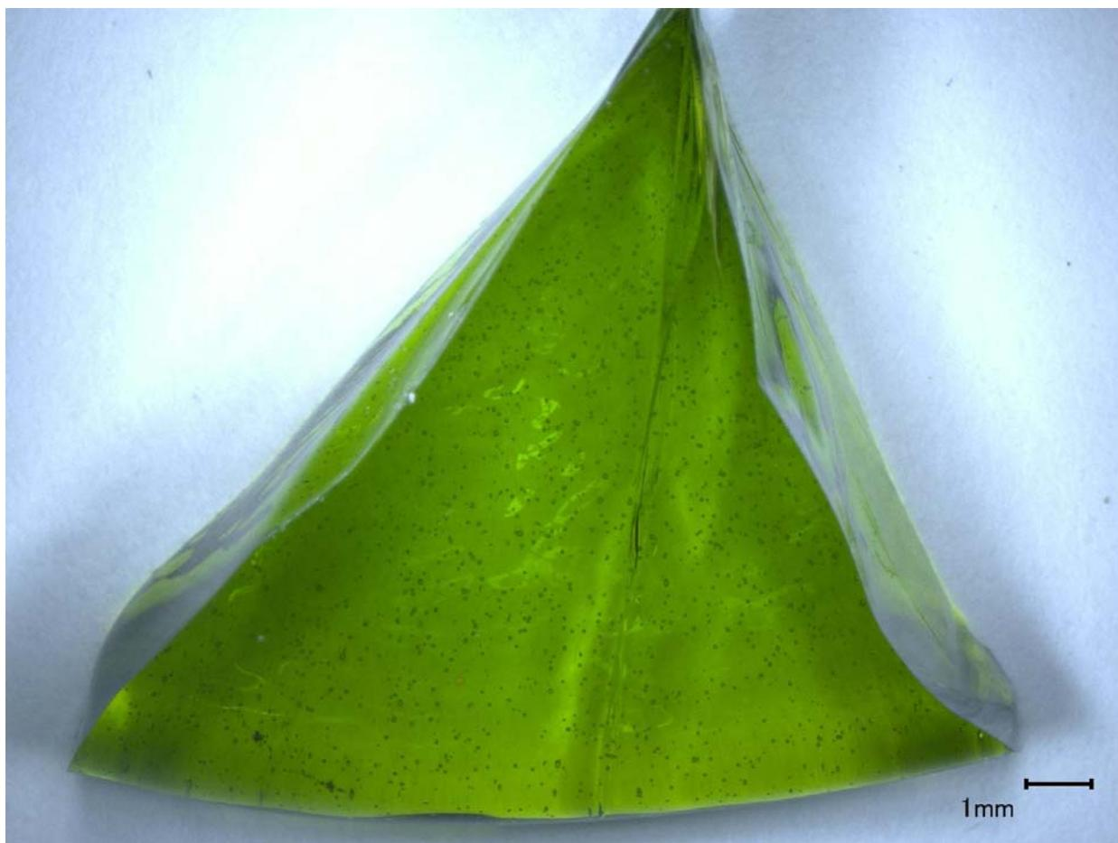
Figure A.11. Image of LAWPh3-12-Q, morphology of second melt at 1250°C for 1 h.
