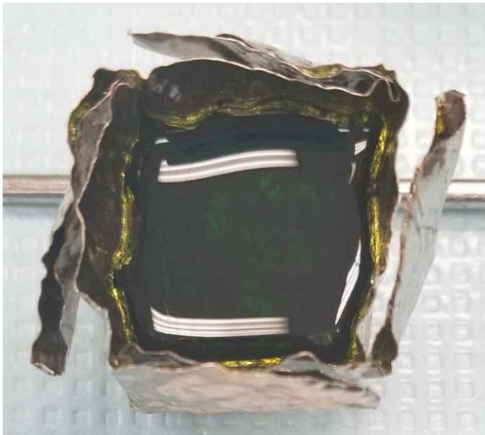
Figure F.18(b). Photograph of glass LAWPh3-20 after CCC heat treatment.
