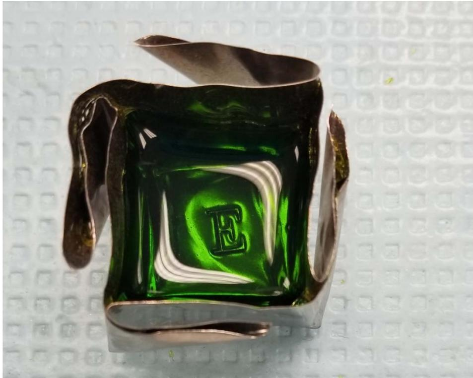
Figure F.10(b). Photograph of glass LAWPh3-11 after CCC heat treatment.
