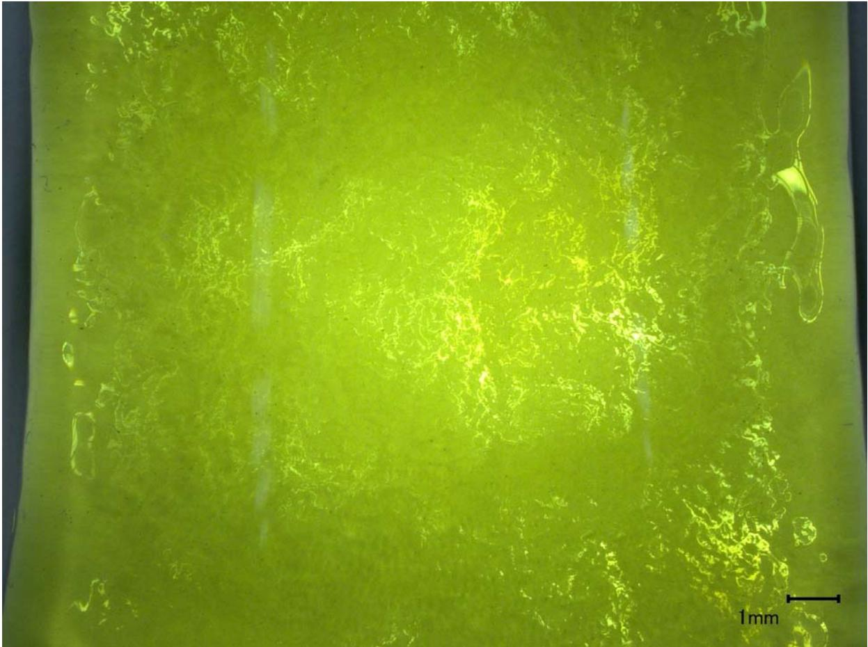
Figure A.8. Image of LAWPh3-09-Q, morphology of second melt at 1150°C for 1 h.
