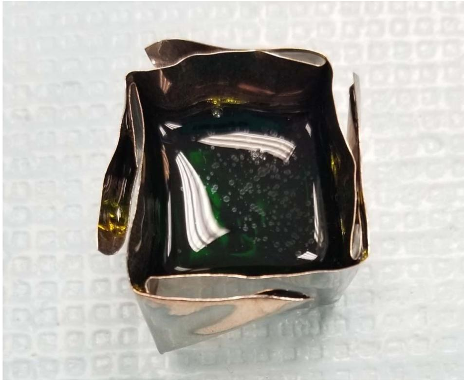
Figure F.11(b). Photograph of glass LAWPh3-12 after CCC heat treatment.
