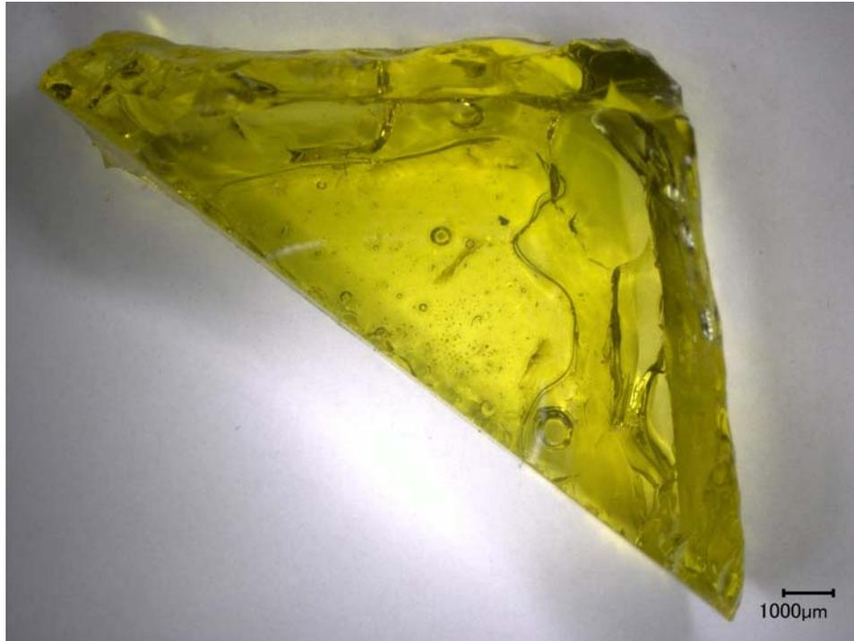
Figure F.3(a). Optical micrograph of glass LAWPh3-03 after isothermal treatment at 950°C for 24 h.
