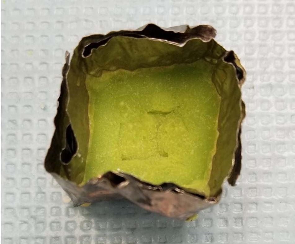
Figure F.12(b). Photograph of glass LAWPh3-13 after CCC heat treatment.
