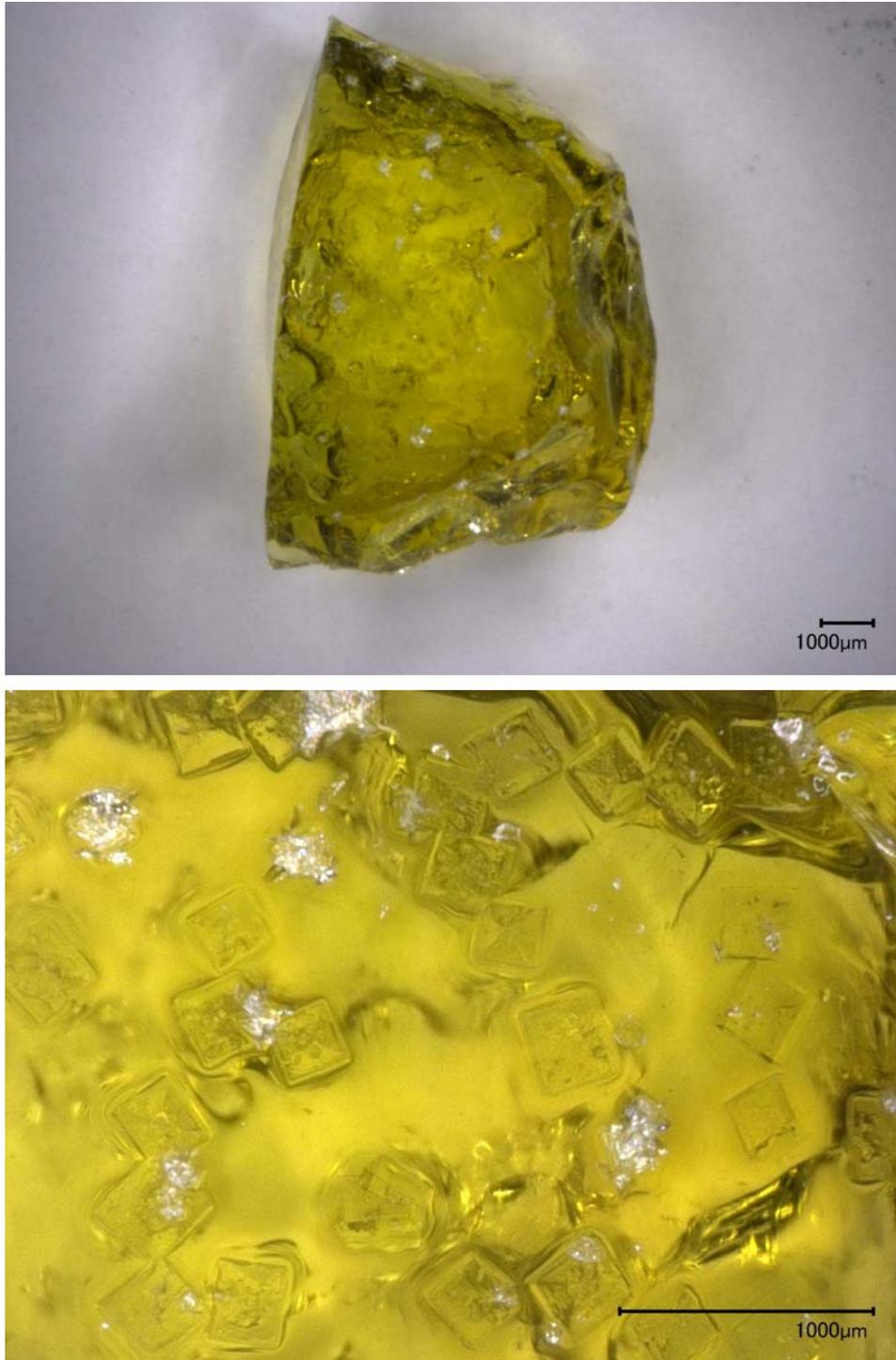
Figure F.16(a). Optical micrograph of glass LAWPh3-17 after isothermal treatment at 950°C for 24 h magnified 10X (top) and 100X (bottom).
