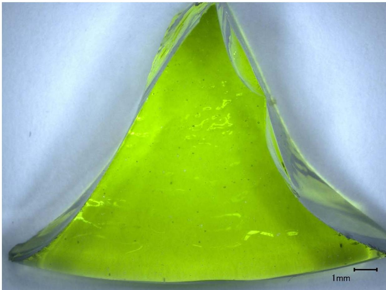
Figure A.17. Image of LAWPh3-18-Q, morphology of second melt at 1250°C for 1 h.
