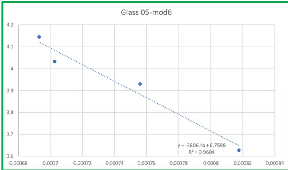
Figure E.4. Electrical conductivity data (ln(EC, S/m) versus inverse temperature in Kelvin) for LAWPh3-05\_mod6.
