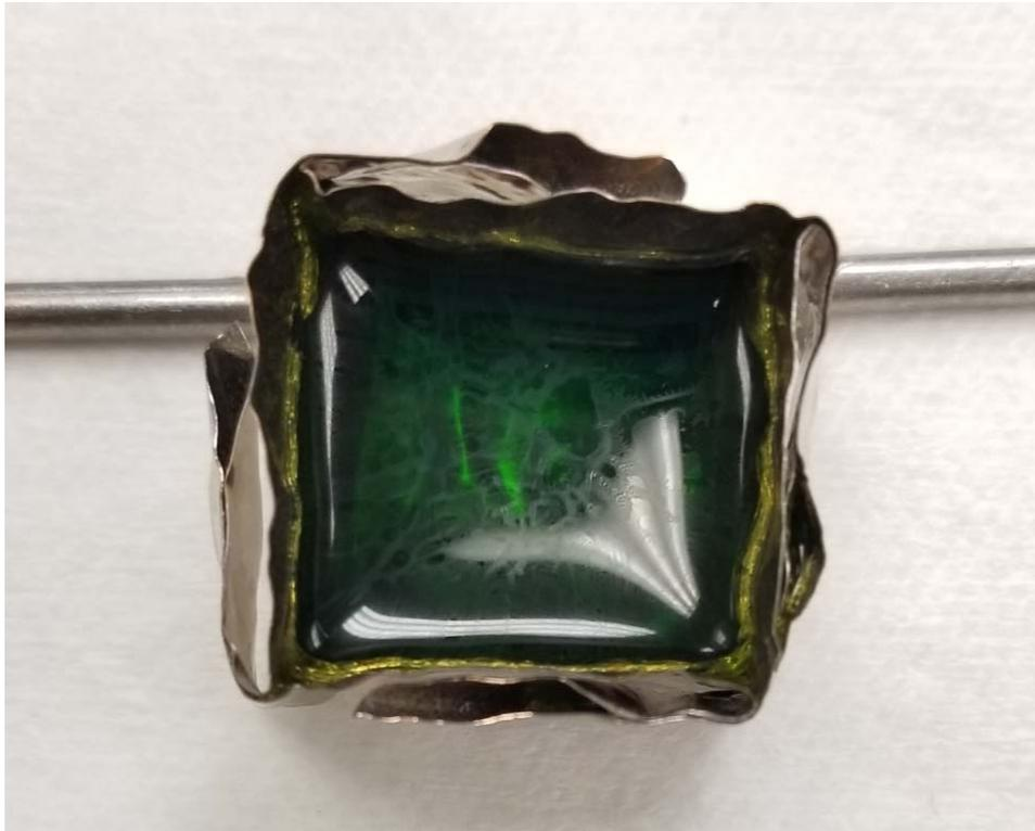
Figure F.17(b). Photograph of glass LAWPh3-18 after CCC heat treatment.
