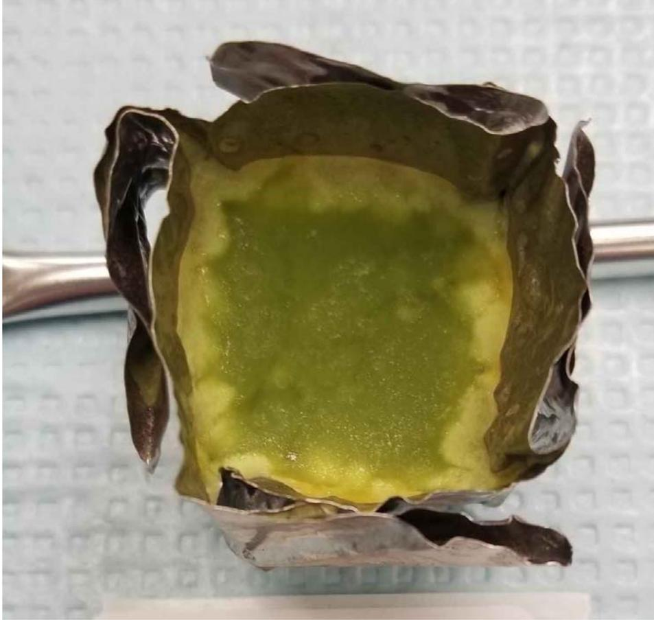
Figure F.8(b). Photograph of glass LAWPh3-09 after CCC heat treatment.
