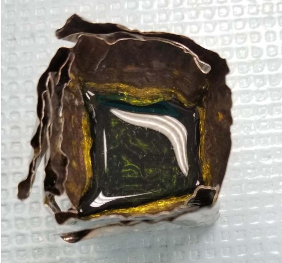
Figure F.14(b). Photograph of glass LAWPh3-15 after CCC heat treatment.
