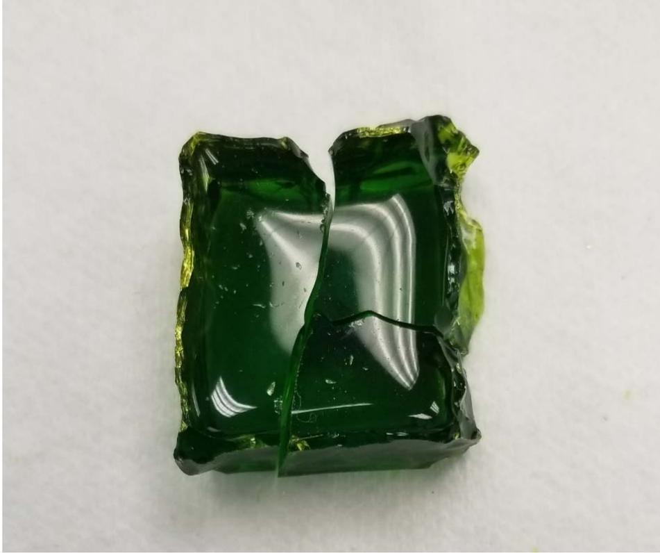
Figure F.4(b). Photograph of glass LAWPh3-04 after CCC heat treatment (top).
