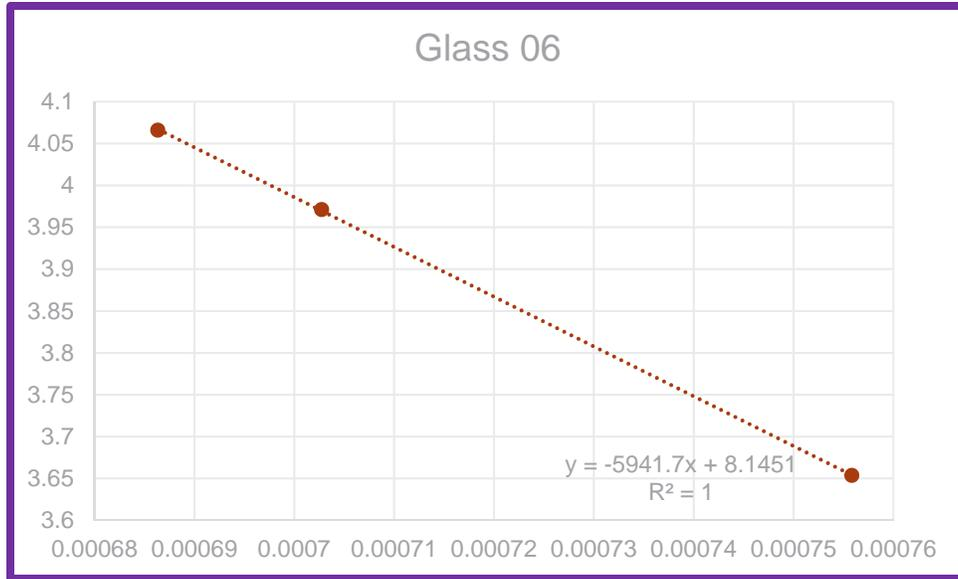
Figure E.5. Electrical conductivity data (ln(EC, S/m) versus inverse temperature in Kelvin) for LAWPh3-06.
