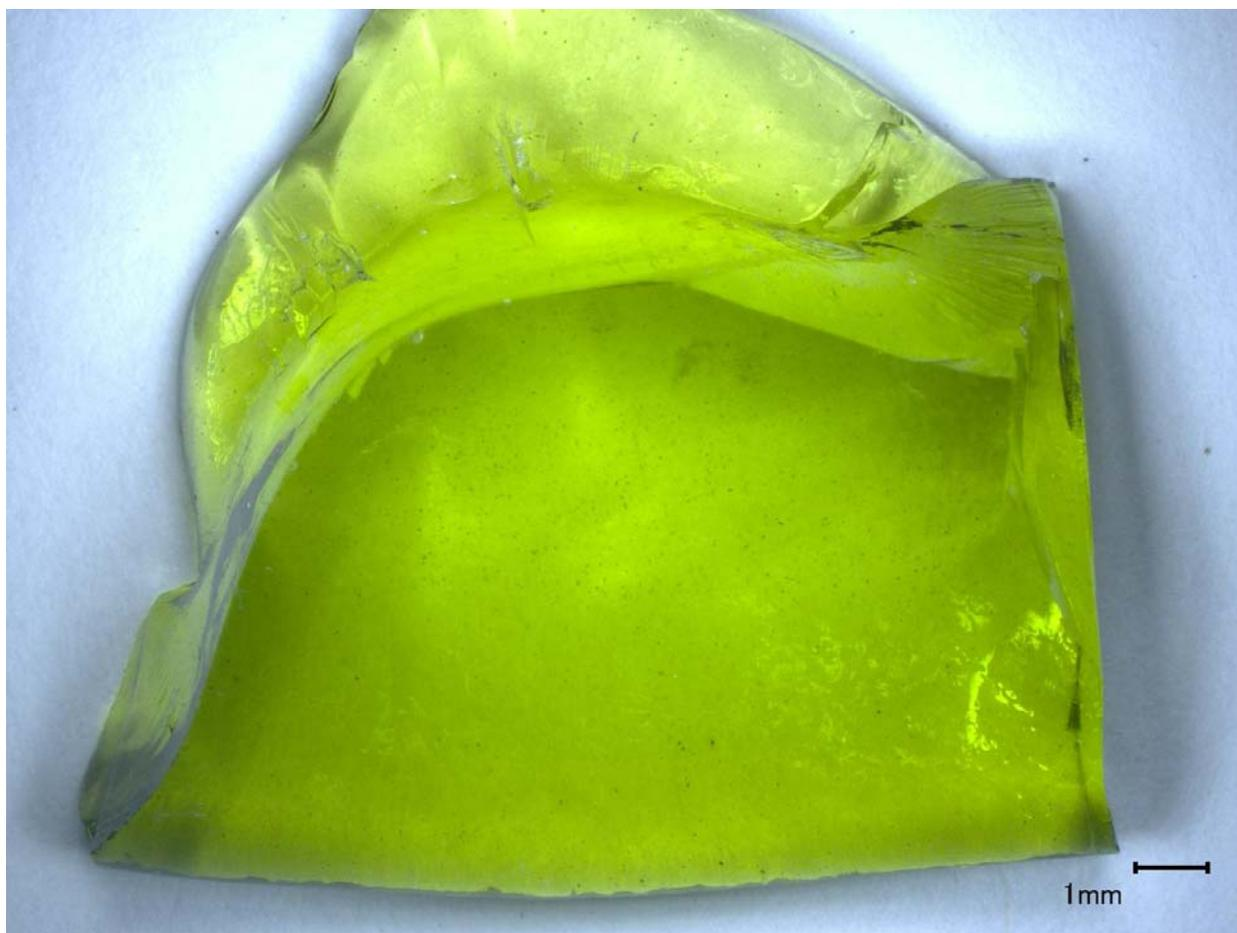
Figure A.16. Image of LAWPh3-17-Q, morphology of second melt at 1150°C for 1 h.
