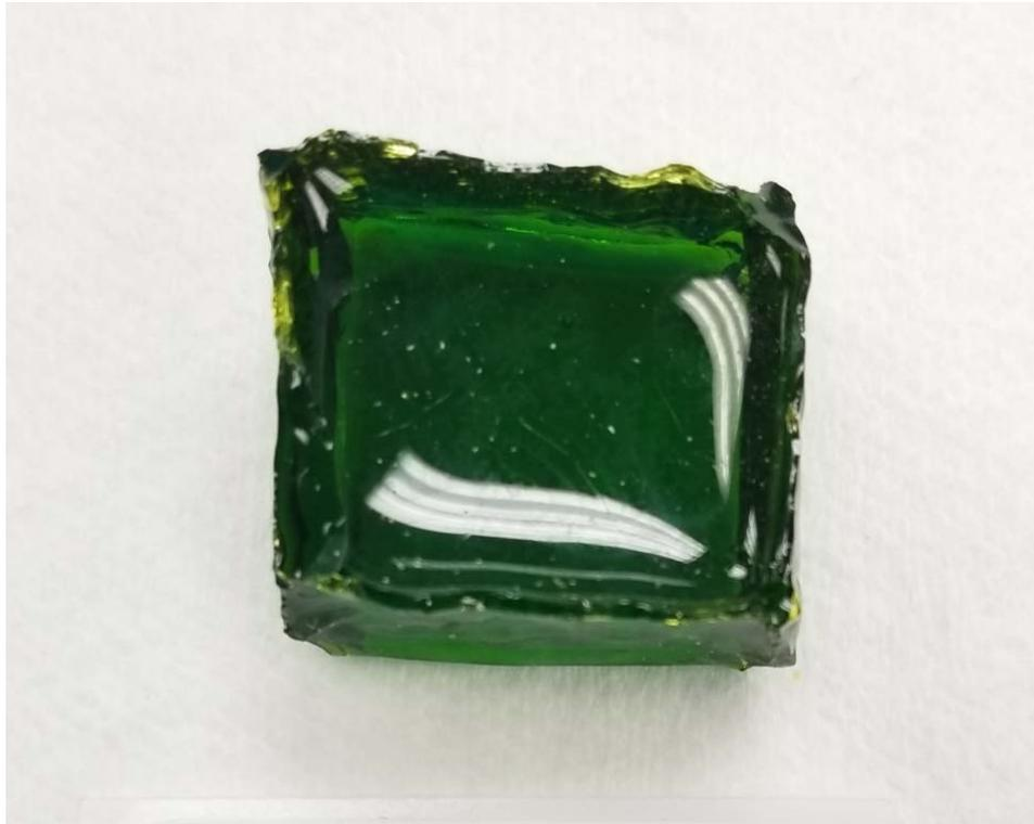
Figure F.1(b). Photograph of glass LAWPh3-01 after CCC heat treatment (top).
