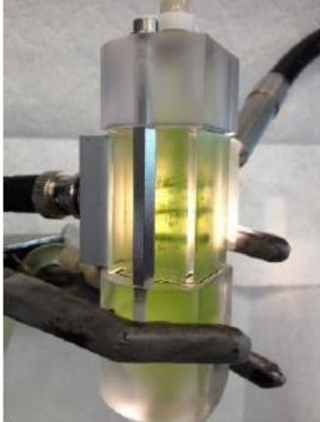
Ultrasonic Test System
