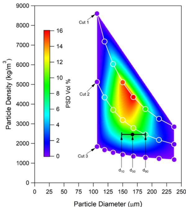
**Measured PSDD for Particle 2 from Flow Cell Test where Particles were Collected in Cuts 1-3 and Comparison to known Particle Density and Size (black line showing  $d_{10}$ ,  $d_{50}$ , and  $d_{90}$  at  $2460 \text{ kg/m}^3$ )**
