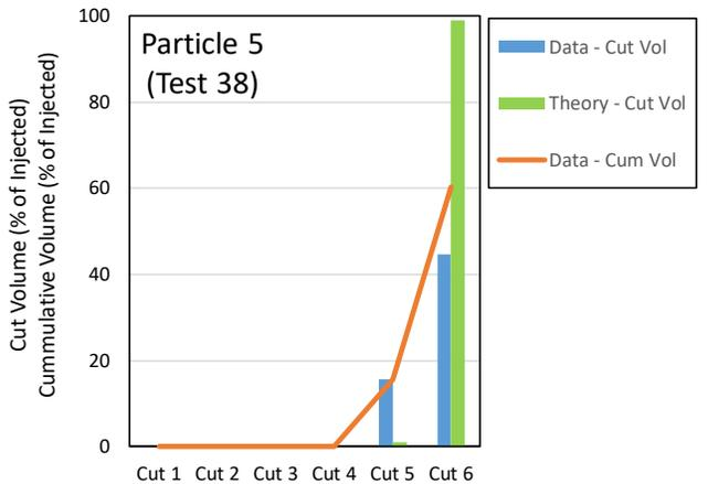
**Three Particles with Different Settling Rates Separating and being Collected in Different Cuts and Comparison to Theoretical Predictions**
