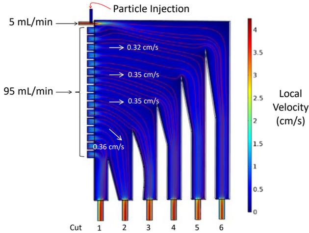
**COMSOL Predicted Streamlines and Centerline Velocities in the Flow Cell for a Flow of 100 mL/min**
