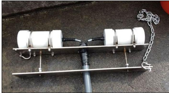
**Figure 2.6.** Direct-Mounted Underwater Balanced Loop-Vee Radio Antenna as Installed on Penstock Trash Racks at Foster
