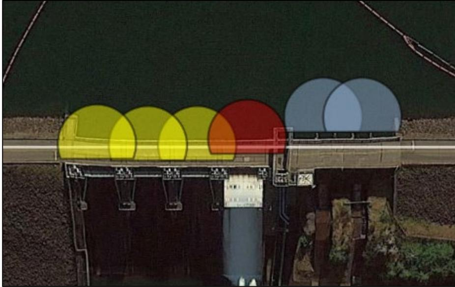
**Figure 2.8.** Approximate Detection Zone (70 ft) of Underwater Radio Telemetry Antennas Installed at Foster (yellow = Spill Bays 1–3; red = Fish Weir/Spill Bay 4; blue = Turbine Units 1–2)
