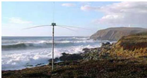
Figure 7. CODAR Ocean Sensors SeaSonde HF radar system in California.
