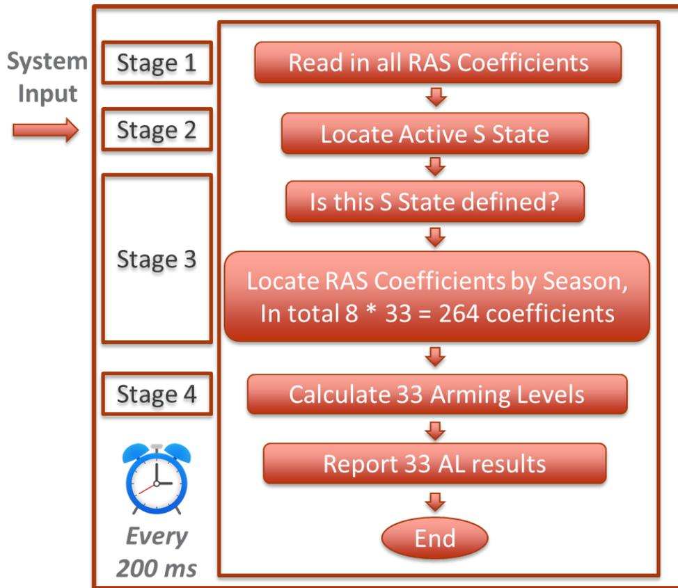
**Figure 2.** Flow chart illustrating the arming-level calculation logic for Jim Bridger RAS.
