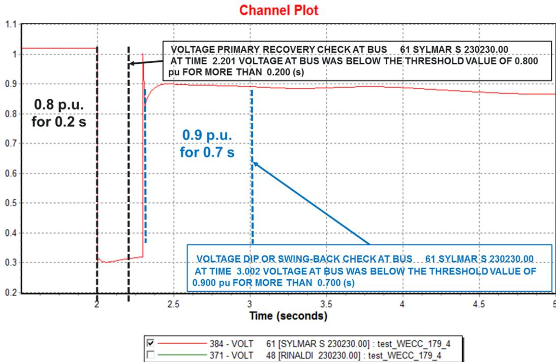
**Figure 21** An example for implementing WECC CRT-3 Criterion in TRAST based on PSS/E.
