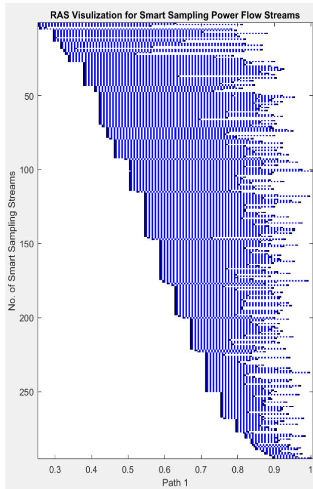
**Figure 17** An illustration of 295 stressing streams for further power system transient stability assessment. Blue block indicates a power flow case in the streams, and there is a black block (indicator of stream) before the first case and after the last case for each stream.
