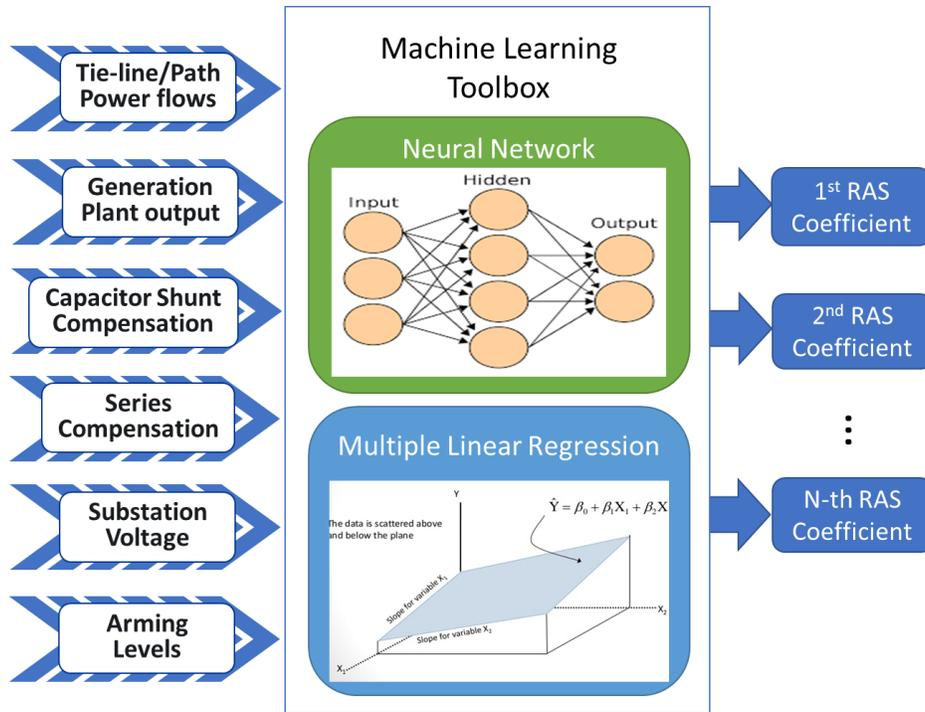
**Figure 22.** The machine learning framework for Jim Bridger RAS coefficient derivation in TRAST.
