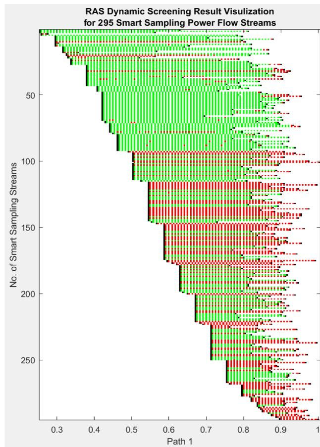
Figure 19 The pre-screening results of dynamic initialization for 295 Smart Sampling stressing streams. Green block indicates a power flow case passed the dynamic screening, and red block indicates a failed power flow case for dynamic simulation initialization. There is a black block (indicator of stream) before the first case and after the last case for each stream.
