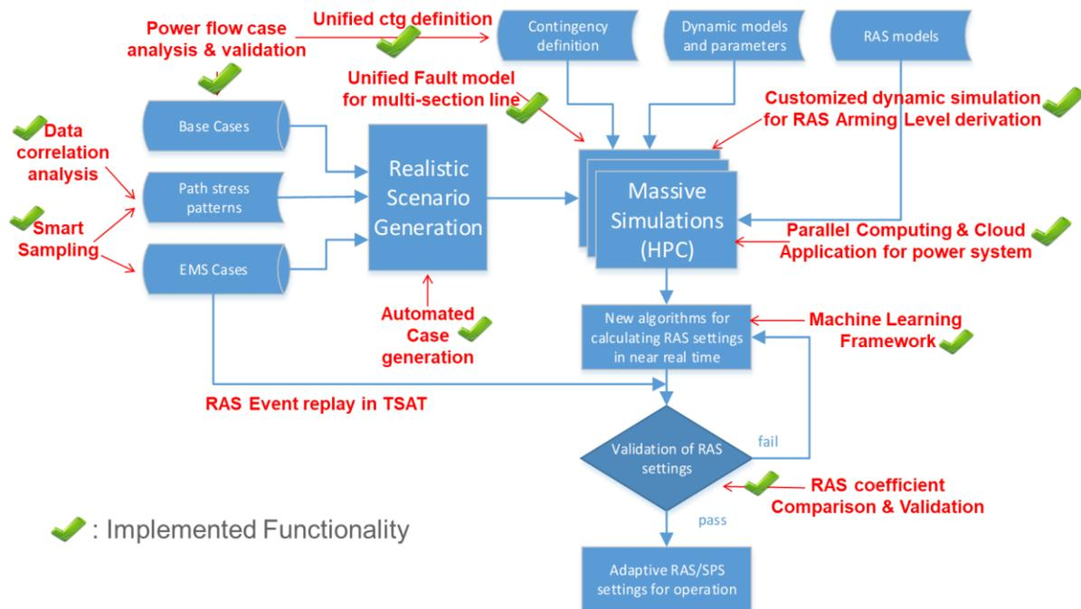
**Figure 4.** Overview of data-driven analytical functionalities in TRAST.
