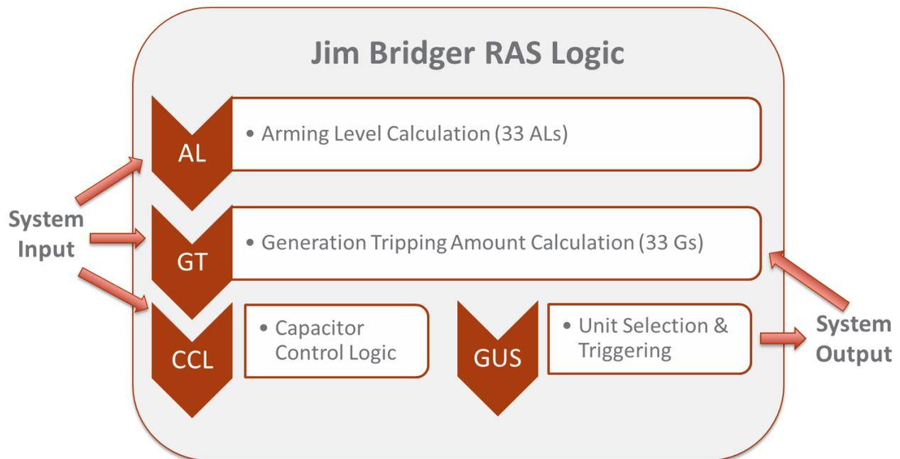
**Figure 1.** Flow chart illustrating the Jim Bridger RAS logic.
