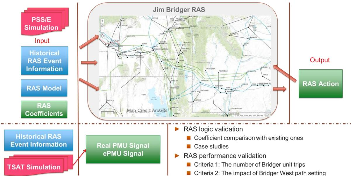
**Figure 27.** Data interface for RAS validation and evaluation in TRAST.
