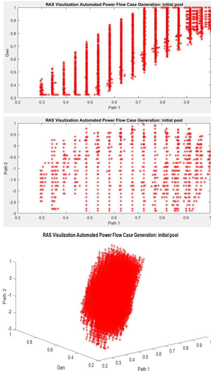
**Figure 15** An illustration of initial power flow case pool. The top figure shows the full distribution of one variable with Path1 in the initial power flow case pool, the middle figure shows another variable with Path1 in the initial power flow case pool, the bottom figure shows a 3-D plot for three variables.
