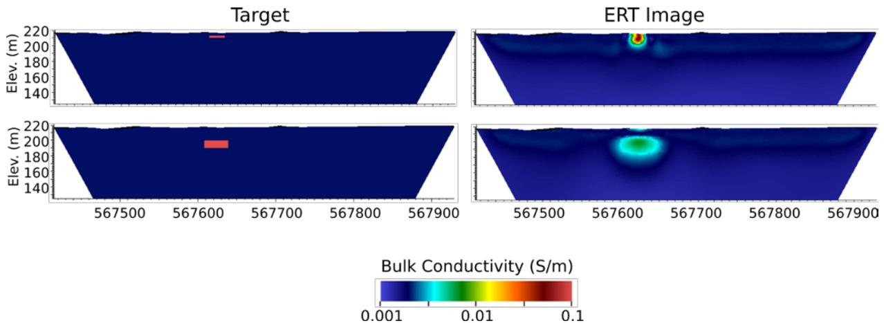
Figure 7. Synthetic imaging example demonstrating the effects of limited resolution.
