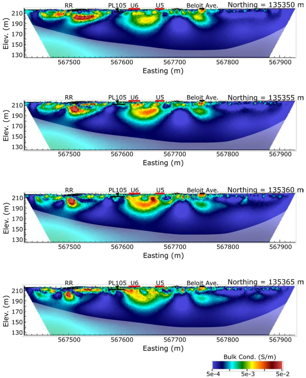
Figure 9. Northing-normal ERT image cross-sections from northing 135350 m to 135365 m.
