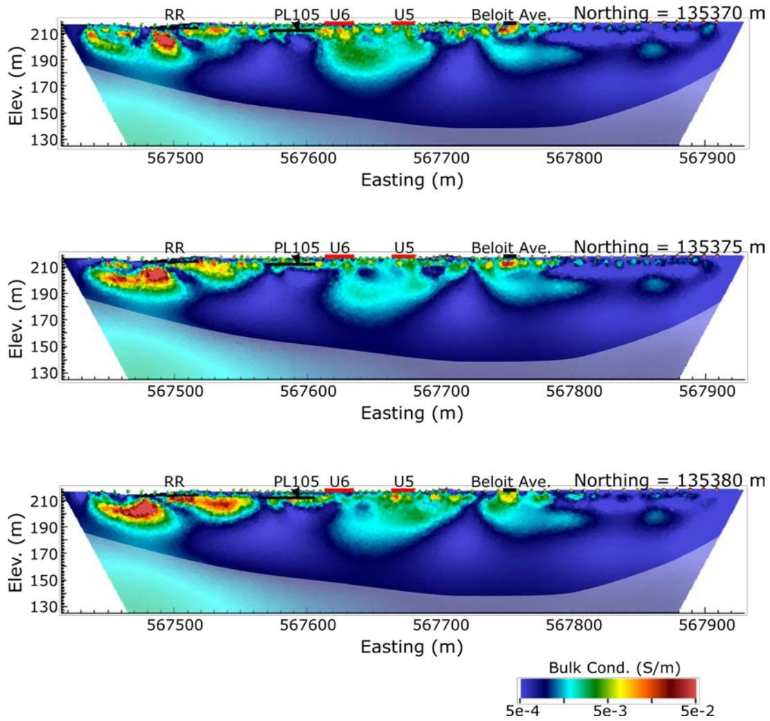
Figure 10. Northing-normal ERT image cross-sections from northing 135370 m to 135380 m.
