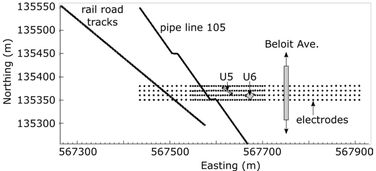
Figure 6. Plan view of electrode layout with respect to 216-U-5 and 216-U-6 cribs and buried metallic infrastructure (i.e., railroad tracks and waste transfer pipeline 200-W-105-PL).
