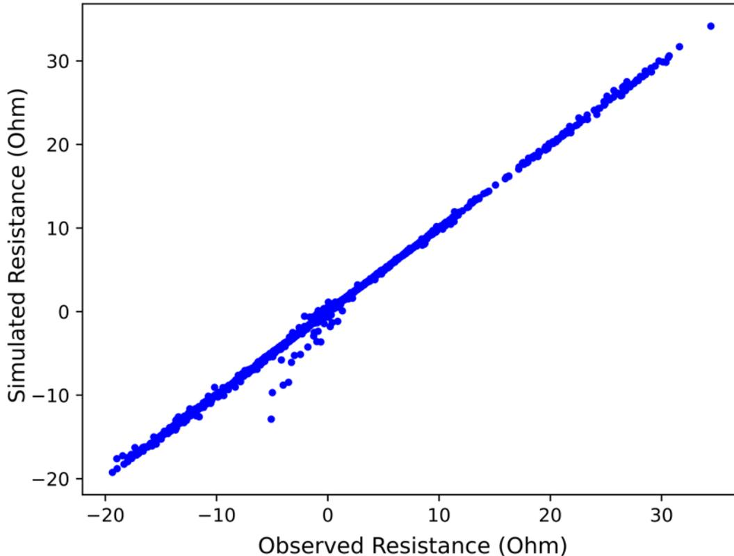
Figure 8. Simulated ERT vs. observed ERT data for each of the 11,944 measurements.
