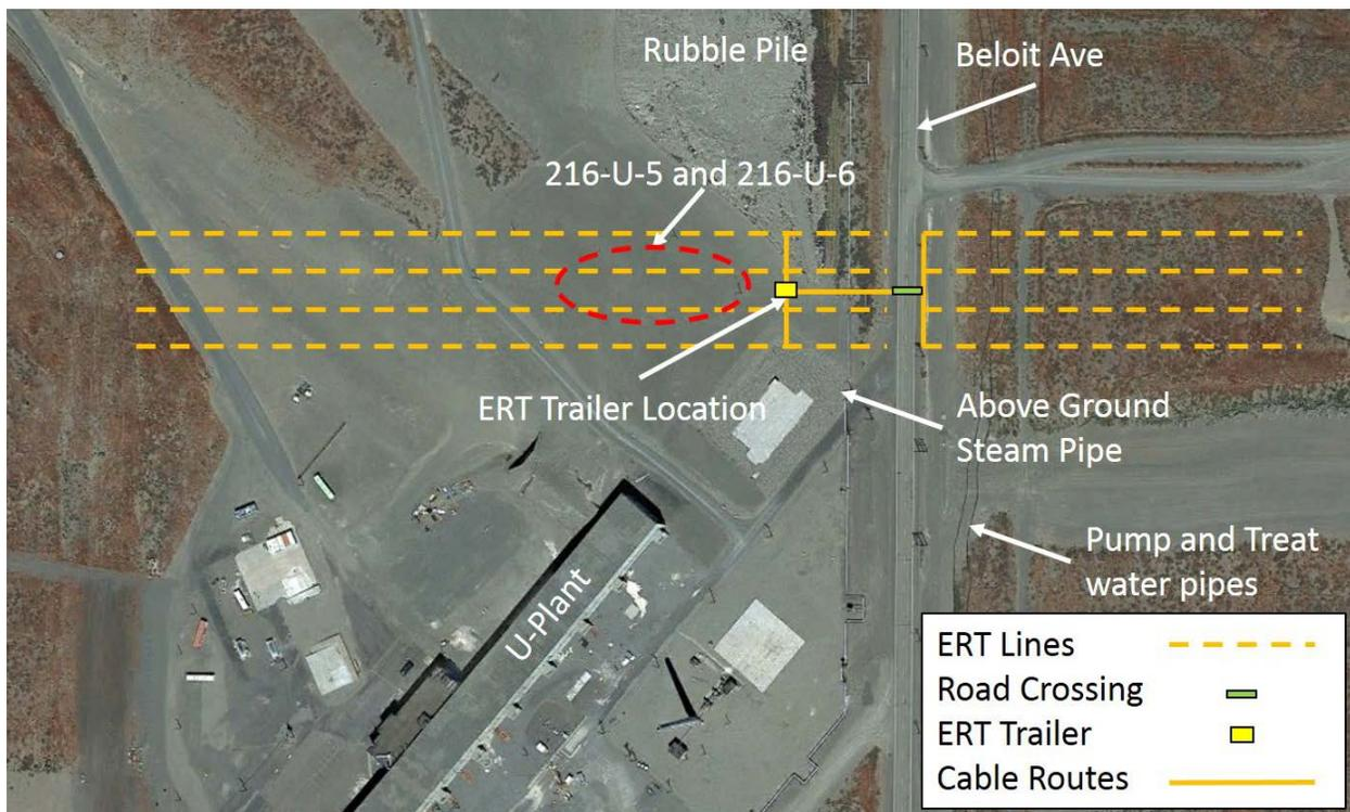
Figure 4. Location of ERT trailer, electrode lines, and cable routing at the survey site.
