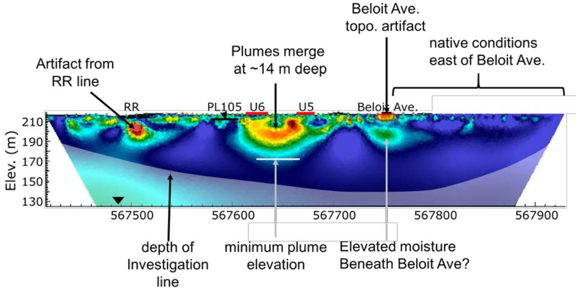
Figure 13. Summary results of 216-U-5 and 216-U-6 electrical resistivity tomography imaging.
