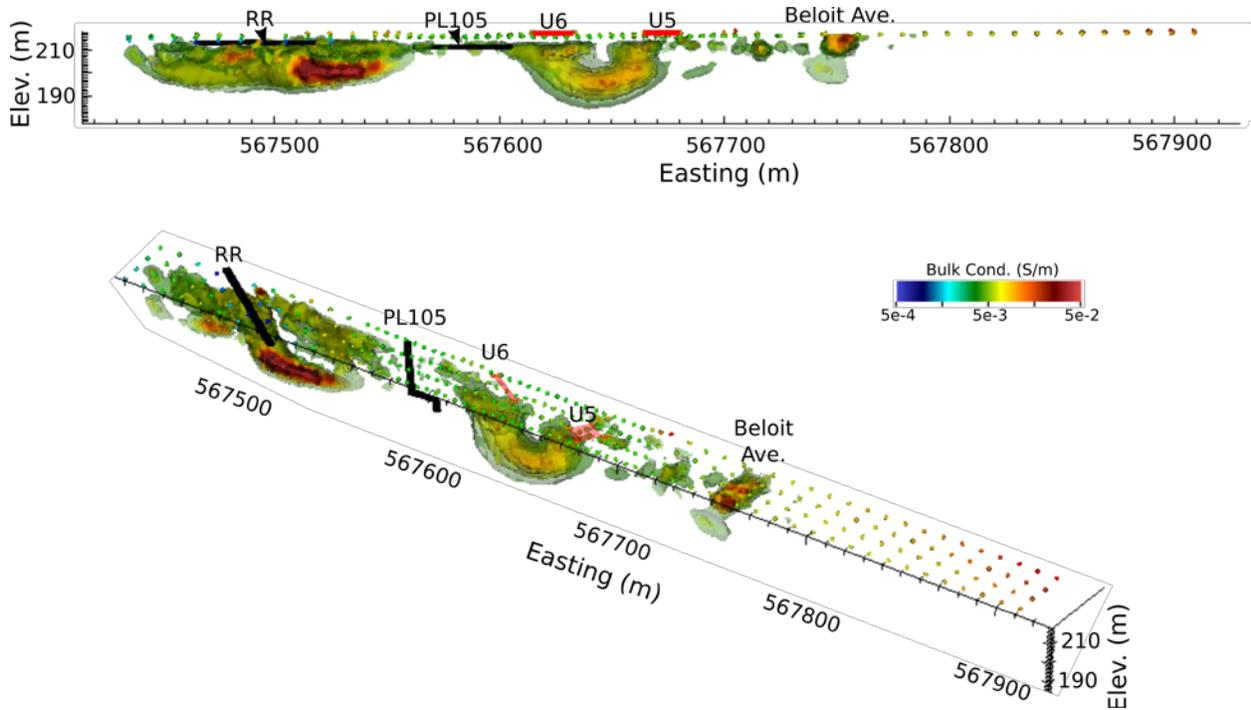
Figure 12. Iso-surface representations of bulk conductivity anomalies show the estimated three-dimensional extent of U5 and U6 vadose zone plumes. Anomalies associated with Beloit Avenue and the buried 221-U railroad tracks are also evident.
