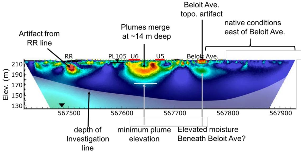
Figure S.1. Summary results of 216-U-5 and 216-U-6 electrical resistivity tomography imaging.
