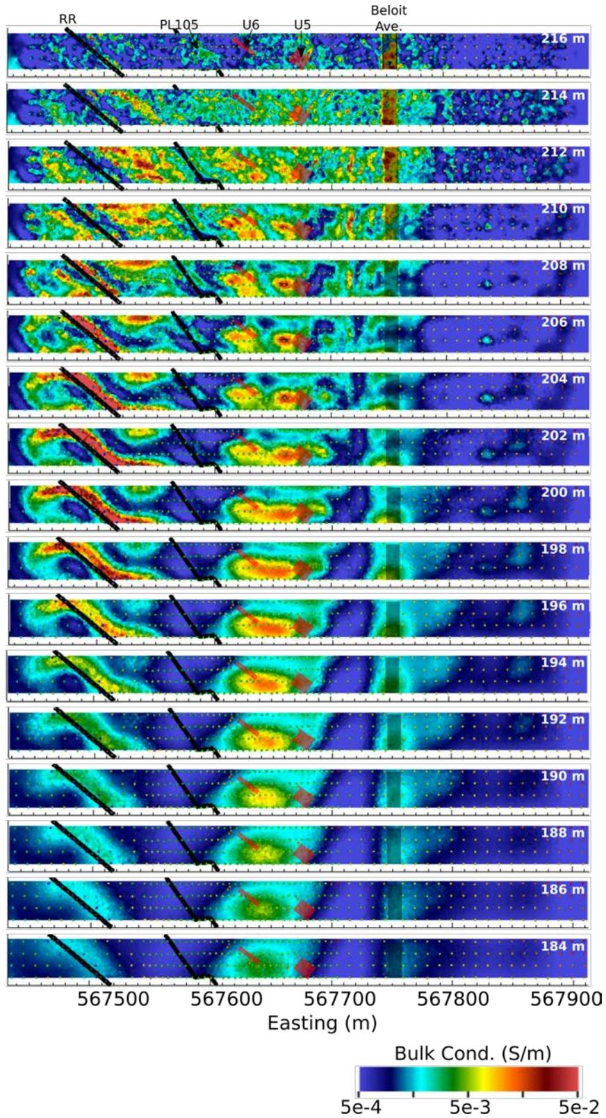
Figure 11. ERT depth cross-sections from ground surface (~216 m) to 184 m elevation.
