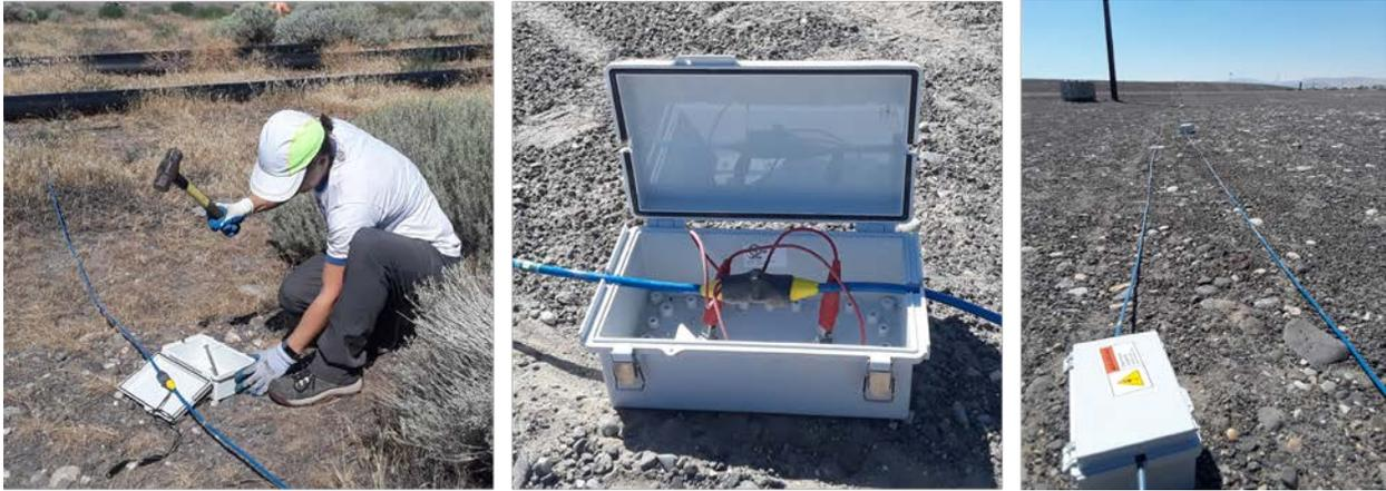
Figure 5. Electrode installation detail: (left) installation of two 10-inch- long steel spikes through the bottom of the electrical isolation box; (middle) multi-conductor electrode cable attached to electrodes in isolation box; (right) final configuration showing electrode isolation boxes and ERT cables.
