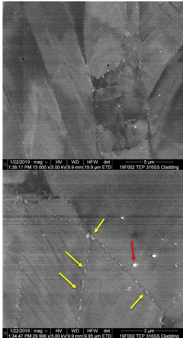
Figure 4. The yellow arrows point to fine carbides located on each grain boundary in the coated cladding welded to the end plug cap. The bright spots (red arrow) are colloidal silica particles that didn't rinse off.
