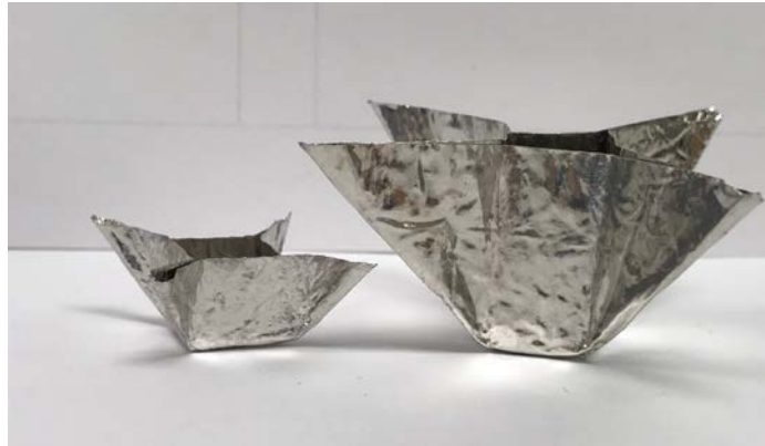
Figure 13. Standard and taller platinum boats used in the current study for 48-h heat treatments at 1200°C for AmCm2-19.
