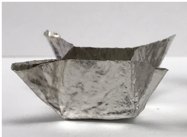
Figure 3. Pt/10%Rh boat used for heat treatments.
