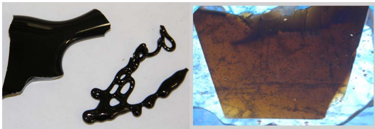
Figure 1. ARG-1 air quenched glass (left) and thin slice for OM observation (right).
