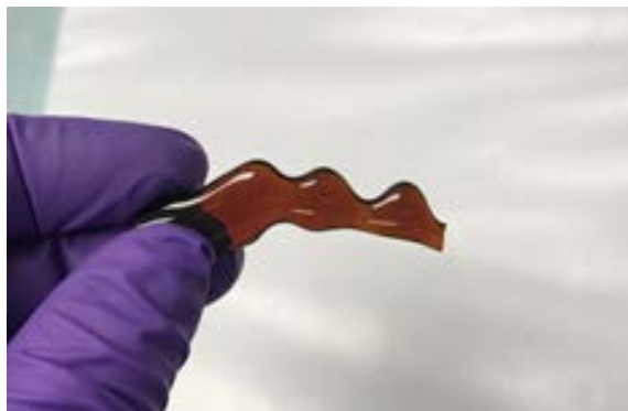
Figure 2. AmCm2-19 glass after the second melt.
