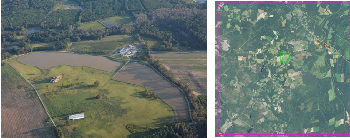
Figure 31. Example CAP image similarity matching. Pink square = extent of NAIP image chipping; Green triangle point = CAP photo/aircraft location; Green polygon = approximate true ground extent; Orange points = "similar" NAIP chips; Yellow cross = triangulated centroid.
