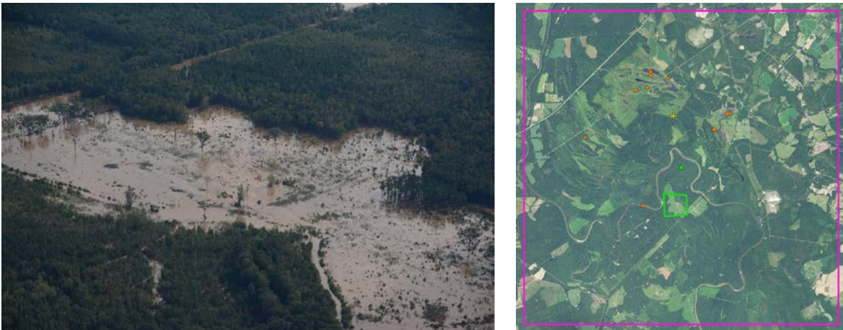
Figure 30. Example CAP image similarity matching. Pink square = extent of NAIP image chipping; Green triangle point = CAP photo/aircraft location; Green polygon = approximate true ground extent; Orange points = "similar" NAIP chips; Yellow cross = triangulated centroid.
