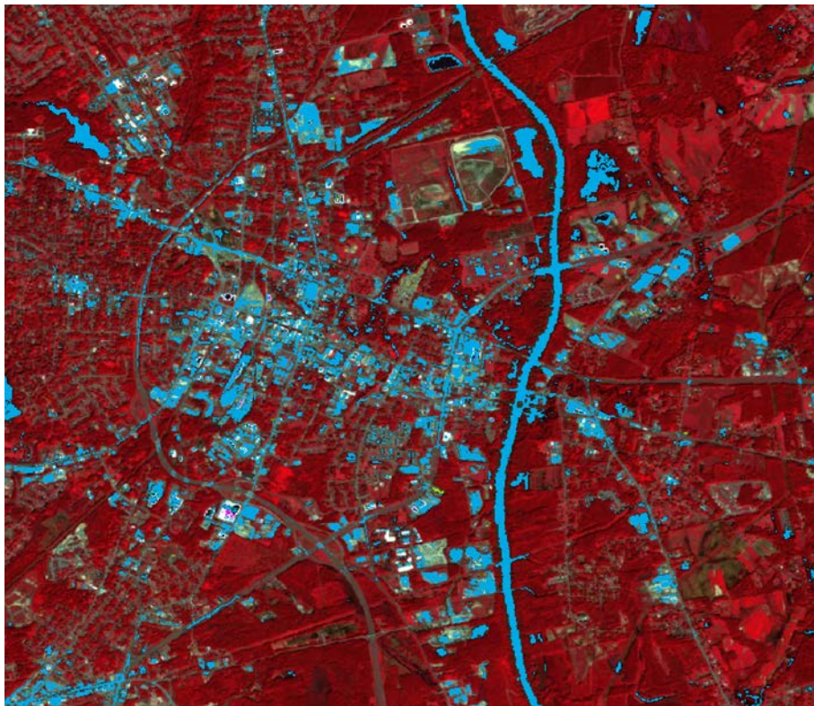
Figure 4. Example flood detection (blue) from multispectral satellite image over Fayetteville, North Carolina during Hurricane Florence, (September 17, 2018).
