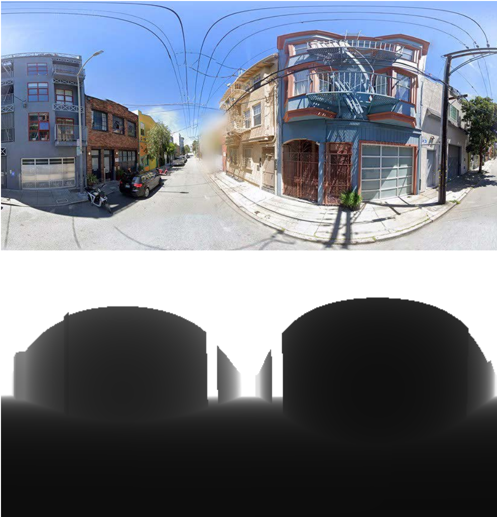
Figure 35. Google StreetView images including a panoramic view (top) and the associated distance map (bottom) that is retrieved and processed.
