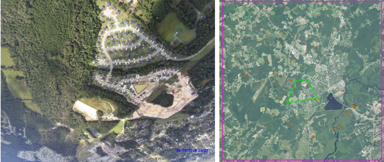
Figure 29. Example CAP image similarity matching. Pink square = extent of NAIP image chipping; Green triangle point = CAP photo/aircraft location; Green polygon = approximate true ground extent; Orange points = "similar" NAIP chips; Yellow cross = triangulated centroid.
