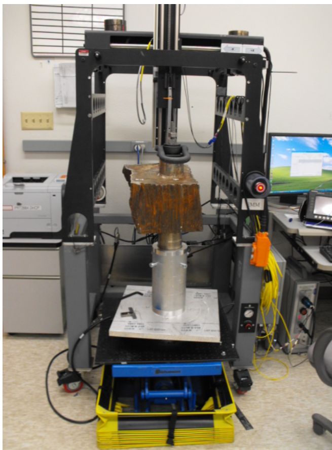
Figure 4.4. Translation Stage Capable of Motion in Four Axes (X, Y, Z, rotation) Used for Examining Specimens in this Study
