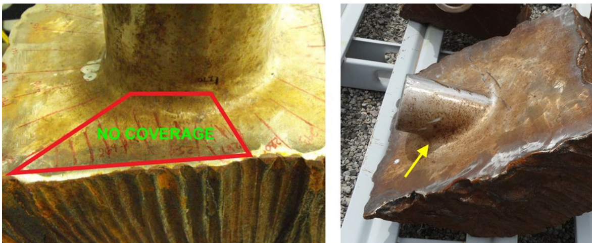
Figure 4.9. Example of Regions with Limited or No Examination Access Due to the Curvature of the Inside Surface of the RPV Head that Occurs Downhill from the Top-Center of the RPV Head
