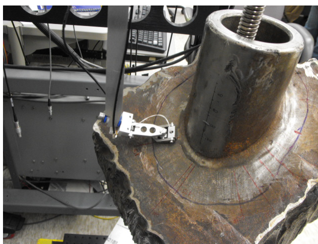
Figure 4.7. Photo Showing CRDM Nozzle Examination Region from the Edge of Cladding, Indicated by Black Line, up to the J-groove Weld
