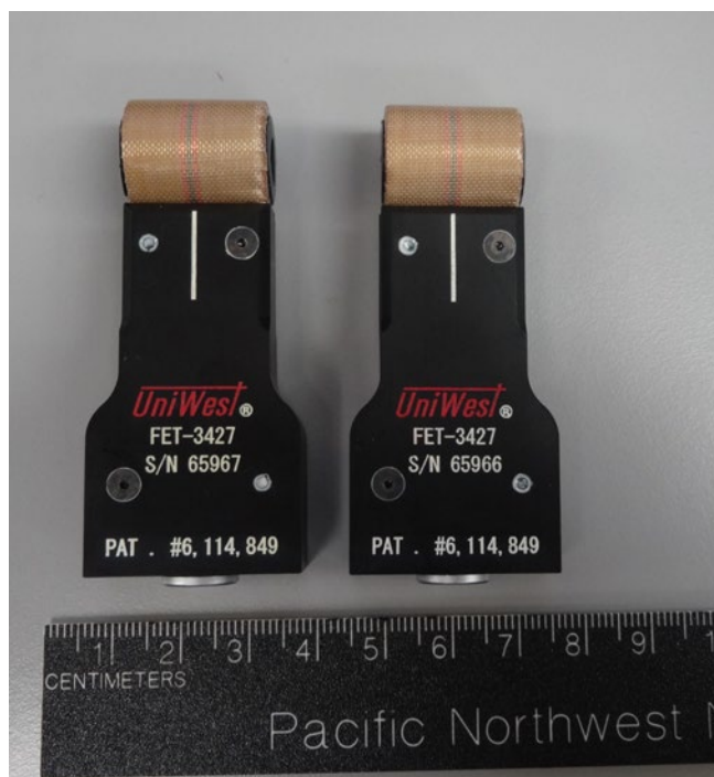
Figure 4.2. Flex Probe with Coils Wound in the Circumferential Direction
