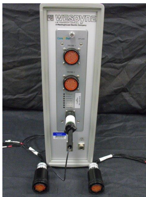
Figure 4.6. WesDyne IntraSpect Eddy Current Examination System
