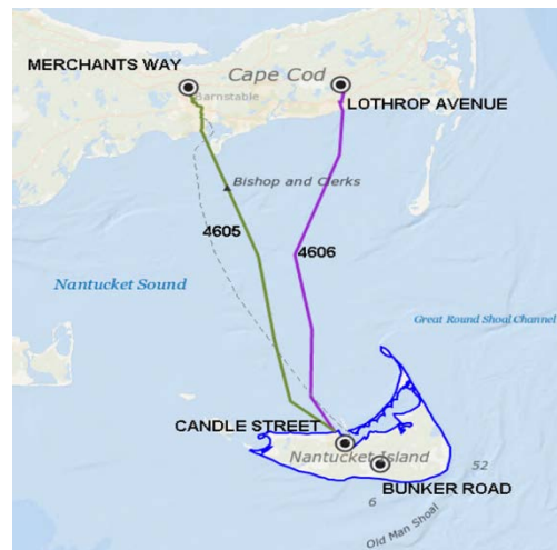
Figure 3.2. Two Supply Cables Connecting Massachusetts to Nantucket Island
