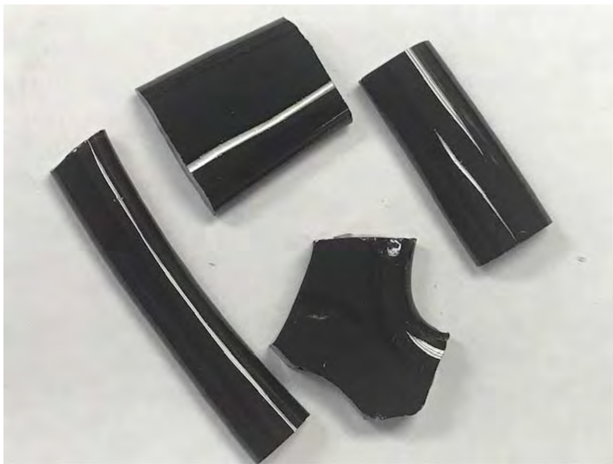
Figure A.2. Photograph of glass CST19-02 after melting three times at 1150°C.
