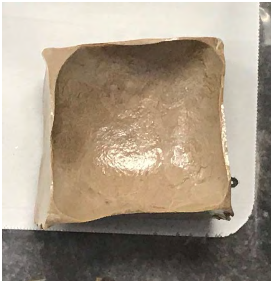
Figure D.1. Photograph of glass CST19-01 after being held at 950°C for 24 hours.
