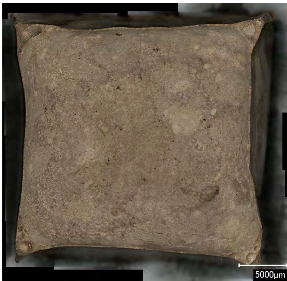
Figure B.2. Optical micrograph of glass CST19-01 after CCC beginning at 1150°C.
