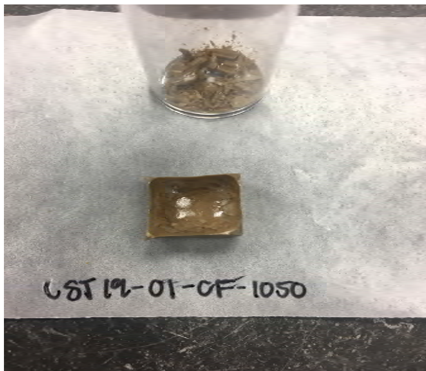
Figure D.2. Photograph of glass CST19-01 after being held at 1050°C for 24 hours.
