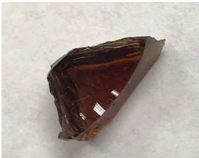
Figure D.7. Photograph of glass CST19-04 after being held at 950°C for 24 hours.
