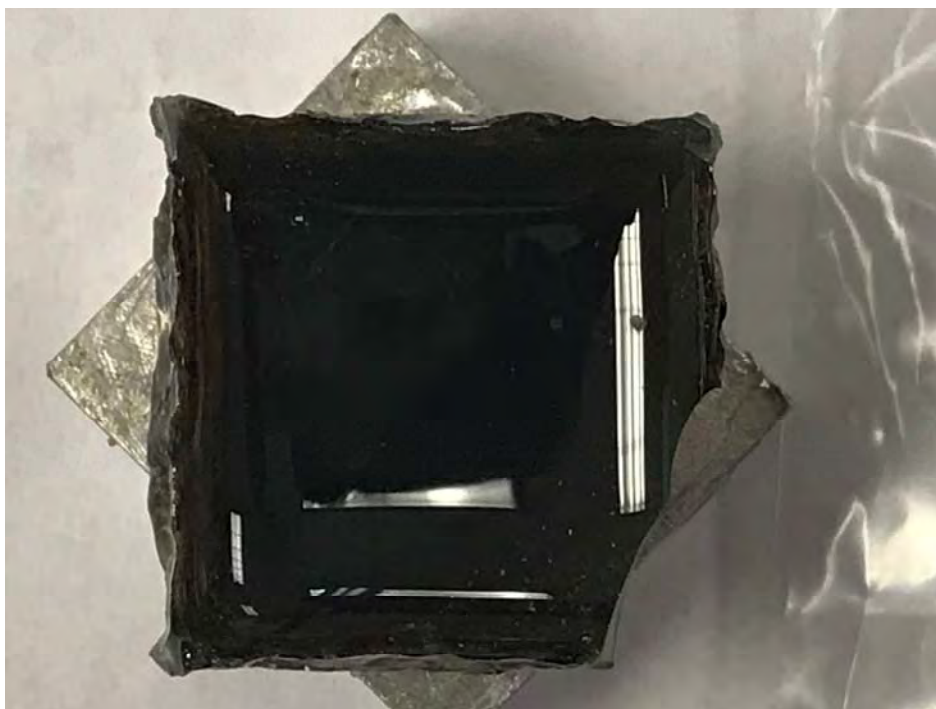
Figure B.7. Photograph of glass CST19-CST-04 after CCC beginning at 1150°C.
