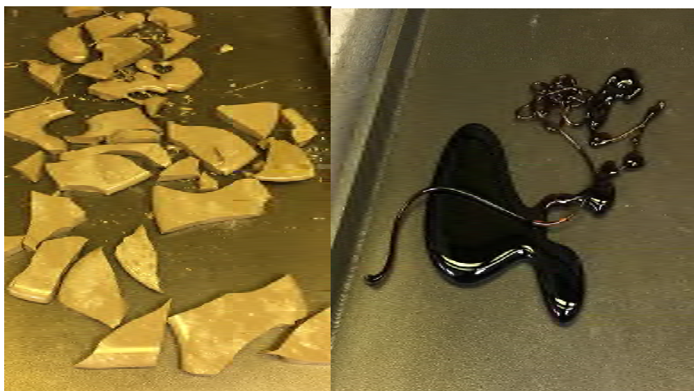
Figure 2.1. Glass CST19-01 after melting at 1150°C for 1 hour (left) and at 1250°C for 2 hours (right).
