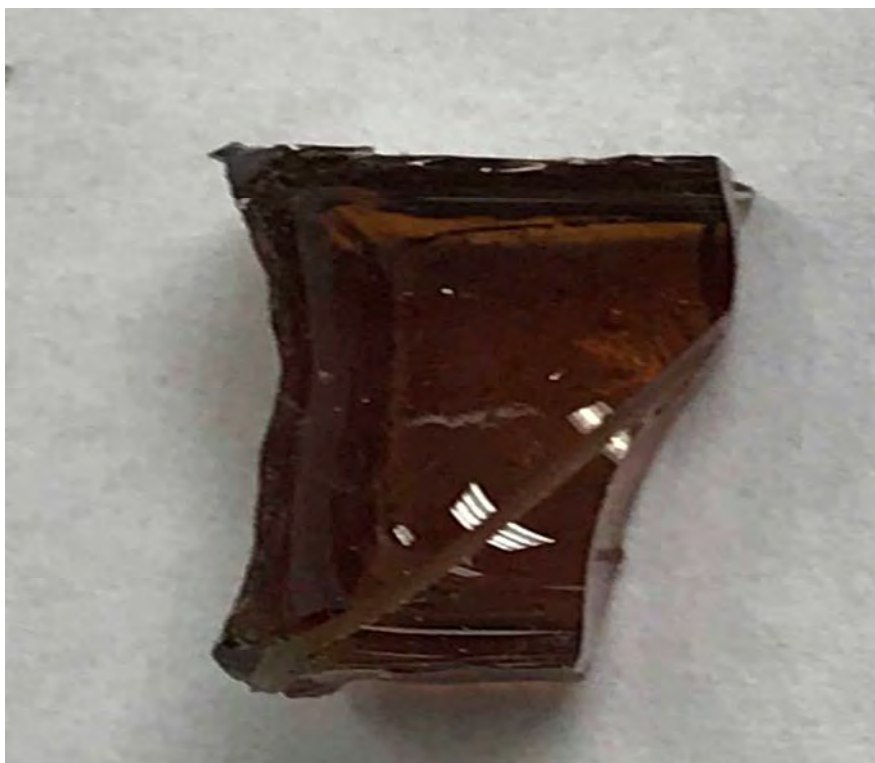
Figure D.8. Photograph of glass CST19-04 after being held at 1050°C for 24 hours.
