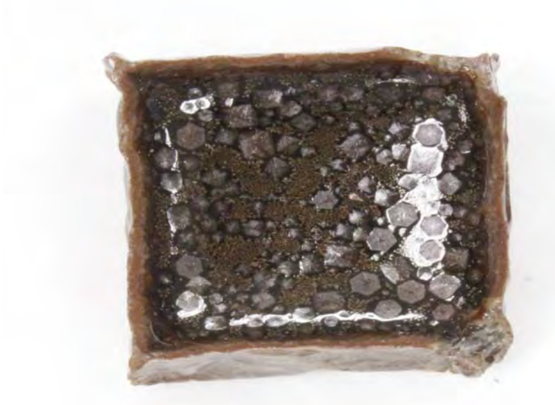
Figure B.5. Photograph of glass CST19-03 after CCC beginning at 1150°C.
