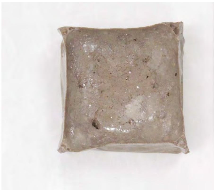
Figure B.1. Photograph of glass CST19-01 after CCC beginning at 1150°C.
