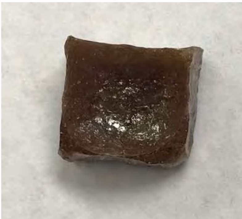
Figure D.6. Photograph of glass CST19-04 after being held at 850°C for 24 hours.
