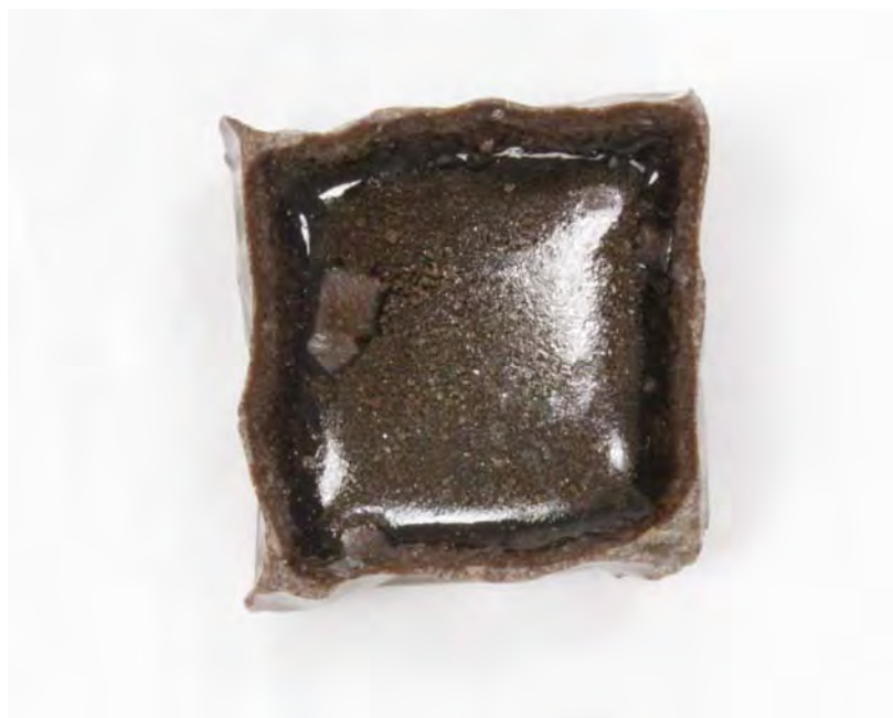
Figure B.3. Photograph of glass CST19-02 after CCC beginning at 1150°C.
