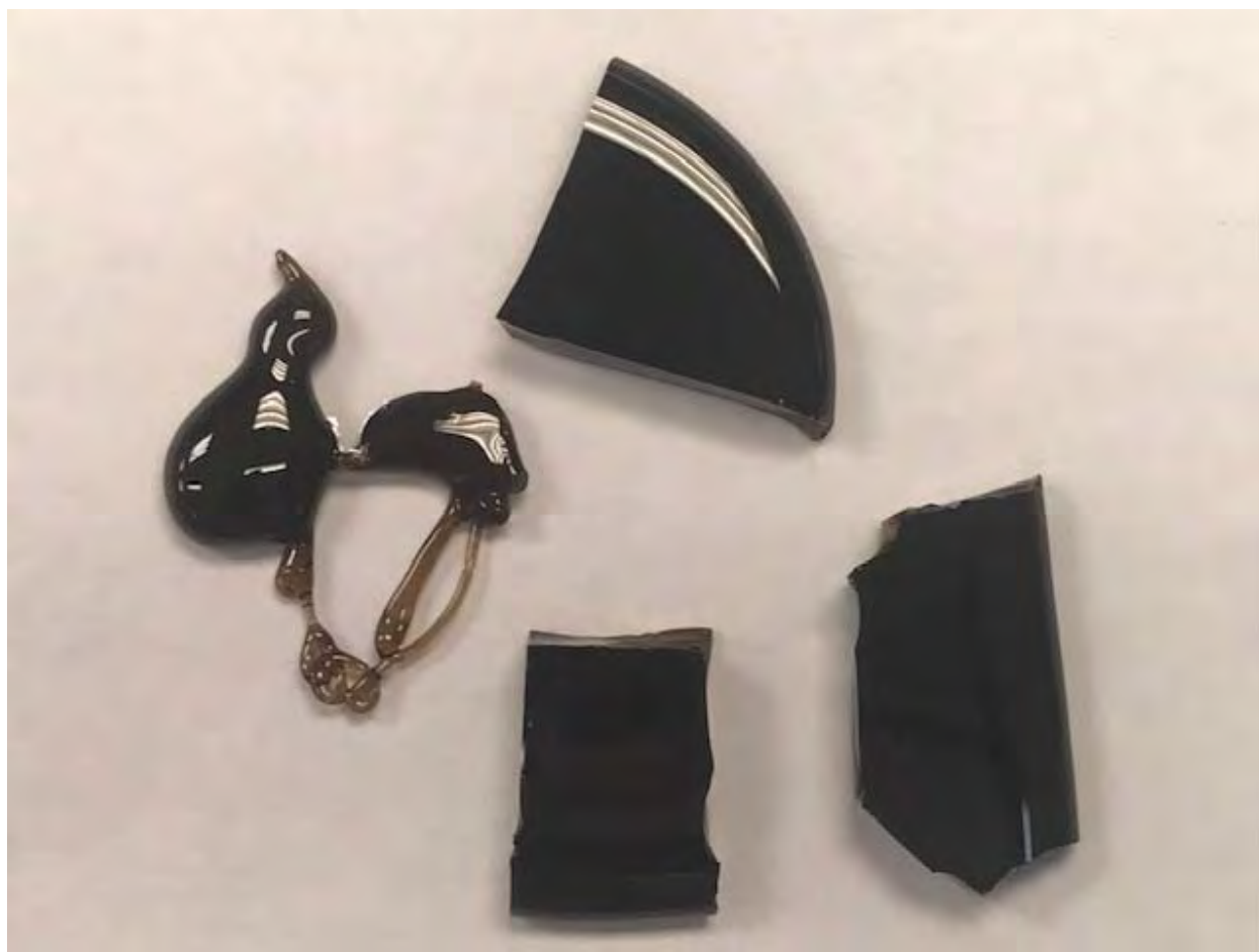
Figure A.3. Photograph of glass CST19-03 after melting twice at 1150°C.
