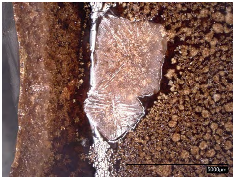
Figure B.4. Optical micrograph of glass CST19-02 after CCC beginning at 1150°C.
