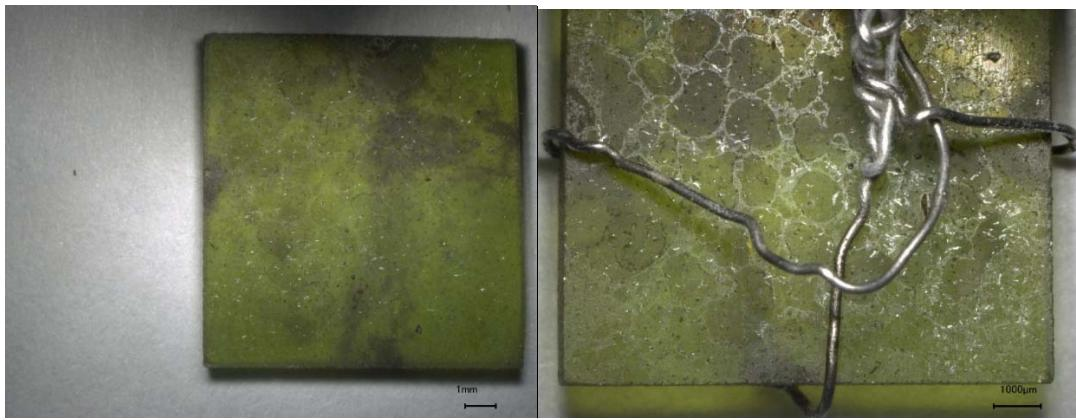
a) Glass square magnified 20X after VHT; b) Glass surface magnified 30X after VHT
