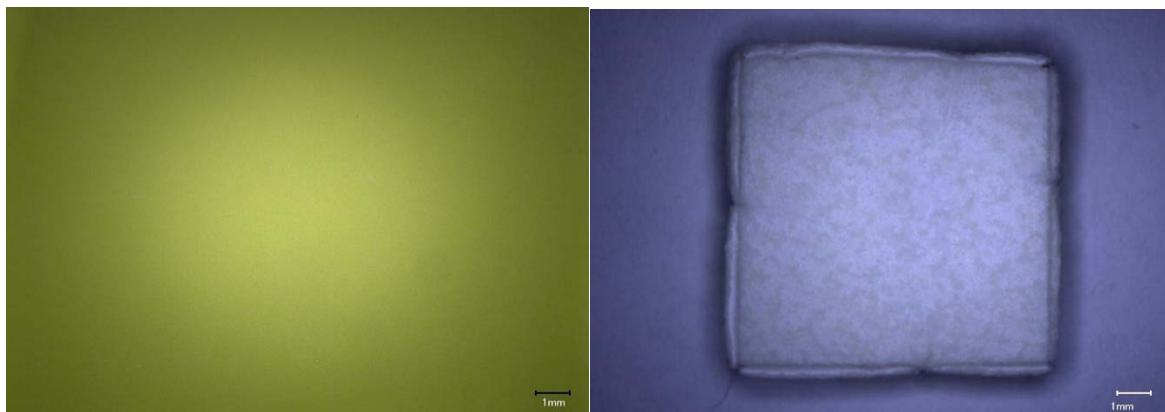
a) Glass square magnified 20X before VHT; b) Glass square magnified 20X after VHT
