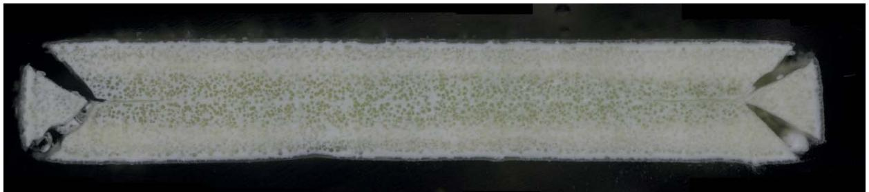
b) Glass cross section magnified after VHT
