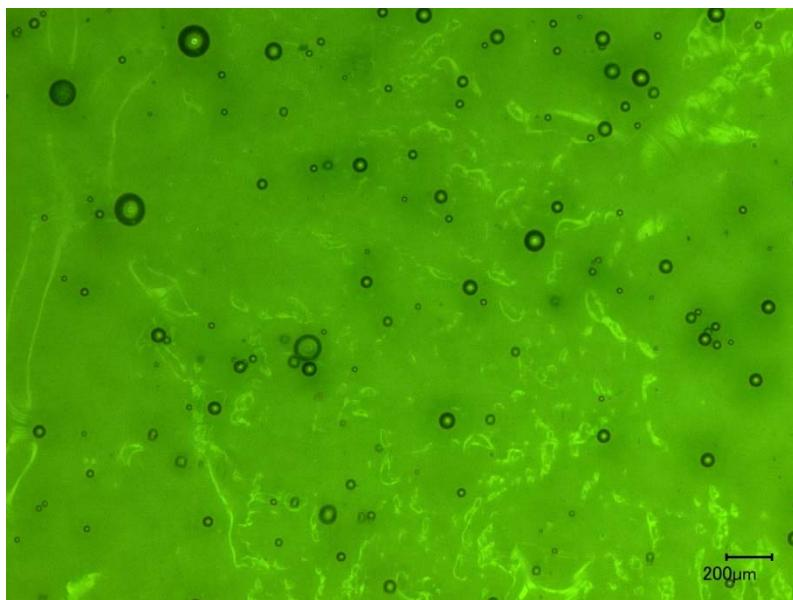
Figure A.2. Photo of Glass LP2-IL-02 Morphology of Fourth Melt at 1150 °C for 0.5 h
