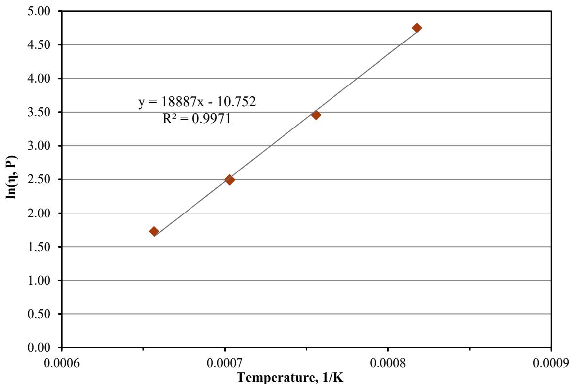
Figure C.39. Viscosity-Temperature Data and Arrhenius Equation Fit for Glass LP2-OL-23
