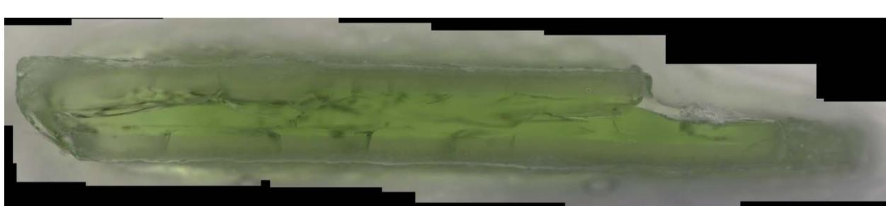
Figure I.19. Quenched Glass LP2-IL-12 after VHT for 24 Days
