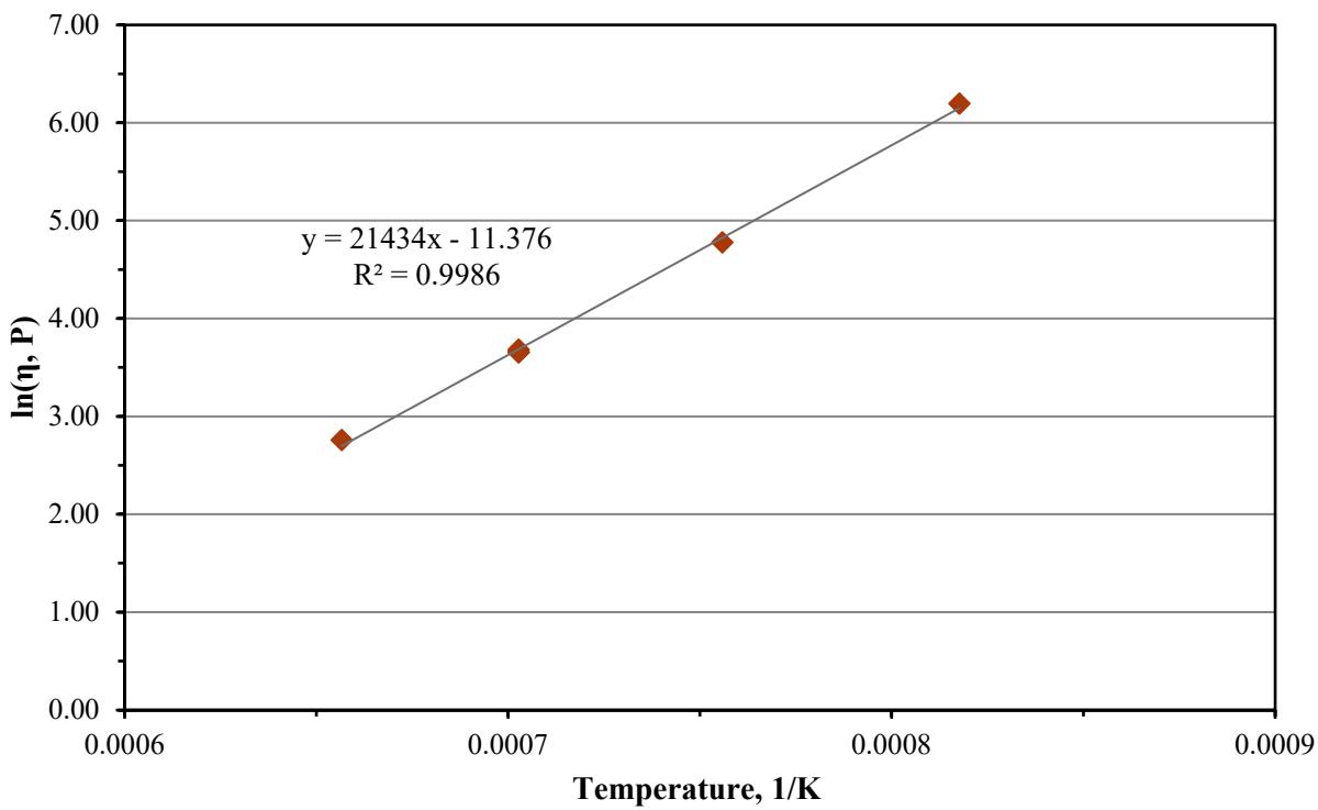
Figure C.21. Viscosity-Temperature Data and Arrhenius Equation Fit for Glass LP2-OL-04-1
