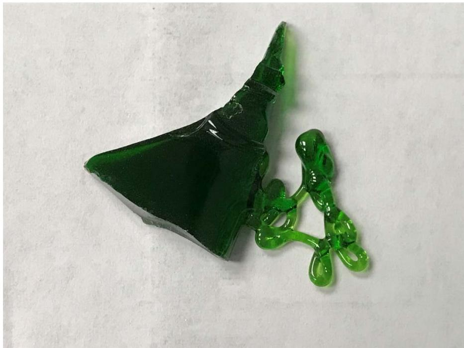
Figure A.15. Photo of Glass LP2-IL-15 Morphology of Third Melt at 1150 °C for 1 h
