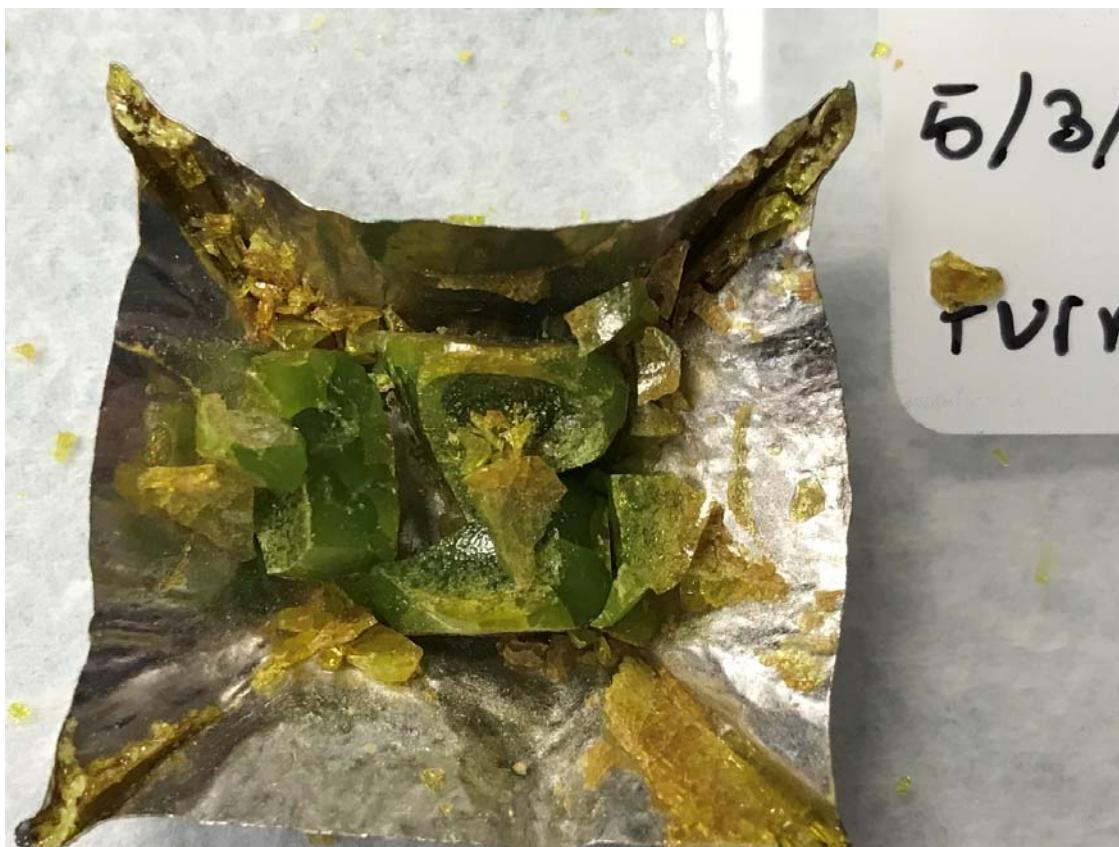
Figure E.33. Glass LP2-OL-18 after CF Heat Treatment at 950 °C for 24 h
