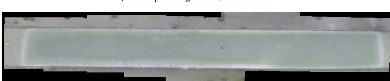
Figure I.99. CCC-Treated Glass LP2-OL-03 MOD2 after VHT for 24 Days
