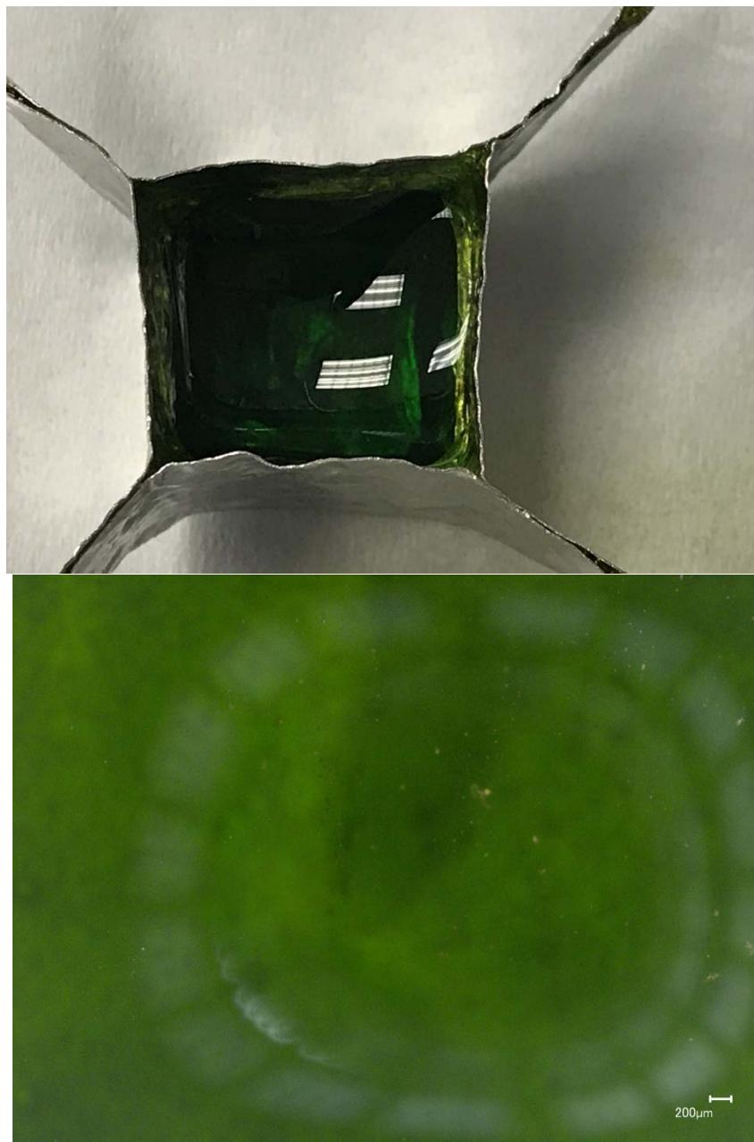
Figure E.9. Glass LP2-IL-10 after CF Heat Treatment at 950 °C for 24 h both in Crucible (top) and Magnified 50X (bottom)
