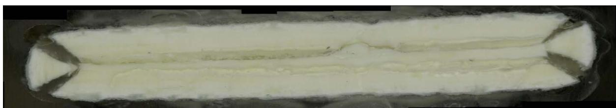
c) Glass cross section magnified after VHT
