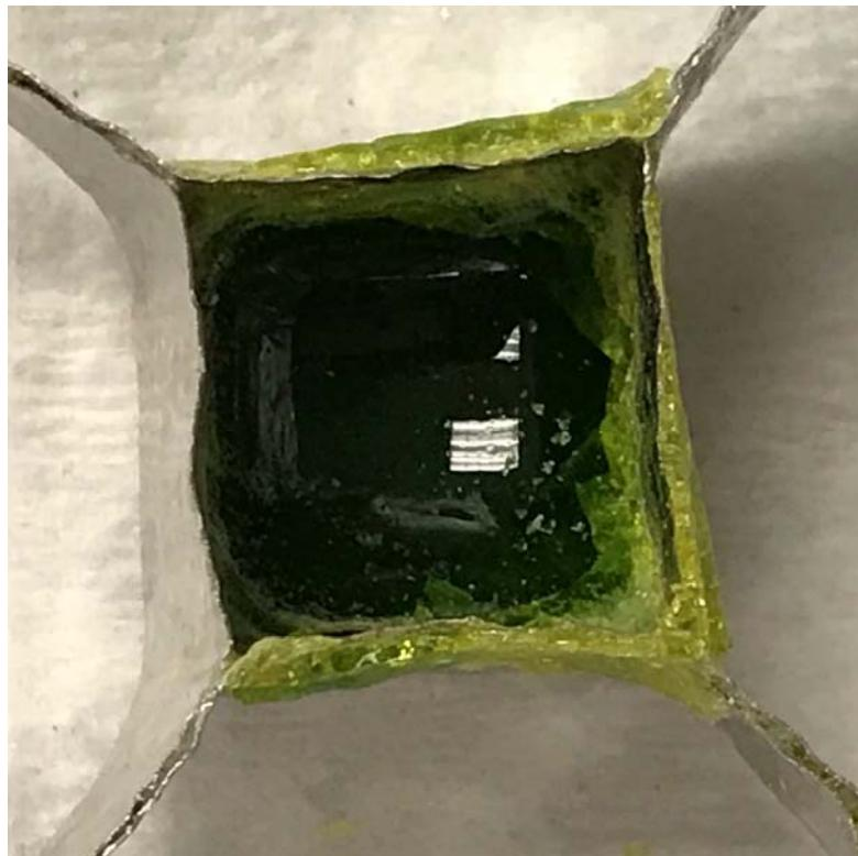
Figure E.2. Glass LP2-IL-03 after CF Heat Treatment at 950 °C for 24 h
