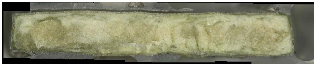
c) Glass cross section magnified after VHT
