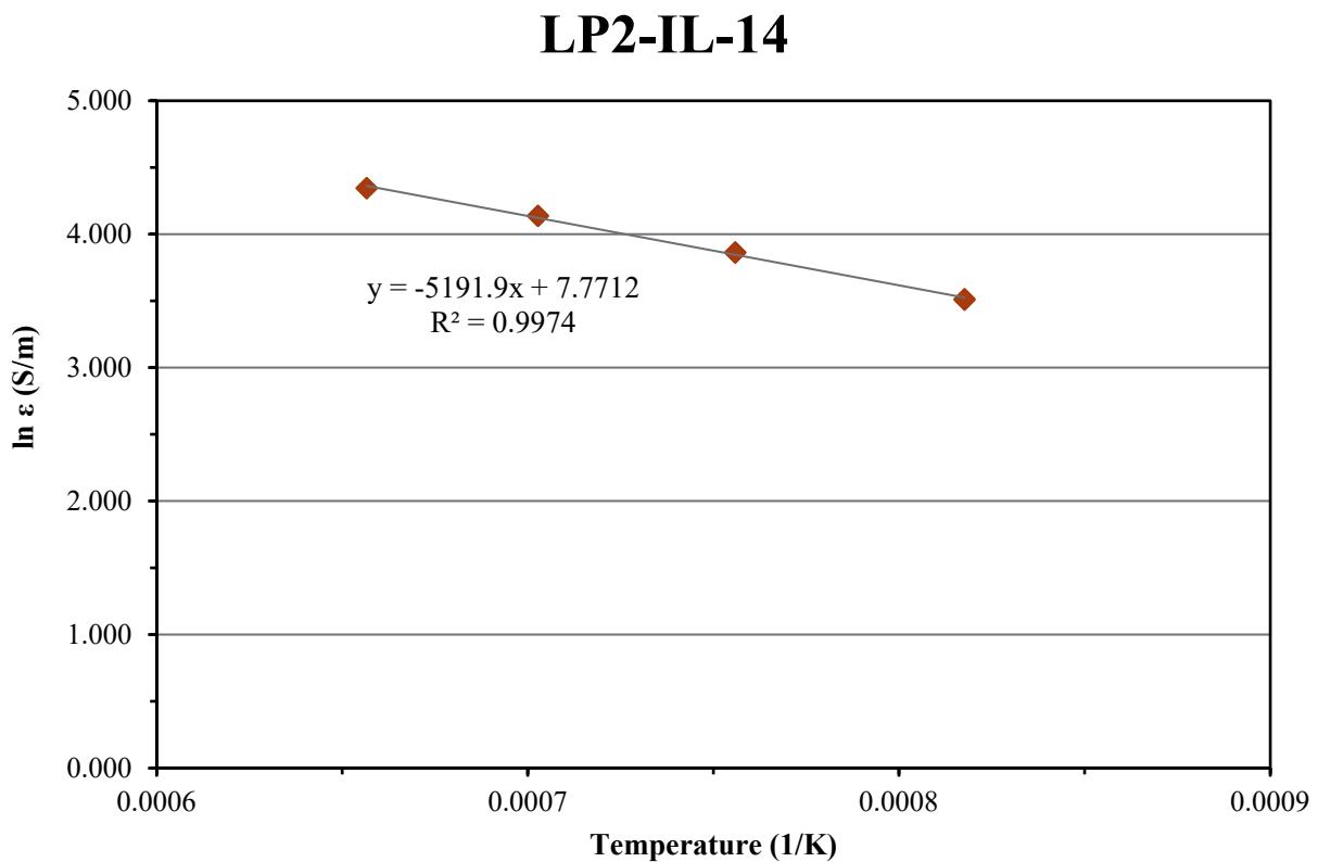
Figure D.14. Electrical Conductivity-Temperature Data and Arrhenius Equation Fit for Glass LP2-IL-14
