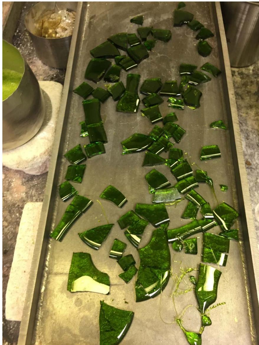
Figure A.39. Photo of Glass LP2-OL-23 Morphology of Second Melt at 1150 °C for 1.5 h
