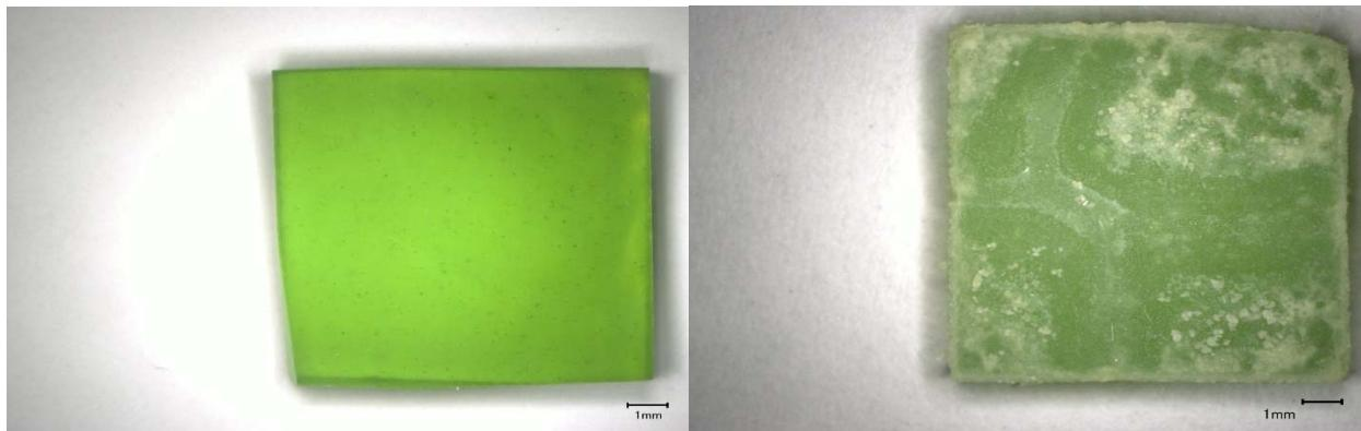
a) Glass square magnified 20X before VHT; b) Glass surface magnified after VHT
