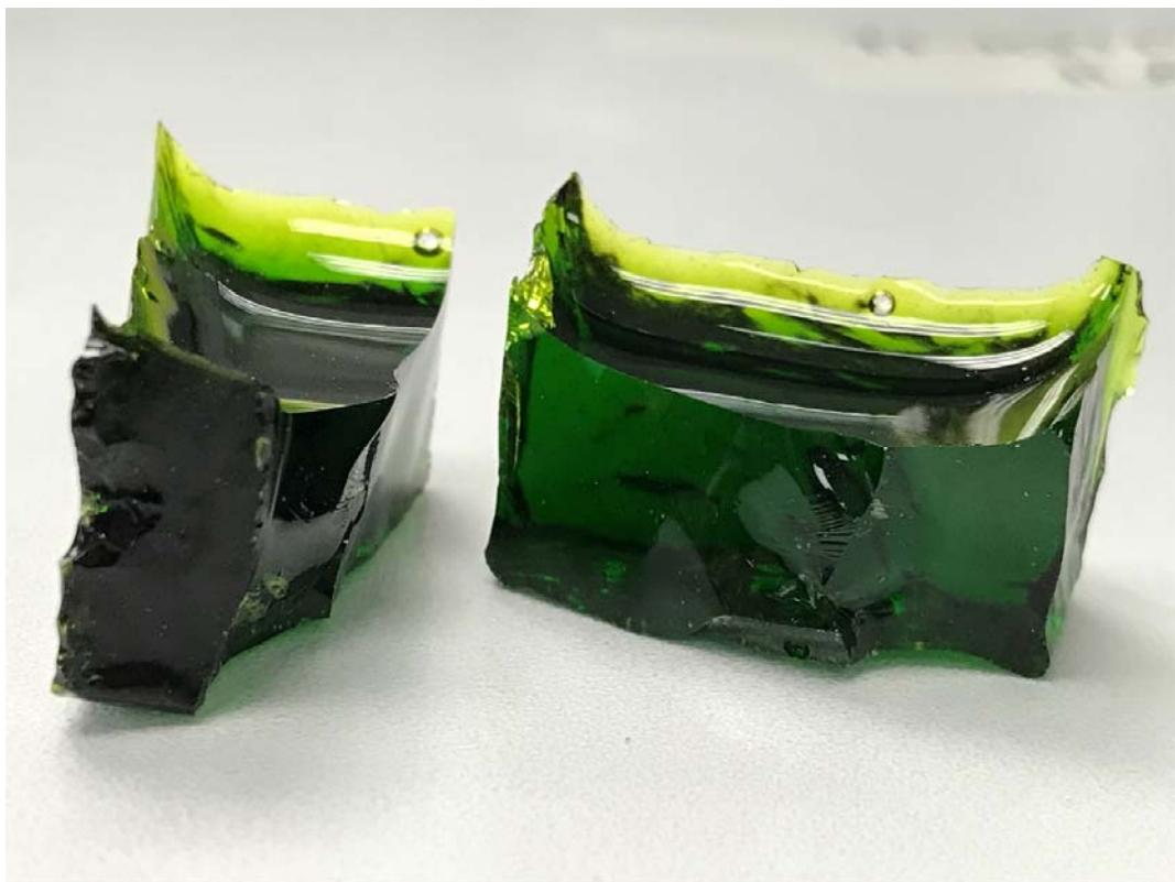
Figure G.25. Glass LP2-OL-09-1 after CCC Beginning at 1150 °C
