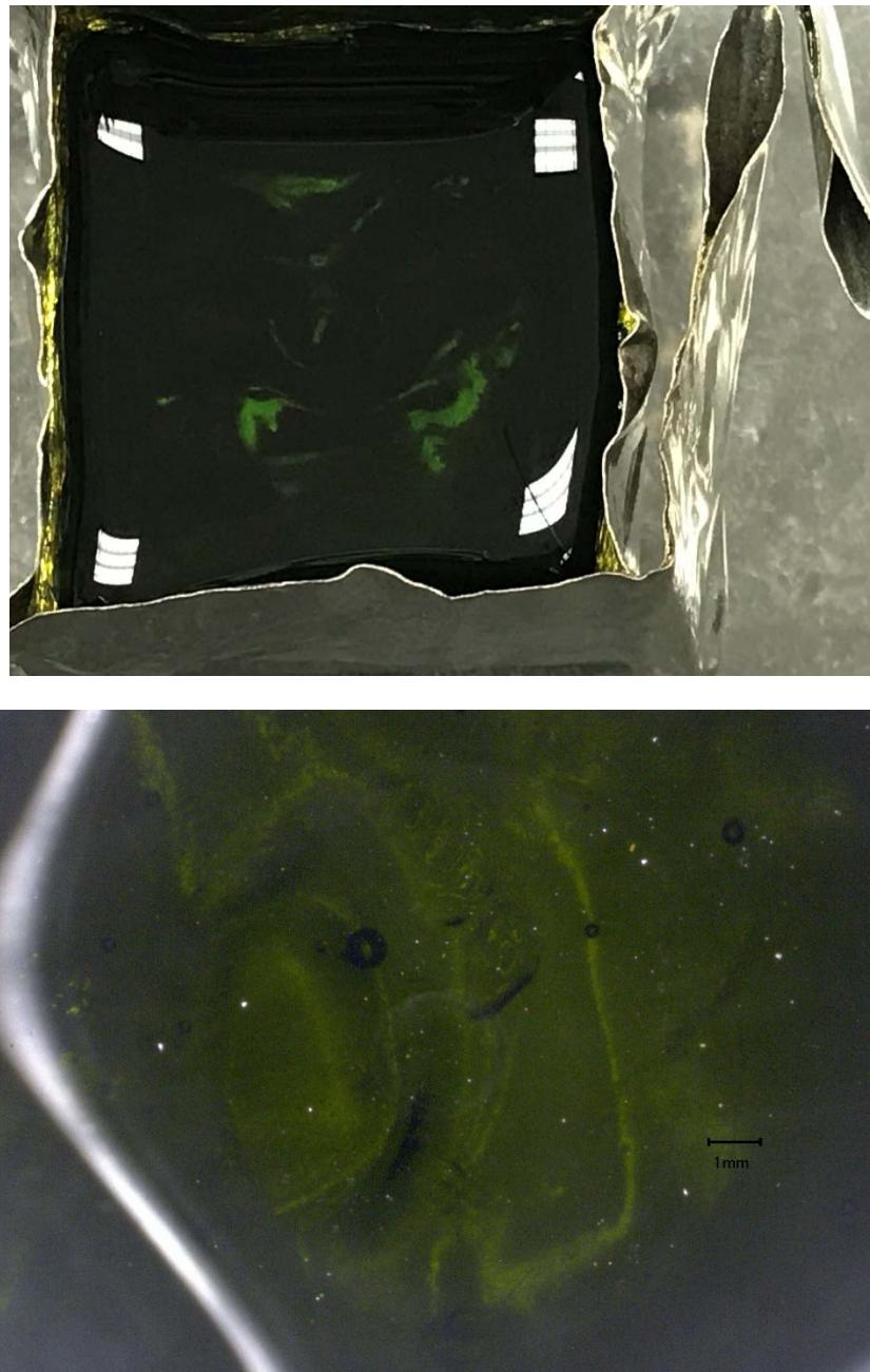
Figure G.38. Glass LP2-OL-22 after CCC Beginning at 1150 °C both in Crucible (top) and Magnified 20X (bottom)
