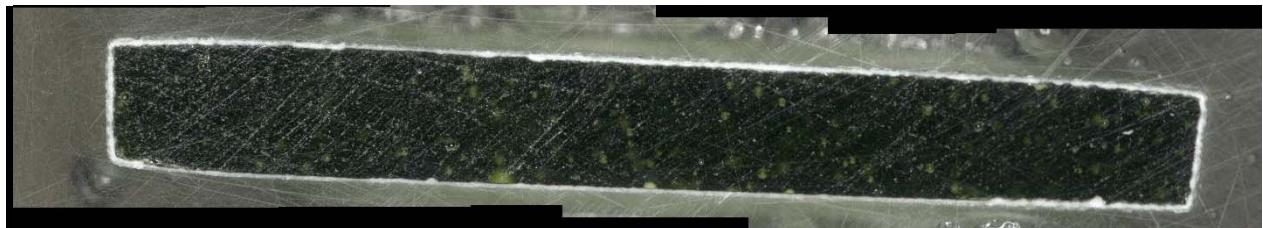
b) Glass cross section magnified after VHT
