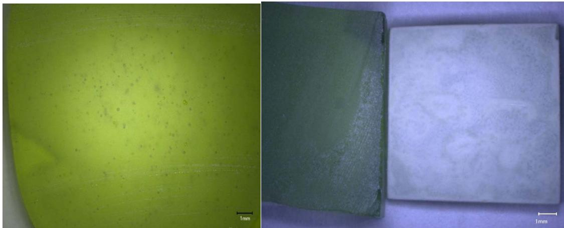
a) Glass square magnified 20X before VHT; b) Glass square after (right) and before (left) VHT
