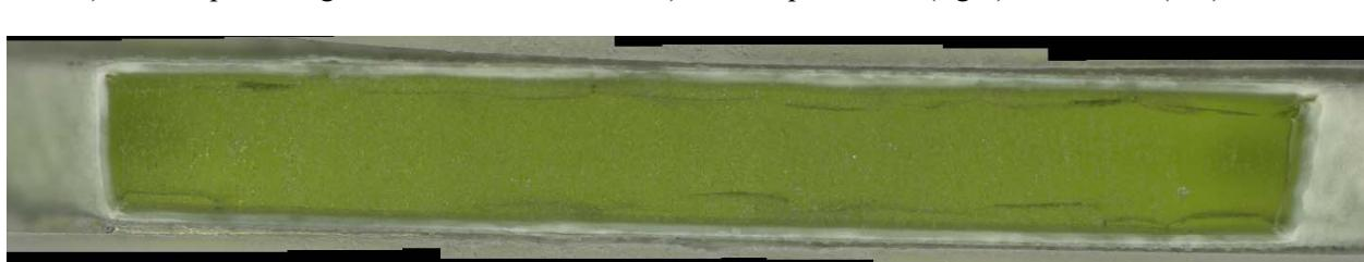
Figure I.95. CCC-Treated Glass LP2-OL-01-3 after VHT for 11 Days
