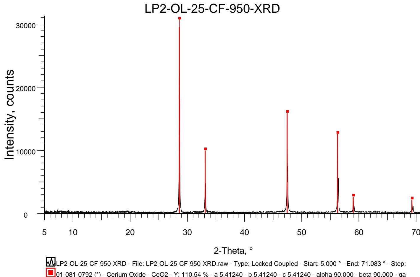
Figure F.25. XRD Spectrum of Heat-Treated Glass LP2-OL-25
