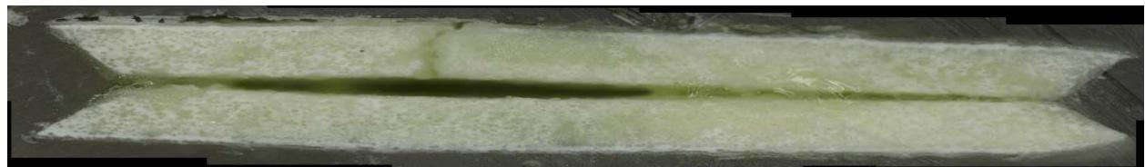
b) Glass cross section magnified after VHT
