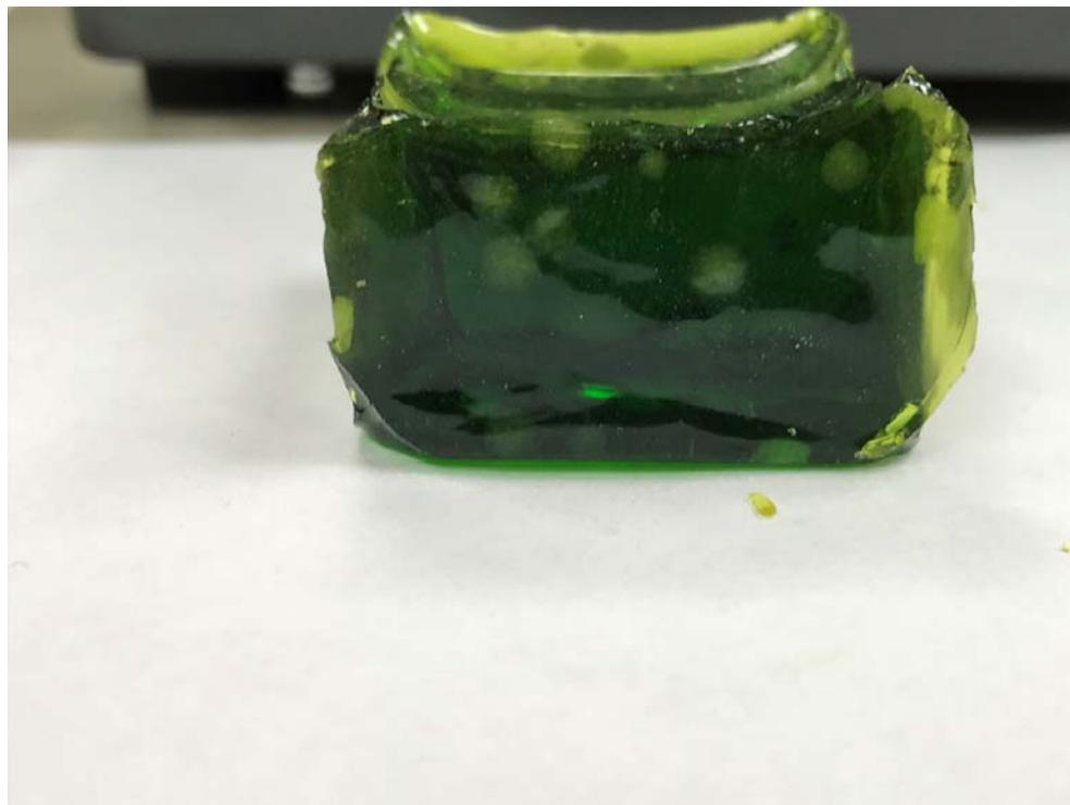
Figure G.37. Glass LP2-OL-21 after CCC Beginning at 1150 °C
