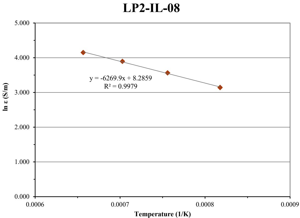
Figure D.8. Electrical Conductivity-Temperature Data and Arrhenius Equation Fit for Glass LP2-IL-08
