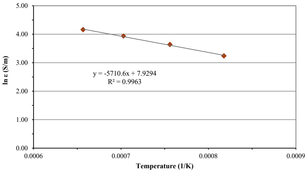
Figure D.30. Electrical Conductivity-Temperature Data and Arrhenius Equation Fit for Glass LP2-OL-14
