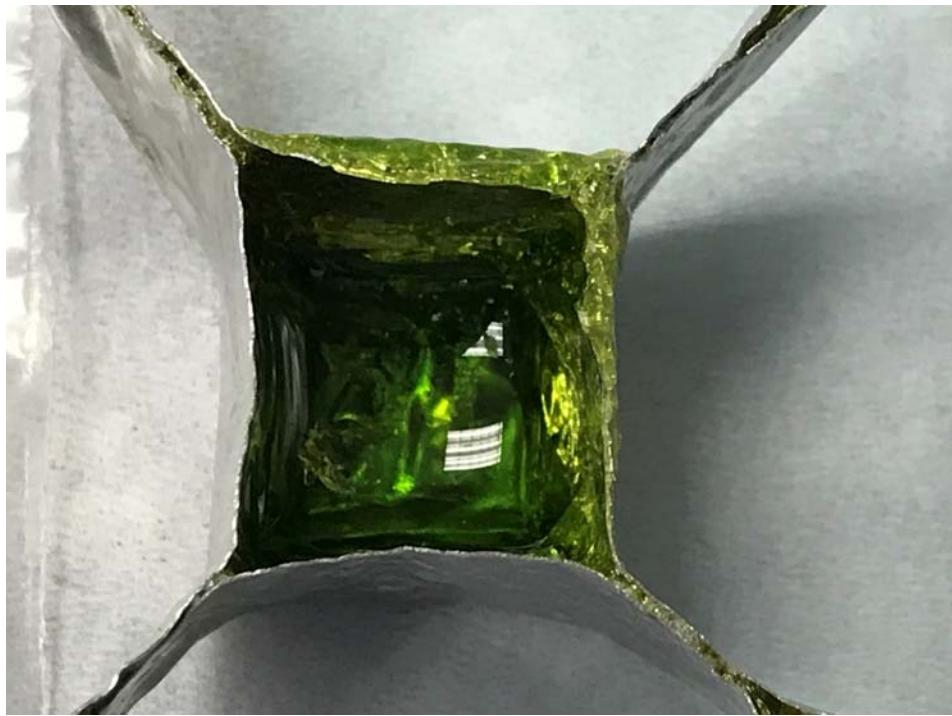
Figure E.13. Glass LP2-IL-14 after CF Heat Treatment at 950 °C for 24 h
