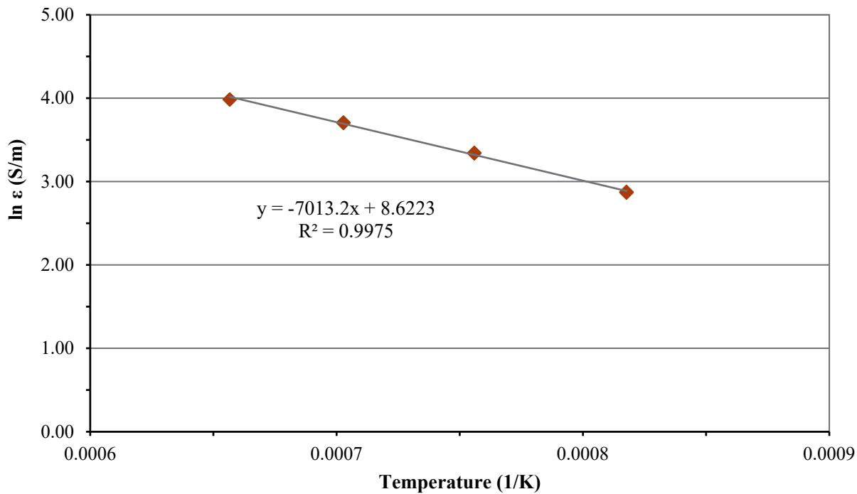
Figure D.38. Electrical Conductivity-Temperature Data and Arrhenius Equation Fit for Glass LP2-OL-22
