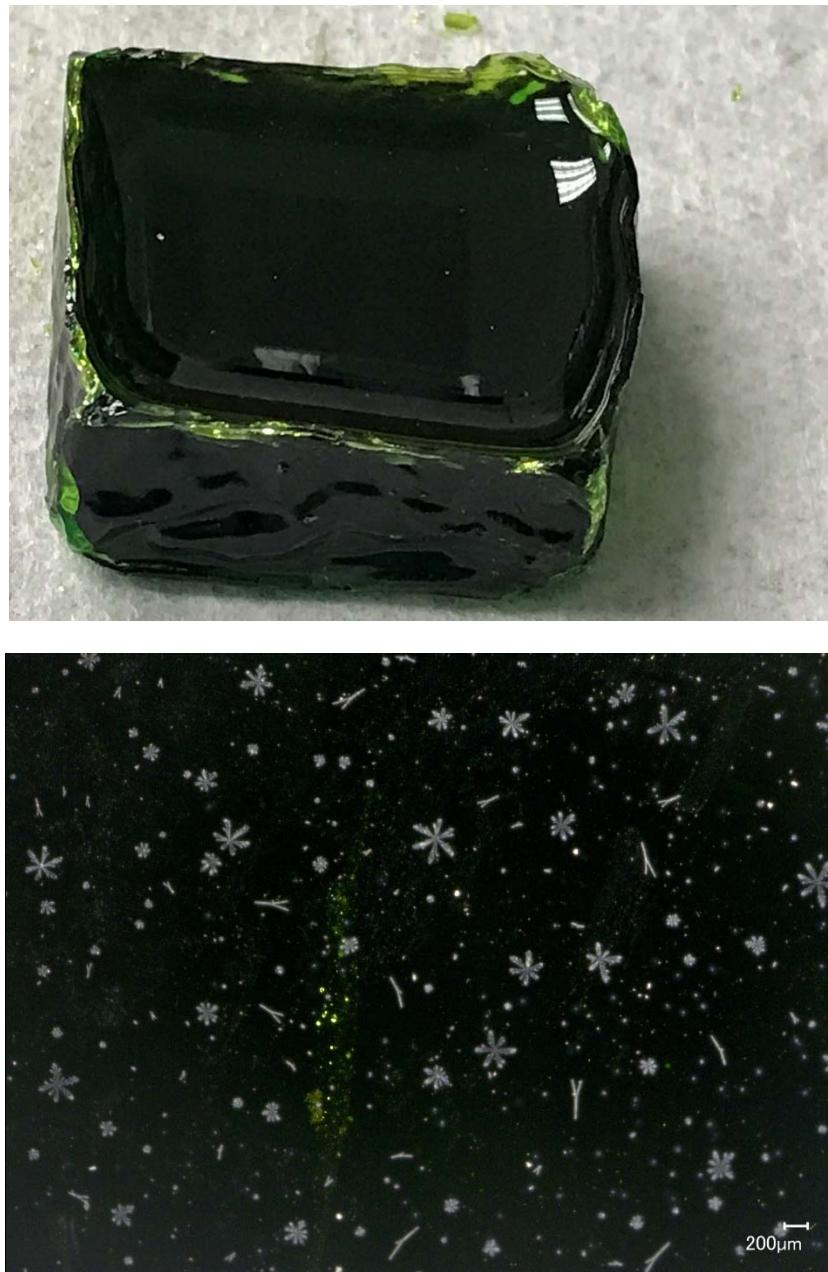
Figure G.13. Glass LP2-IL-13 after CCC Beginning at 1150 °C both Glass (top) and Magnified 50X (bottom)
