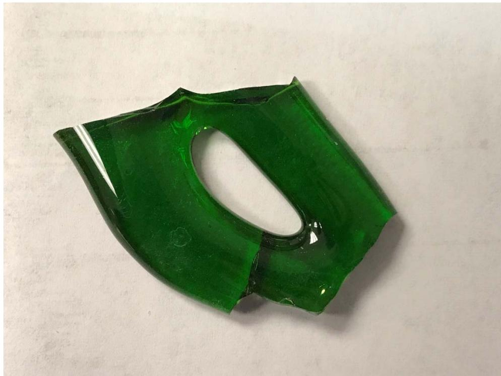
Figure A.11. Photo of Glass LP2-IL-11 Morphology of Third Melt at 1175 °C for 1 h
