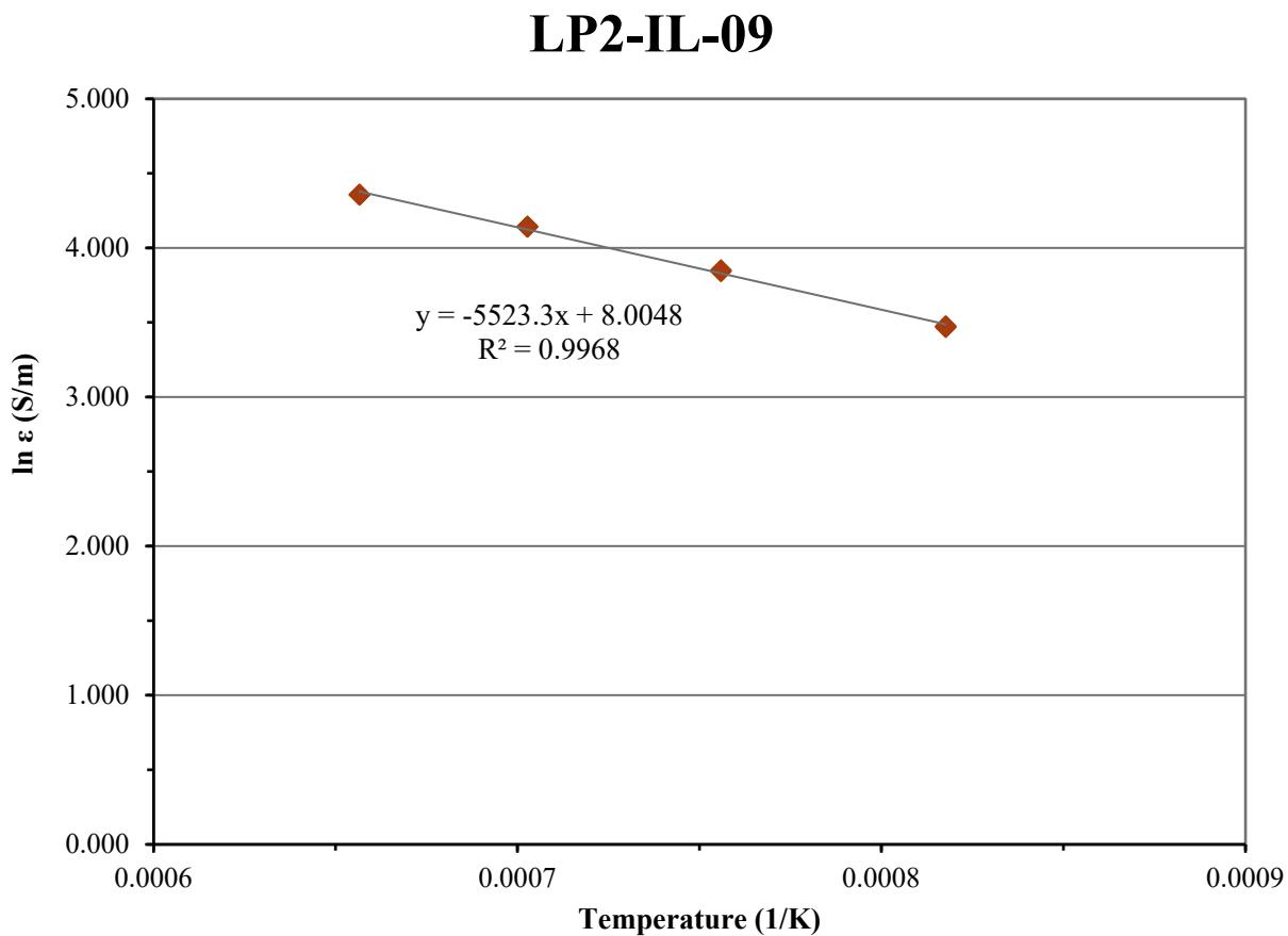
Figure D.9. Electrical Conductivity-Temperature Data and Arrhenius Equation Fit for Glass LP2-IL-09
