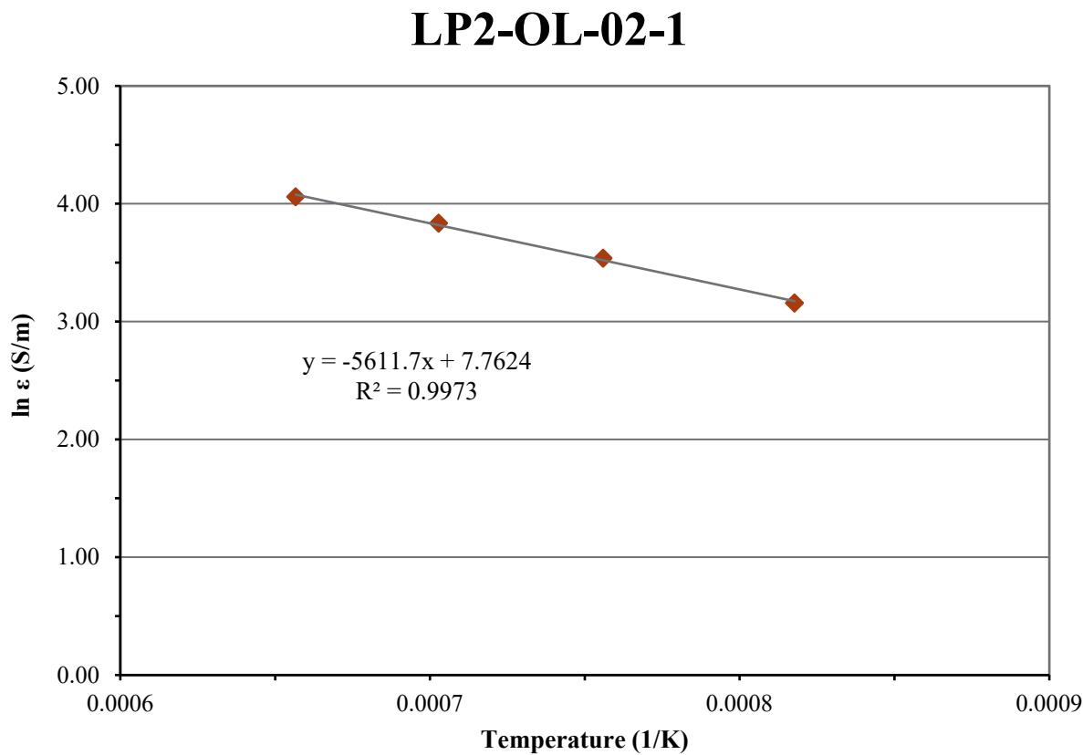
Figure D.19. Electrical Conductivity-Temperature Data and Arrhenius Equation Fit for Glass LP2-OL-02-1
