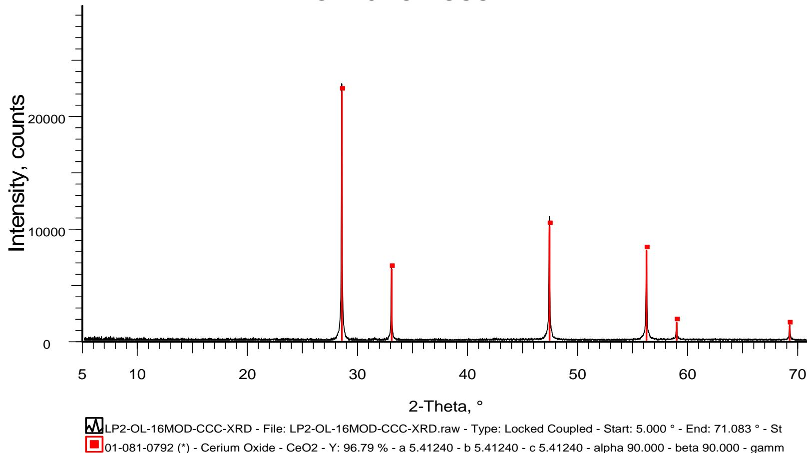
Figure H.16. XRD Spectrum of CCC-Treated Glass LP2-OL-16 MOD
