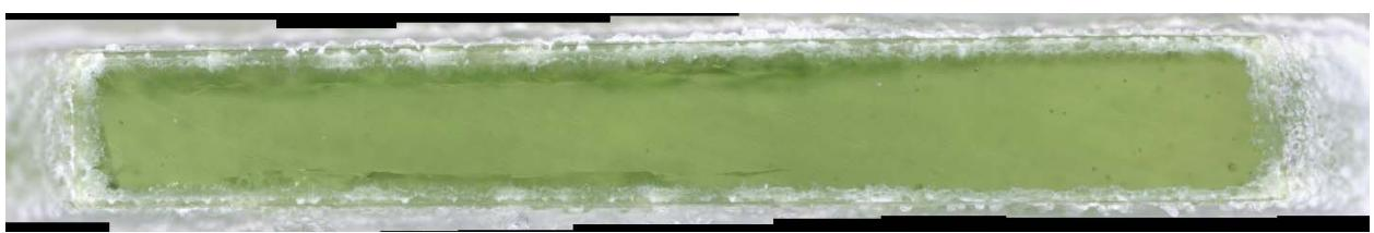
b) Glass cross section magnified after VHT
