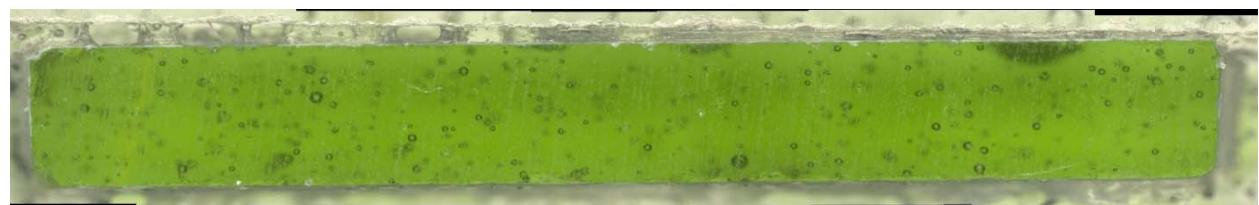
c) Glass cross section magnified after VHT
