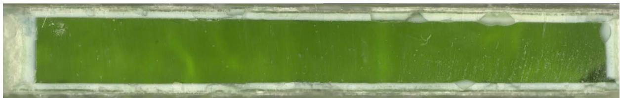
c) Glass cross section magnified after VHT
