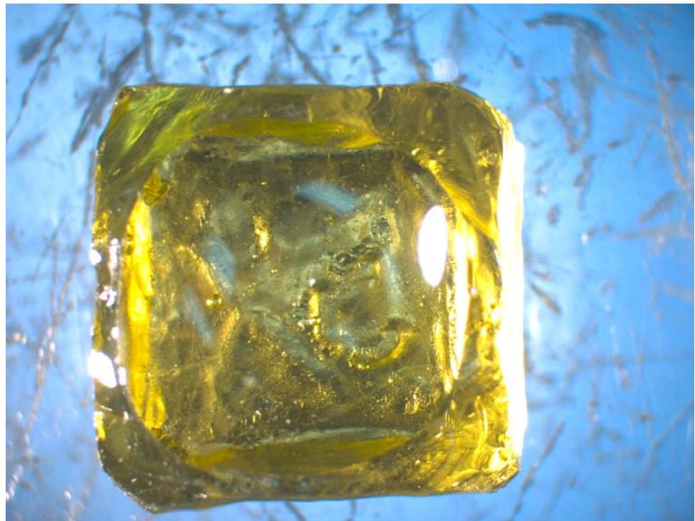
Figure E.26. Glass LP2-OL-11 after CF Heat Treatment at 950 °C for 24 h
