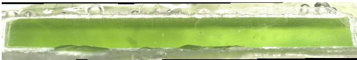
Figure I.82. CCC-Treated Glass LP2-IL-10 after VHT for 7 Days
