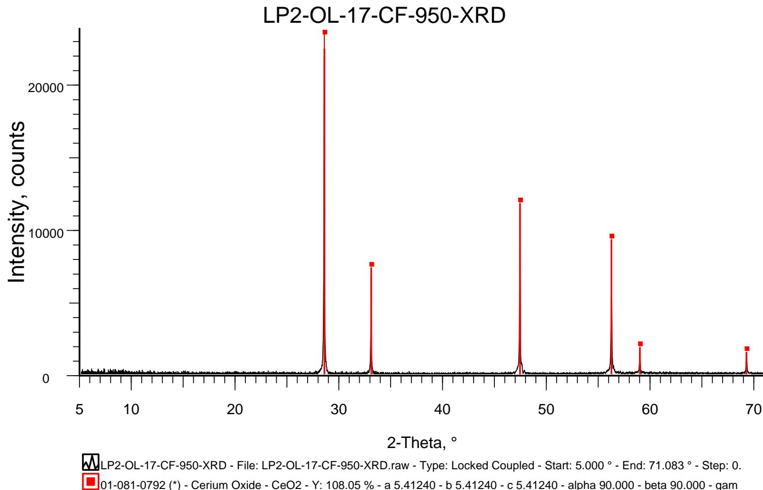
Figure F.19. XRD Spectrum of Heat-Treated Glass LP2-OL-17
