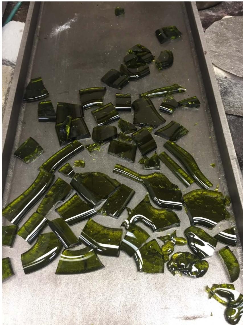
Figure A.38. Photo of Glass LP2-OL-22 Morphology of Third Melt at 1150 °C for 1.5 h
