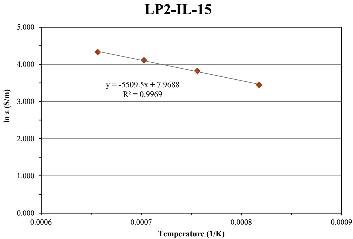
Figure D.15. Electrical Conductivity-Temperature Data and Arrhenius Equation Fit for Glass LP2-IL-15
