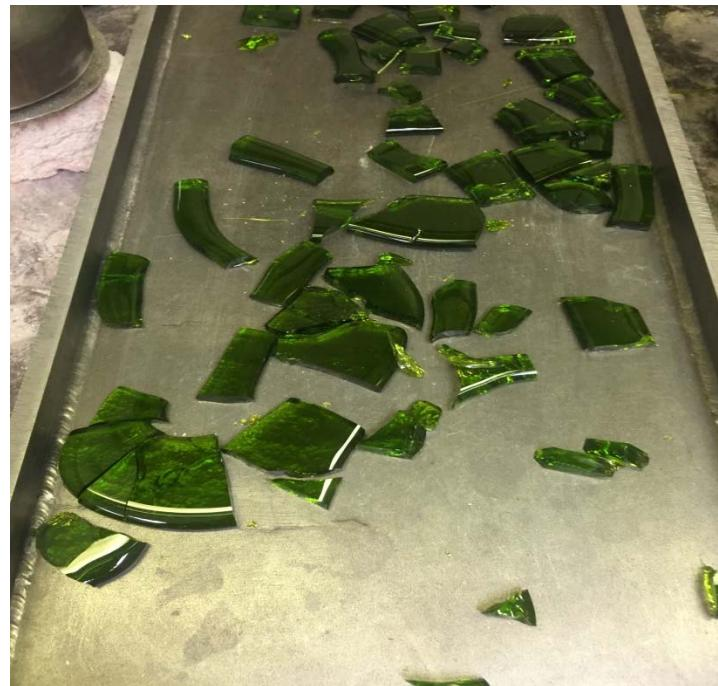
Figure A.19. Photo of Glass LP2-OL-02-1 Morphology of Second Melt at 1150 °C for 1.3 h
