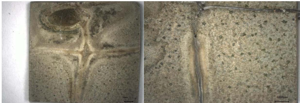
a) Glass square magnified 20X after VHT; b) Glass square magnified 30X after VHT
