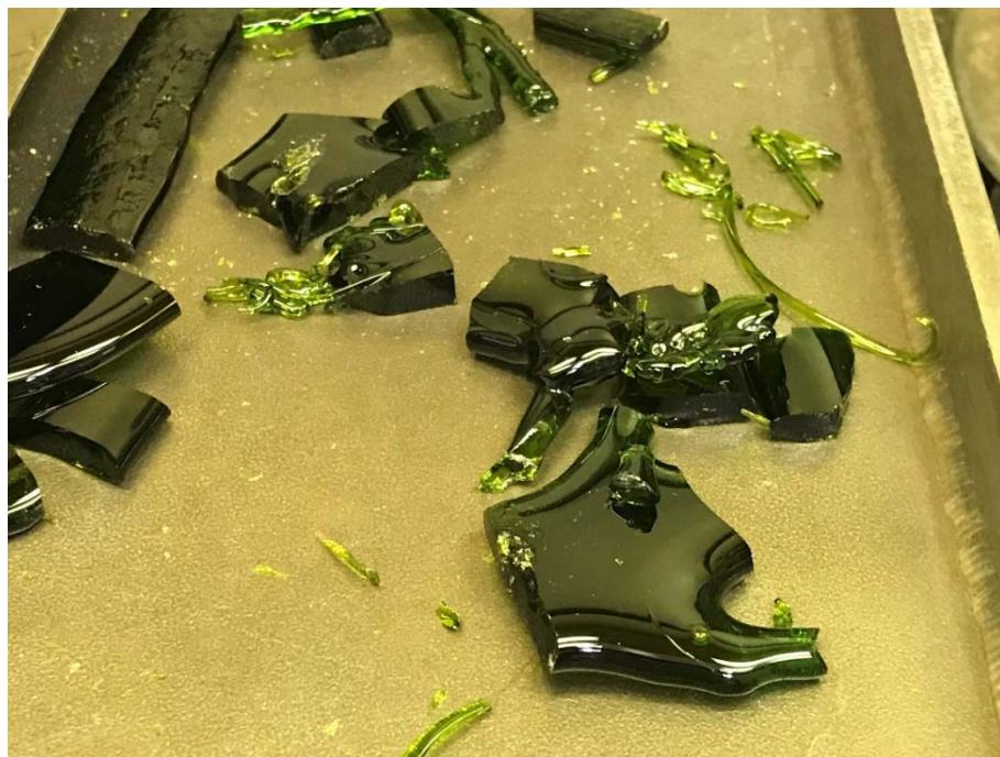
Figure 2.15. Glass LP2-OL-16 after First Modification
