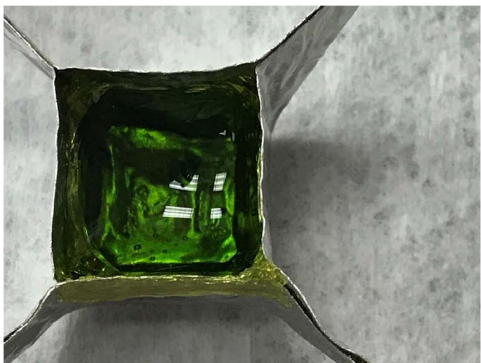
Figure E.18. Glass LP2-OL-02-1 after CF Heat Treatment at 950 °C for 24 h
