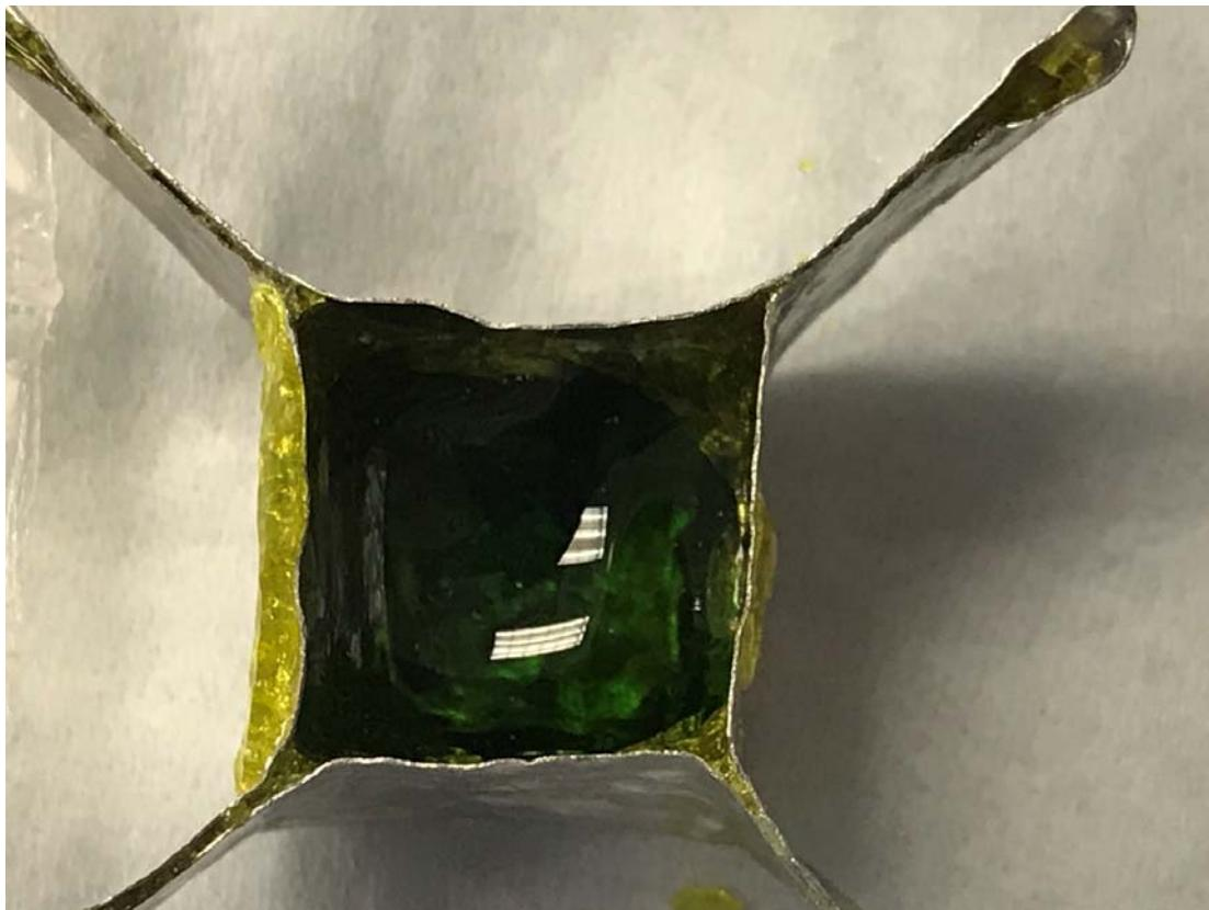
Figure E.8. Glass LP2-IL-09 after CF Heat Treatment at 950 °C for 24 h
