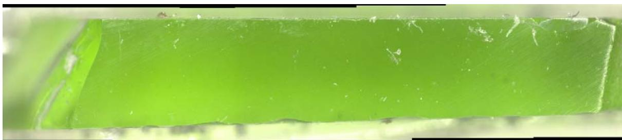
c) Glass cross section magnified after VHT
