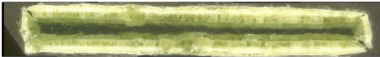
c) Glass cross section magnified after VHT
