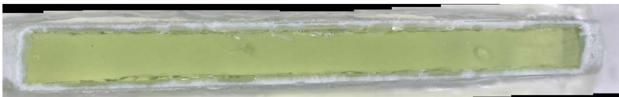
b) Glass cross section magnified after VHT
