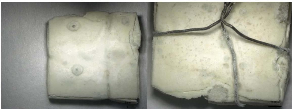
a) Glass square magnified 20X after VHT; b) Glass square magnified 30X after VHT
