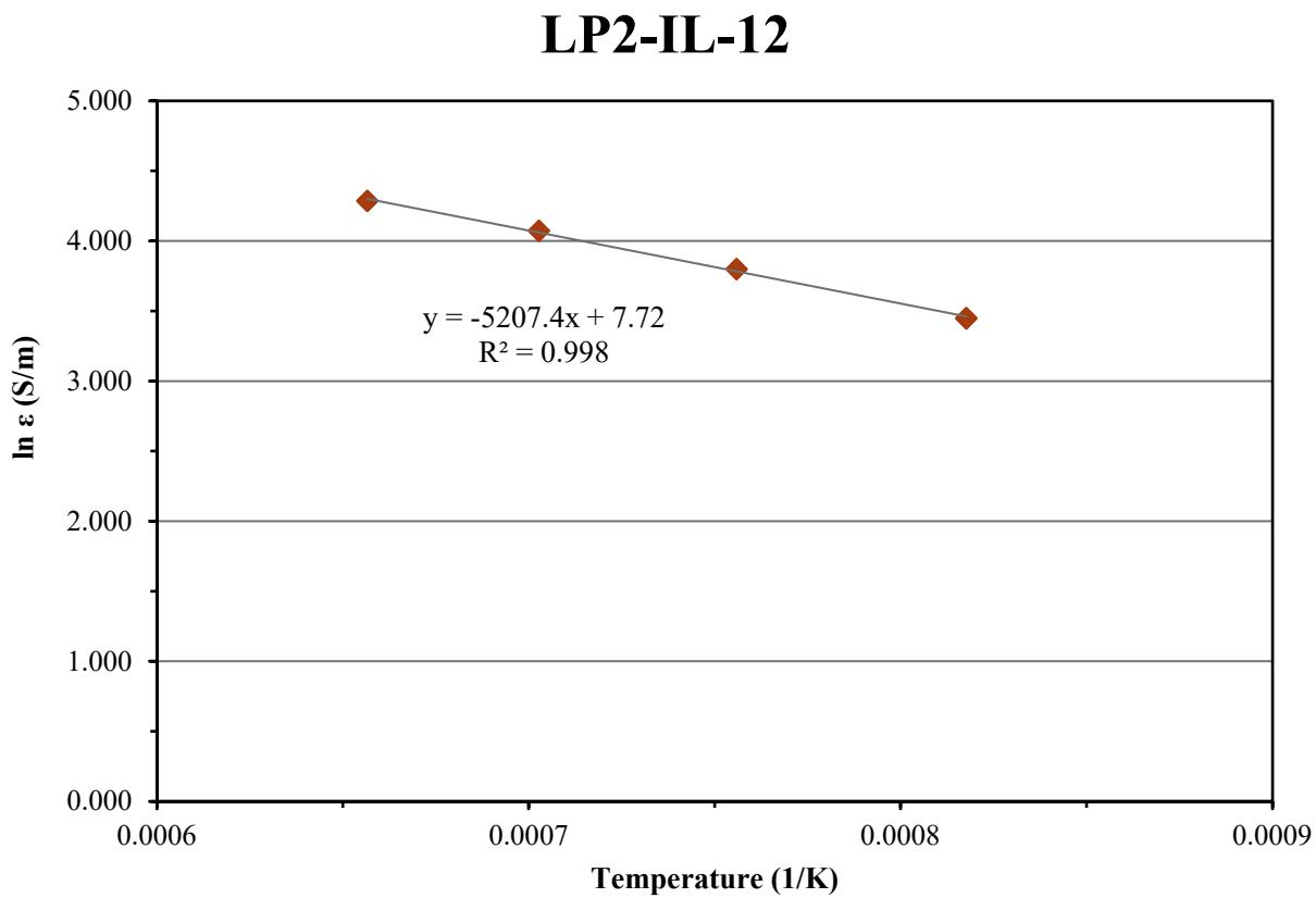
Figure D.12. Electrical Conductivity-Temperature Data and Arrhenius Equation Fit for Glass LP2-IL-12
