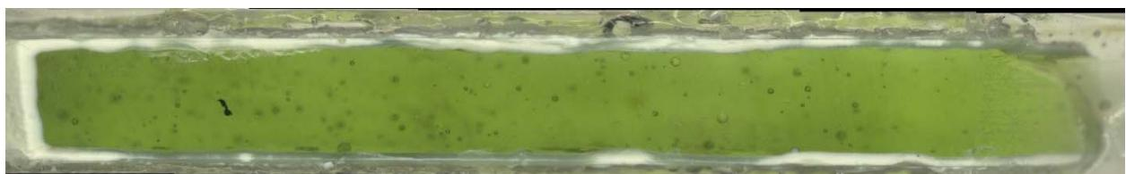
c) Glass cross section magnified after VHT
