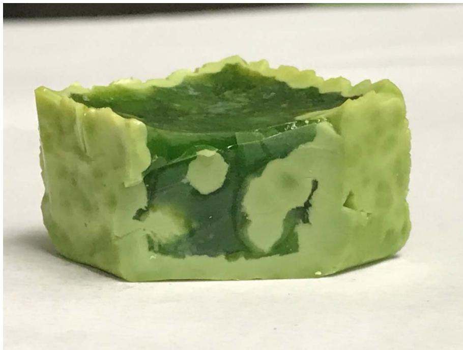
Figure 3.4. Glass LP2-OL-05 Cooled in a Pt Crucible with Crystals along Edge
