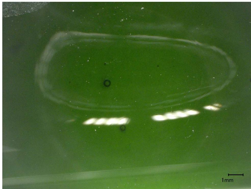
Figure A.4. Photo of Glass LP2-IL-04 Morphology of Second Melt at 1150 °C for 2.3 h
