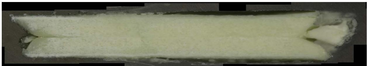
b) Glass cross section magnified after VHT
