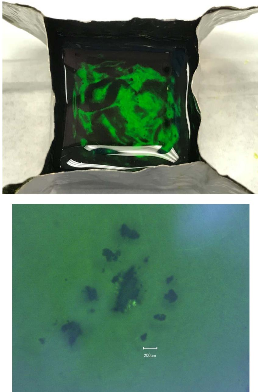
Figure G.18. Glass LP2-OL-01-3 after CCC Beginning at 1150 °C both in Crucible (top) and Magnified 100X (bottom)
