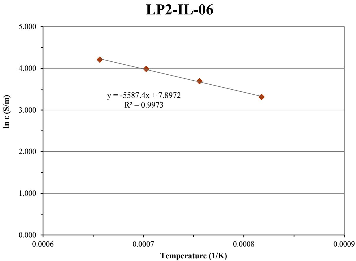
Figure D.6. Electrical Conductivity-Temperature Data and Arrhenius Equation Fit for Glass LP2-IL-06
