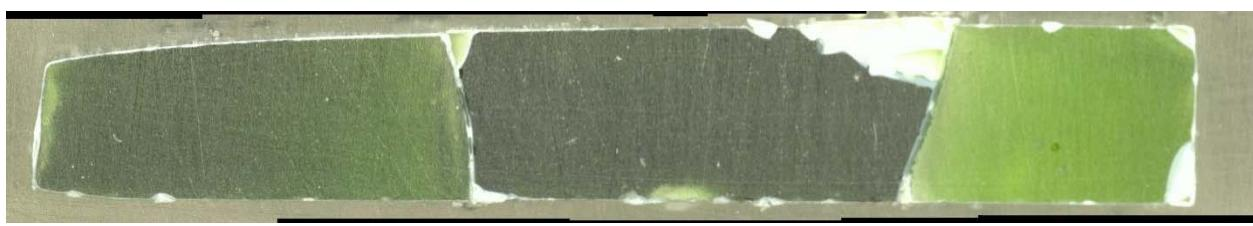
Figure I.90. CCC-Treated Glass LP2-IL-15 after VHT for 7 Days
