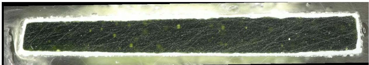
b) Glass cross section magnified after VHT
