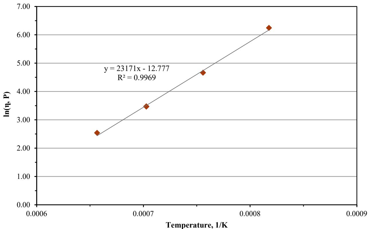
Figure C.38. Viscosity-Temperature Data and Arrhenius Equation Fit for Glass LP2-OL-22
