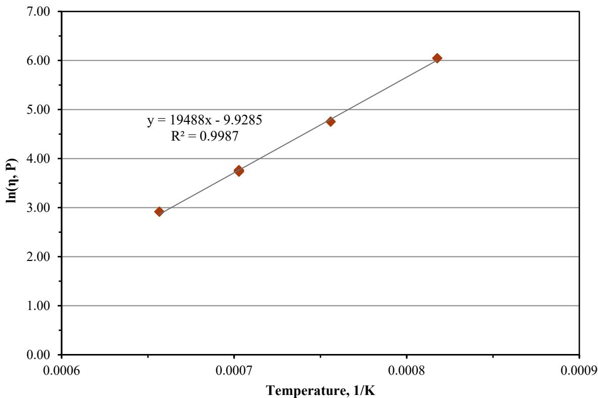
Figure C.37. Viscosity-Temperature Data and Arrhenius Equation Fit for Glass LP2-OL-21
