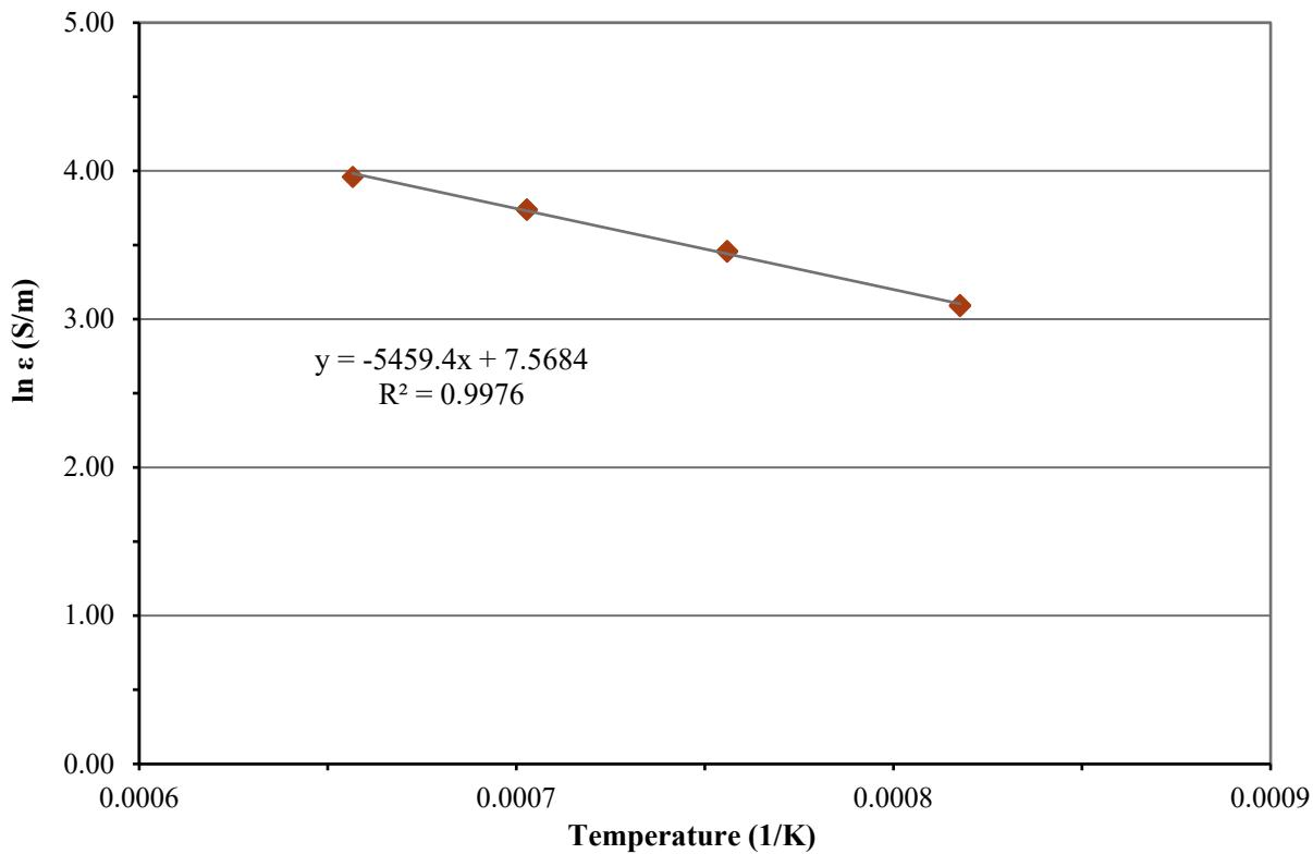
Figure D.32. Electrical Conductivity-Temperature Data and Arrhenius Equation Fit for Glass LP2-OL-16 MOD
