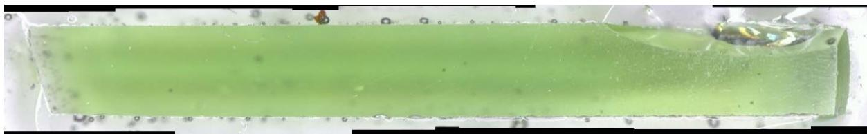
c) Glass cross section magnified after VHT
