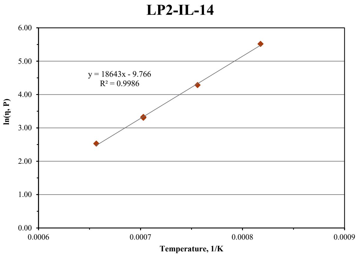
Figure C.14. Viscosity-Temperature Data and Arrhenius Equation Fit for Glass LP2-IL-14
