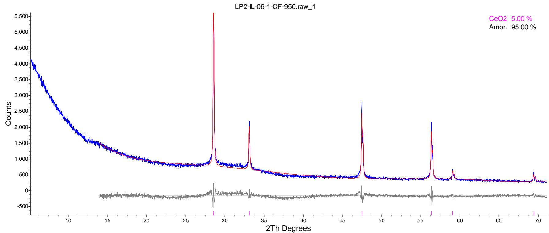
Figure F.6. XRD Spectrum of Heat-Treated Glass LP2-IL-06
