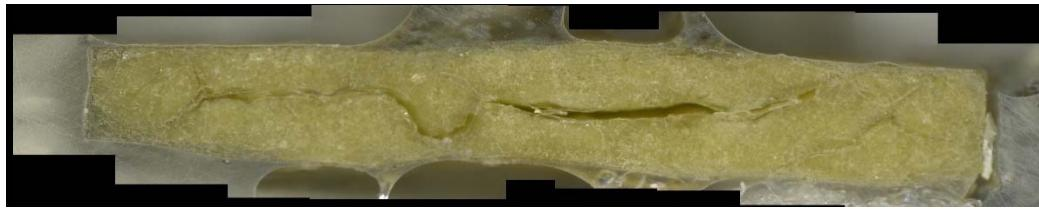
c) Glass cross section magnified after VHT
