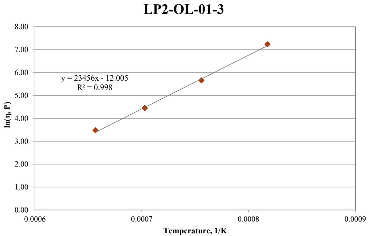
Figure C.18. Viscosity-Temperature Data and Arrhenius Equation Fit for Glass LP2-OL-01-3
