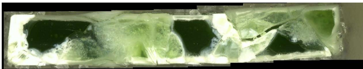
c) Glass cross section magnified after VHT
