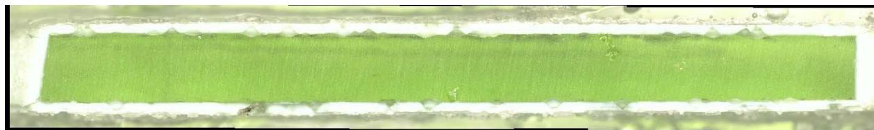
c) Glass cross section magnified after VHT
