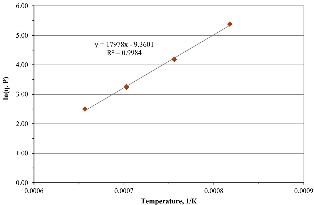
Figure C.7. Viscosity-Temperature Data and Arrhenius Equation Fit for Glass LP2-IL-07
