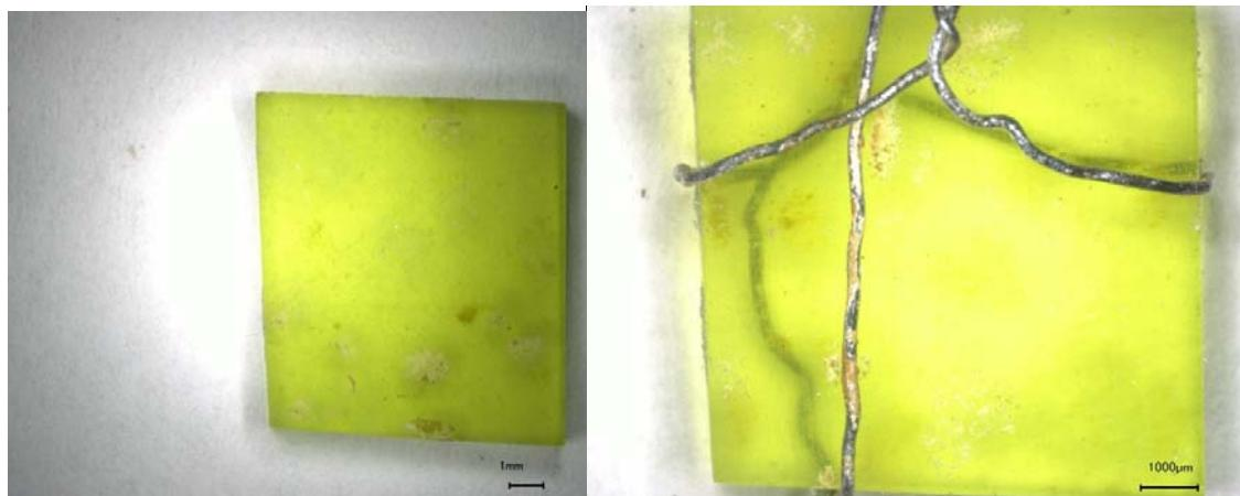
a) Glass square magnified 20X after VHT; b) Glass square magnified 30X after VHT
