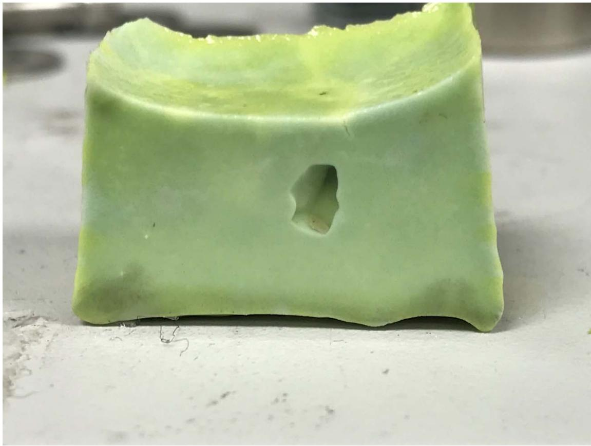
Figure G.20. Glass LP2-OL-03MOD2 after CCC Beginning at 1150 °C
