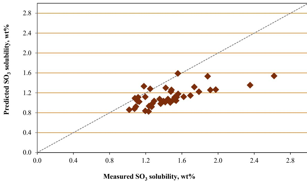
Figure 3.15. Predicted versus Measured  $\text{SO}_3$  Solubility (wt%) for Phase 2 Enhanced LAW Glasses. The predicted values were obtained using the model in Equation (3.6) with coefficients as listed in Table 3.16.
