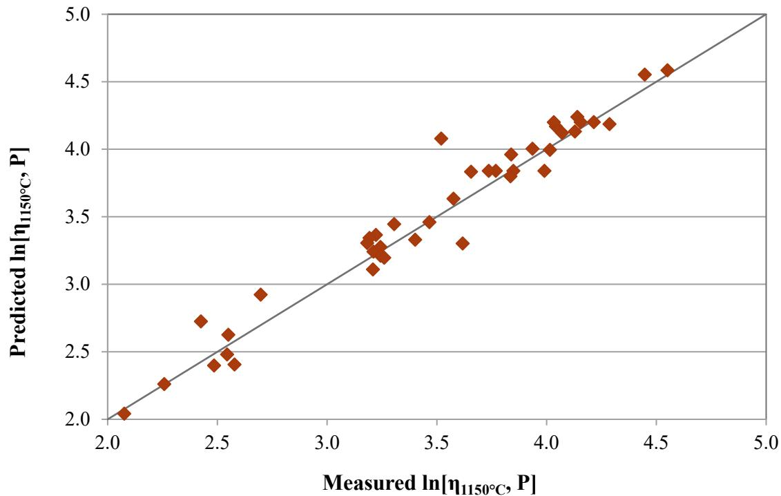
Figure 3.2. Predicted Versus Measured Viscosity at 1150°C Values for Phase 2 Enhanced LAW Glasses. The predicted values were obtained using the model in Equation (3.4).
