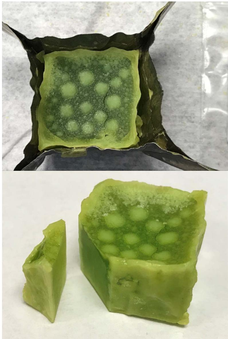
Figure G.29. Glass LP2-OL-13 after CCC Beginning at 1150 °C both in Crucible (top) and Glass (bottom)
