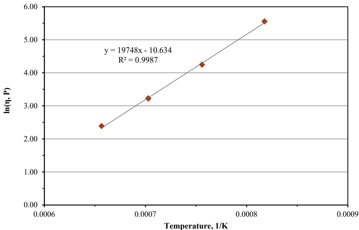
Figure C.1. Viscosity-Temperature Data and Arrhenius Equation Fit for Glass LP2-IL-01
