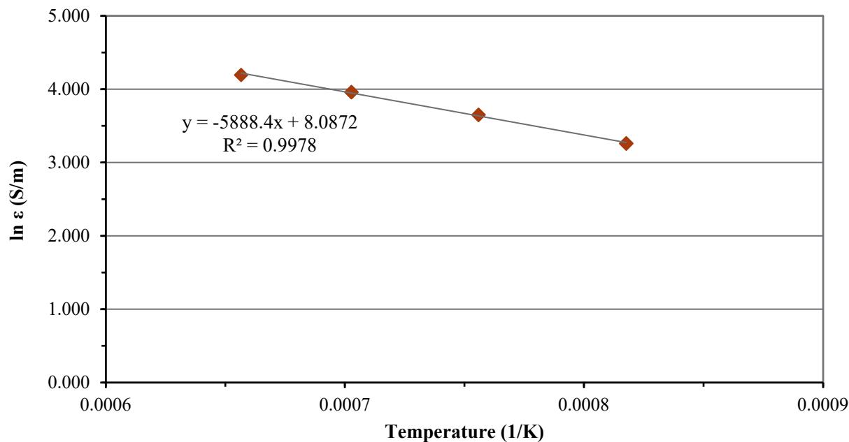
Figure D.10. Electrical Conductivity-Temperature Data and Arrhenius Equation Fit for Glass LP2-IL-10
