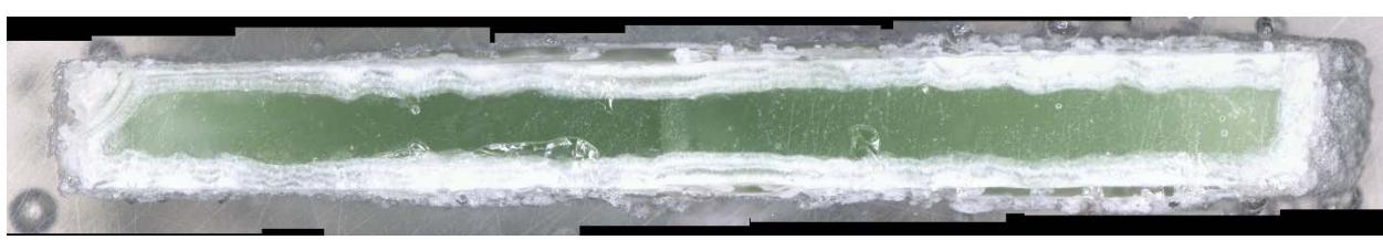
Figure I.94. CCC-Treated Glass LP2-IL-17 after VHT for 24 Days
