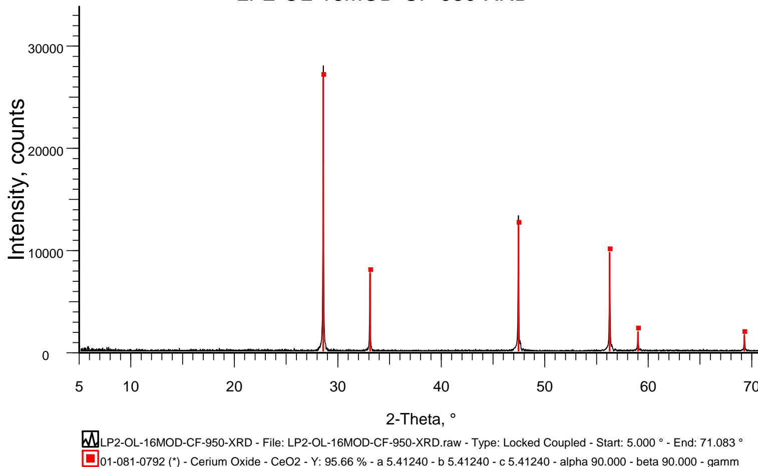
Figure F.18. XRD Spectrum of Heat-Treated Glass LP2-OL-16 MOD
