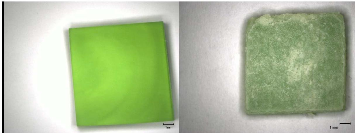
a) Glass square magnified 20X before VHT; b) Glass surface magnified after VHT
