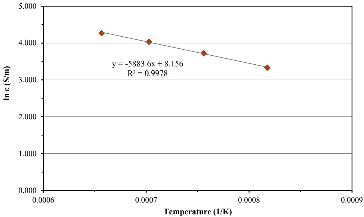
Figure D.16. Electrical Conductivity-Temperature Data and Arrhenius Equation Fit for Glass LP2-IL-16
