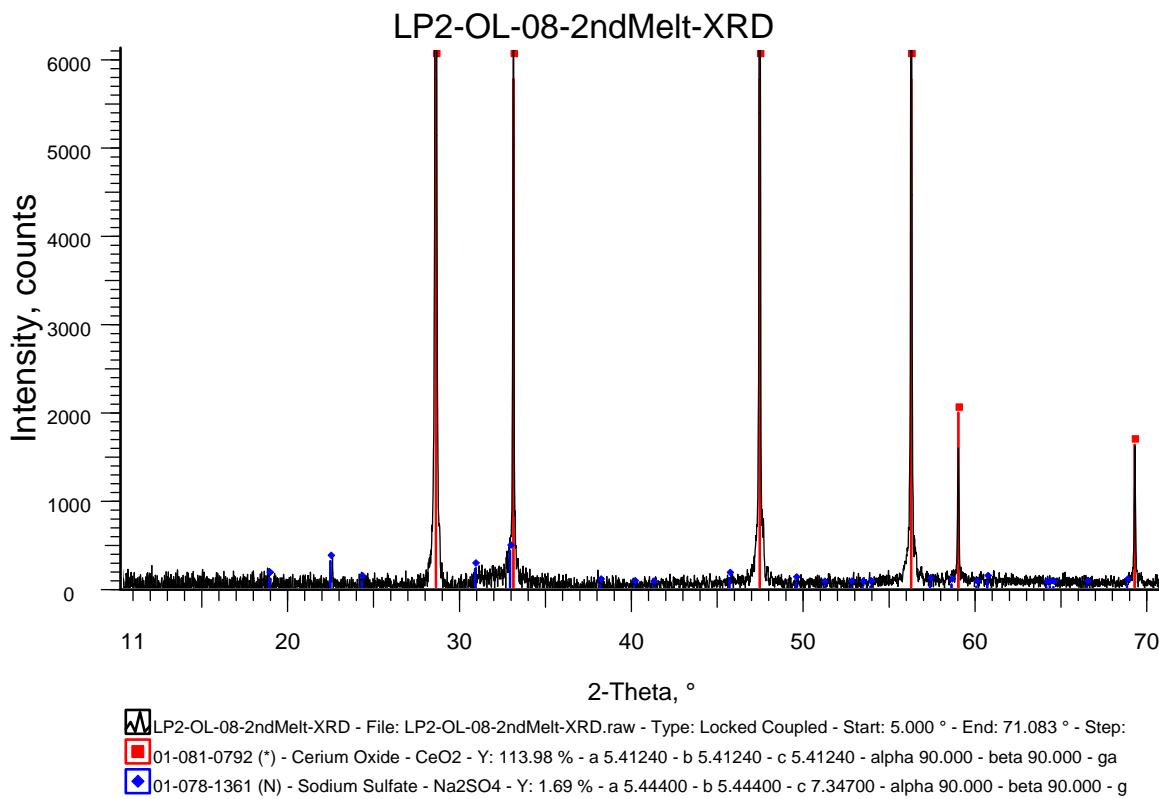
Figure 2.10. XRD Pattern of Original LP2-OL-08 Composition
