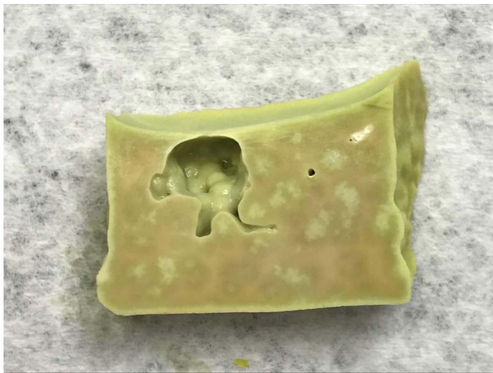
Figure G.21. Glass LP2-OL-04-1 after CCC Beginning at 1150 °C
