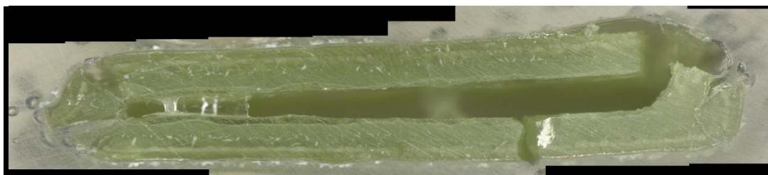
b) Glass cross section magnified after VHT
