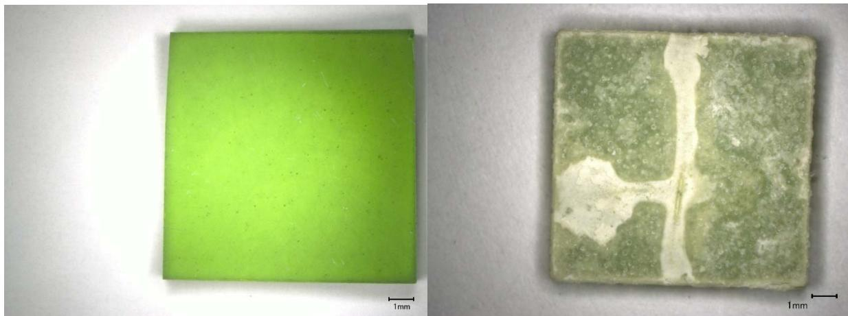
a) Glass square magnified 20X before VHT; b) Glass square magnified 20X after VHT
