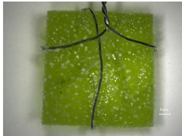
a) Glass surface magnified 20X after VHT
