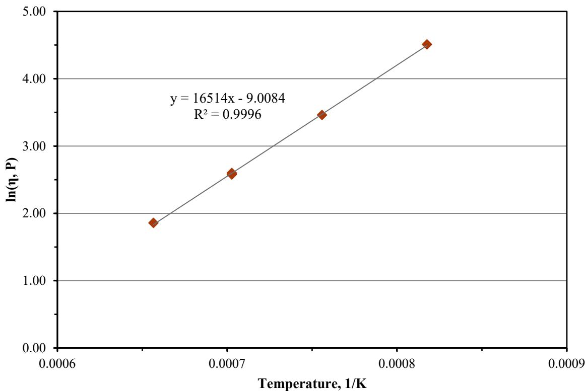
Figure C.29. Viscosity-Temperature Data and Arrhenius Equation Fit for Glass LP2-OL-13
