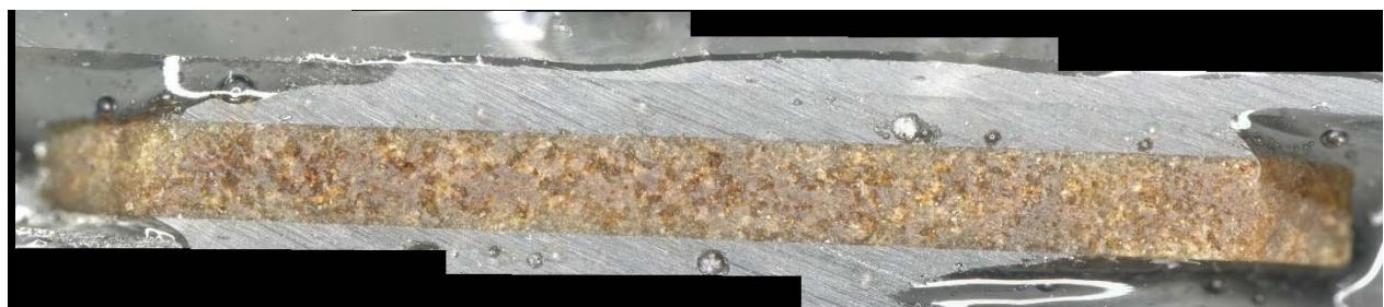
c) Glass cross section magnified after VHT
