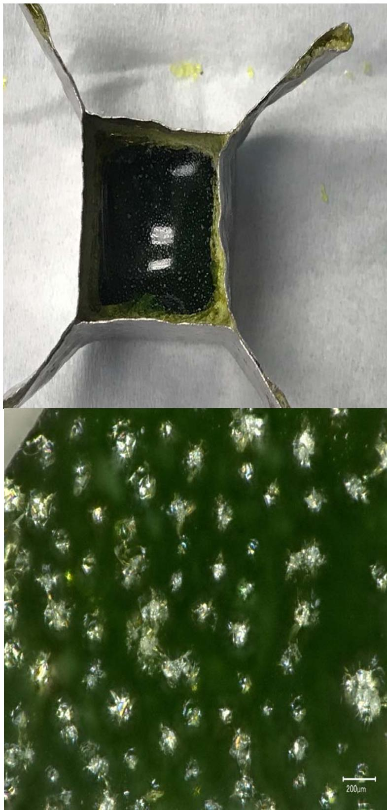
Figure E.7. Glass LP2-IL-08 after CF Heat Treatment at 950 °C for 24 h both in Crucible (top) and Magnified 150X (bottom)
