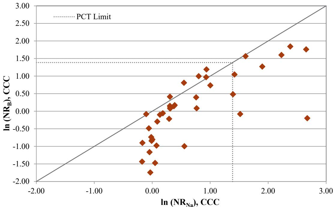
Figure 3.7. Comparison of Natural Logarithms of PCT Normalized Releases of B and Na (g/L) for CCC Samples of Phase 2 Enhanced LAW Glasses
