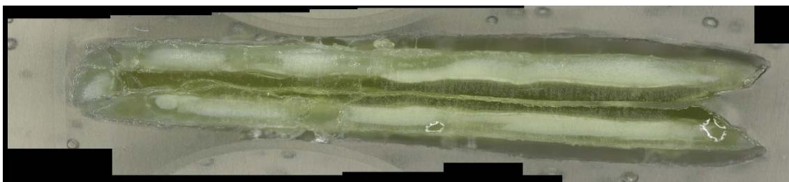
c) Glass cross section magnified after VHT
