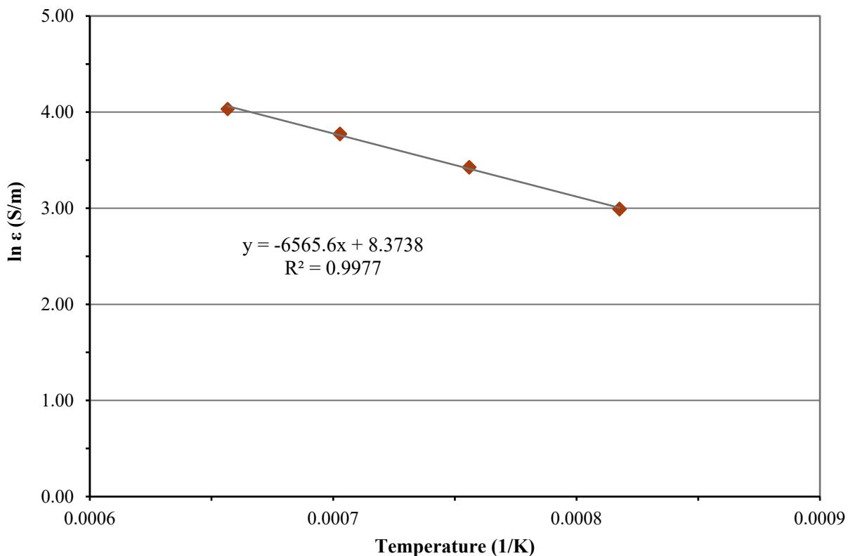
Figure D.34. Electrical Conductivity-Temperature Data and Arrhenius Equation Fit for Glass LP2-OL-18
