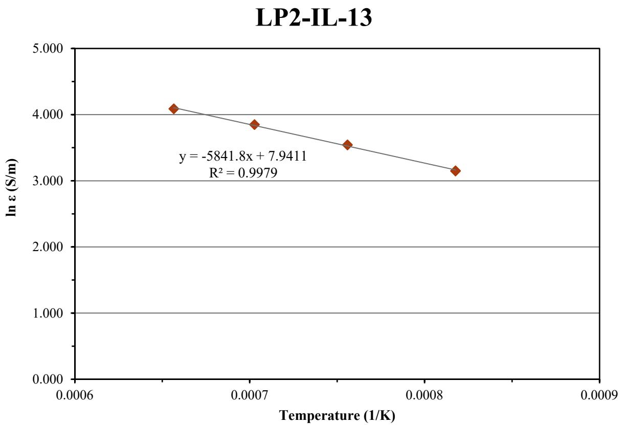
Figure D.13. Electrical Conductivity-Temperature Data and Arrhenius Equation Fit for Glass LP2-IL-13
