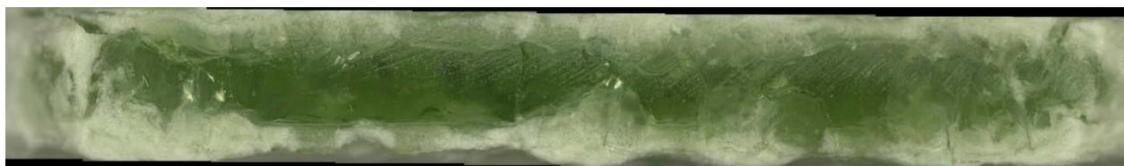
c) Glass cross section magnified after VHT
