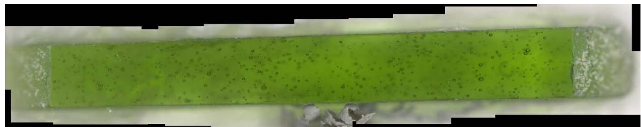
c) Glass cross section magnified after VHT
