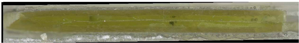
Figure I.34. Quenched Glass LP2-OL-04-1 after VHT for 11 Days
