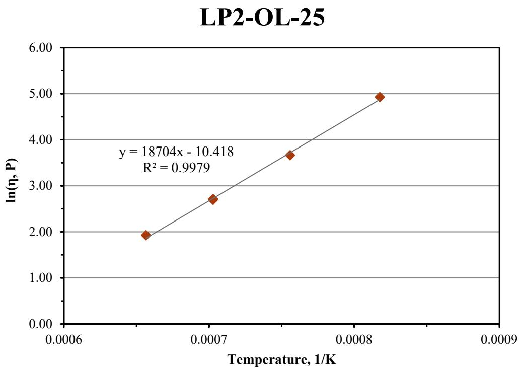
Figure C.41. Viscosity-Temperature Data and Arrhenius Equation Fit for Glass LP2-OL-25
