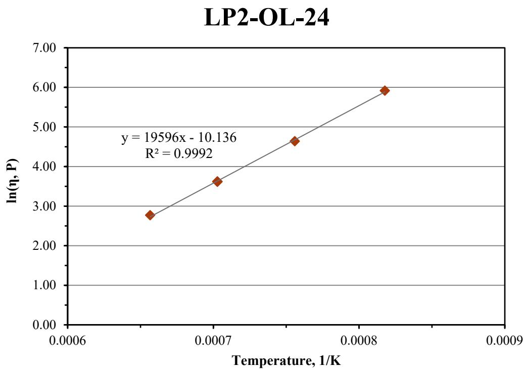
Figure C.40. Viscosity-Temperature Data and Arrhenius Equation Fit for Glass LP2-OL-24
