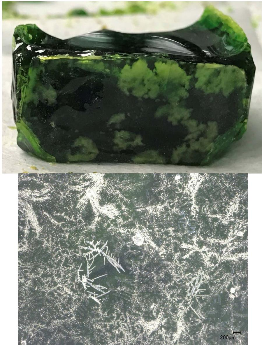
Figure G.1. Glass LP2-IL-01 after CCC Beginning at 1150 °C both Glass (top) and Magnified 50X (bottom)
