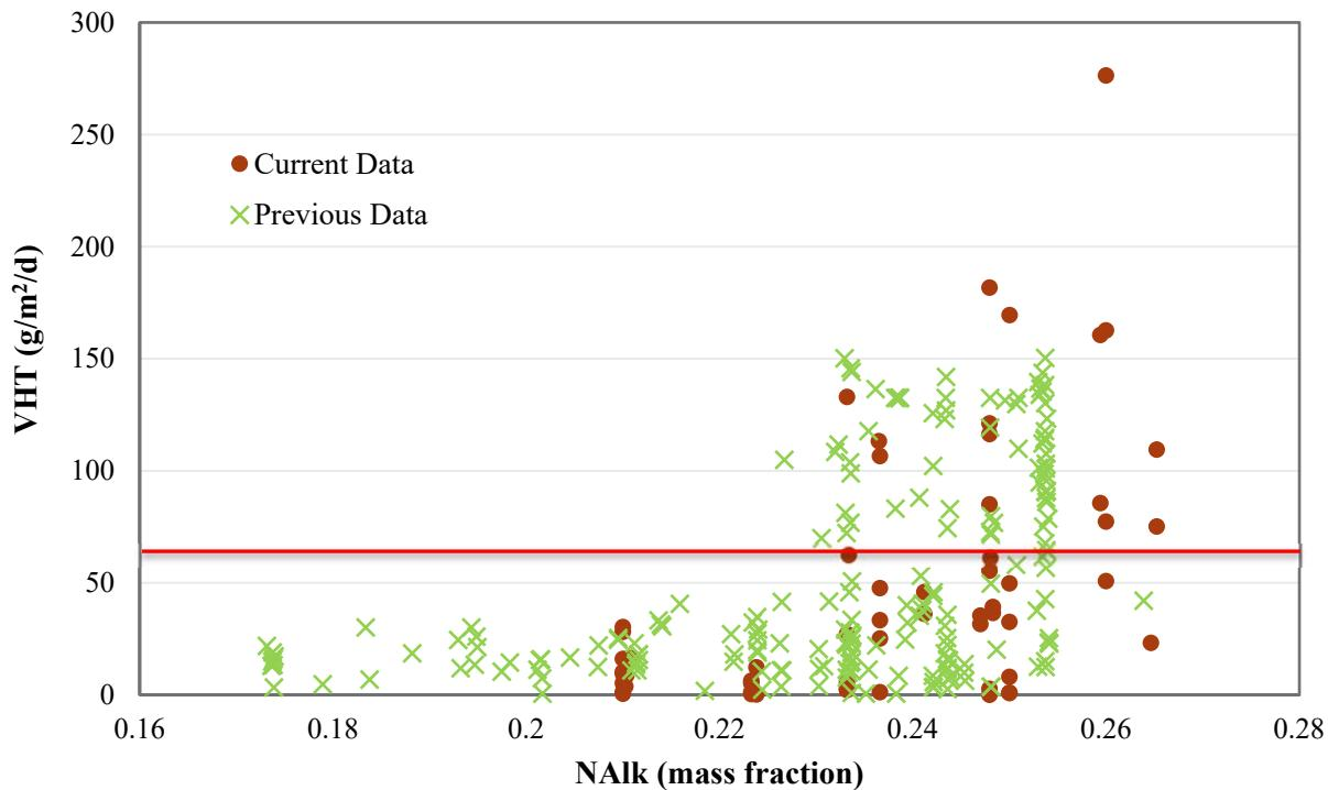
Figure 3.10. VHT Response Compared to the Total Normalized Alkali [ $\text{Nalk} = \text{Na}_2\text{O} + 0.66(\text{K}_2\text{O}) + 2(\text{Li}_2\text{O})$ ] Content of the Glass
