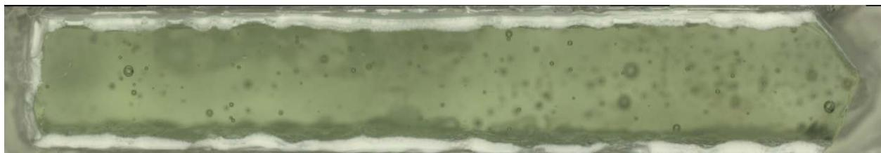
c) Glass cross section magnified after VHT
