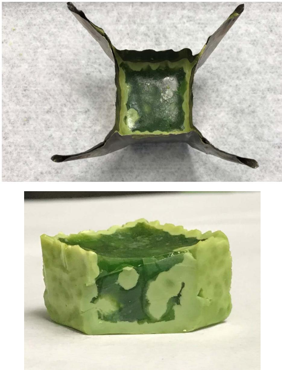
Figure G.22. Glass LP2-OL-05 after CCC Beginning at 1150 °C both in Crucible (top) and Glass (bottom)
