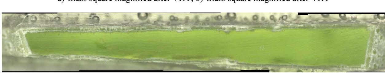
Figure I.89. CCC-Treated Glass LP2-IL-14 after VHT for 7 Days
