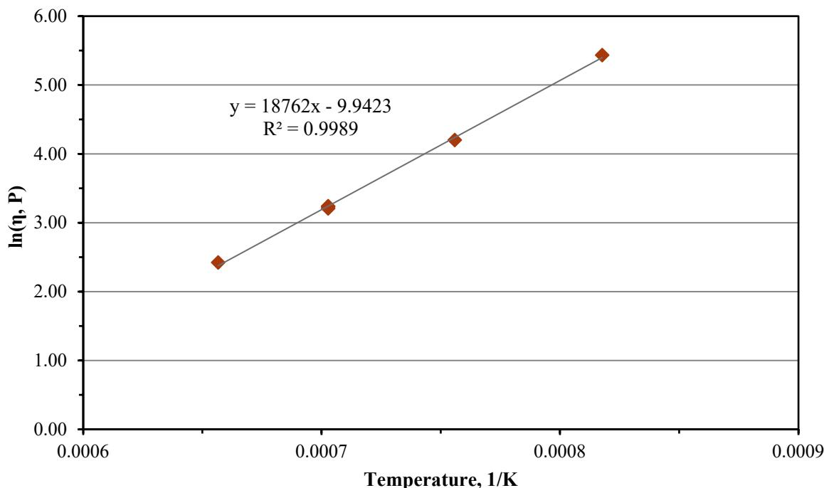
Figure C.33. Viscosity-Temperature Data and Arrhenius Equation Fit for Glass LP2-OL-17
