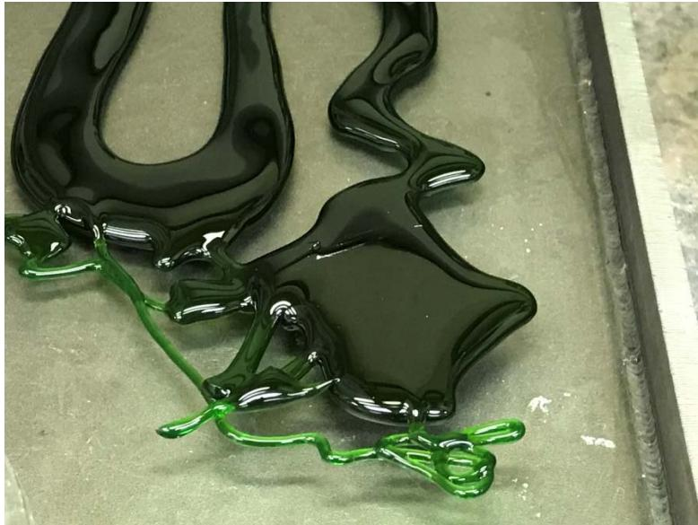
Figure A.1. Photo of Glass LP2-IL-01 Morphology of Second Melt at 1150 °C for 1.5 h
