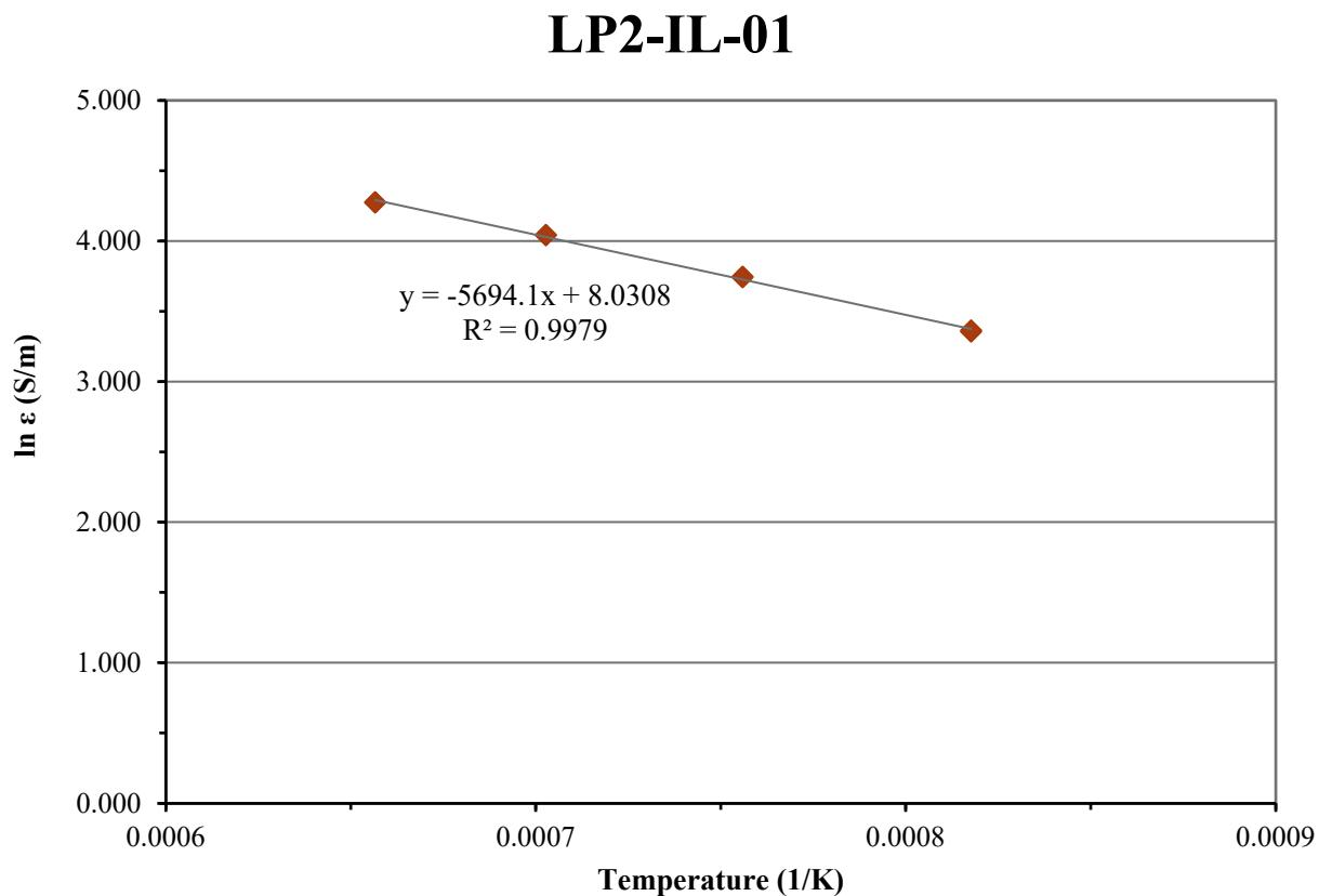
Figure D.1. Electrical Conductivity-Temperature Data and Arrhenius Equation Fit for Glass LP2-IL-01
