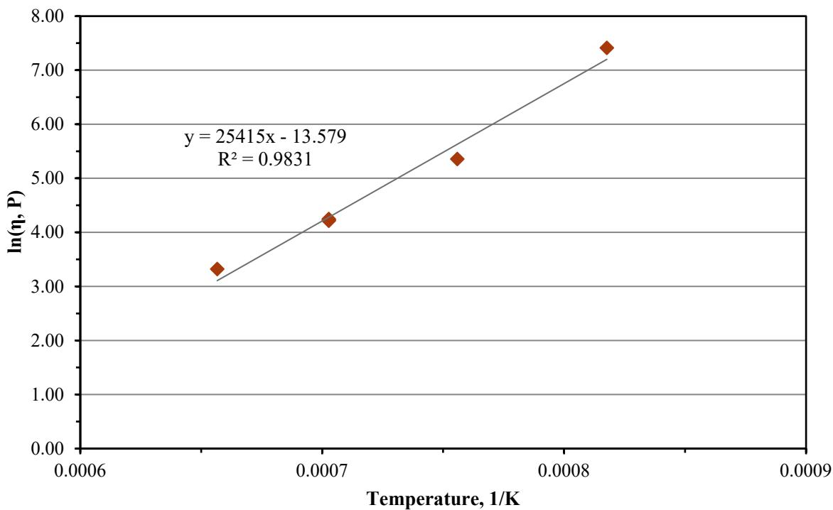
Figure C.22. Viscosity-Temperature Data and Arrhenius Equation Fit for Glass LP2-OL-05
