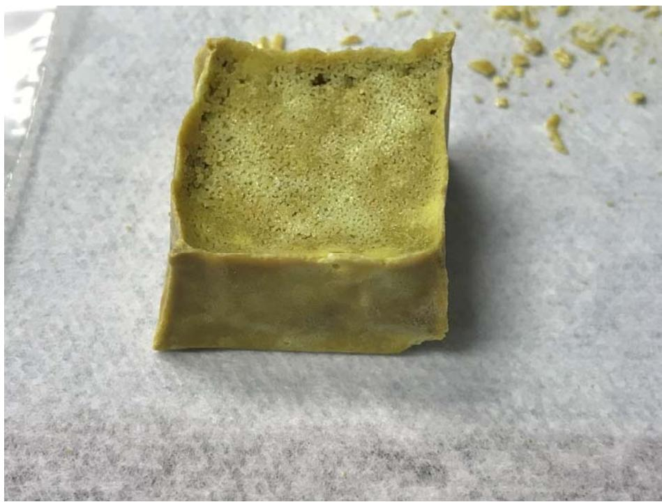
Figure G.24. Glass LP2-OL-08MOD after CCC Beginning at 1150 °C
