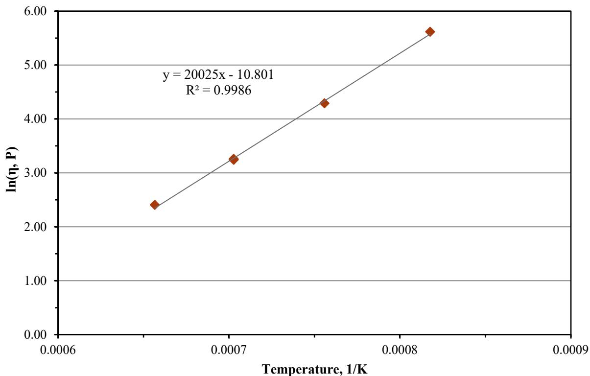
Figure C.20. Viscosity-Temperature Data and Arrhenius Equation Fit for Glass LP2-OL-03 MOD2
