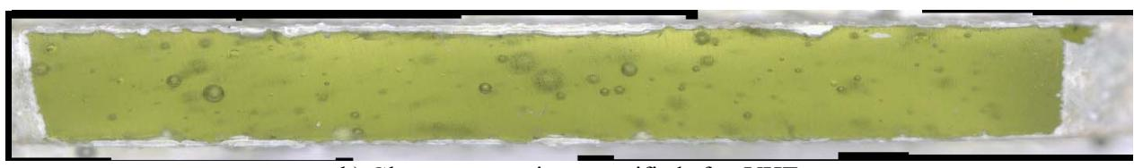
b) Glass cross section magnified after VHT
