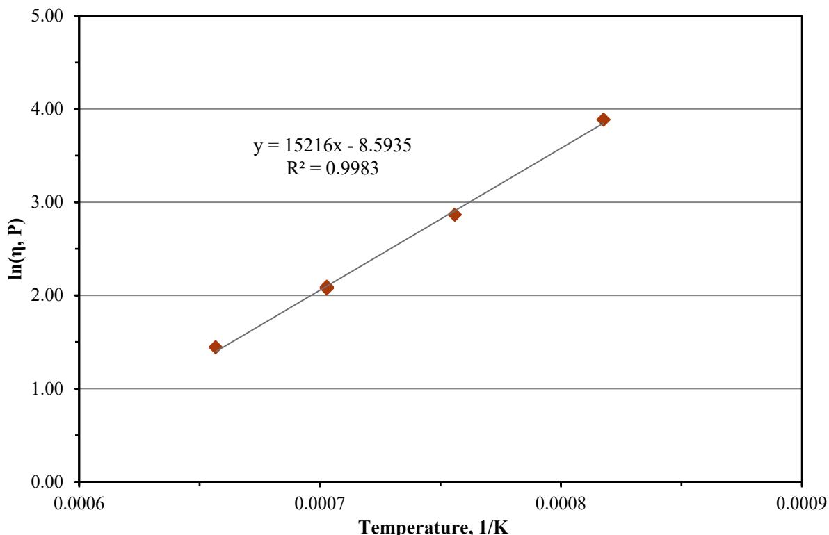
Figure C.28. Viscosity-Temperature Data and Arrhenius Equation Fit for Glass LP2-OL-12
