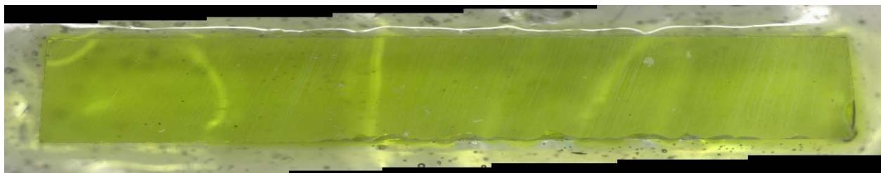
c) Glass cross section magnified after VHT
