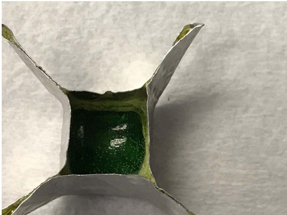
Figure E.1. Glass LP2-IL-02 after CF Heat Treatment at 950 °C for 24 h
