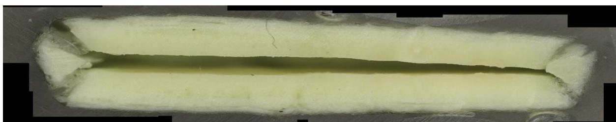
b) Glass cross section magnified after VHT
