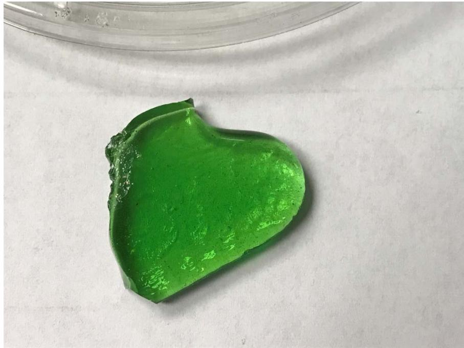
Figure A.17. Photo of Glass LP2-IL-17 Morphology of Second Melt at 1150 °C for 1.5 h
