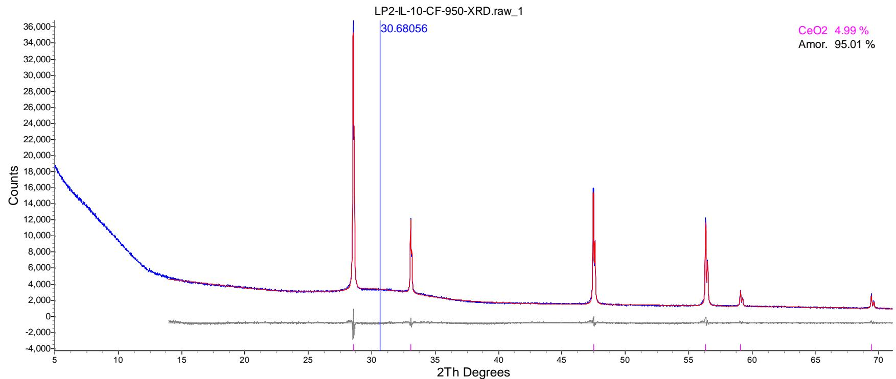
Figure F.8. XRD Spectrum of Heat-Treated Glass LP2-IL-10
