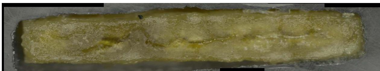
c) Glass cross section magnified after VHT
