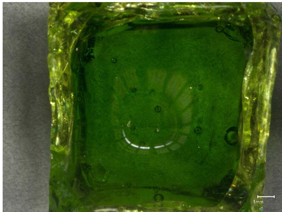
Figure E.11. Glass LP2-IL-12 after CF Heat Treatment at 950 °C for 24 h Magnified 20X
