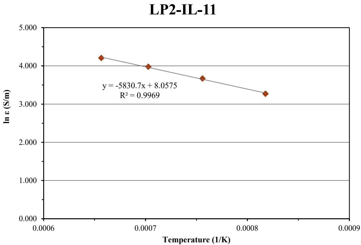
Figure D.11. Electrical Conductivity-Temperature Data and Arrhenius Equation Fit for Glass LP2-IL-11
