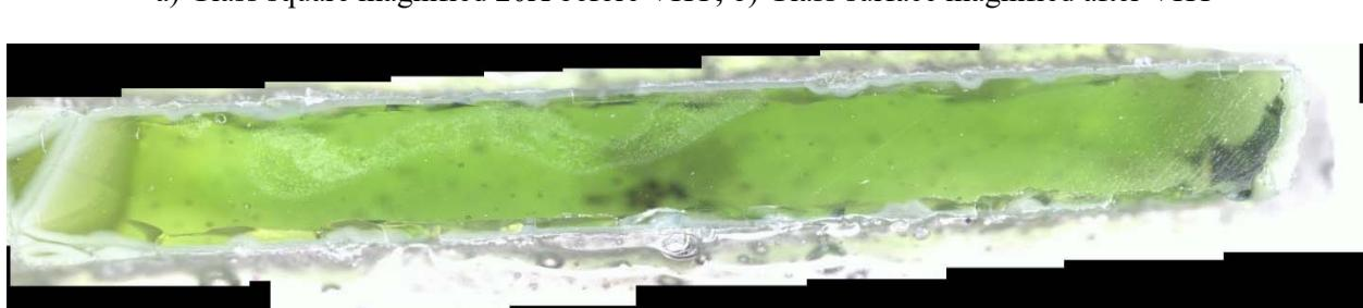
Figure I.91. CCC-Treated Glass LP2-IL-15 after VHT for 24 Days
