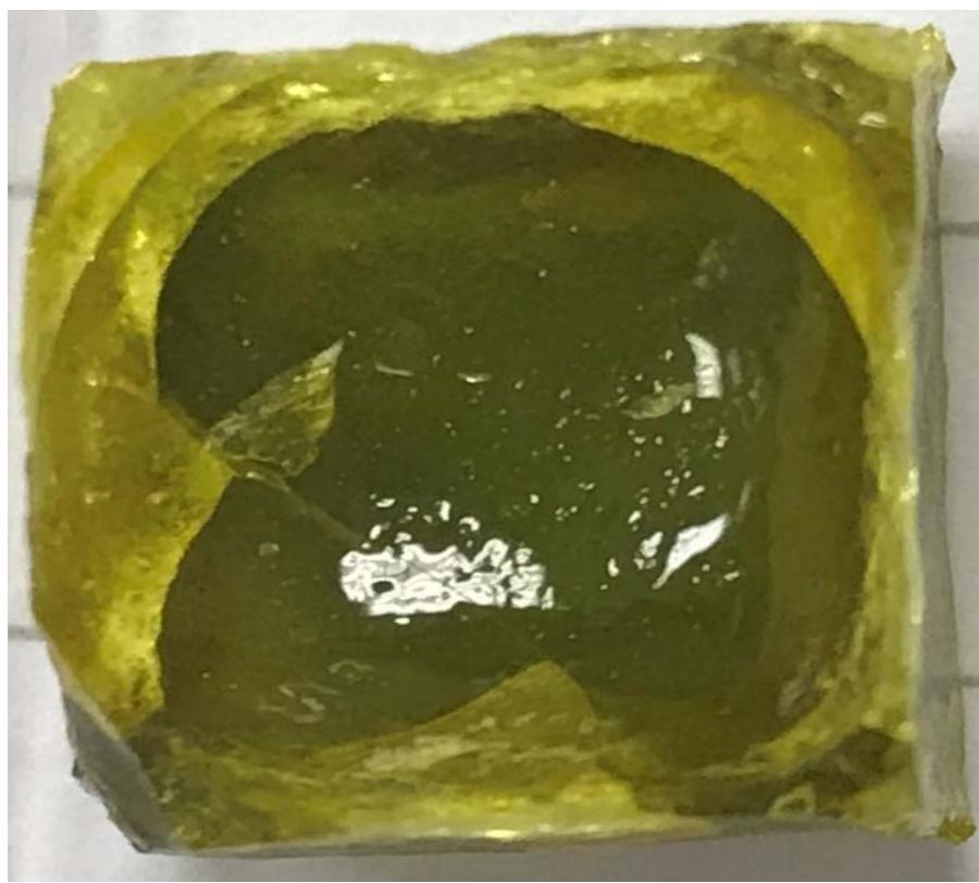
Figure E.39. Glass LP2-OL-24 after CF Heat Treatment at 950 °C for 24 h
