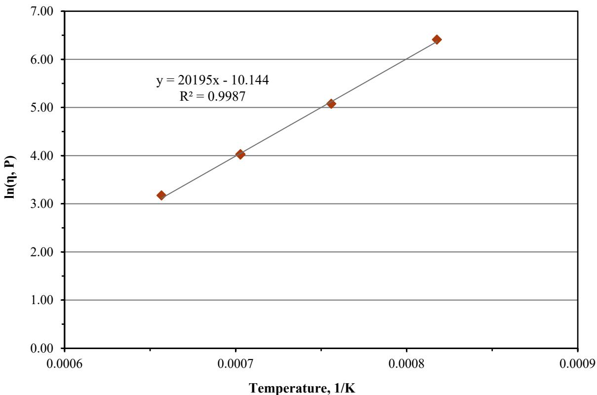
Figure C.13. Viscosity-Temperature Data and Arrhenius Equation Fit for Glass LP2-IL-13
