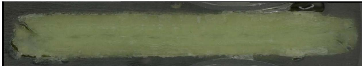
c) Glass cross section magnified after VHT
