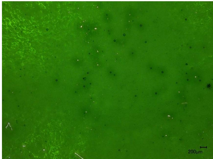
Figure A.5. Photo of Glass LP2-IL-05 Morphology of Second Melt at 1150 °C for 1.5 h
