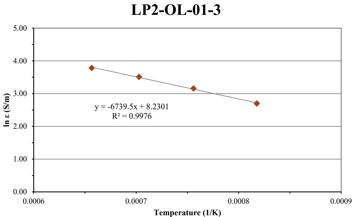
Figure D.18. Electrical Conductivity-Temperature Data and Arrhenius Equation Fit for Glass LP2-OL-01-3
