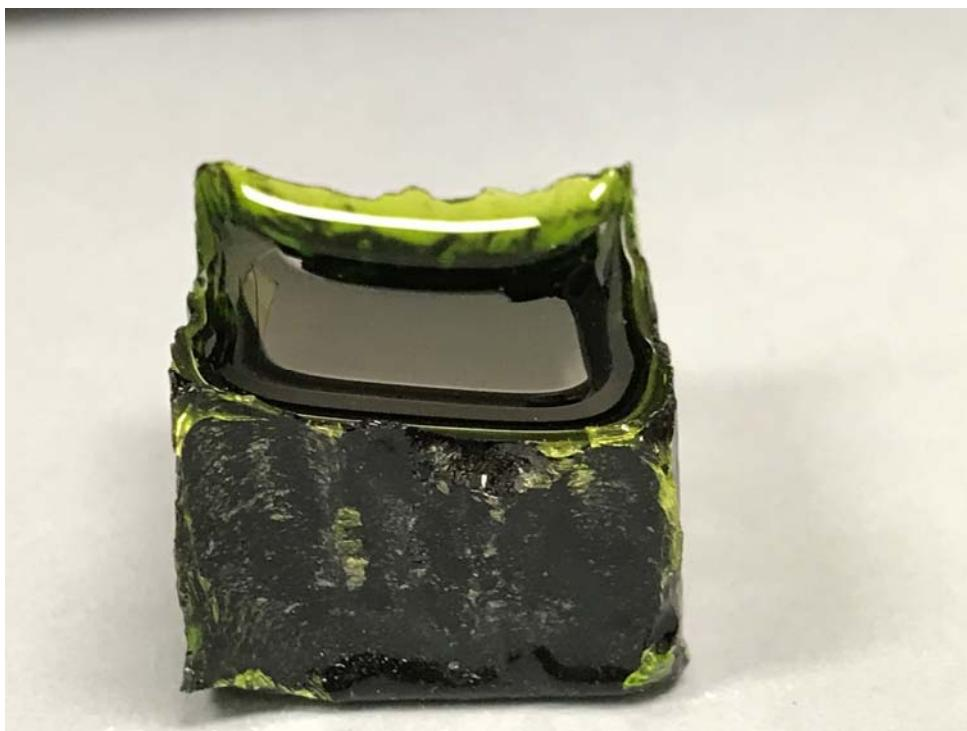
Figure G.31. Glass LP2-OL-15 after CCC Beginning at 1150 °C
