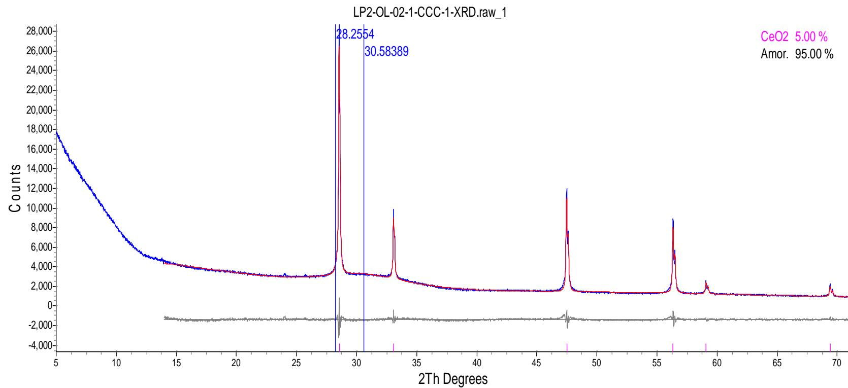
Figure H.7. XRD Spectrum of CCC-Treated Glass LP2-OL-02-1
