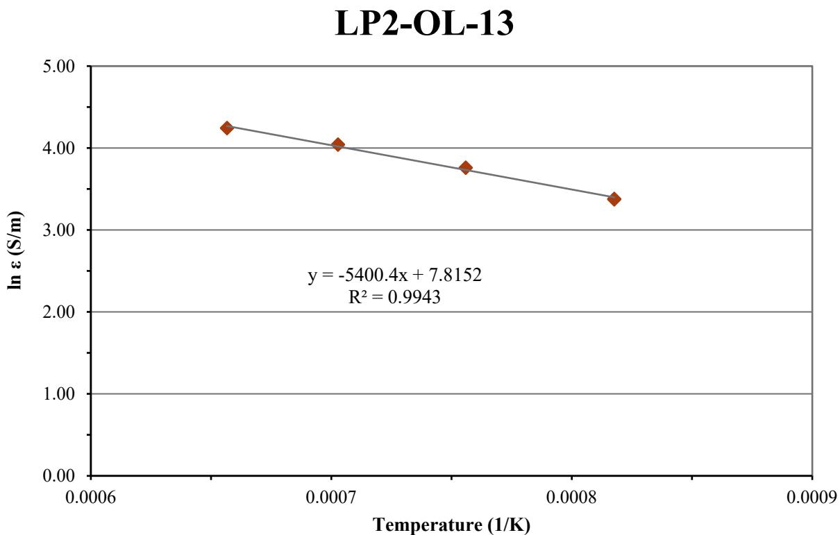
Figure D.29. Electrical Conductivity-Temperature Data and Arrhenius Equation Fit for Glass LP2-OL-13
