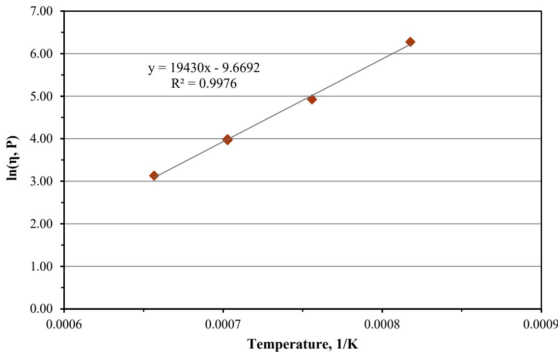
Figure C.19. Viscosity-Temperature Data and Arrhenius Equation Fit for Glass LP2-OL-02-1
