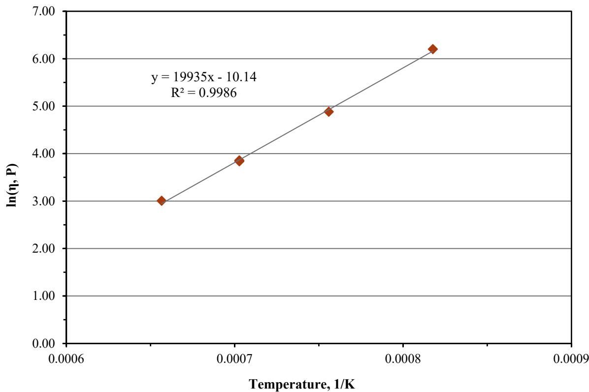
Figure C.6. Viscosity-Temperature Data and Arrhenius Equation Fit for Glass LP2-IL-06
