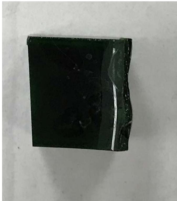
Figure G.16. Glass LP2-IL-16 after CCC Beginning at 1150 °C
