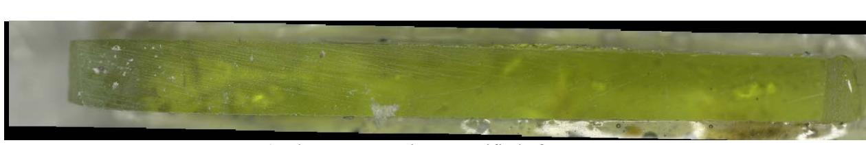
Figure I.103. CCC-Treated Glass LP2-OL-07-1 after VHT for 24 Days
