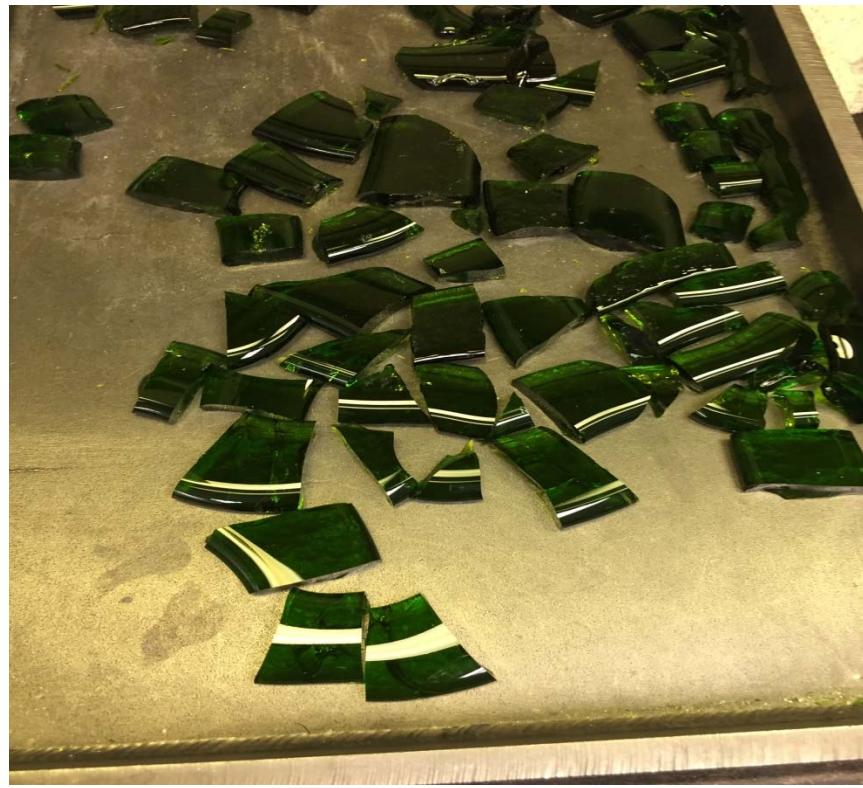
Figure A.18. Photo of Glass LP2-OL-01-3 Morphology of Second Melt at 1150 °C for 1.5 h
