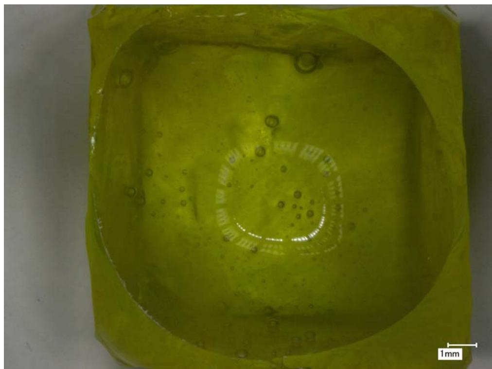
Figure E.34. Glass LP2-OL-19 after CF Heat Treatment at 950 °C for 24 h Magnified 20X
