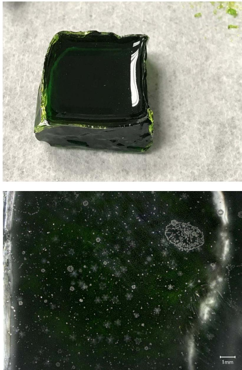
Figure G.11. Glass LP2-IL-11 CCC Beginning at 1150 °C both Glass (top) and Magnified 20X (bottom)
