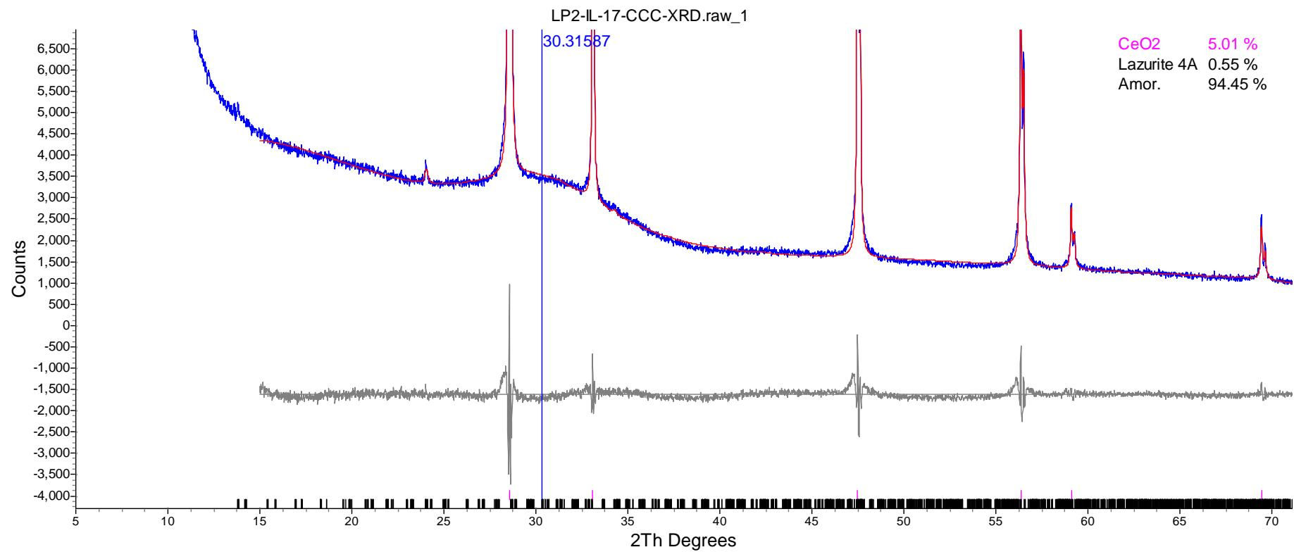
Figure H.6. XRD Spectrum of CCC-Treated Glass LP2-IL-17
