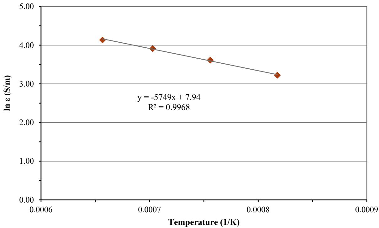
Figure D.37. Electrical Conductivity-Temperature Data and Arrhenius Equation Fit for Glass LP2-OL-21
