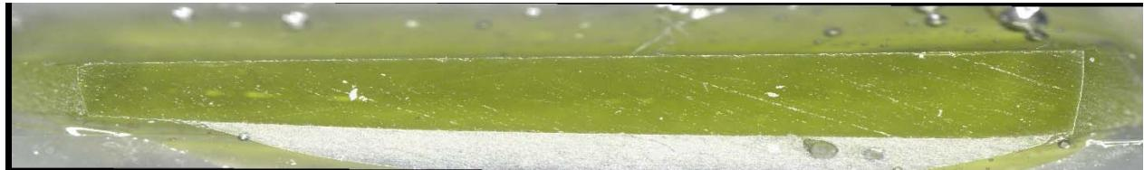
c) Glass cross section magnified after VHT
