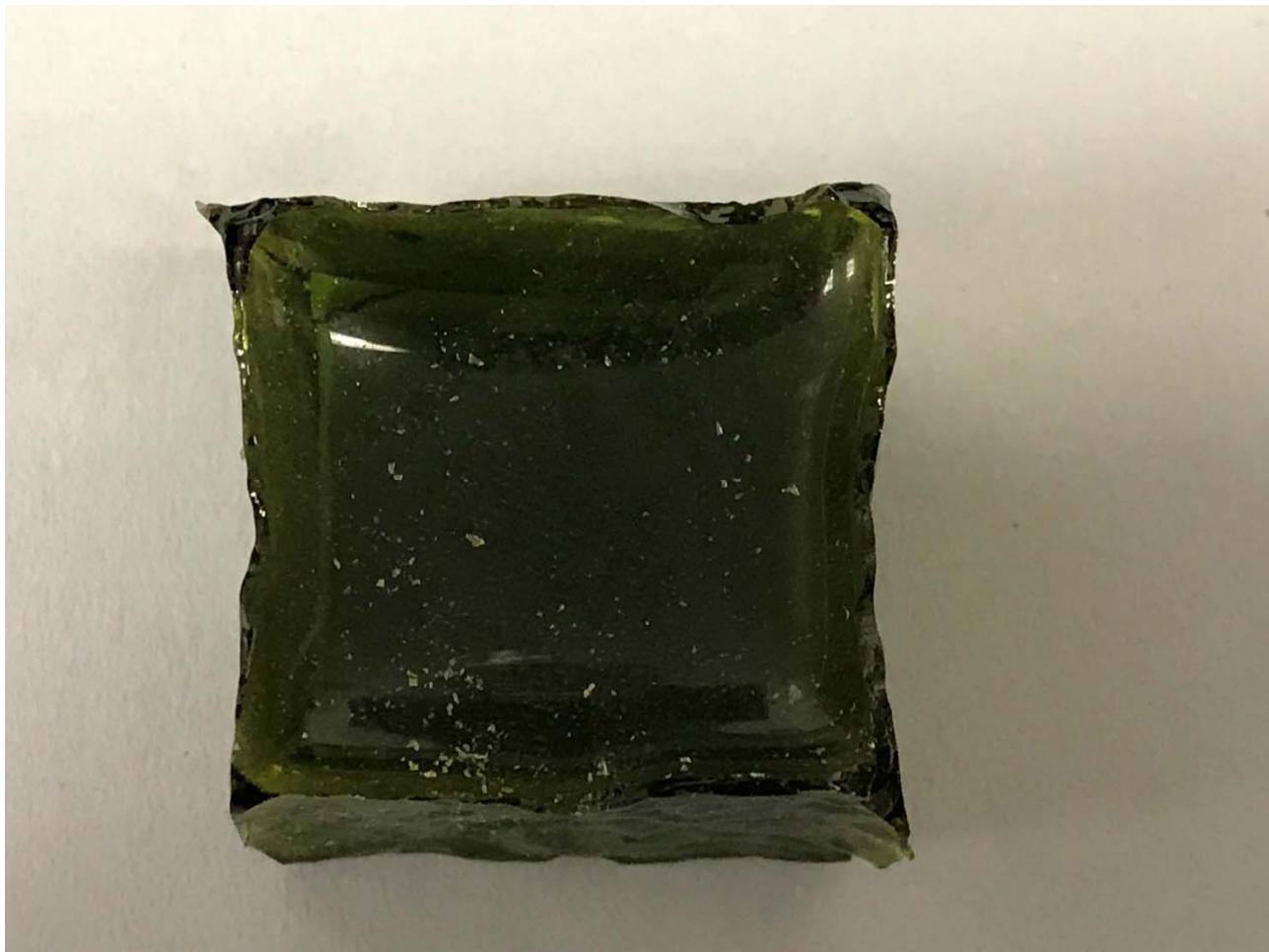
Figure G.41. Glass LP2-OL-25 after CCC Beginning at 1150 °C
