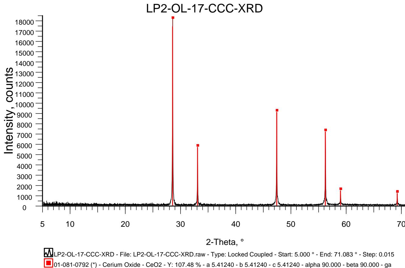
Figure H.17. XRD Spectrum of CCC-Treated Glass LP2-OL-17
