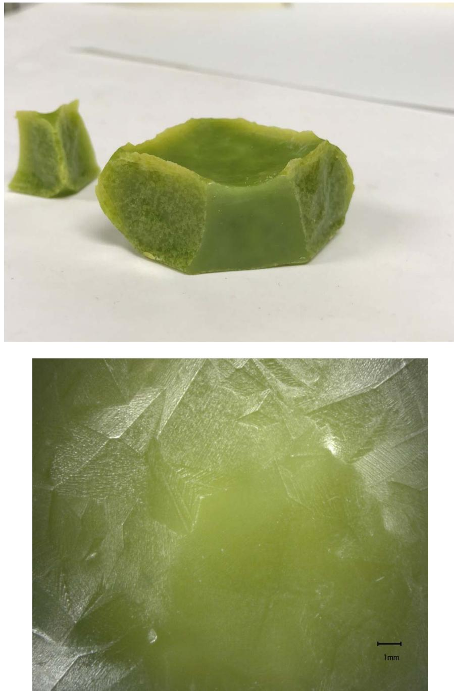
Figure G.40. Glass LP2-OL-24 after CCC Beginning at 1150 °C both Glass (top) and Magnified 20X (bottom)
