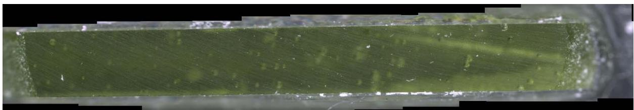
b) Glass cross section magnified after VHT
