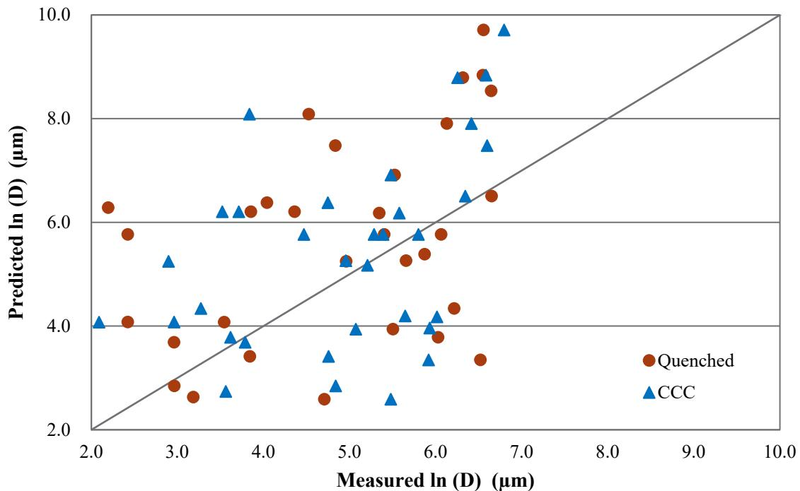
Figure 3.13. Natural Logarithm of VHT Alteration Depth Results Predicted using 16-Term Reduced Partial Quadratic Mixture Model Versus Measured VHT Values for Phase 2 Enhanced LAW Glasses
