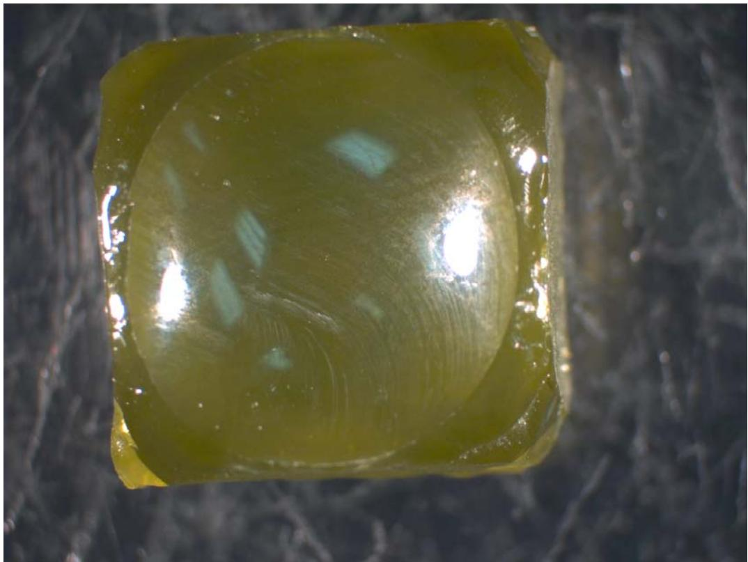
Figure E.22. Glass LP2-OL-07-1 after CF Heat Treatment at 950 °C for 24 h
