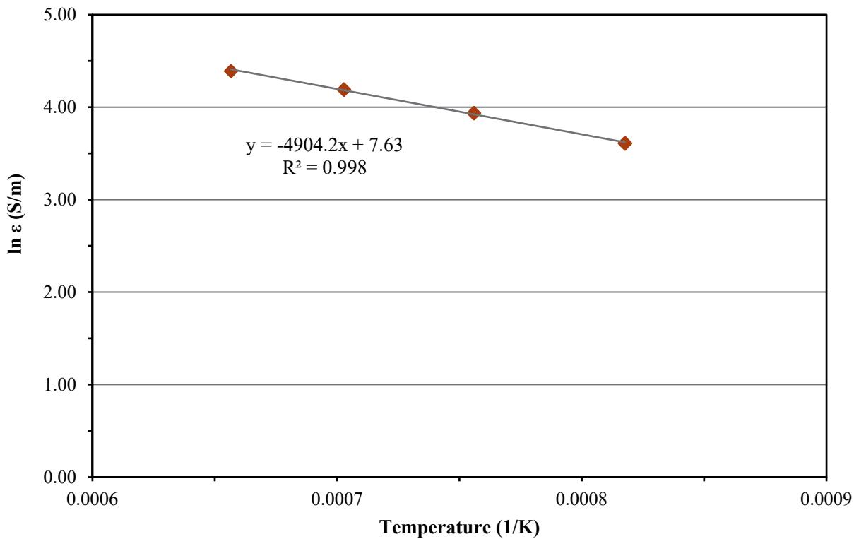
Figure D.24. Electrical Conductivity-Temperature Data and Arrhenius Equation Fit for Glass LP2-OL-08 MOD
