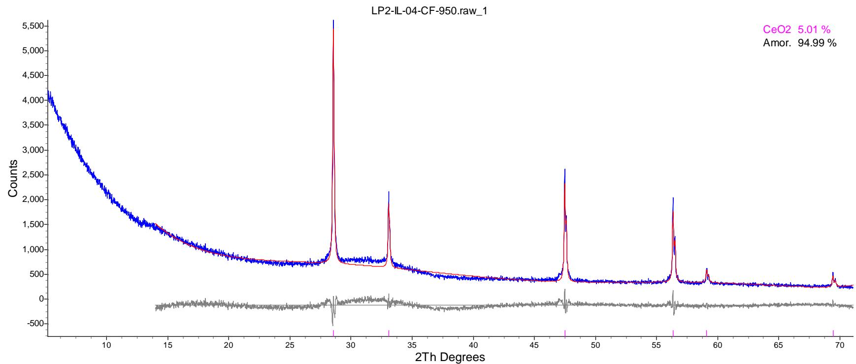
Figure F.4. XRD Spectrum of Heat-Treated Glass LP2-IL-04
