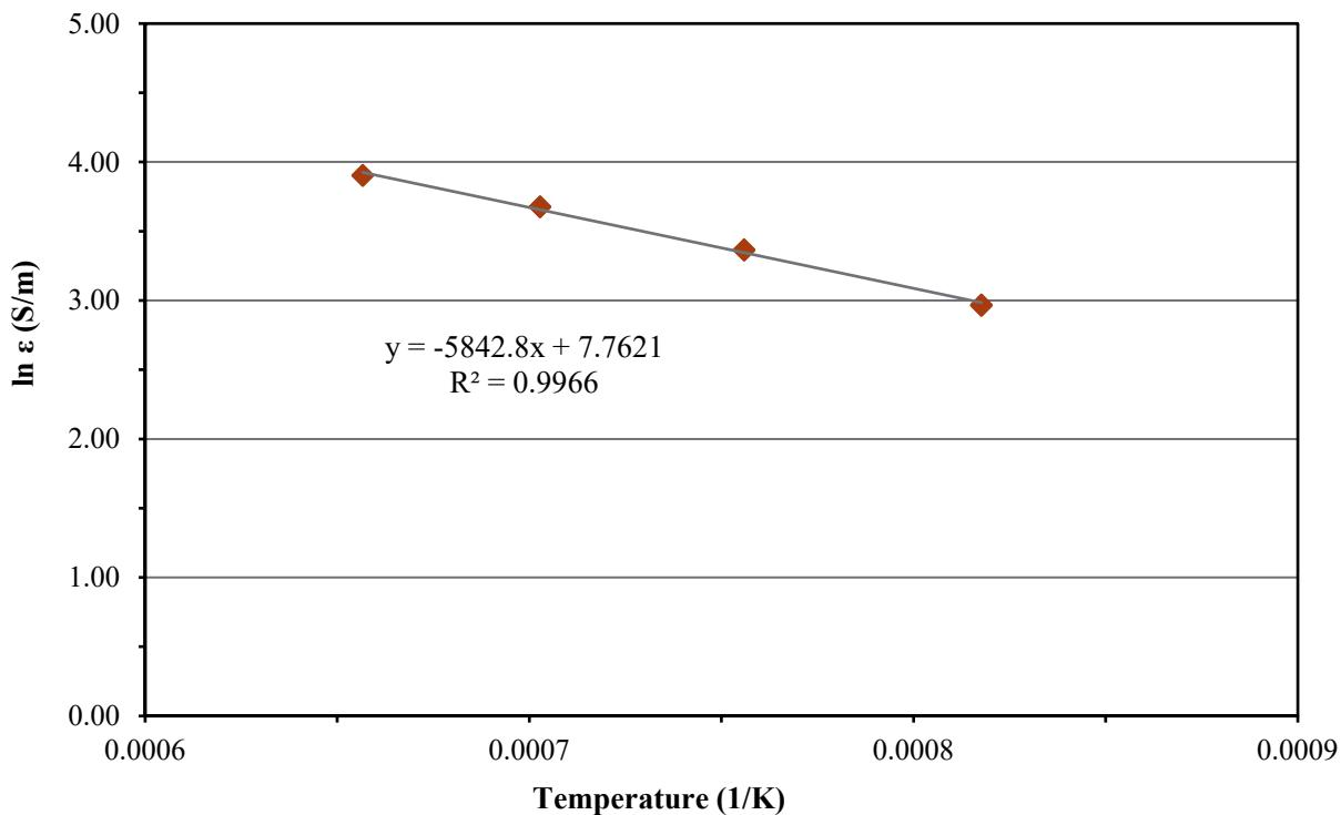
Figure D.25. Electrical Conductivity-Temperature Data and Arrhenius Equation Fit for Glass LP2-OL-09-1
