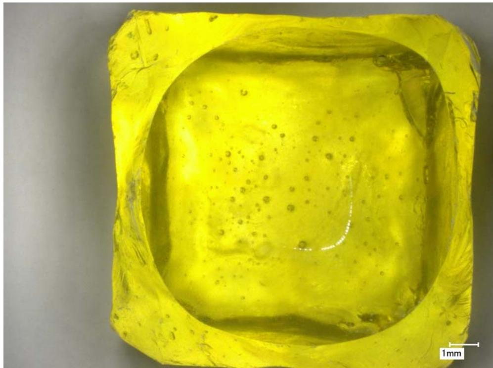
Figure E.28. Glass LP2-OL-13 after CF Heat Treatment at 950 °C for 24 h Magnified 20X
