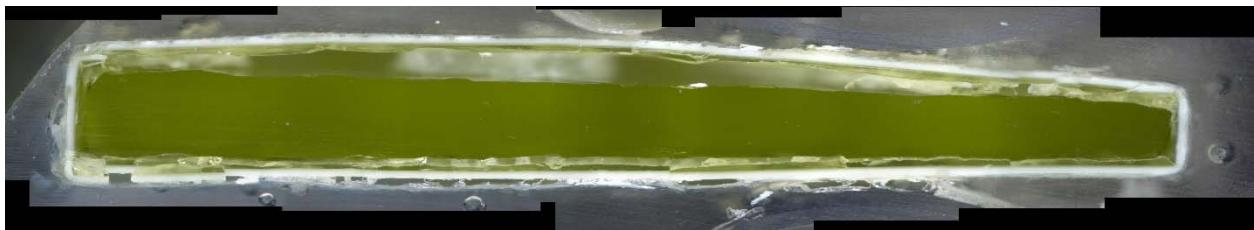
b) Glass cross section magnified after VHT
