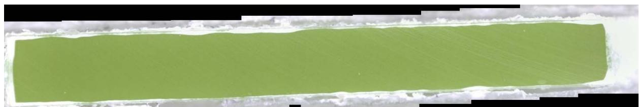
b) Glass cross section magnified after VHT
