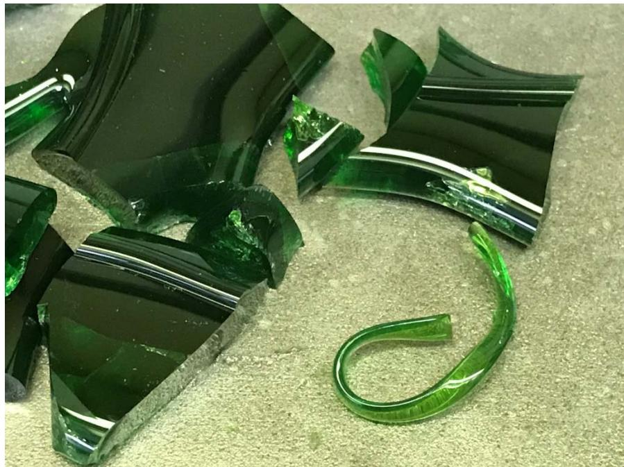
Figure A.3. Photo of Glass LP2-IL-03 Morphology of Second Melt at 1150 °C for 1.5 h
