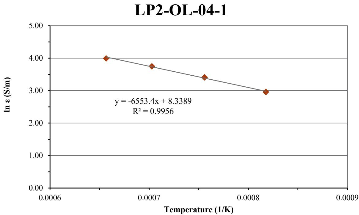
Figure D.21. Electrical Conductivity-Temperature Data and Arrhenius Equation Fit for Glass LP2-OL-04-1
