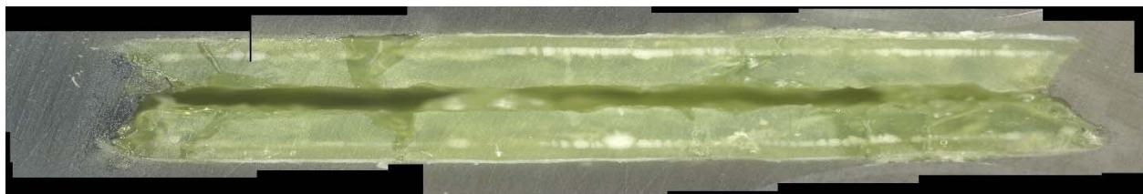
b) Glass cross section magnified after VHT
