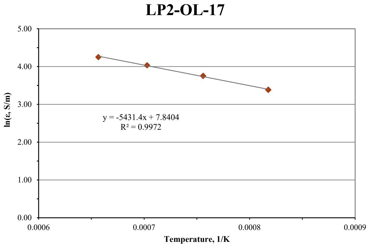
Figure D.33. Electrical Conductivity-Temperature Data and Arrhenius Equation Fit for Glass LP2-OL-17
