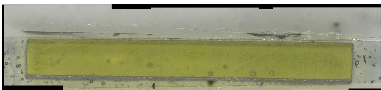
Figure I.35. Quenched Glass LP2-OL-04-1 after VHT for 24 Days
