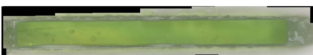
c) Glass cross section magnified after VHT
