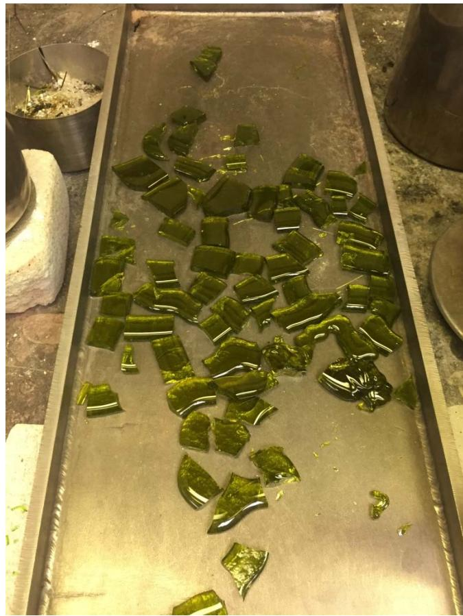
Figure A.35. Photo of Glass LP2-OL-19 Morphology of Second Melt at 1150 °C for 1.5 h
