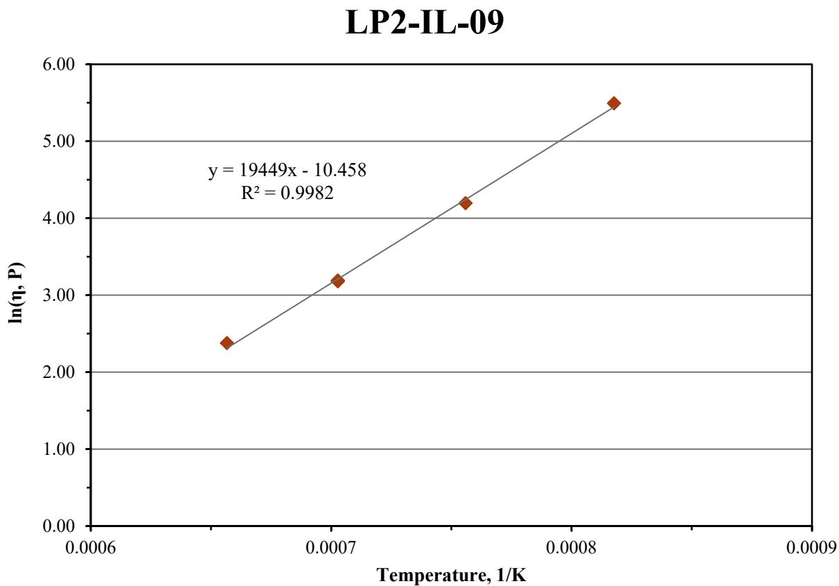
Figure C.9. Viscosity-Temperature Data and Arrhenius Equation Fit for Glass LP2-IL-09
