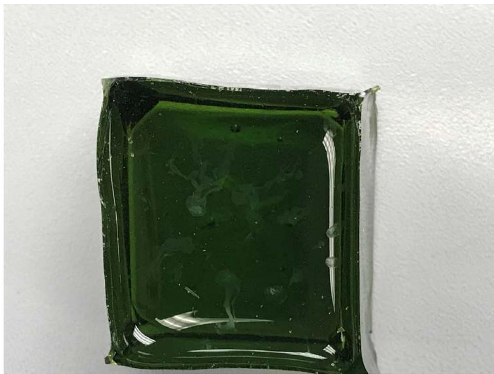
Figure G.35. Glass LP2-OL-19 after CCC Beginning at 1150 °C
