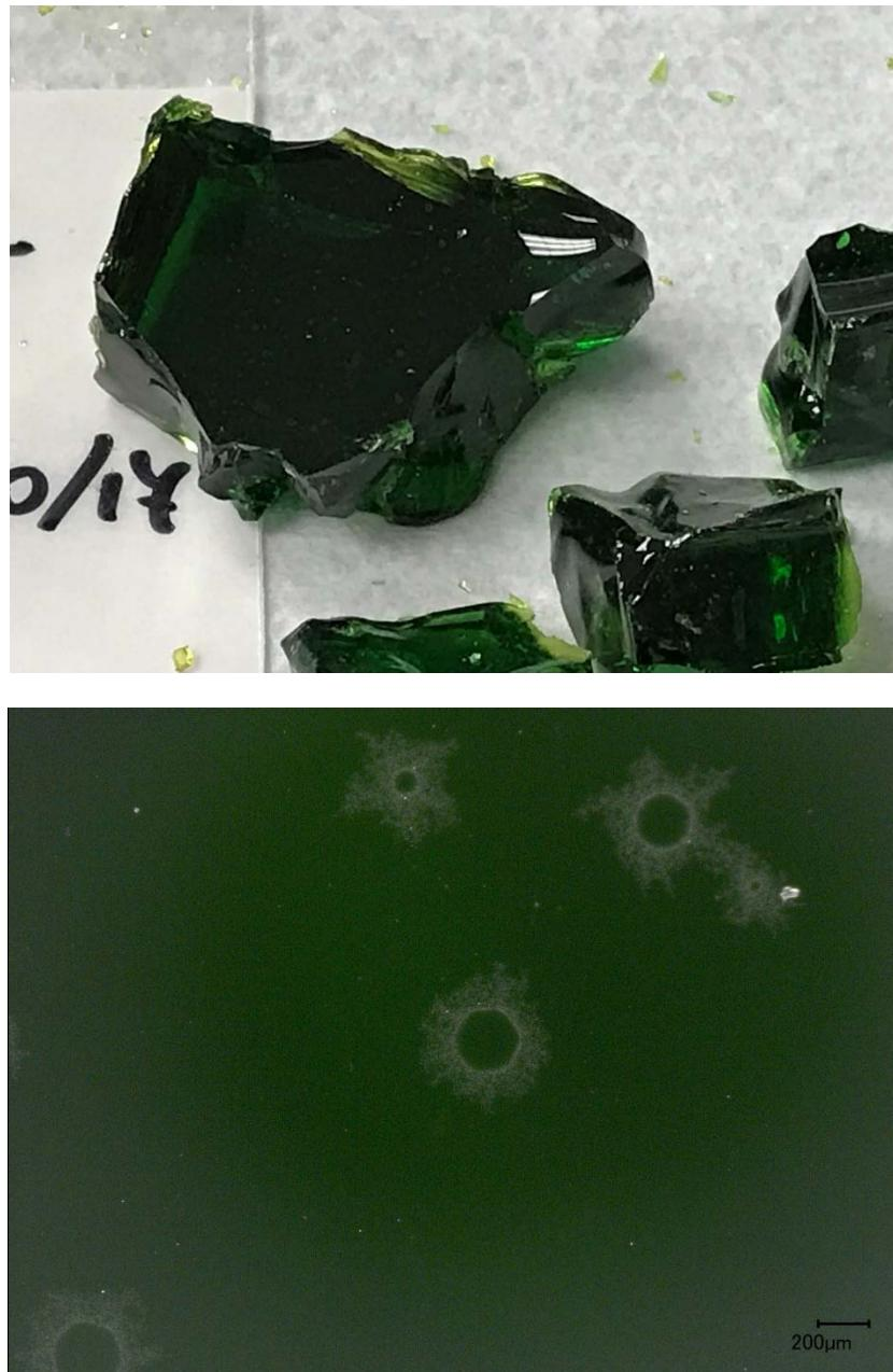
Figure G.5. Glass LP2-IL-05 CCC Beginning at 1150 °C both Glass (top) and Magnified 100X (bottom)
