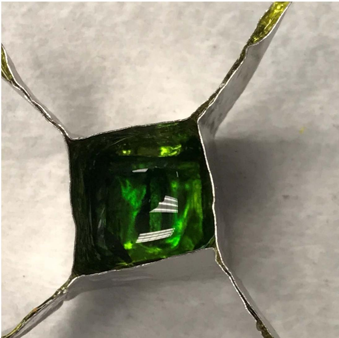
Figure E.4. Glass LP2-IL-05 after CF Heat Treatment at 950 °C for 24 h
