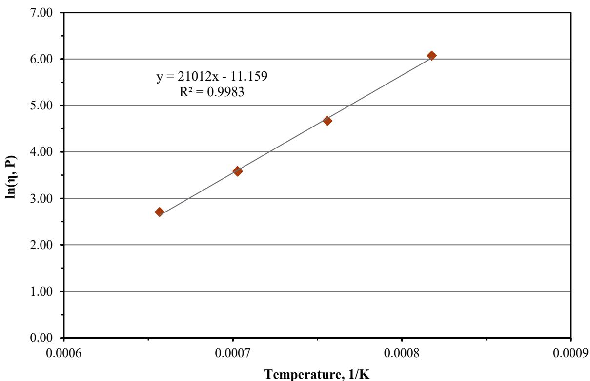
Figure C.8. Viscosity-Temperature Data and Arrhenius Equation Fit for Glass LP2-IL-08
