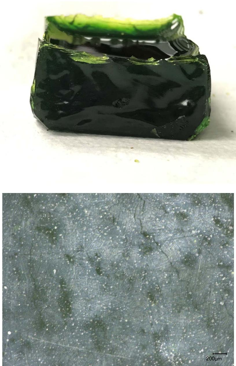
Figure G.3. Glass LP2-IL-03 after CCC Beginning at 1150 °C both Glass (top) and Magnified 100X (bottom)
