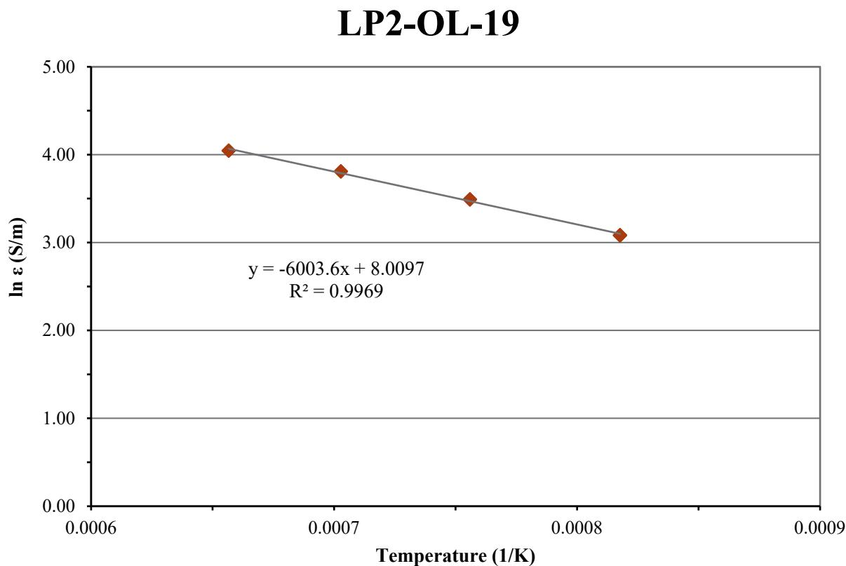
Figure D.35. Electrical Conductivity-Temperature Data and Arrhenius Equation Fit for Glass LP2-OL-19
