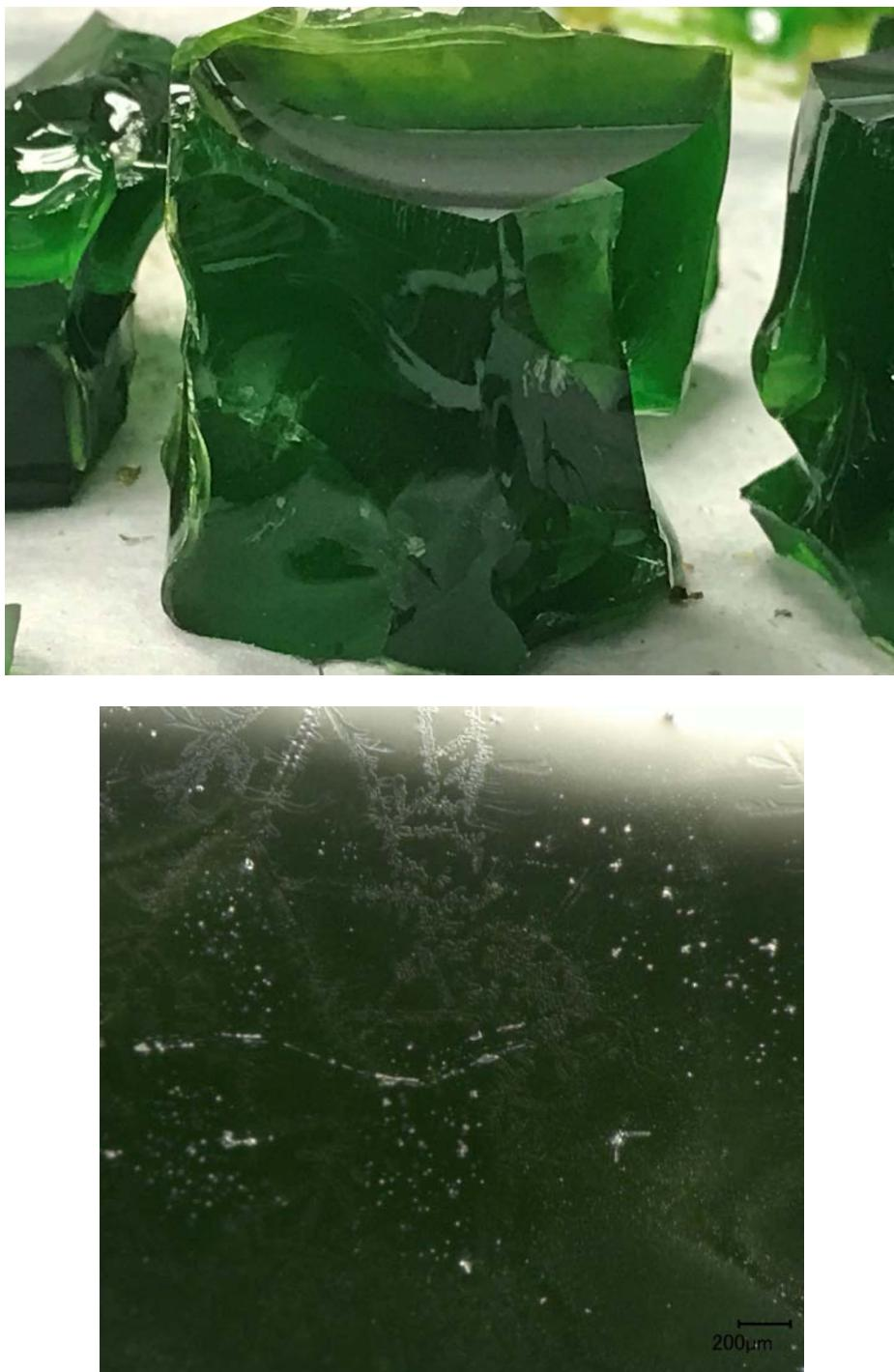
Figure G.2. Glass LP2-IL-02 after CCC Beginning at 1150 °C both Glass (top) and Magnified 100X (bottom)
