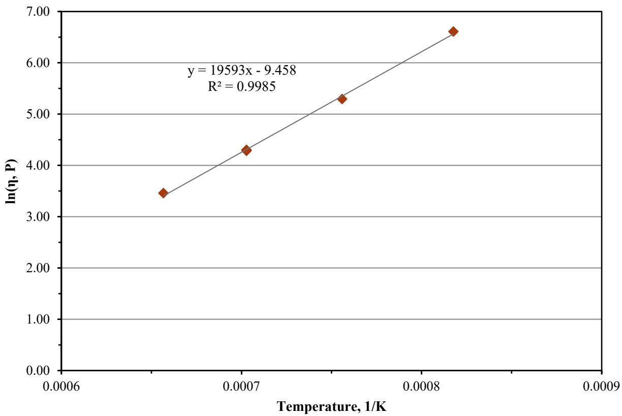
Figure C.32. Viscosity-Temperature Data and Arrhenius Equation Fit for Glass LP2-OL-16 MOD
