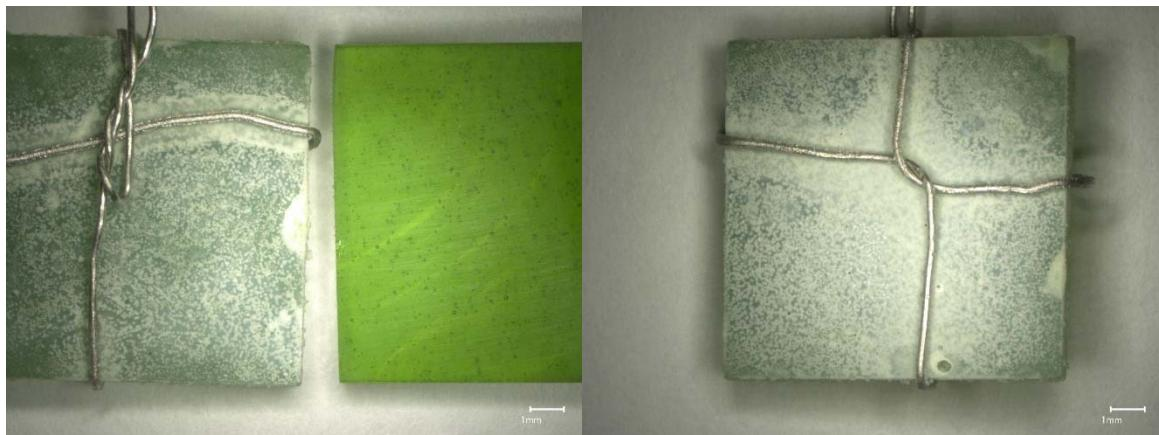
a) Glass square after (left) and before (right) VHT; b) Glass square after VHT
