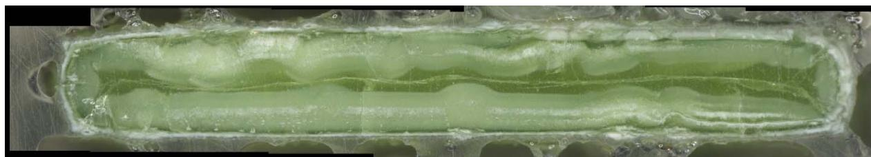
c) Glass cross section magnified after VHT
