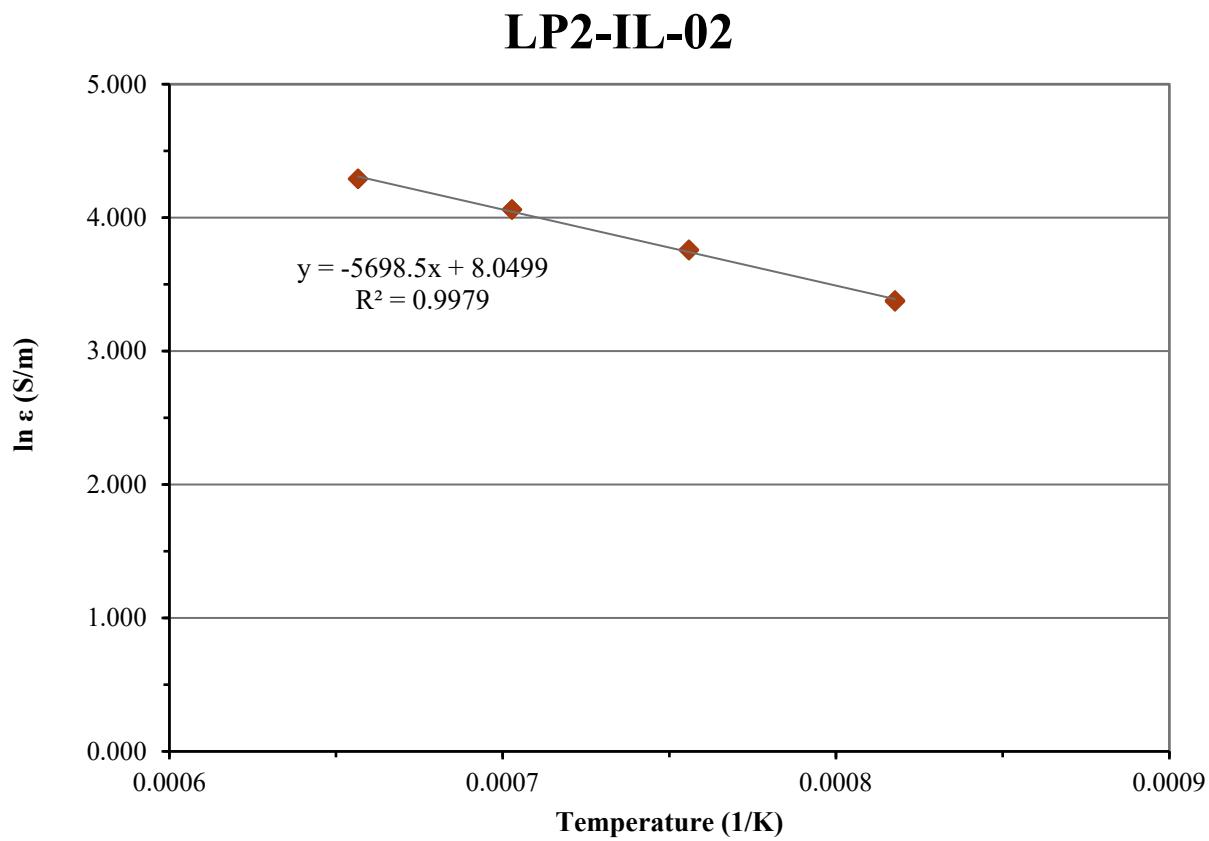
Figure D.2. Electrical Conductivity-Temperature Data and Arrhenius Equation Fit for Glass LP2-IL-02
