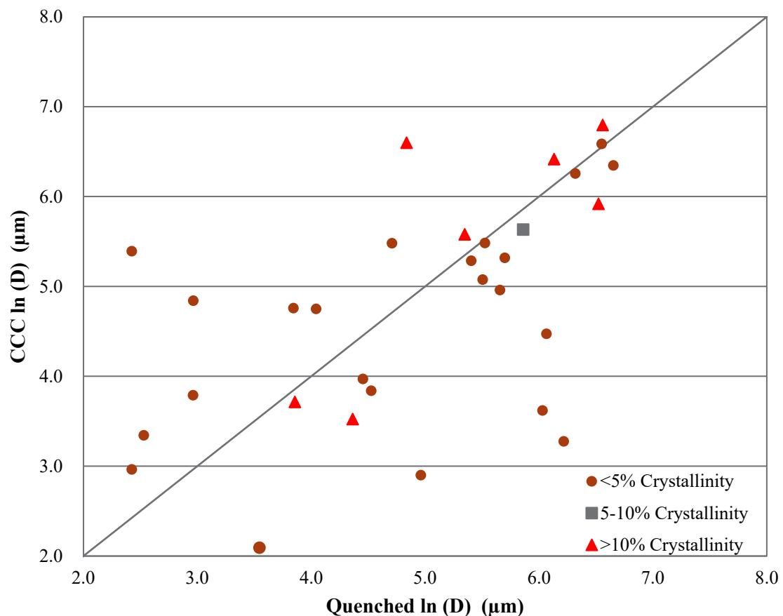
Figure 3.11 Natural Logarithm of VHT Alteration Depth Results for CCC versus Quenched Versions of Phase 2 Enhanced LAW Glasses
