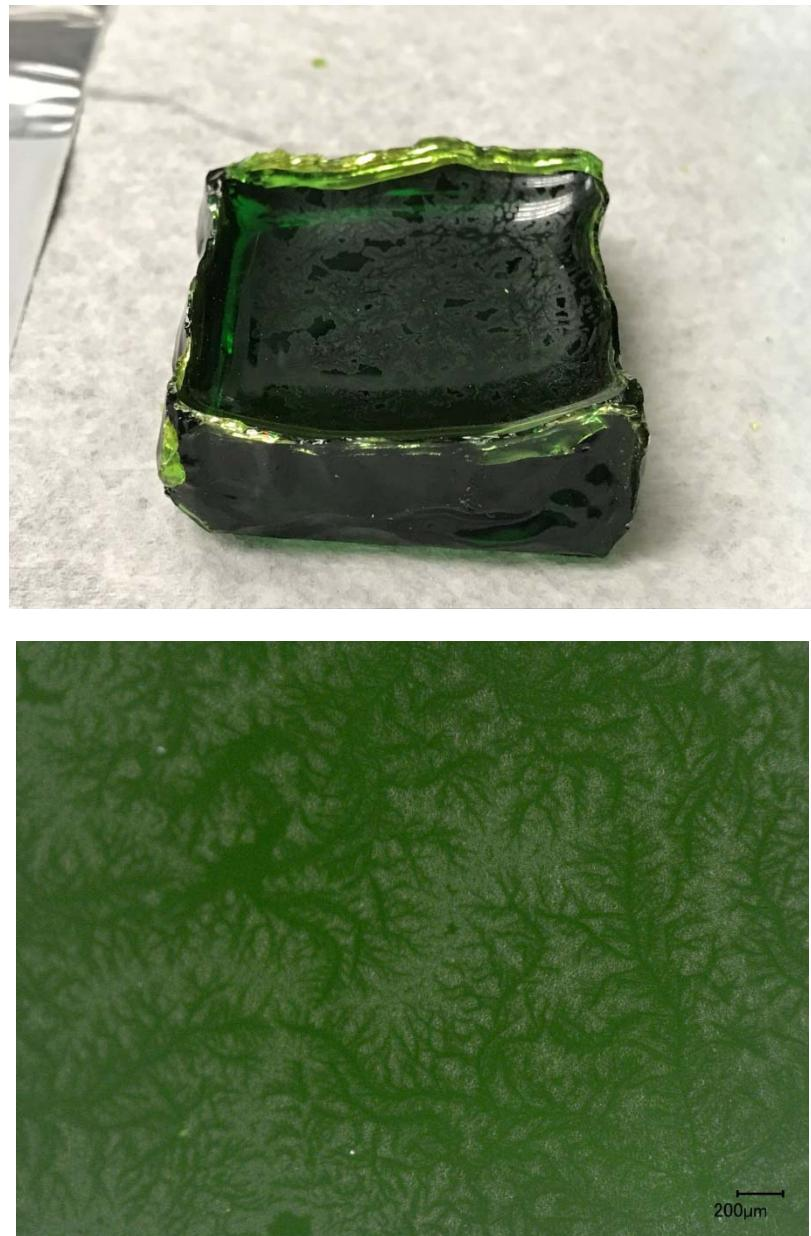
Figure G.7. Glass LP2-IL-07 after CCC Beginning at 1150 °C both Glass (top) and Magnified 100X (bottom)
