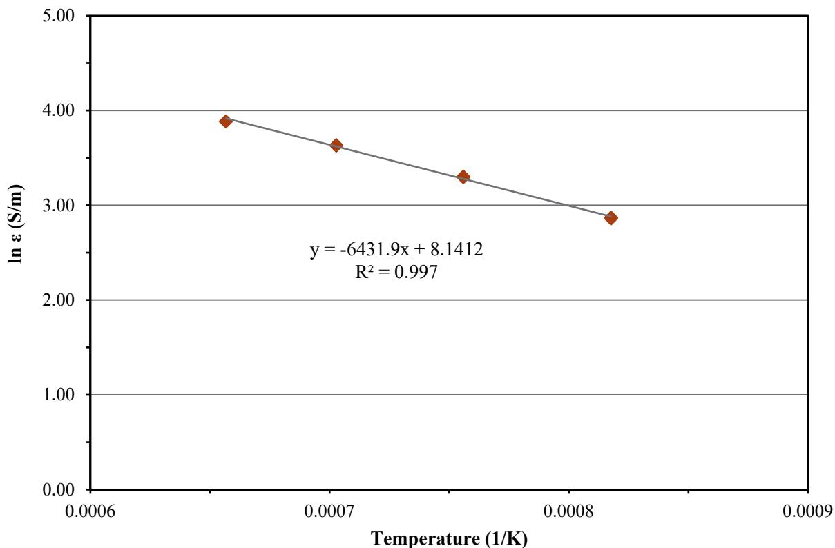
Figure D.23. Electrical Conductivity-Temperature Data and Arrhenius Equation Fit for Glass LP2-OL-07-1
