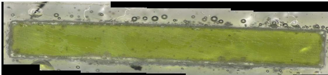
c) Glass cross section magnified after VHT
