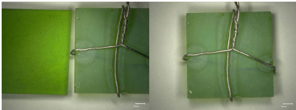
a) Glass square after (right) and before (left) VHT; b) Glass square after VHT
