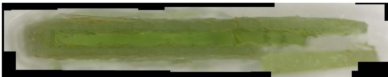
c) Glass cross section magnified after VHT
