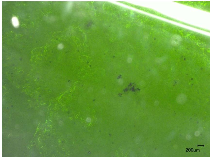
Figure A.9. Photo of Glass LP2-IL-09 Morphology of Third Melt at 1175 °C for 1 h
