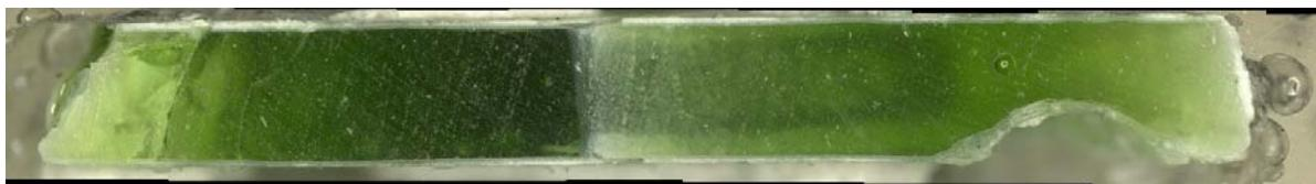
c) Glass cross section magnified after VHT
