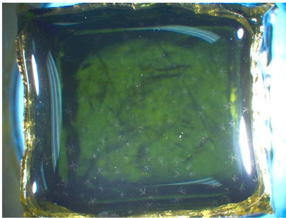
Figure G.28. Glass LP2-OL-12 after CCC Beginning at 1150 °C
