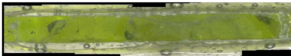
b) Glass cross section magnified after VHT
