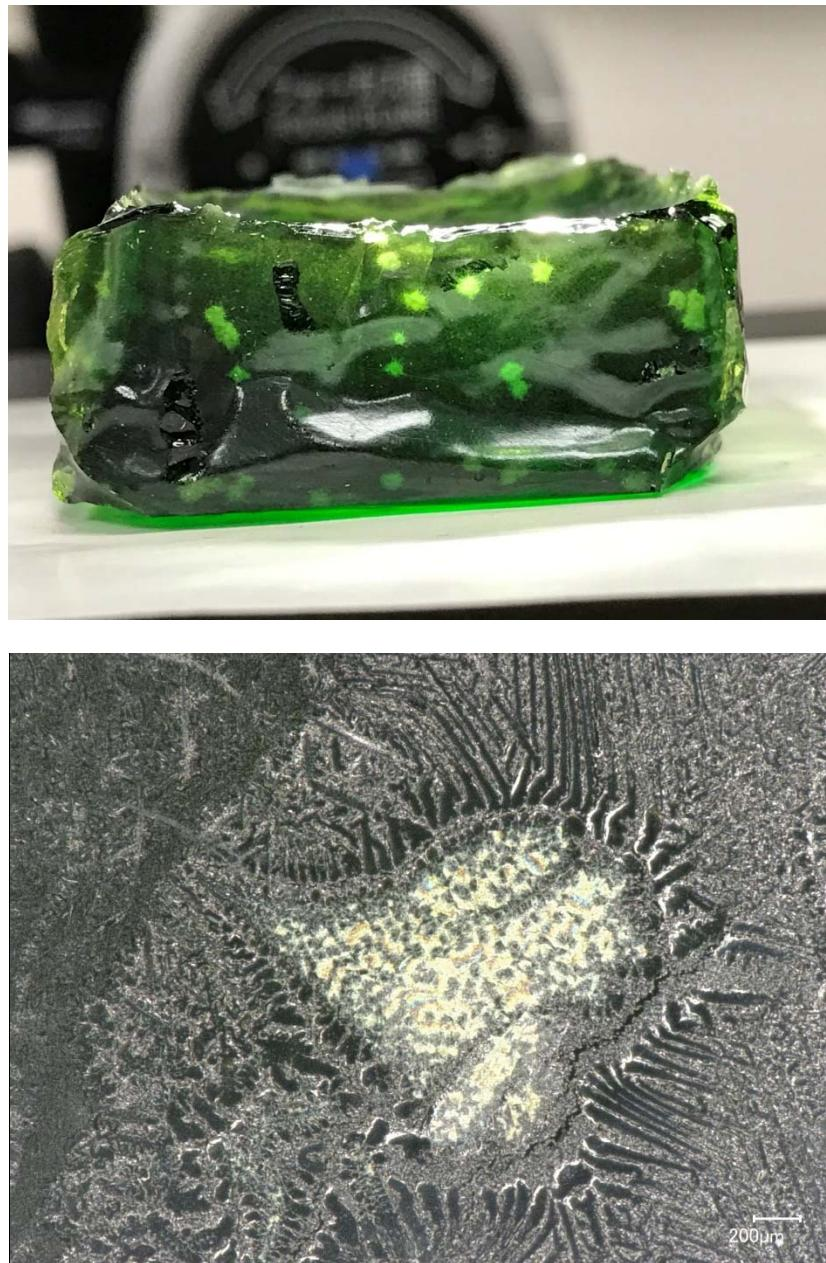
Figure G.8. Glass LP2-IL-08 after CCC Beginning at 1150 °C both Glass (top) and Magnified 100X (bottom)
