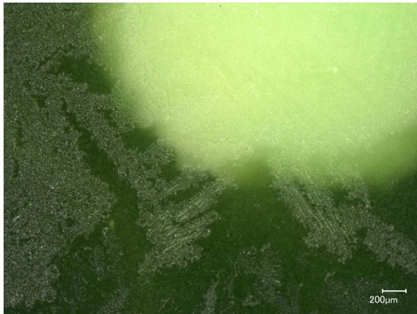
Figure G.6. Glass LP2-IL-06 after CCC Beginning at 1150 °C both Glass (top) and Magnified 100X (bottom)
