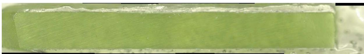
c) Glass cross section magnified after VHT
