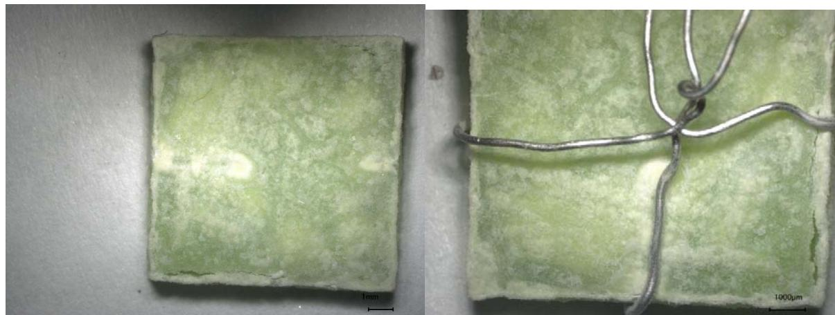
a) Glass square magnified 20X after VHT; b) Glass square magnified 30X after VHT
