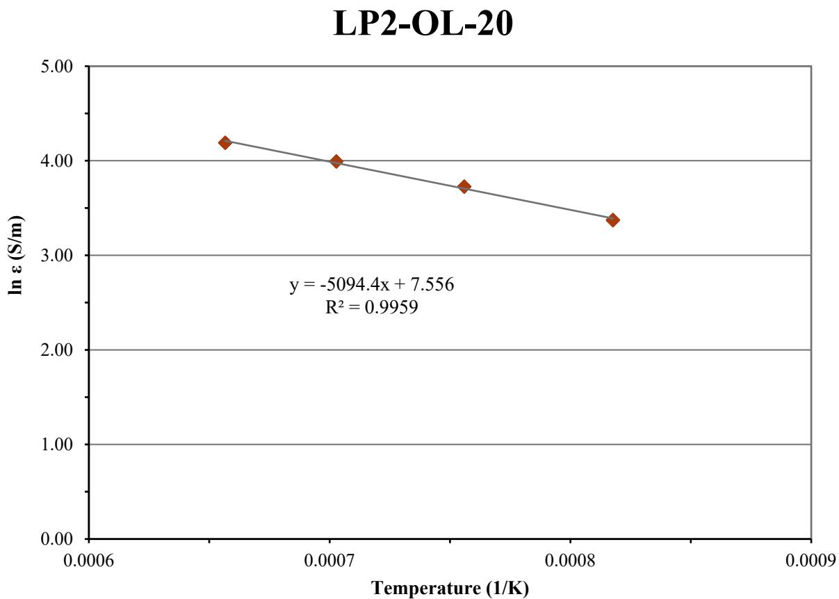
Figure D.36. Electrical Conductivity-Temperature Data and Arrhenius Equation Fit for Glass LP2-OL-20
