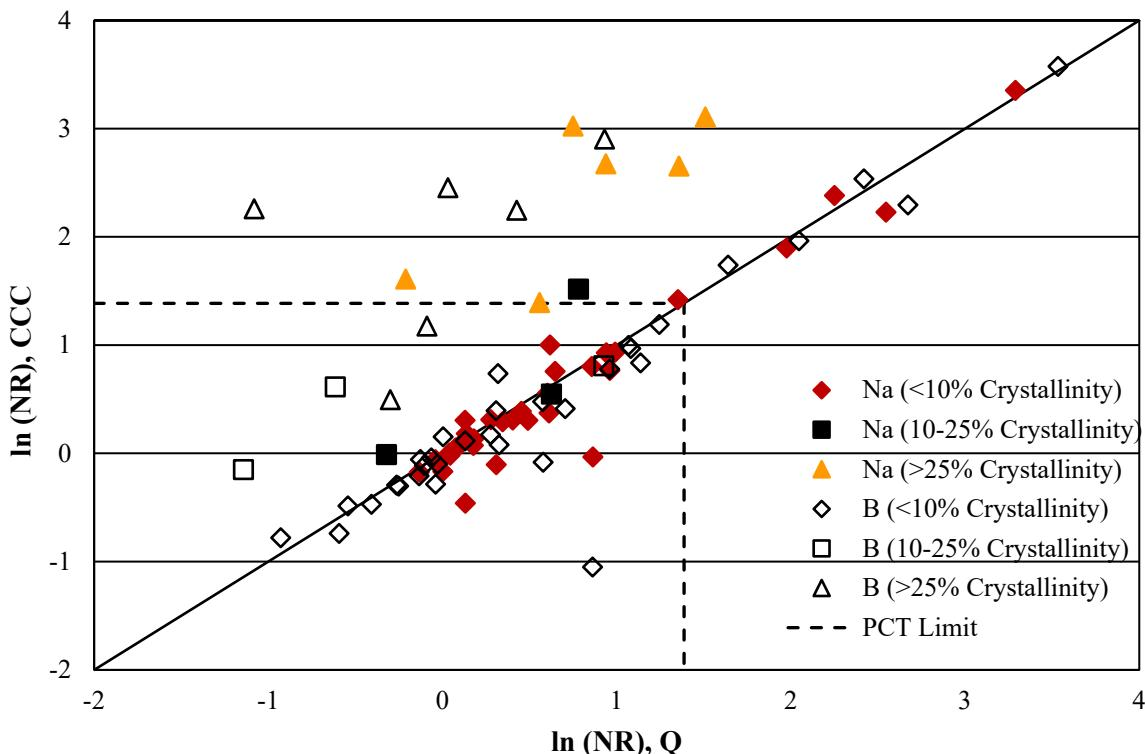
Figure 3.9. Comparison of Natural Logarithm of PCT Normalized Release (g/L) of B and Na for Quenched and CCC-Treated Samples of Phase 2 Enhanced LAW Glasses that Contain Aluminosilicates
