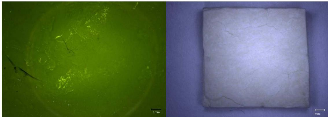
a) Glass square magnified 20X before VHT; b) Glass surface magnified after VHT
