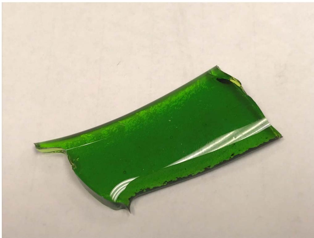
Figure A.20. Photo of Glass LP2-OL-03MOD2 Morphology of Second Melt at 1150 °C for 1.5 h
