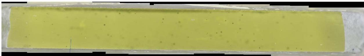
b) Glass cross section magnified after VHT
