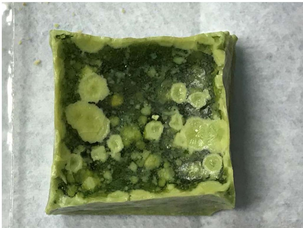
Figure G.26. Glass LP2-OL-10MOD after CCC Beginning at 1150 °C
