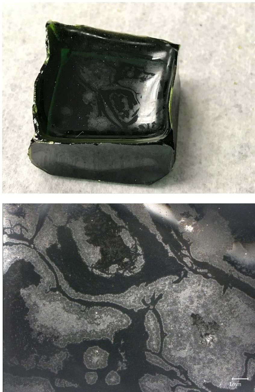
Figure G.14. Glass LP2-IL-14 after CCC Beginning at 1150 °C both Glass (top) and Magnified 20X (bottom)
