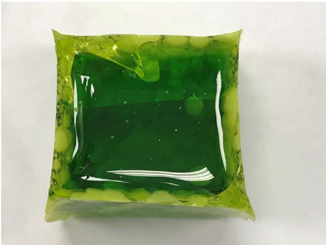
Figure G.36. Glass LP2-OL-20 after CCC Beginning at 1150 °C
