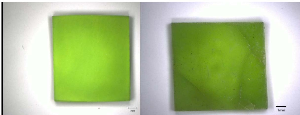
a) Glass square magnified 20X before VHT; b) Glass surface magnified after VHT
