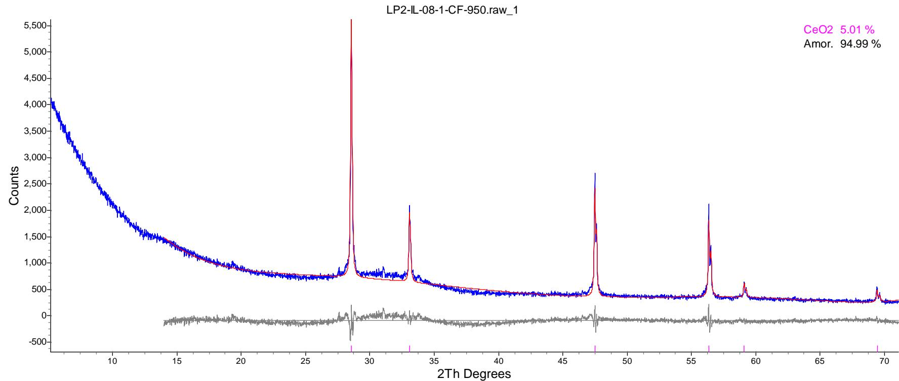
Figure F.7. XRD Spectrum of Heat-Treated Glass LP2-IL-08
