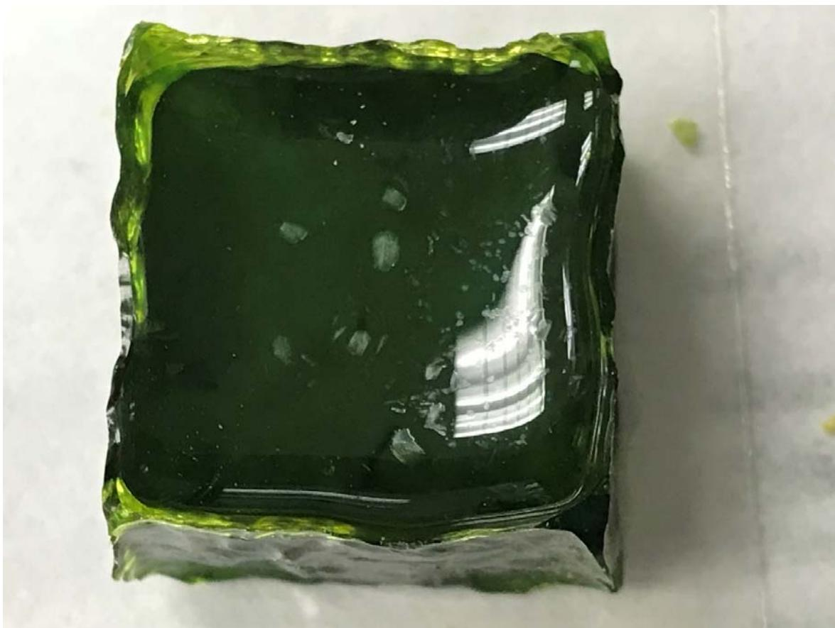
Figure G.32. Glass LP2-OL-16MOD after CCC Beginning at 1150 °C
