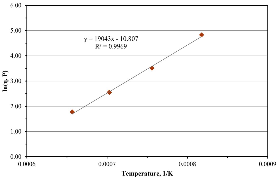
Figure C.24. Viscosity-Temperature Data and Arrhenius Equation Fit for Glass LP2-OL-08 MOD
