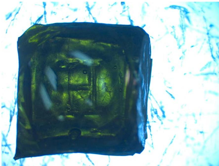
Figure E.24. Glass LP2-OL-09-1 after CF Heat Treatment at 950 °C for 24 h
