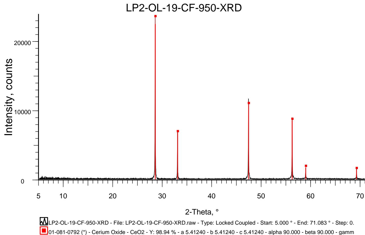
Figure F.21. XRD Spectrum of Heat-Treated Glass LP2-OL-19
