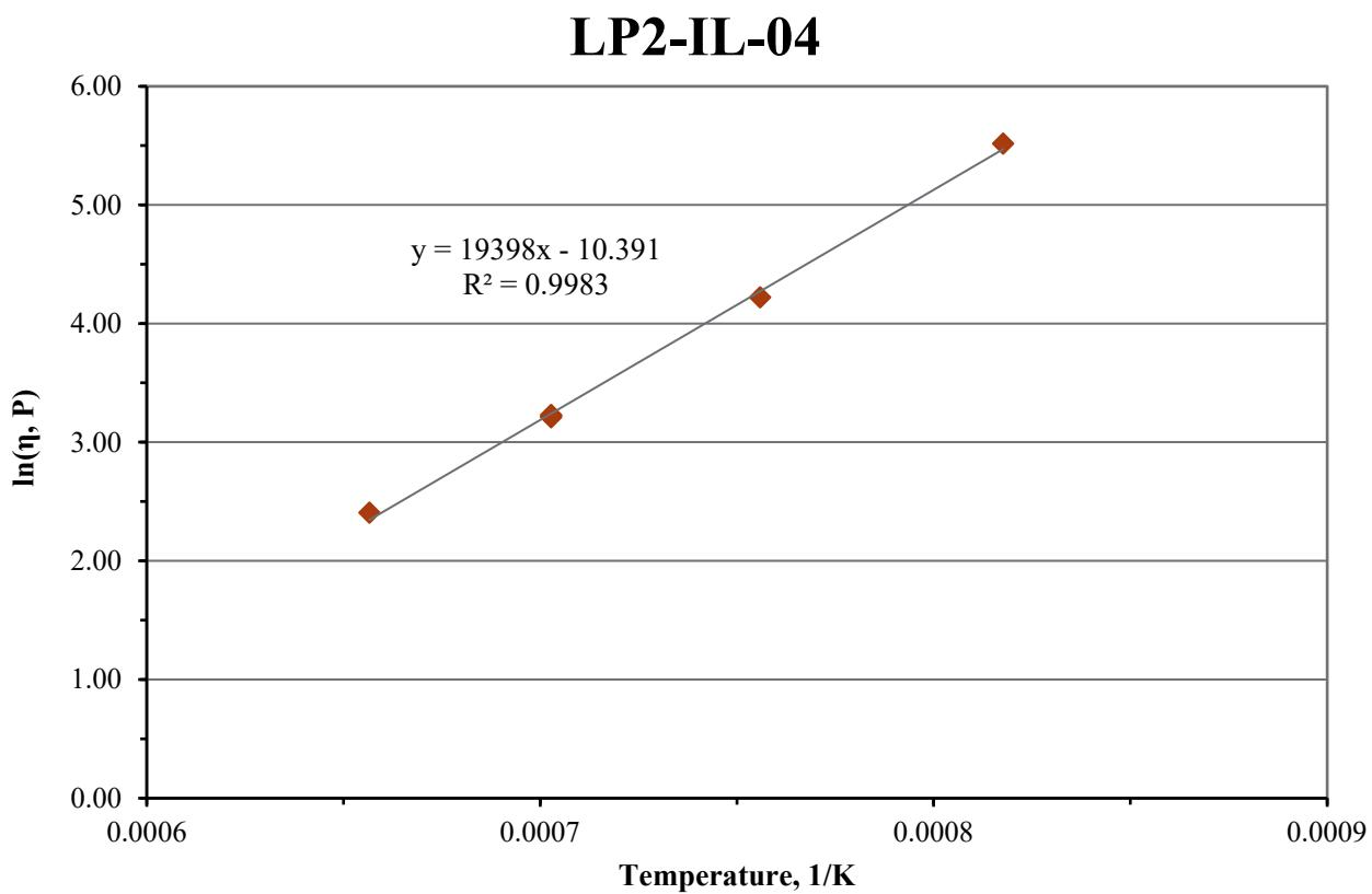
Figure C.4. Viscosity-Temperature Data and Arrhenius Equation Fit for Glass LP2-IL-04
