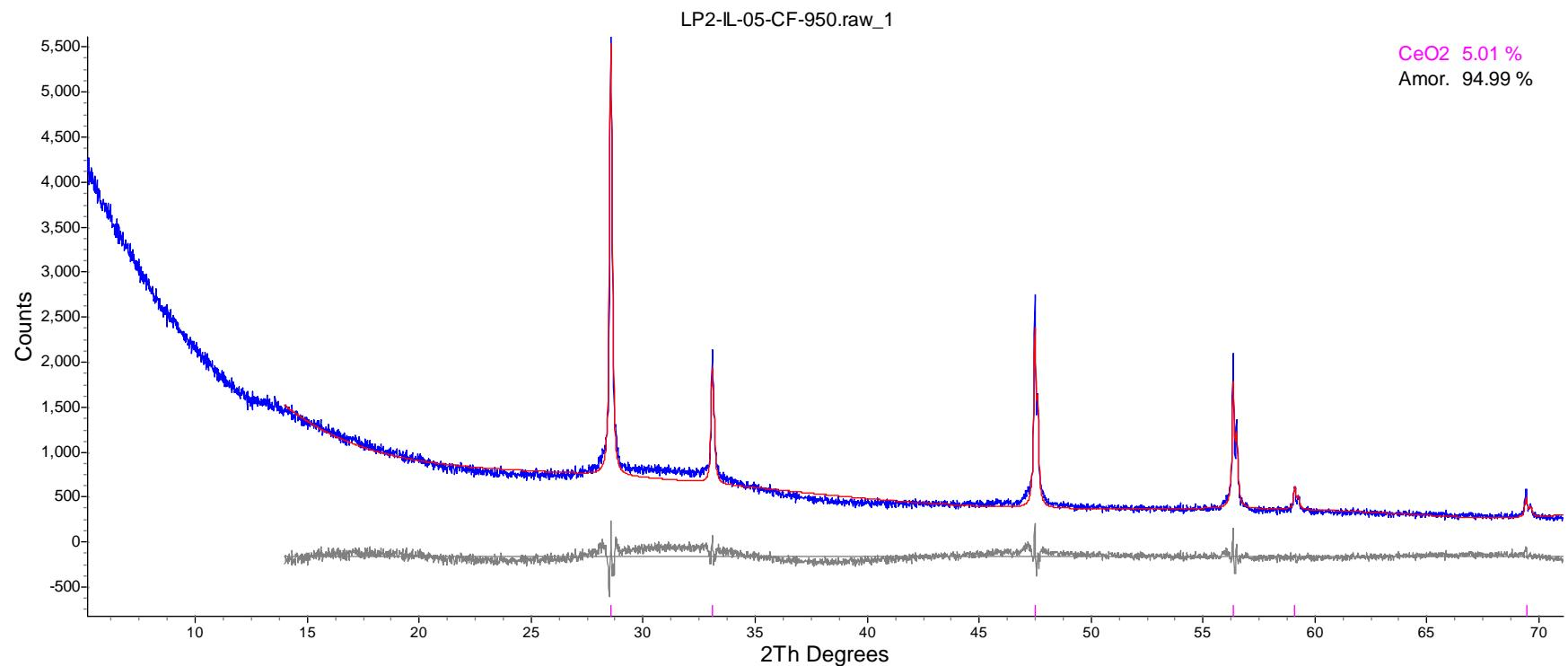
Figure F.5. XRD Spectrum of Heat-Treated Glass LP2-IL-05
