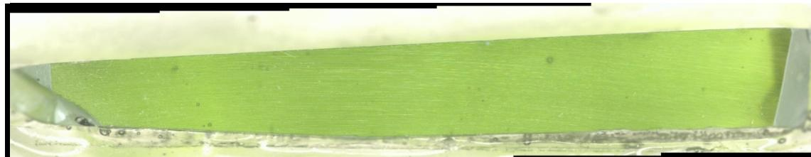
c) Glass cross section magnified after VHT
