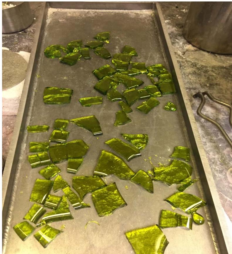
Figure A.27. Photo of Glass LP2-OL-11 Morphology of Second Melt at 1150 °C for 1.6 h
