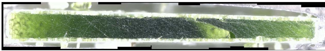
c) Glass cross section magnified after VHT
