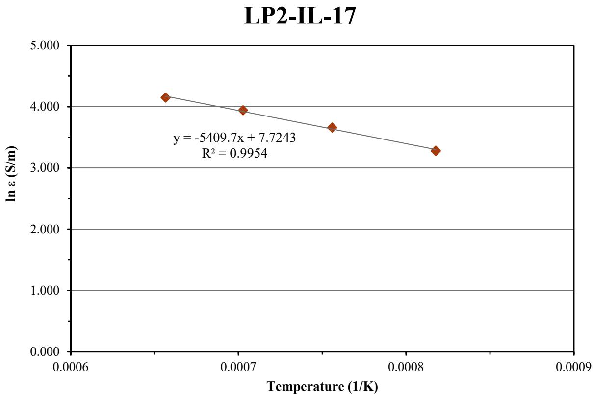
Figure D.17. Electrical Conductivity-Temperature Data and Arrhenius Equation Fit for Glass LP2-IL-17
