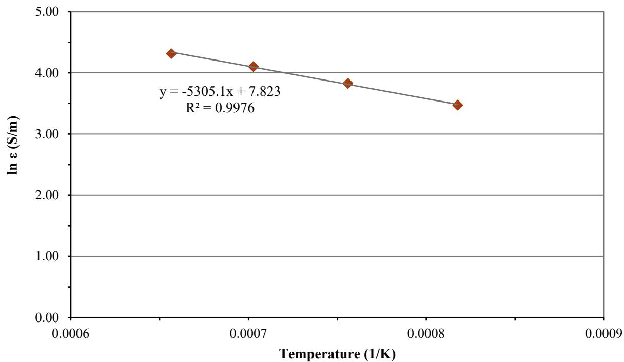
Figure D.28. Electrical Conductivity-Temperature Data and Arrhenius Equation Fit for Glass LP2-OL-12
