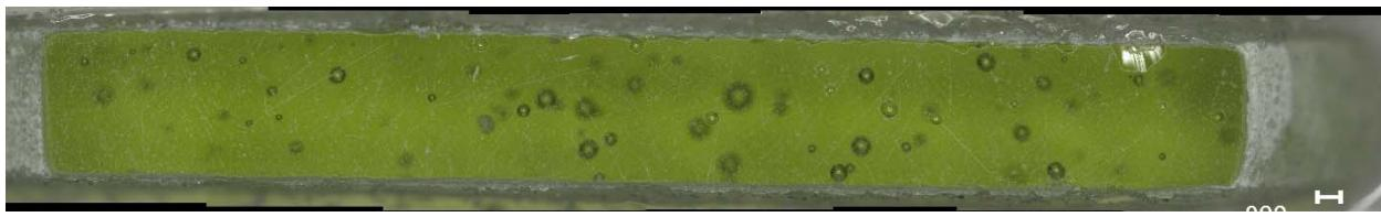
c) Glass cross section magnified after VHT
