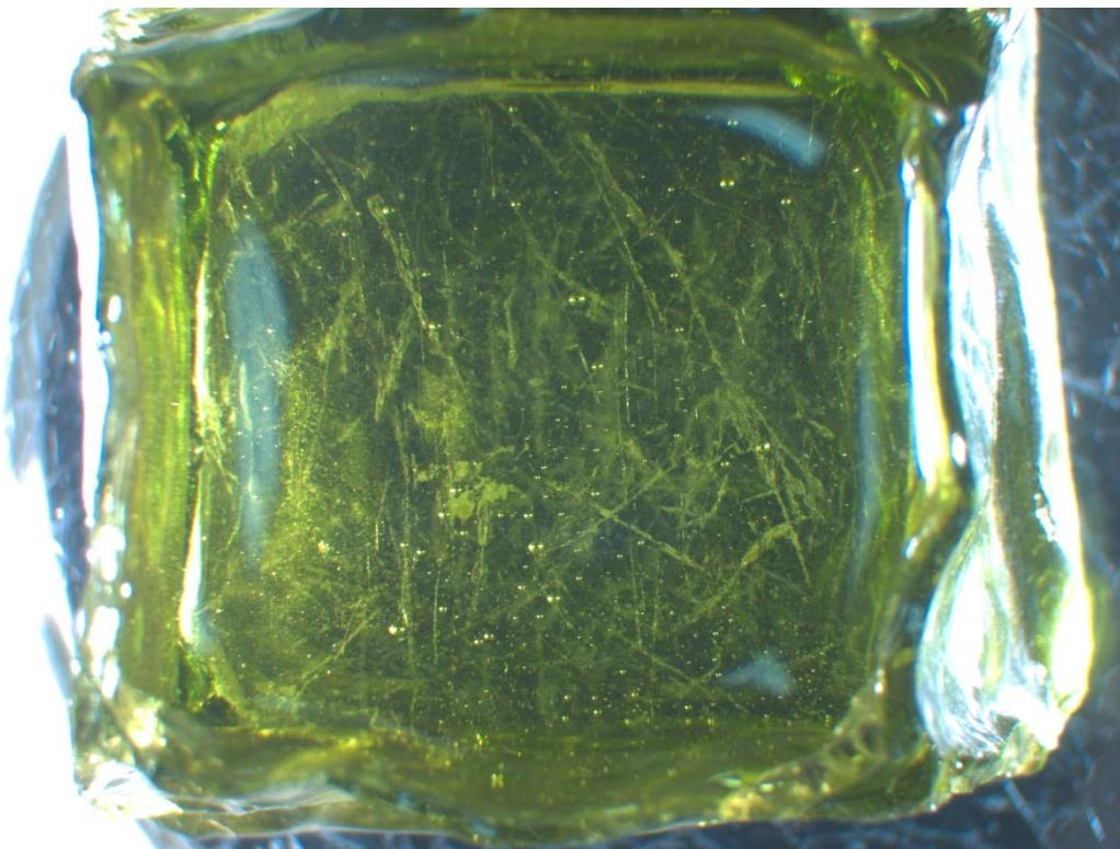
Figure G.27. Glass LP2-OL-11 after CCC Beginning at 1150 °C
