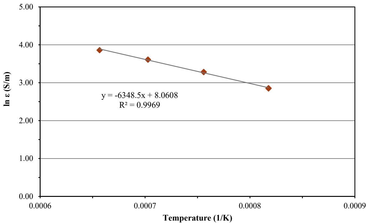
Figure D.26. Electrical Conductivity-Temperature Data and Arrhenius Equation Fit for Glass LP2-OL-10 MOD
