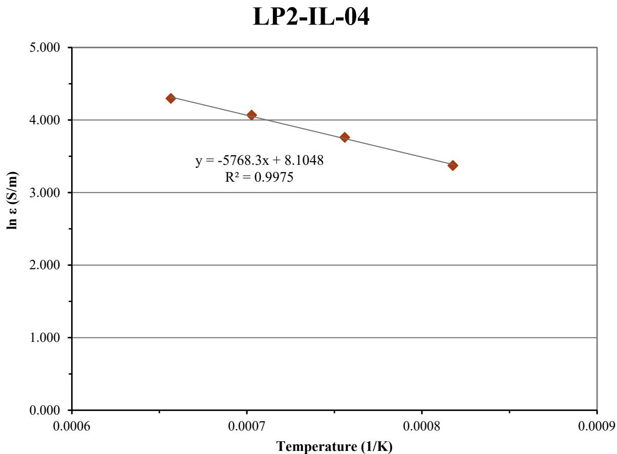
Figure D.4. Electrical Conductivity-Temperature Data and Arrhenius Equation Fit for Glass LP2-IL-04
