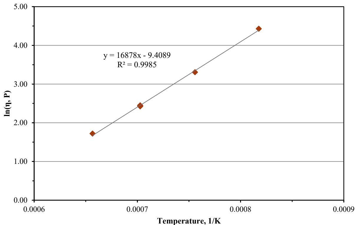
Figure C.27. Viscosity-Temperature Data and Arrhenius Equation Fit for Glass LP2-OL-11
