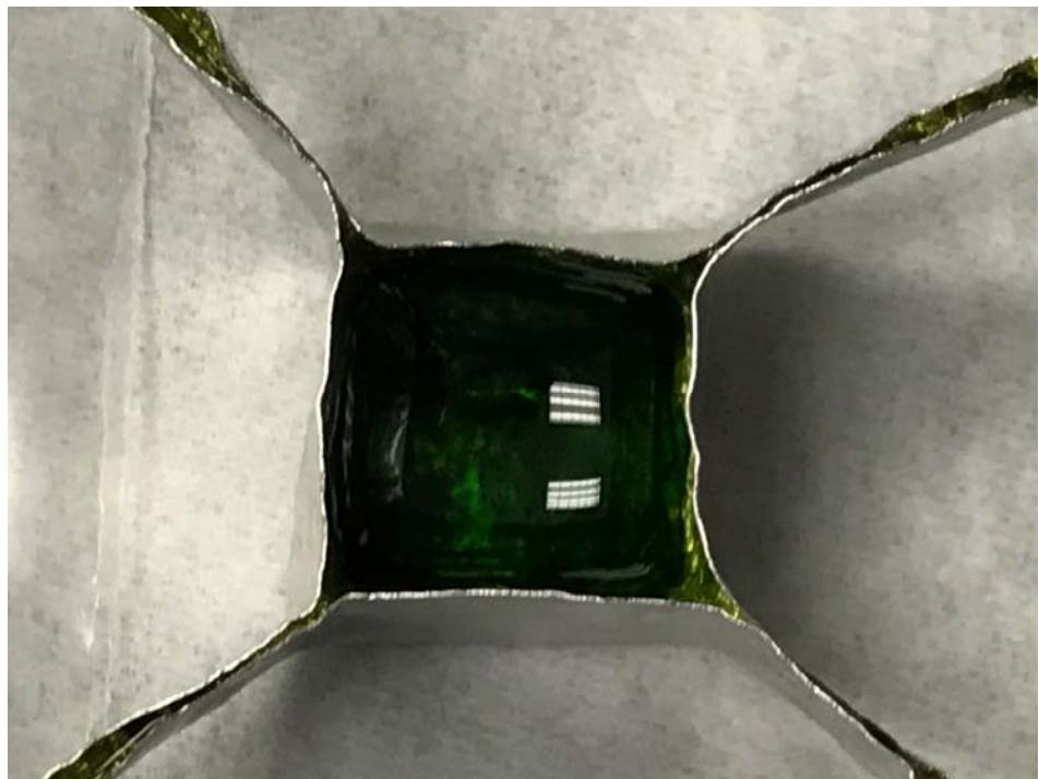
Figure E.14. Glass LP2-IL-15 after CF Heat Treatment at 950 °C for 24 h
