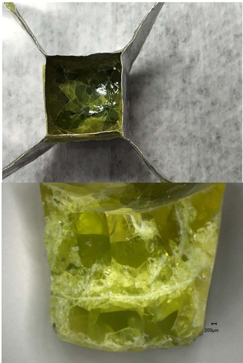
Figure E.20. Glass LP2-OL-04-1 after CF Heat Treatment at 950 °C for 24 h both in Crucible (top) and Magnified 30X (bottom)
