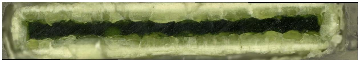
c) Glass surface magnified after VHT
