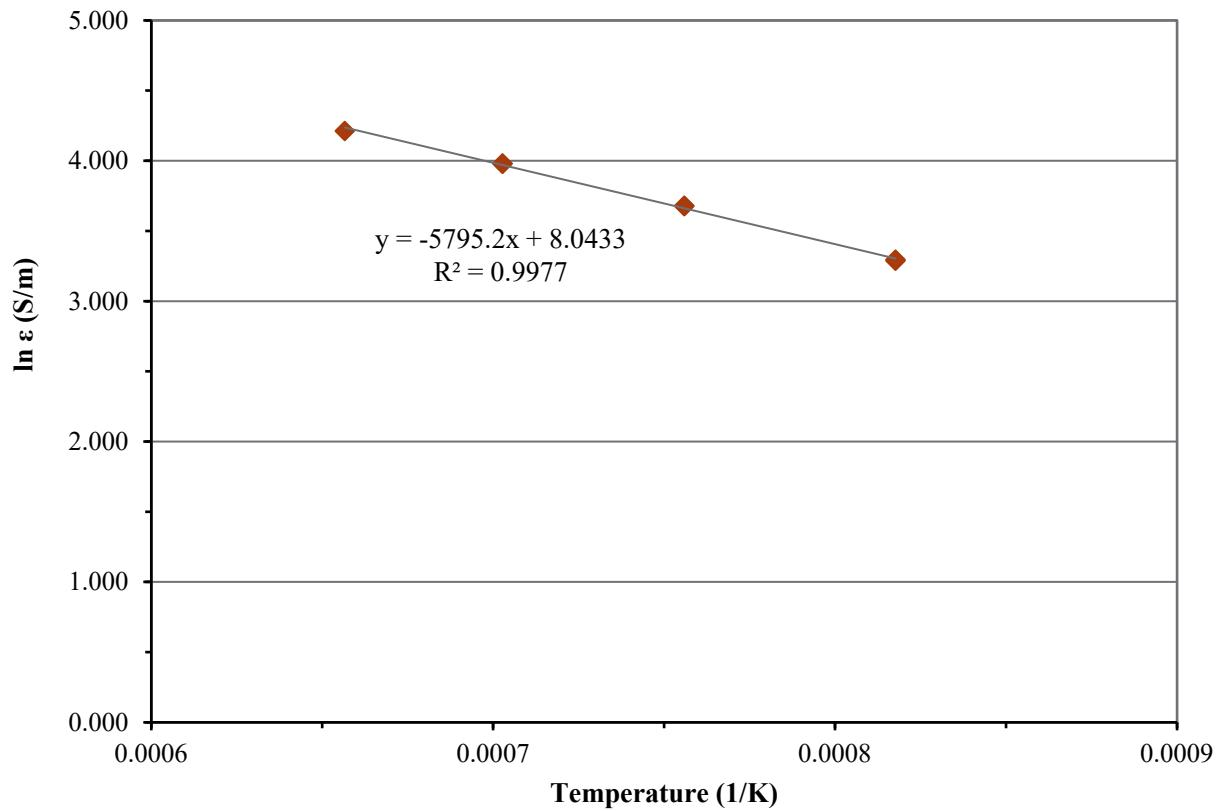
Figure D.7. Electrical Conductivity-Temperature Data and Arrhenius Equation Fit for Glass LP2-IL-07
