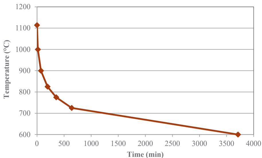
Figure 2.16. Plot of Temperature Schedule During CCC Heat-Treatment of Hanford LAW Glasses
