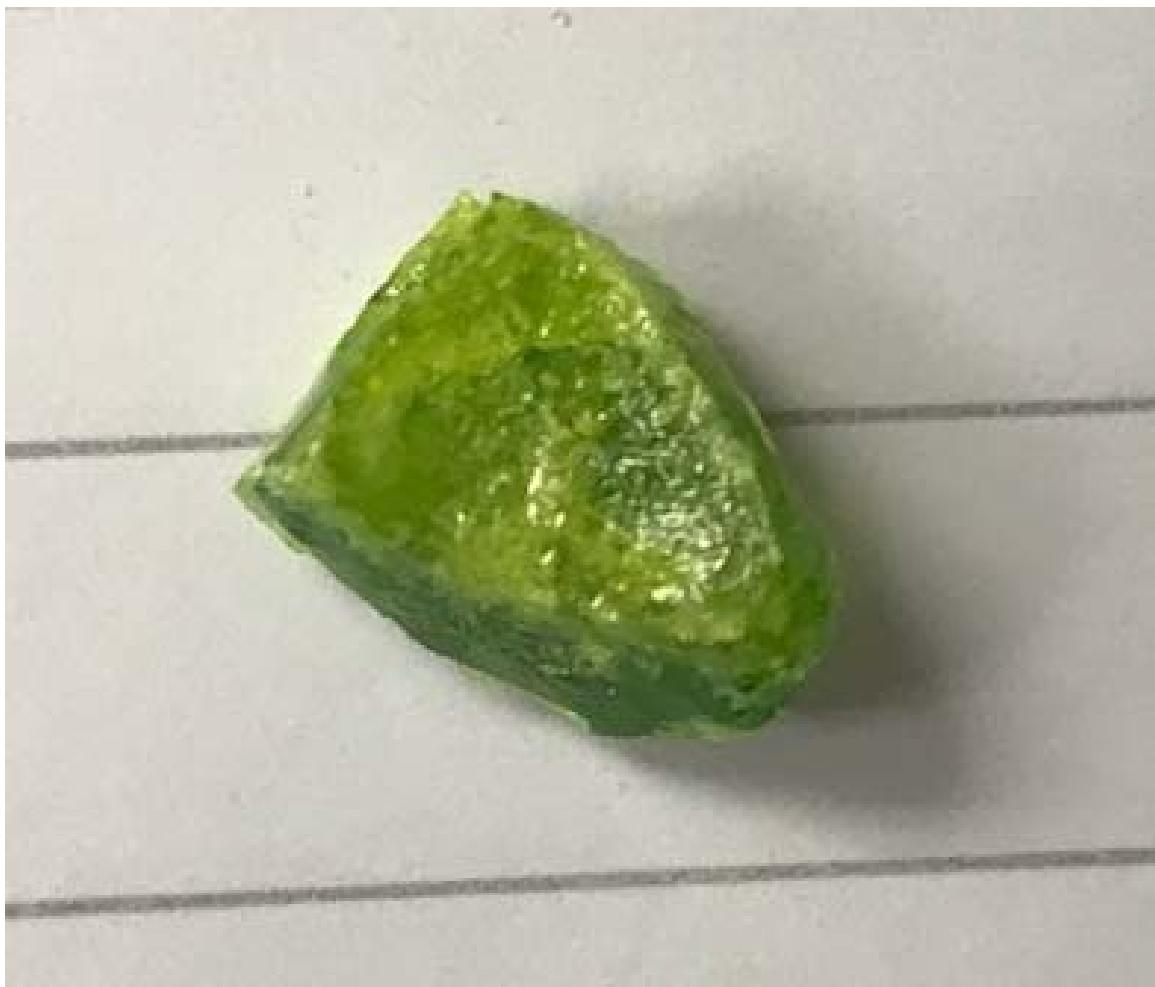
Figure E.19. Glass LP2-OL-03 MOD2 after CF Heat Treatment at 950 °C for 24 h
