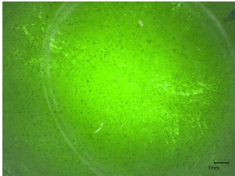
Figure A.7. Photo of Glass LP2-IL-07 Morphology of Second Melt at 1150 °C for 1 h
