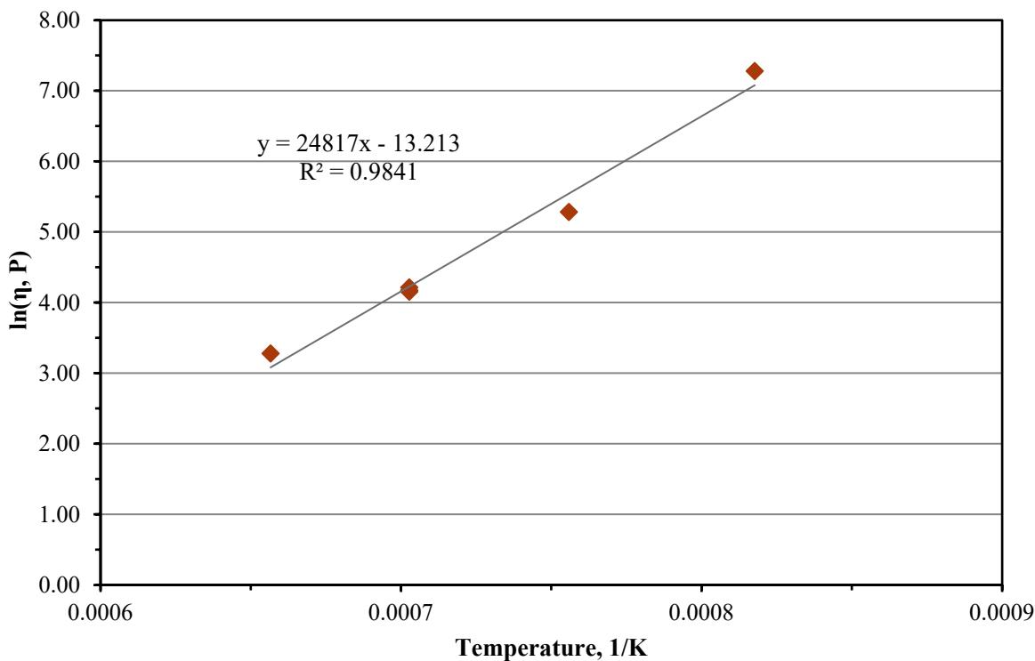
Figure C.26. Viscosity-Temperature Data and Arrhenius Equation Fit for Glass LP2-OL-10 MOD
