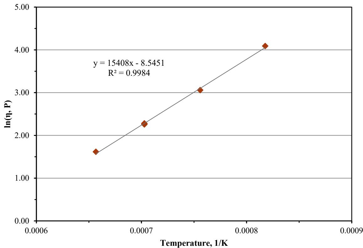
Figure C.30. Viscosity-Temperature Data and Arrhenius Equation Fit for Glass LP2-OL-14
