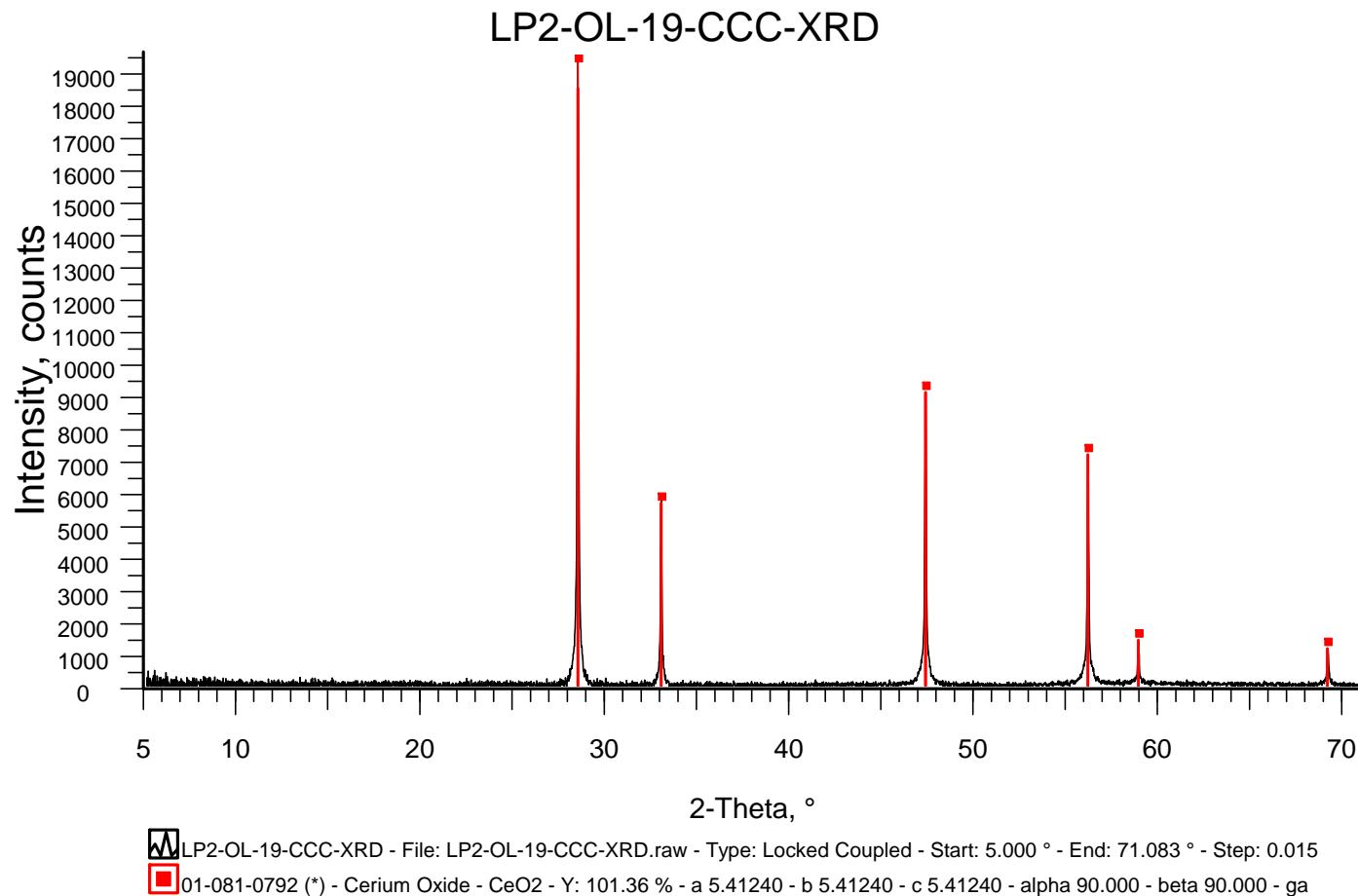
Figure H.19. XRD Spectrum of CCC-Treated Glass LP2-OL-19
