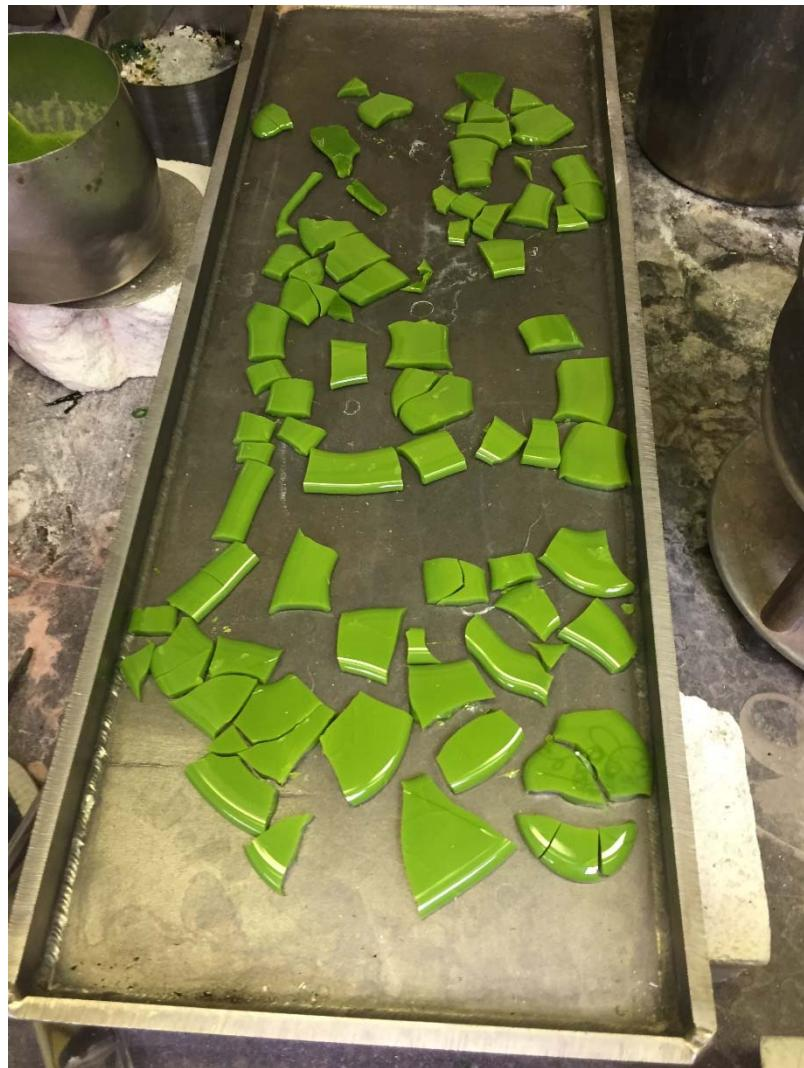
Figure A.34. Photo of Glass LP2-OL-18 Morphology of Second Melt at 1250 °C for 1.6 h
