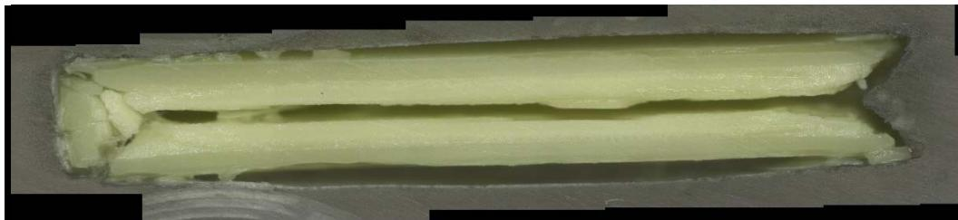
c) Glass cross section magnified after VHT
