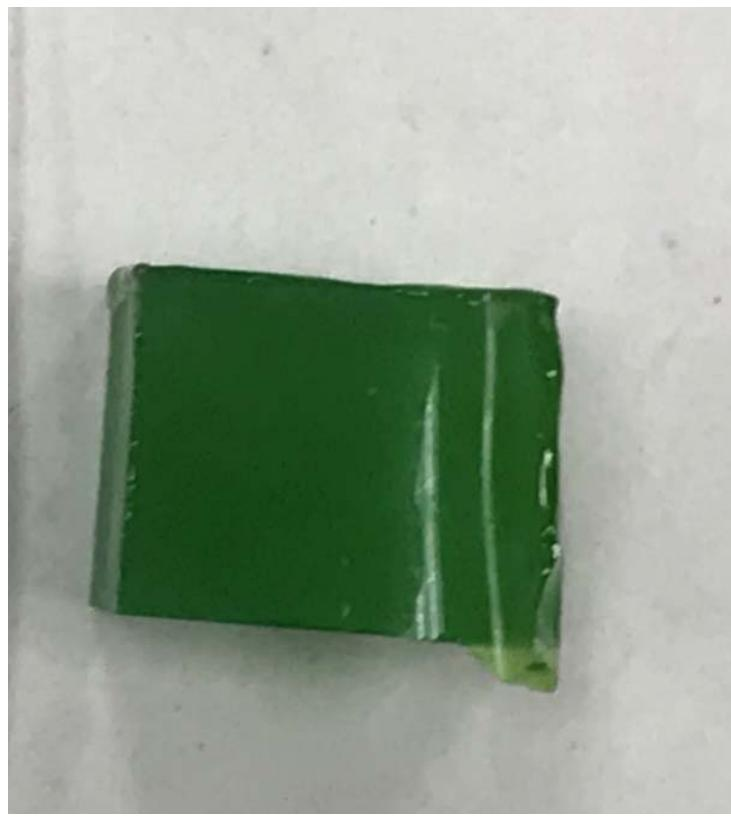
Figure G.17. Glass LP2-IL-17 after CCC Beginning at 1150 °C
