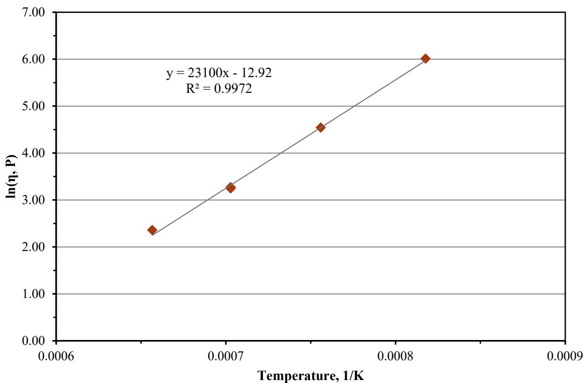
Figure C.34. Viscosity-Temperature Data and Arrhenius Equation Fit for Glass LP2-OL-18
