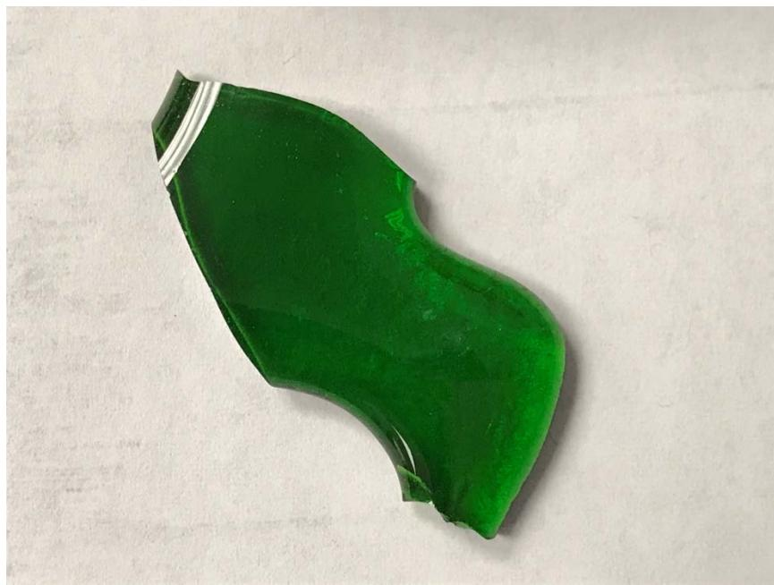
Figure A.14. Photo of Glass LP2-IL-14 Morphology of Second Melt at 1150 °C for 1.5 h
