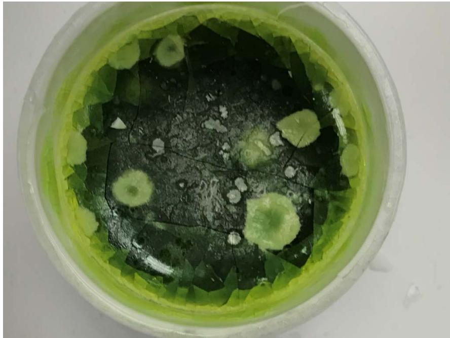
Figure 3.5. Glass LP2-OL-05 Cooled in a Quartz Crucible with Crystals along Edge
