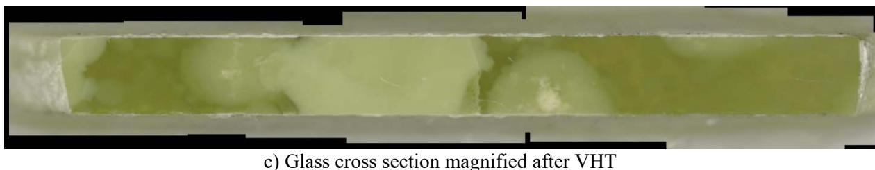
c) Glass cross section magnified after VHT
