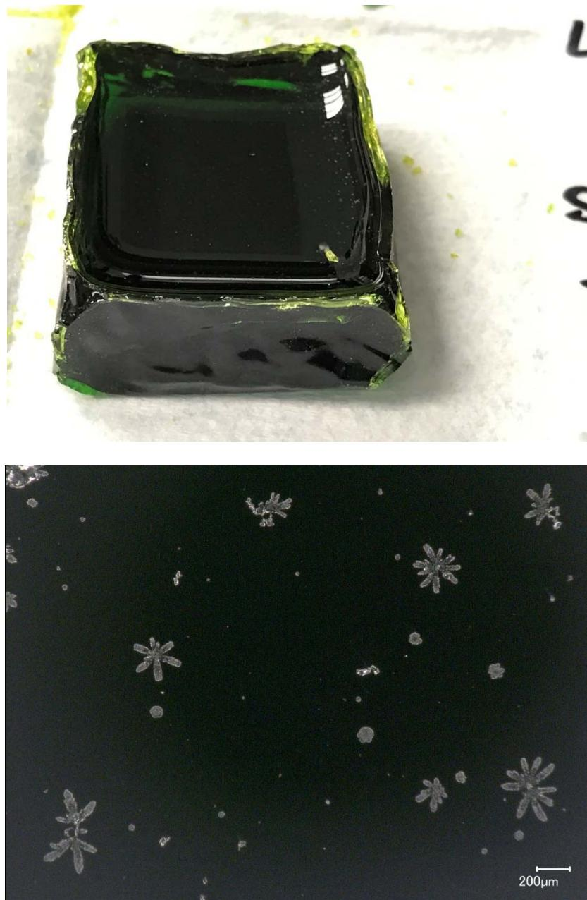
Figure G.4. Glass LP2-IL-04 after CCC Beginning at 1150 °C both Glass (top) and Magnified 100X (bottom)
