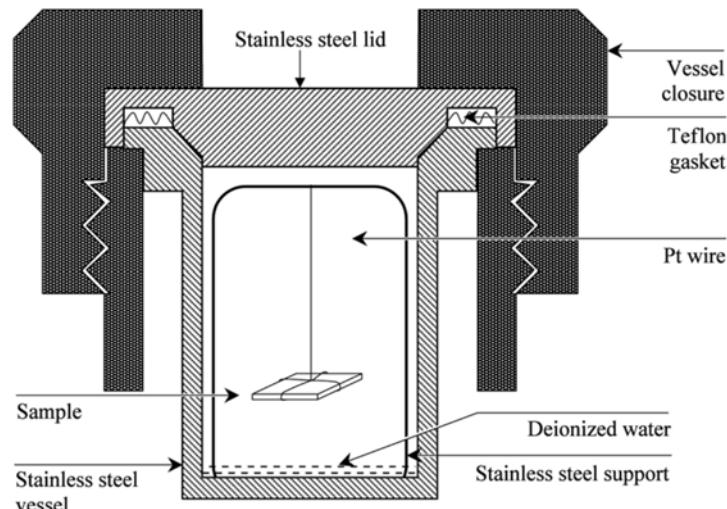
Figure 2.17. Apparatus for Conducting VHTs
