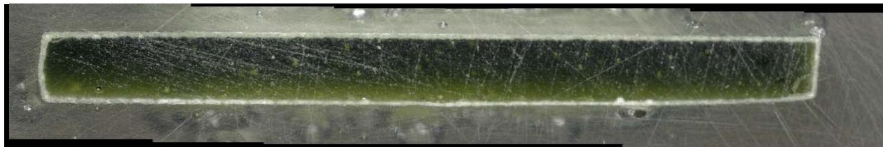
b) Glass cross section magnified after VHT
