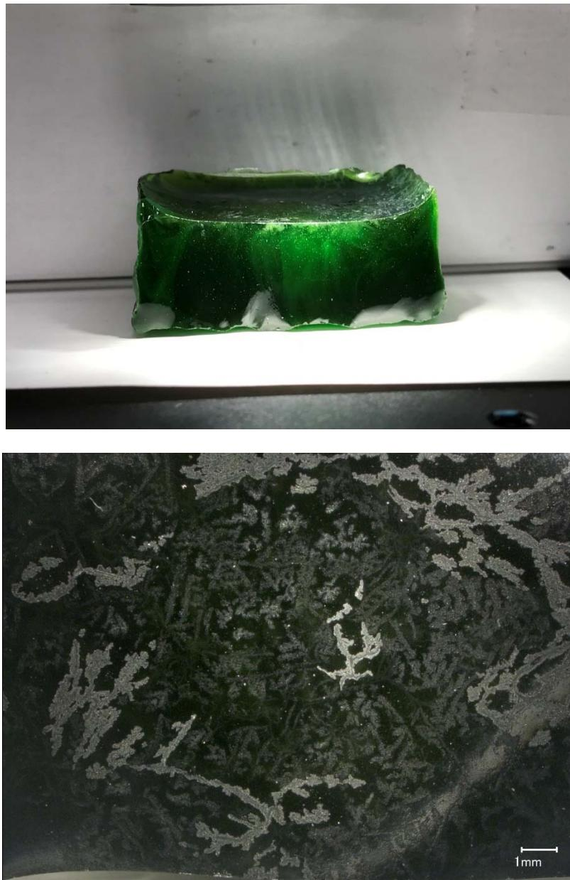
Figure G.15. Glass LP2-IL-15 after CCC Beginning at 1150 °C both Glass (top) and Magnified 20X (bottom)
