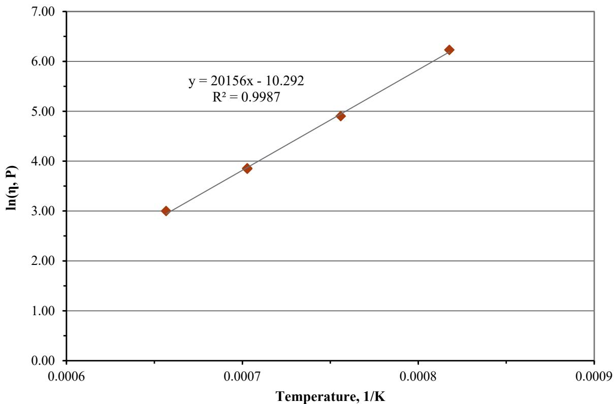
Figure C.10. Viscosity-Temperature Data and Arrhenius Equation Fit for Glass LP2-IL-10
