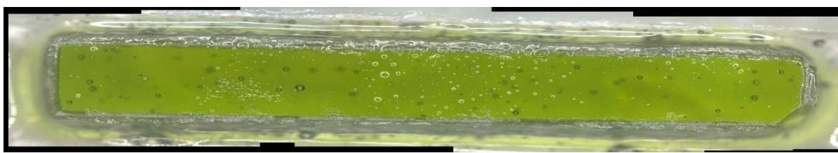
c) Glass cross section magnified after VHT
