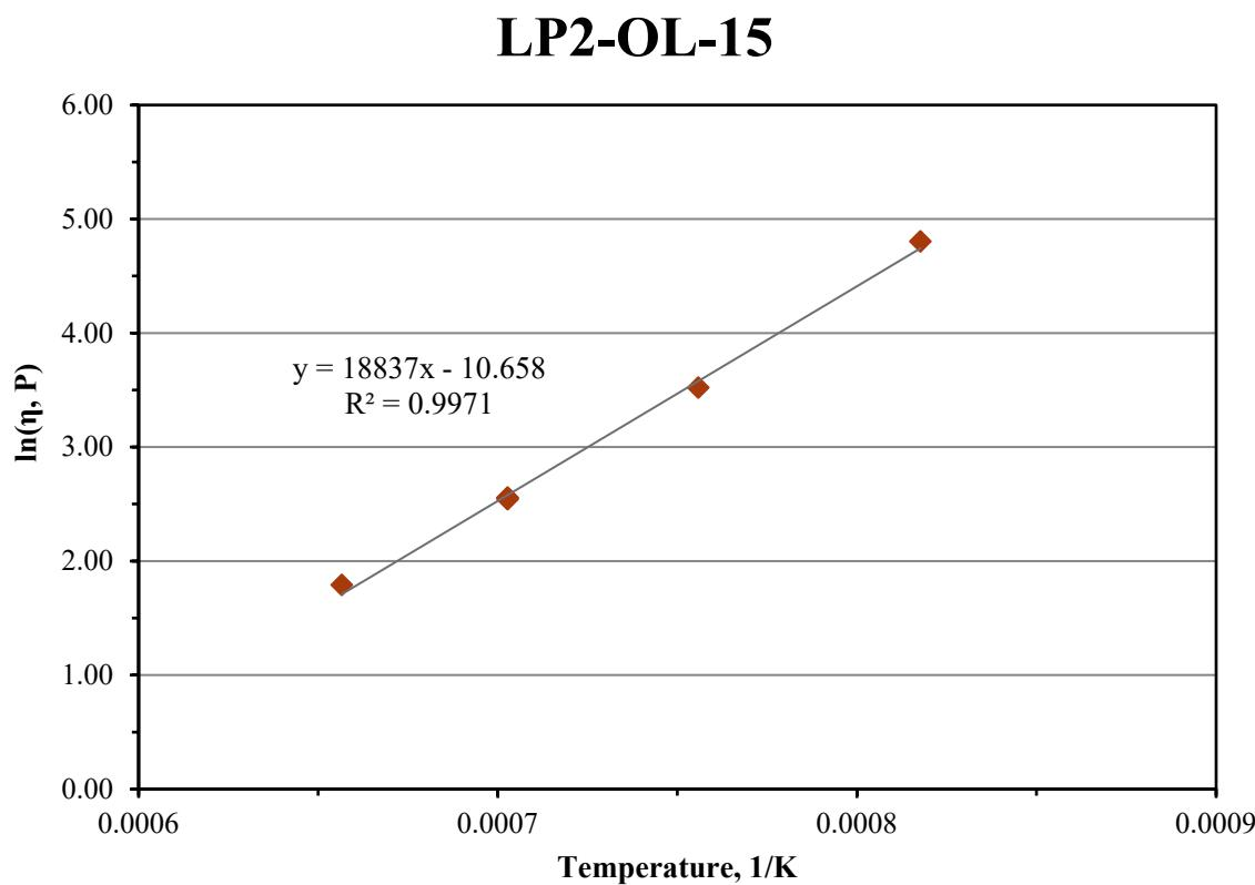
Figure C.31. Viscosity-Temperature Data and Arrhenius Equation Fit for Glass LP2-OL-15
