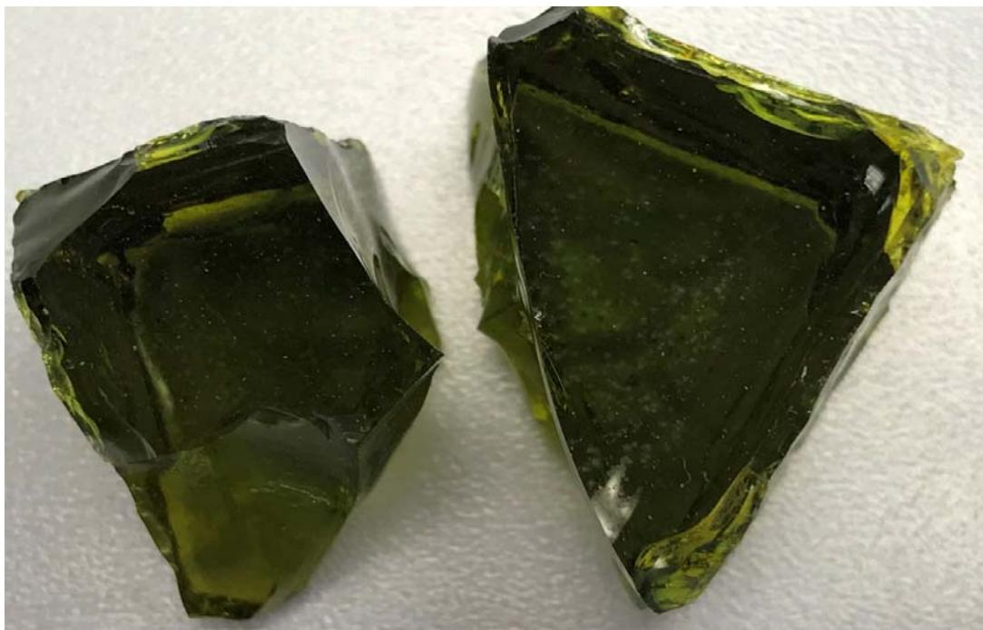
Figure G.33. Glass LP2-OL-17 after CCC Beginning at 1150 °C
