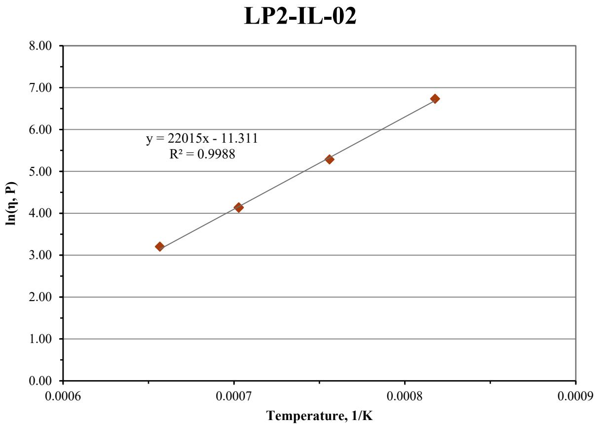
Figure C.2. Viscosity-Temperature Data and Arrhenius Equation Fit for Glass LP2-IL-02
