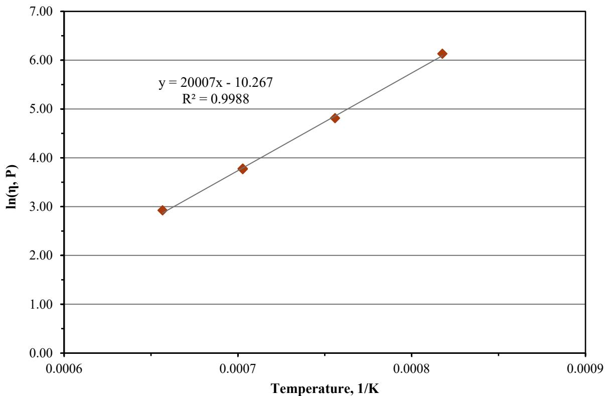
Figure C.16. Viscosity-Temperature Data and Arrhenius Equation Fit for Glass LP2-IL-16
