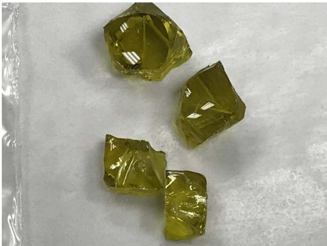
Figure E.27. Glass LP2-OL-12 after CF Heat Treatment at 950 °C for 24 h
