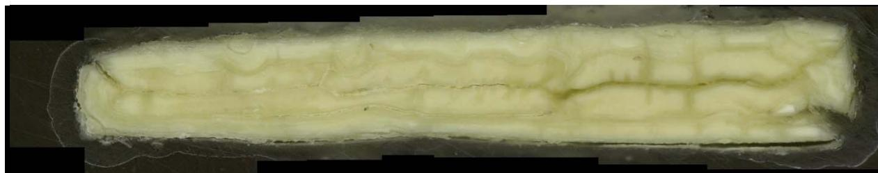
c) Glass cross section magnified after VHT
