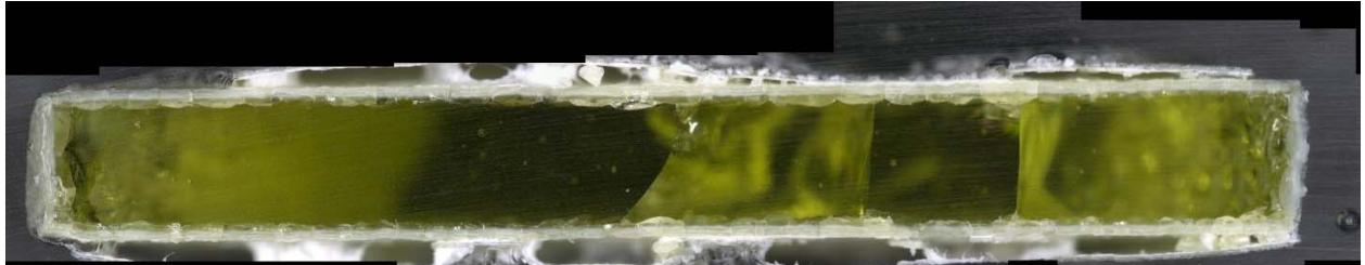
b) Glass cross section magnified after VHT
