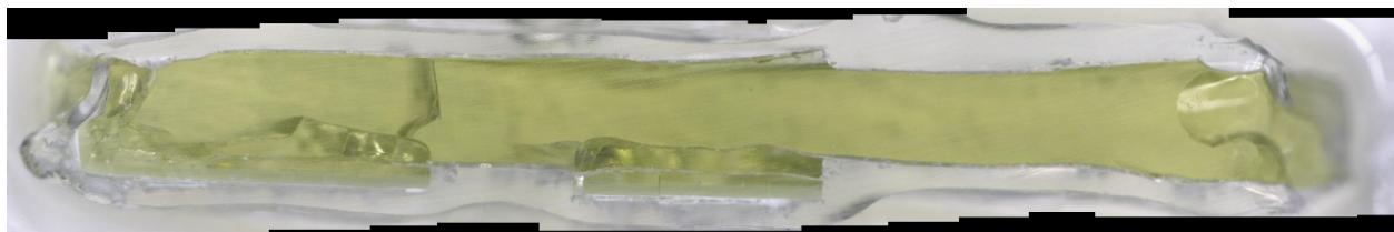
b) Glass cross section magnified after VHT
