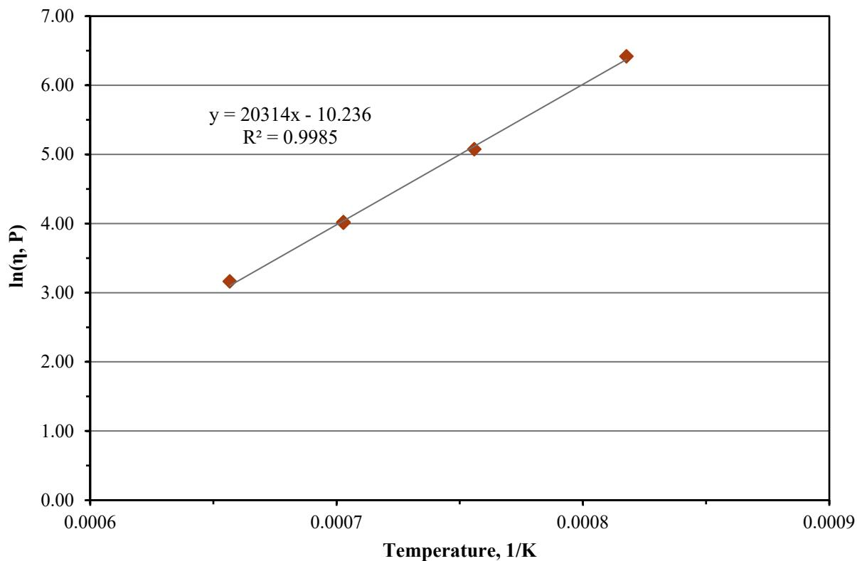
Figure C.15. Viscosity-Temperature Data and Arrhenius Equation Fit for Glass LP2-IL-15
