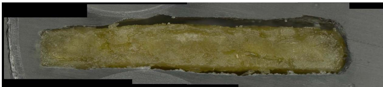
c) Glass cross section magnified after VHT
