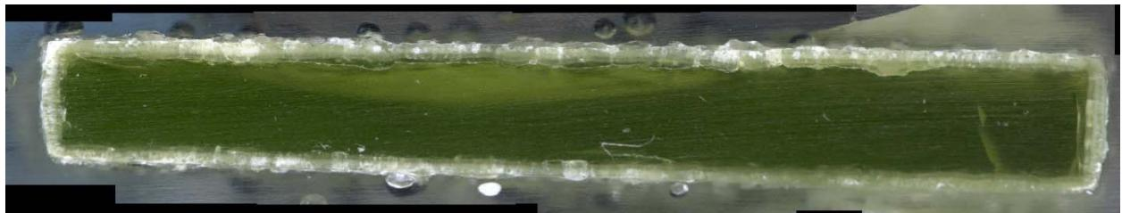
b) Glass cross section magnified after VHT
