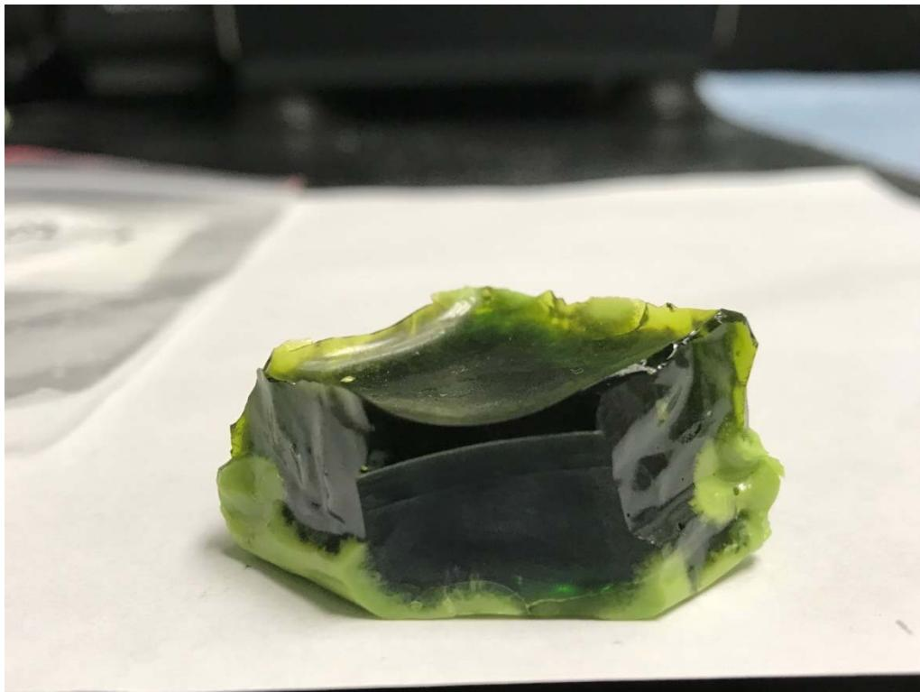
Figure G.23. Glass LP2-OL-07-1 after CCC Beginning at 1150 °C
