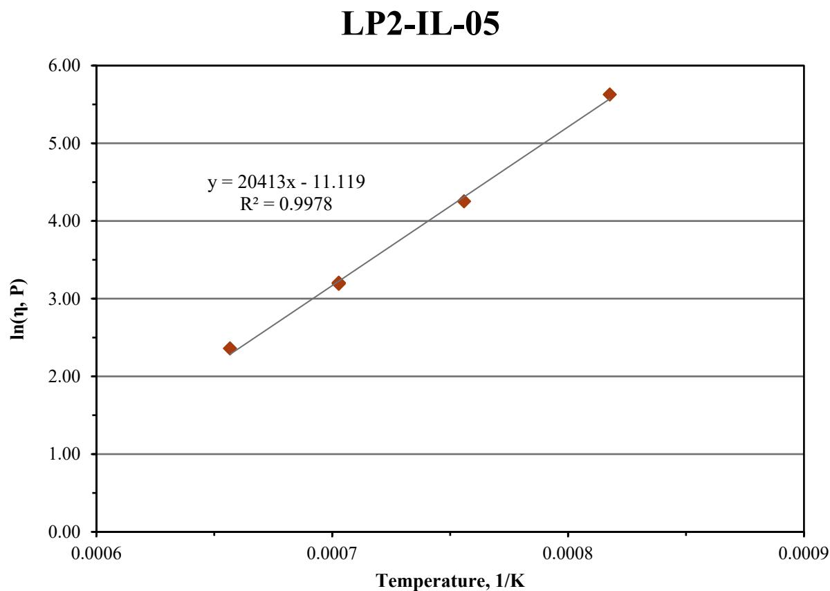
Figure C.5. Viscosity-Temperature Data and Arrhenius Equation Fit for Glass LP2-IL-05
