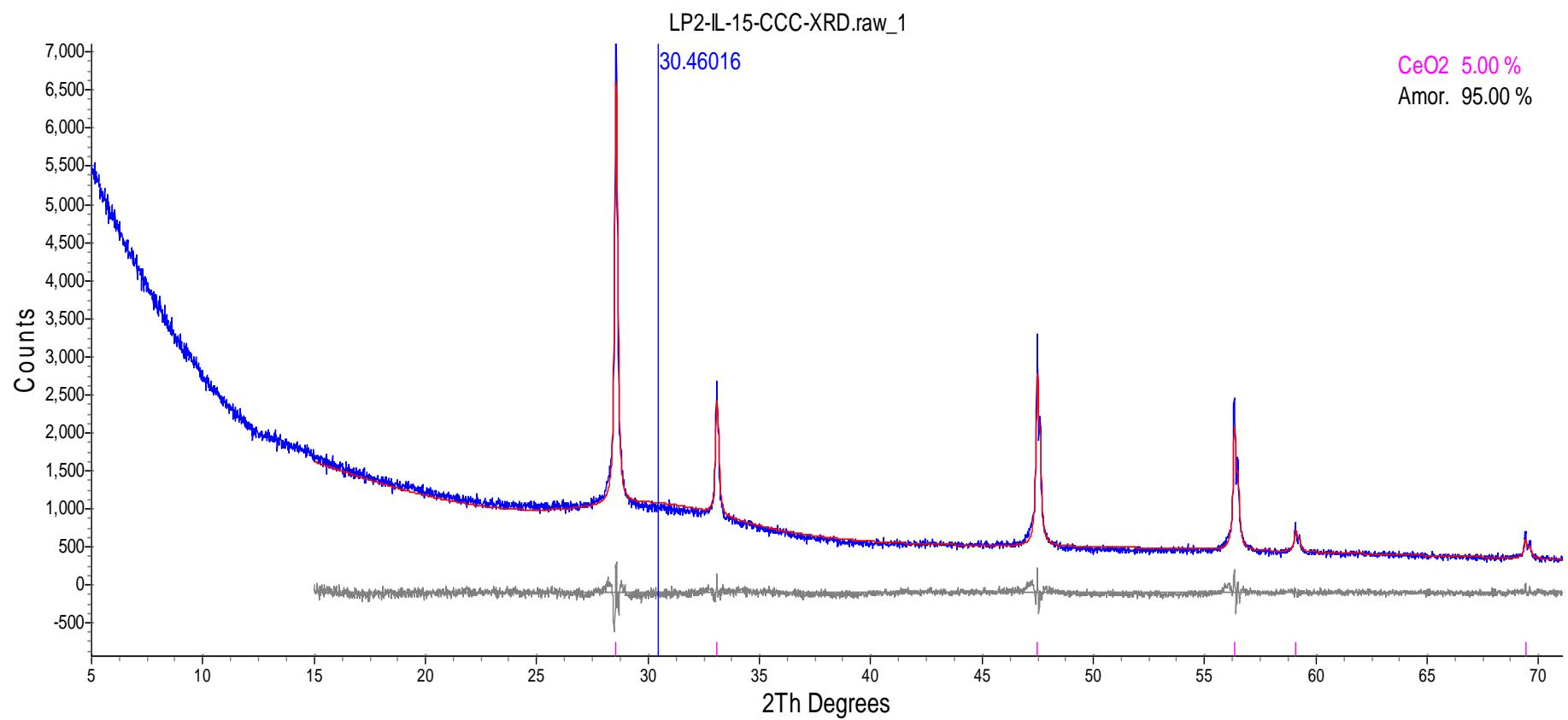
Figure H.5. XRD Spectrum of CCC-Treated Glass LP2-IL-15
