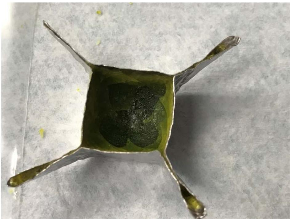
Figure E.25. Glass LP2-OL-10 MOD after CF Heat Treatment at 950 °C for 24 h
