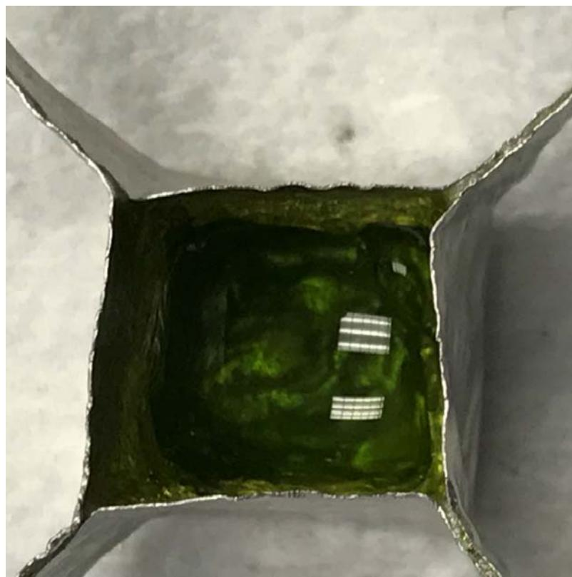
Figure E.3. Glass LP2-IL-04 after CF Heat Treatment at 950 °C for 24 h
