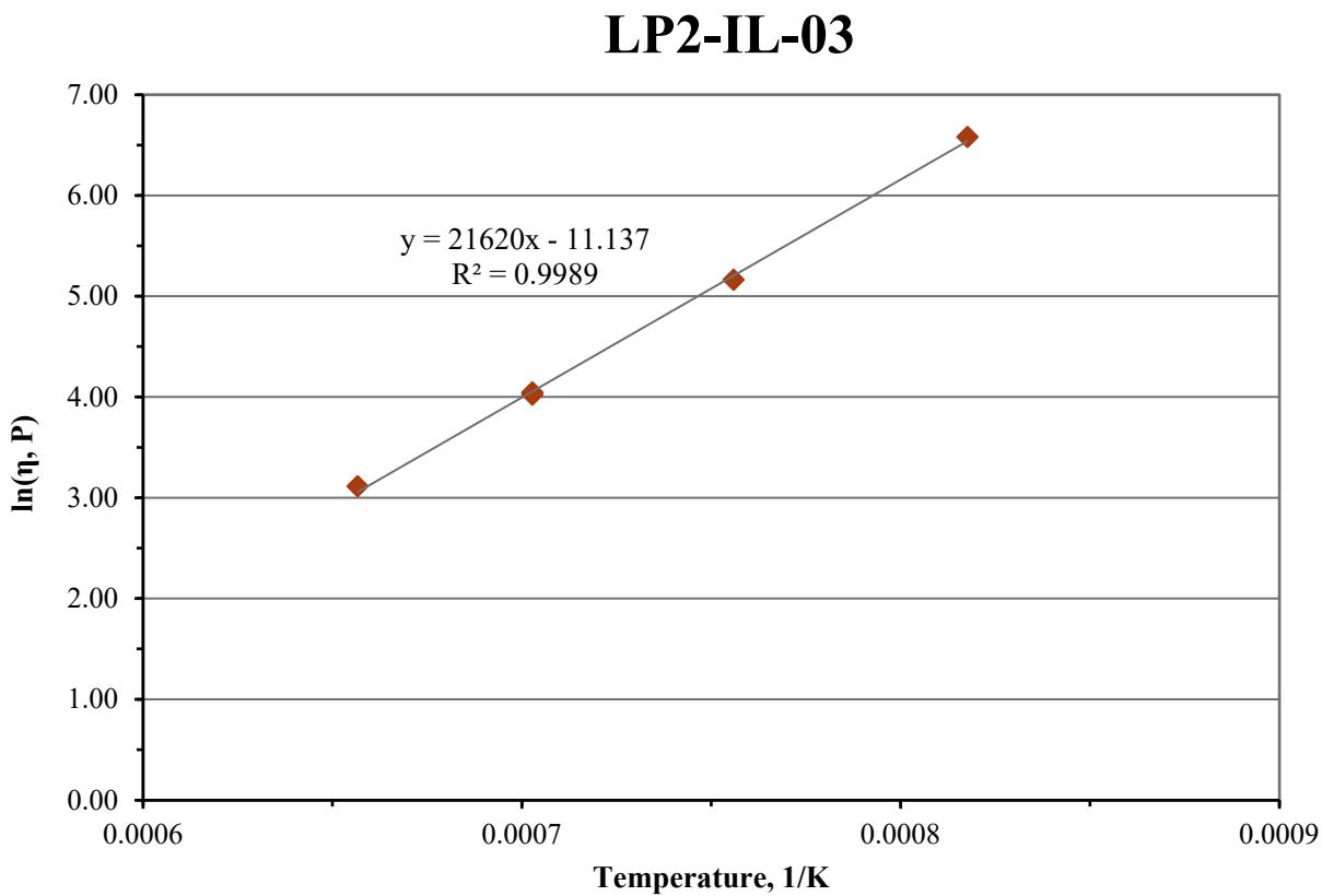
Figure C.3. Viscosity-Temperature Data and Arrhenius Equation Fit for Glass LP2-IL-03
