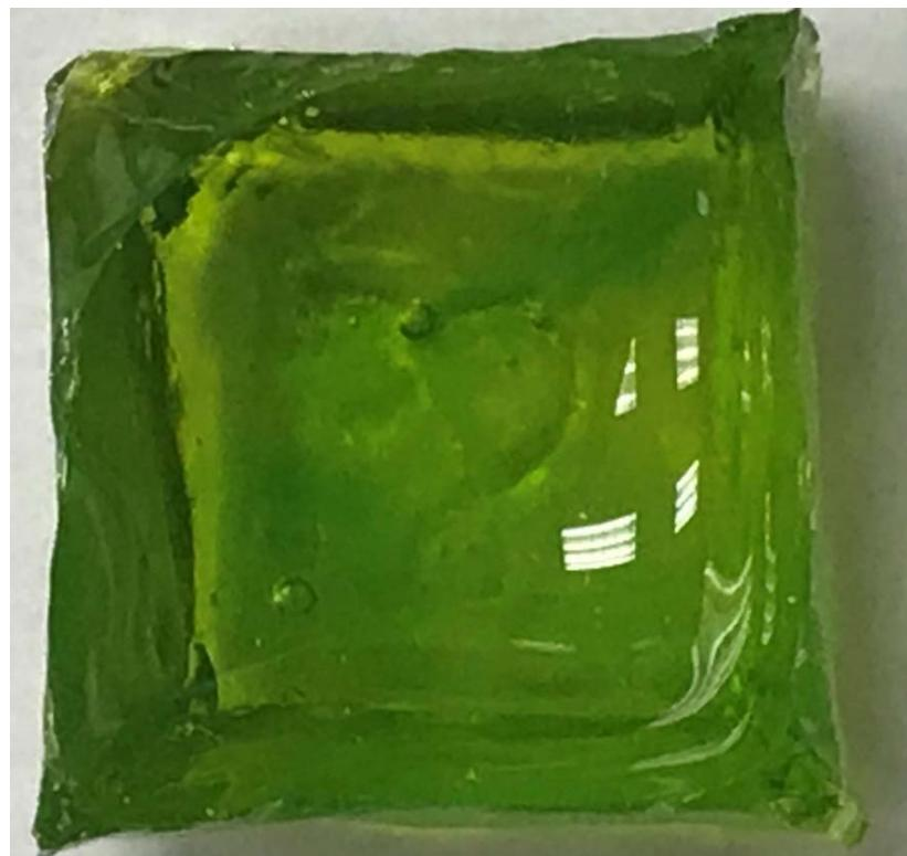
Figure E.38. Glass LP2-OL-23 after CF Heat Treatment at 950° C for 24 h
