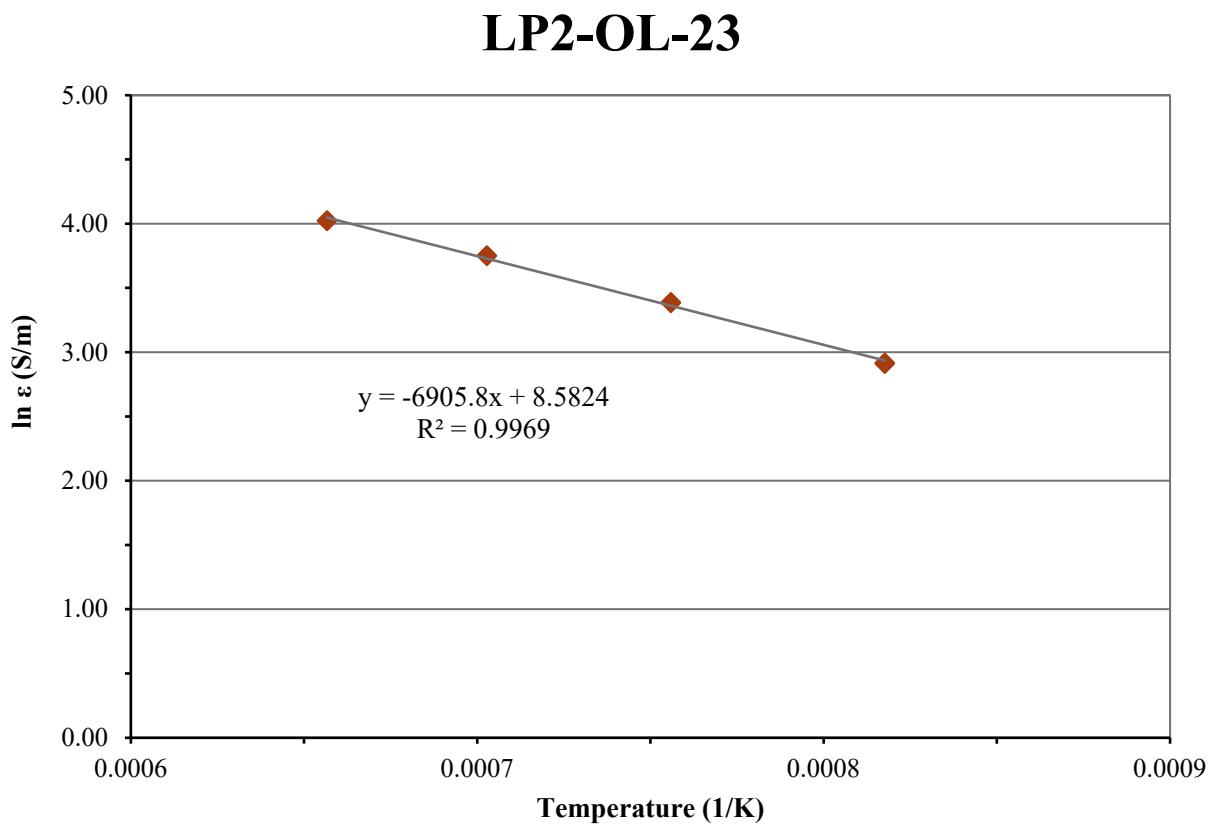
Figure D.39. Electrical Conductivity-Temperature Data and Arrhenius Equation Fit for Glass LP2-OL-23
