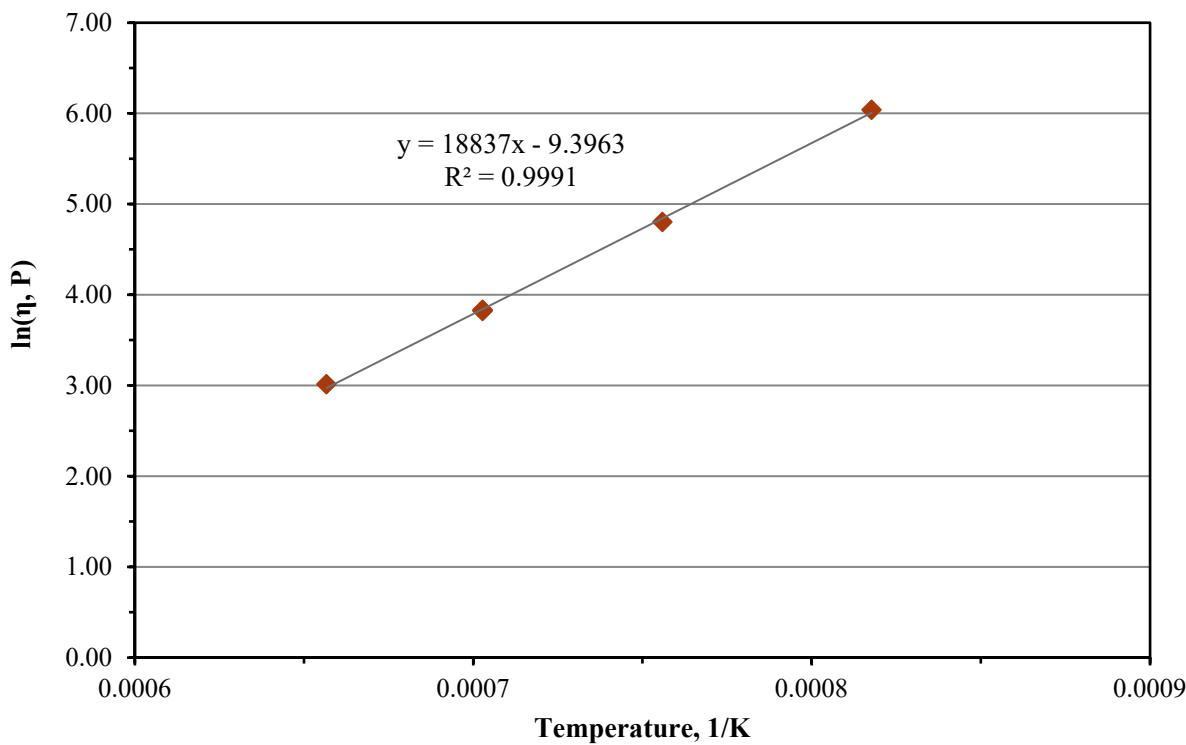
Figure C.36. Viscosity-Temperature Data and Arrhenius Equation Fit for Glass LP2-OL-20
