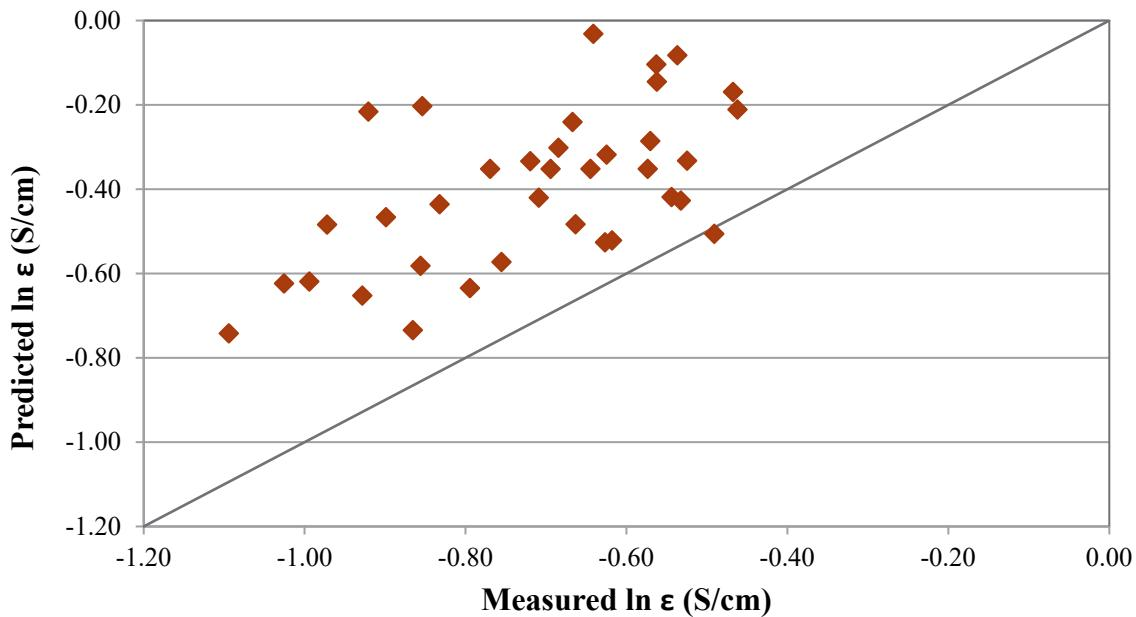
Figure 3.3. Predicted versus Measured Electrical Conductivity at 1150 °C Values for Phase 2 Enhanced LAW Glasses. The predicted values were obtained using the model in Equation (3.7) with coefficients in Table 3.6.
