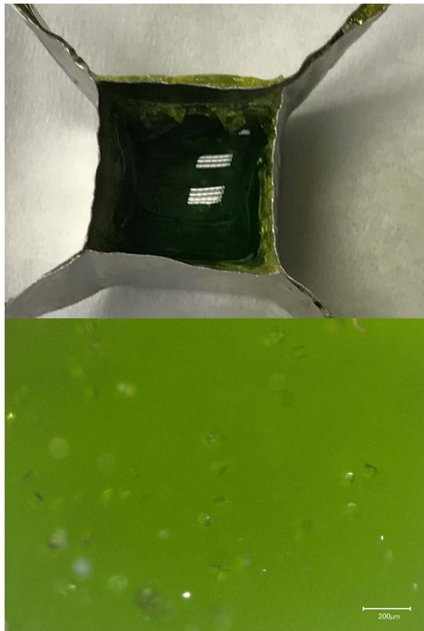
Figure E.10. Glass LP2-IL-11 after CF Heat Treatment at 950 °C for 24 h both in Crucible (top) and Magnified 200X (bottom)
