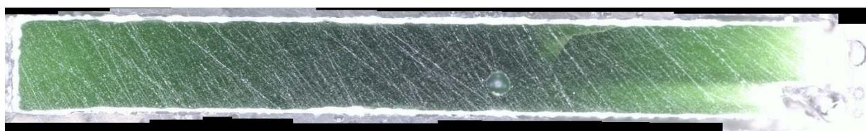
c) Glass cross section magnified after VHT
