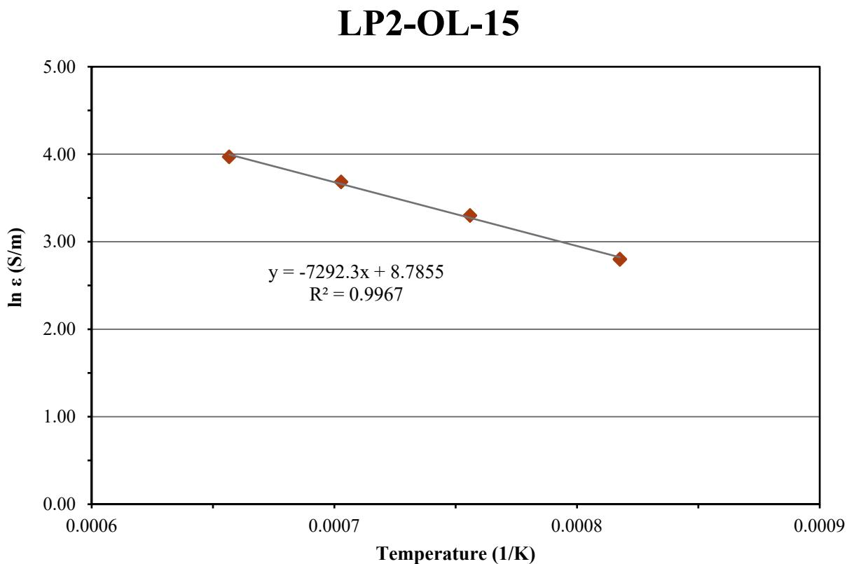
Figure D.31. Electrical Conductivity-Temperature Data and Arrhenius Equation Fit for Glass LP2-OL-15
