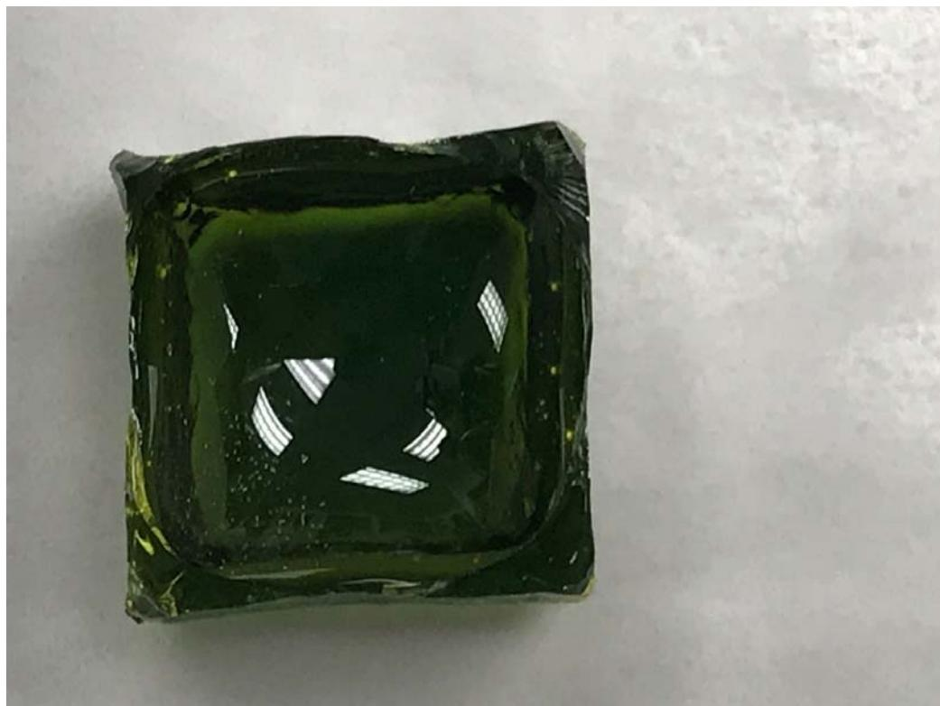
Figure E.30. Glass LP2-OL-15 after CF Heat Treatment at 950 °C for 24 h
