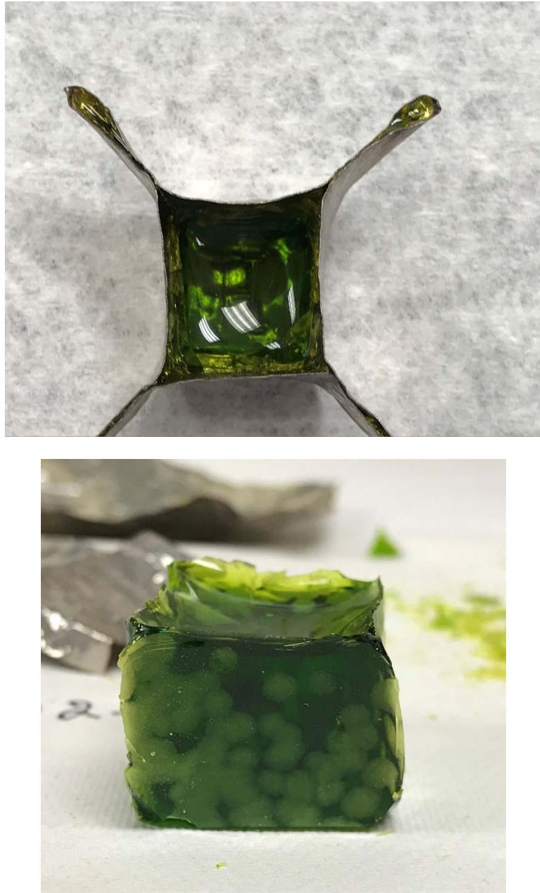
Figure G.19. Glass LP2-OL-02-1 after CCC Beginning at 1150 °C both in Crucible (top) and Glass (bottom)
