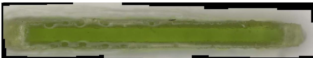
c) Glass cross section magnified after VHT
