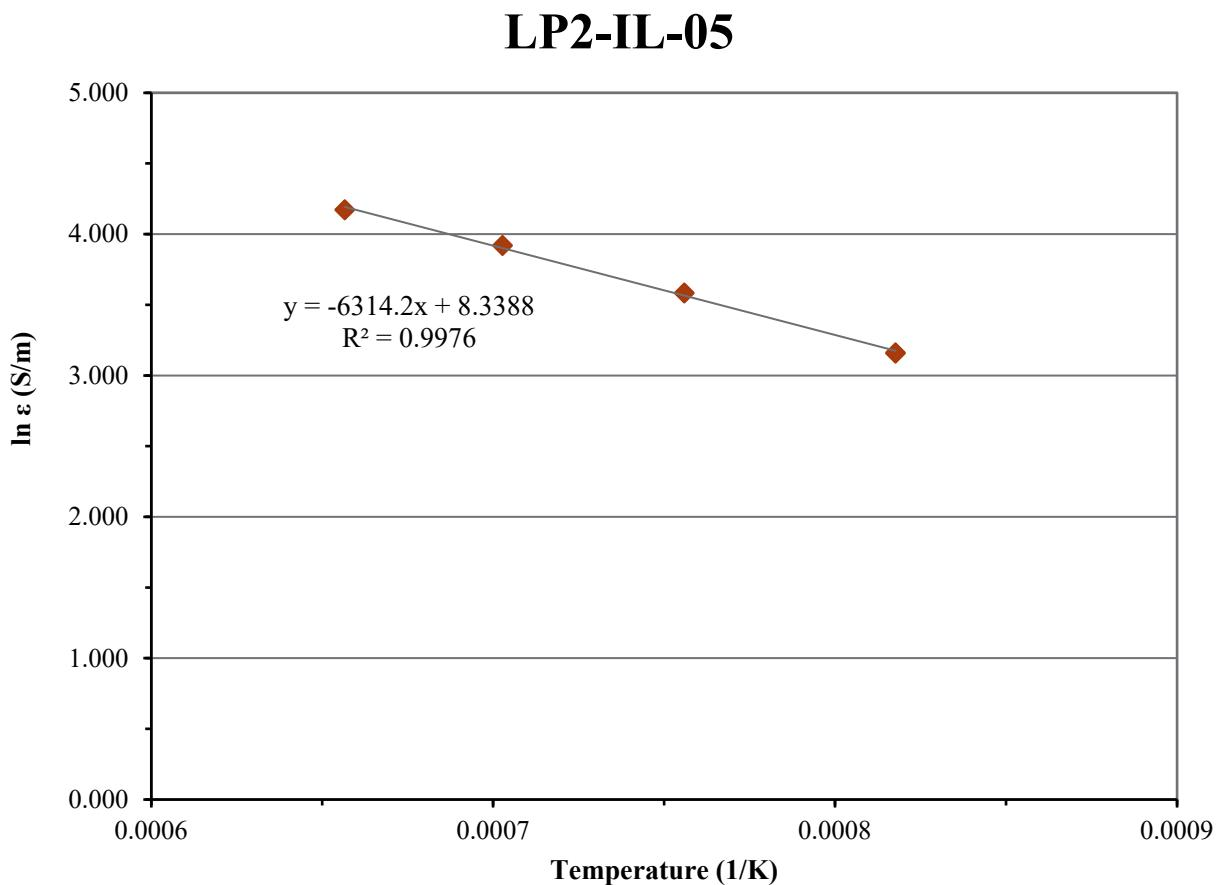
Figure D.5. Electrical Conductivity-Temperature Data and Arrhenius Equation Fit for Glass LP2-IL-05
