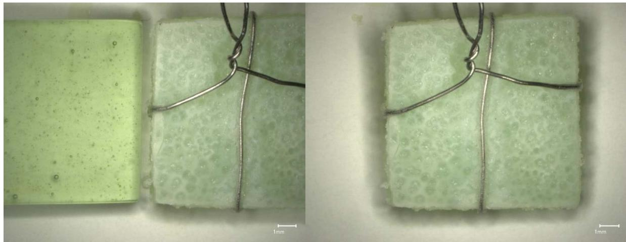
a) Glass square after (right) and before (left) VHT; b) Glass square after VHT
