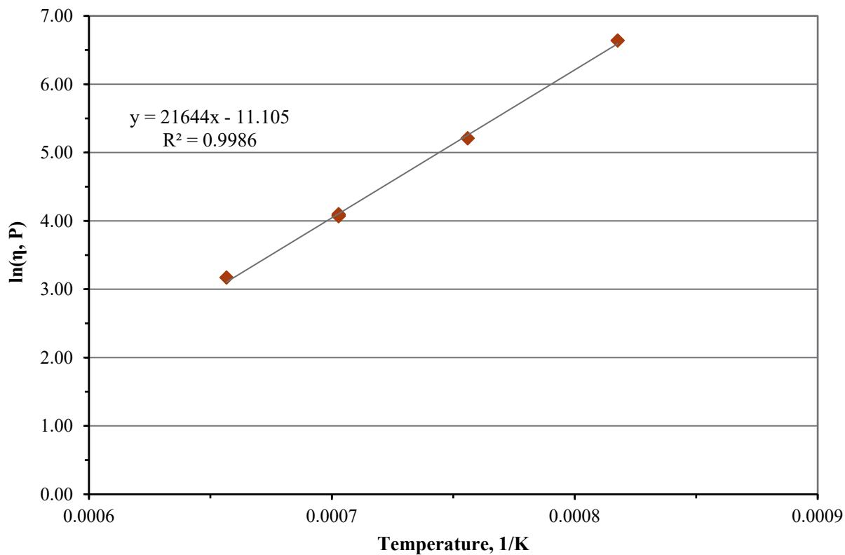
Figure C.11. Viscosity-Temperature Data and Arrhenius Equation Fit for Glass LP2-IL-11
