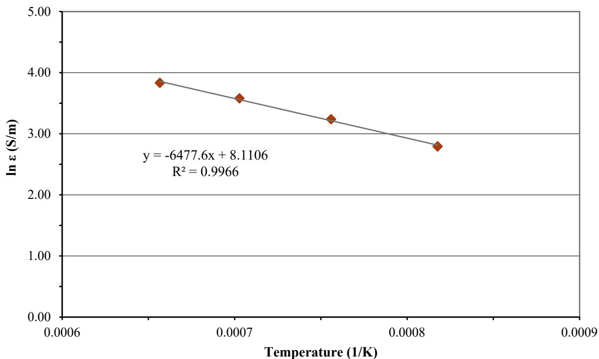
Figure D.22. Electrical Conductivity-Temperature Data and Arrhenius Equation Fit for Glass LP2-OL-05
