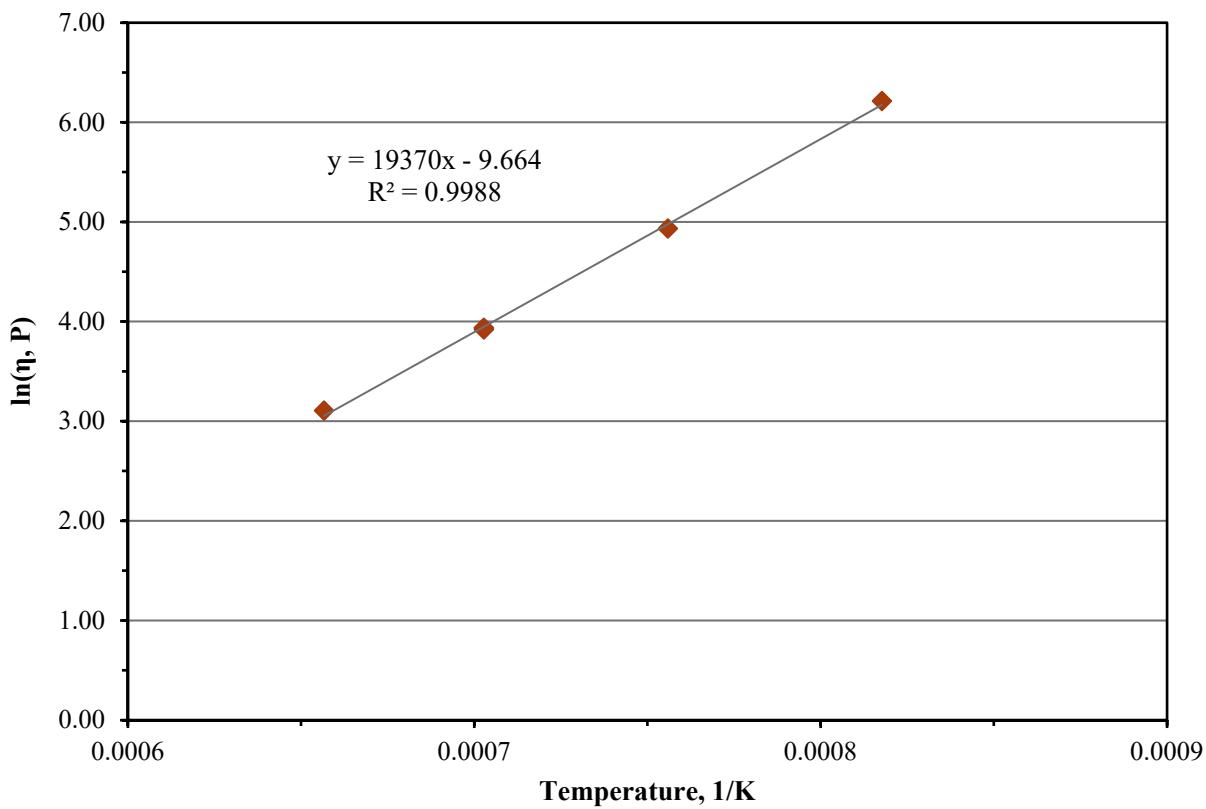
Figure C.17. Viscosity-Temperature Data and Arrhenius Equation Fit for Glass LP2-IL-17
