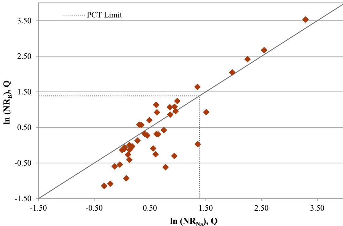
Figure 3.6. Comparison of Natural Logarithms of PCT Normalized Releases of B and Na (both g/L) for Quenched Samples of Phase 2 Enhanced LAW Glasses
