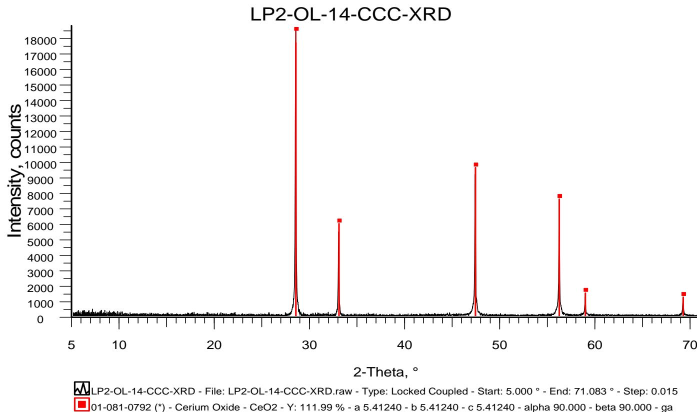
Figure H.15. XRD Spectrum of CCC-Treated Glass LP2-OL-14
