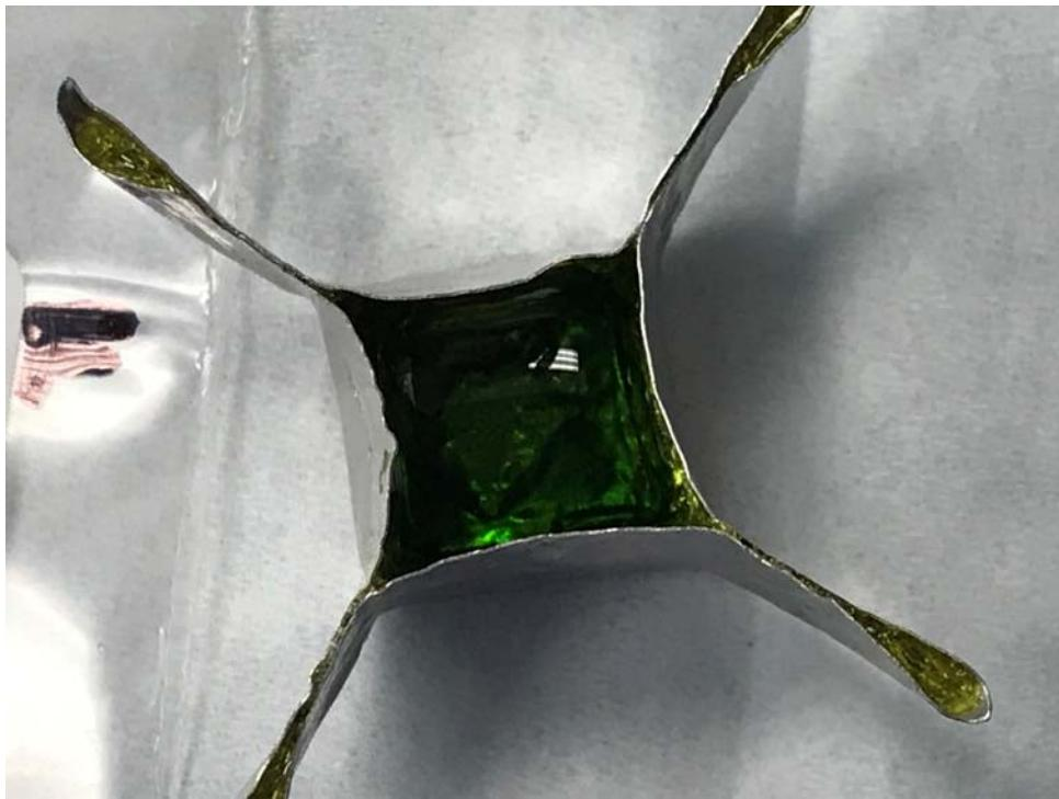
Figure E.15. Glass LP2-IL-16 after CF Heat Treatment at 950 °C for 24 h
