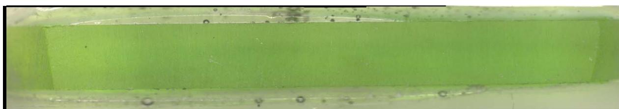
c) Glass cross section magnified after VHT
