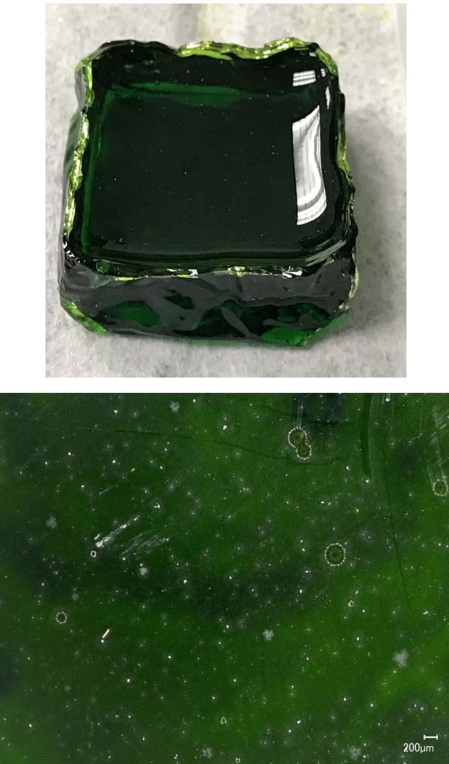
Figure G.12. Glass LP2-IL-12 after CCC Beginning at 1150 °C both Glass (top) and Magnified 50X (bottom)
