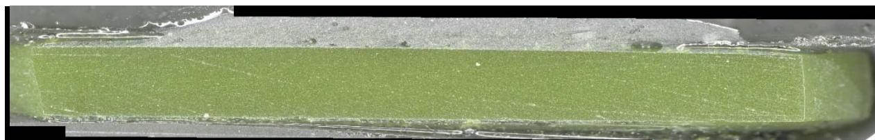
c) Glass cross section magnified after VHT
