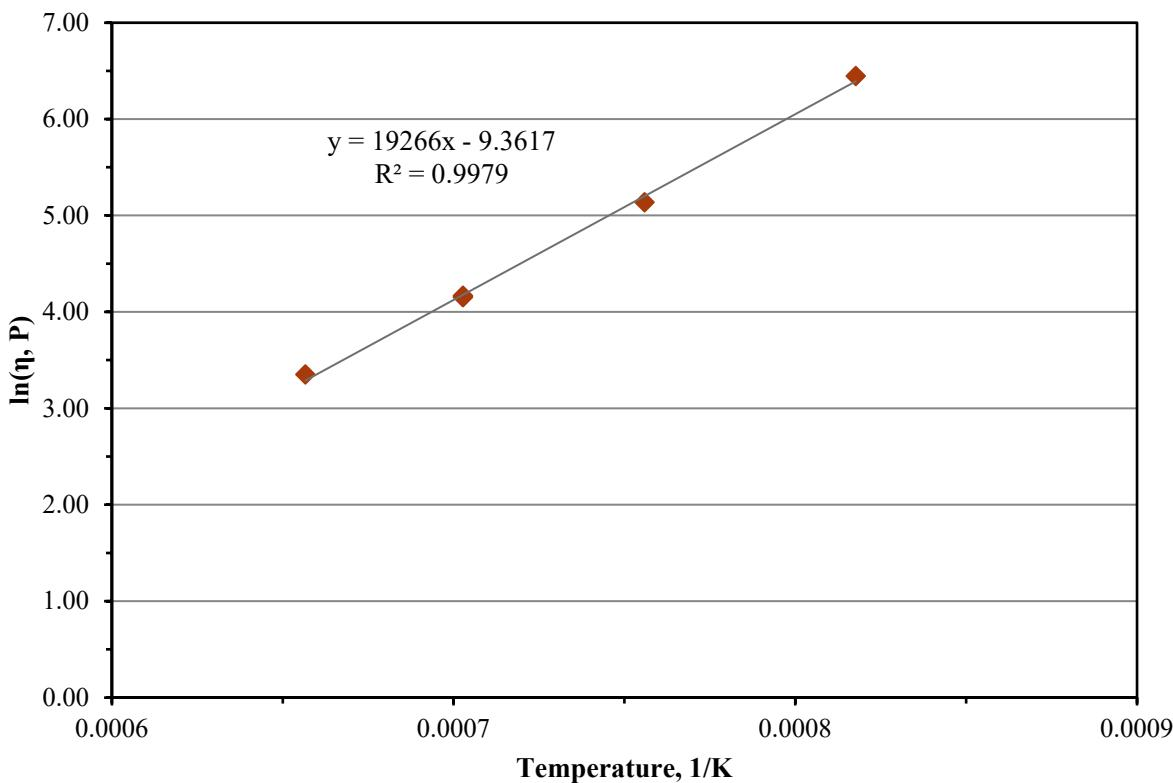
Figure C.25. Viscosity-Temperature Data and Arrhenius Equation Fit for Glass LP2-OL-09-1
