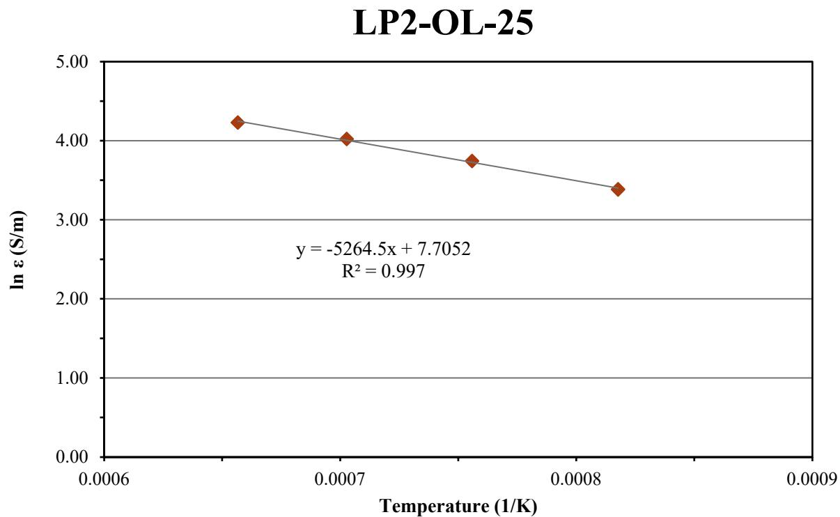
Figure D.41. Electrical Conductivity-Temperature Data and Arrhenius Equation Fit for Glass LP2-OL-25
