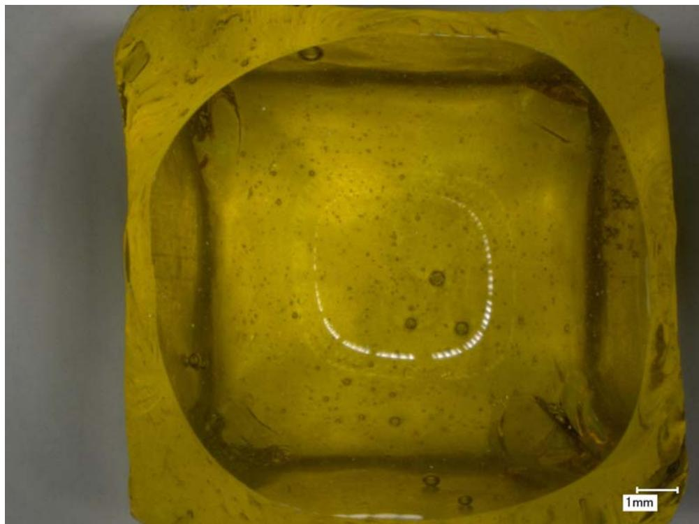
Figure E.32. Glass LP2-OL-17 after CF Heat Treatment at 950 °C for 24 h Magnified 20X
