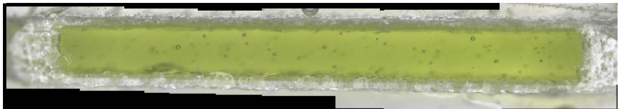
b) Glass cross section magnified after VHT
