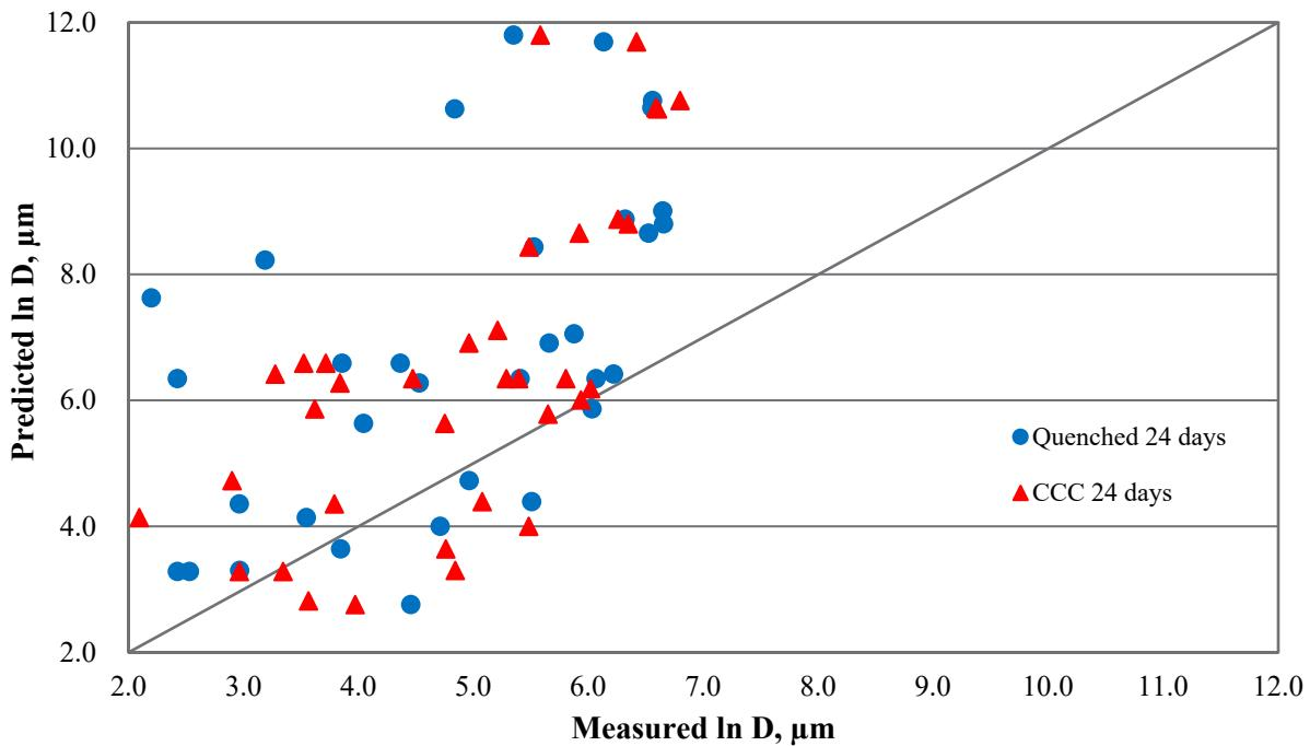
Figure 3.12. Natural Logarithm of VHT Alteration Depth Results Predicted using 15-Term Reduced Partial Cubic Mixture Model Versus Measured Values for Phase 2 Enhanced LAW Glasses
