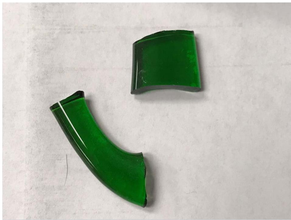
Figure A.12. Photo of Glass LP2-IL-12 Morphology of Third Melt at 1175 °C for 1 h
