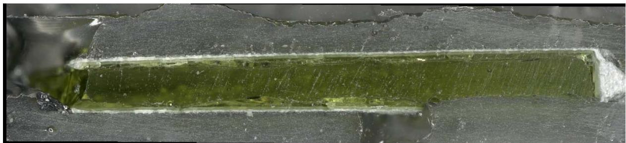
b) Glass cross section magnified after VHT
