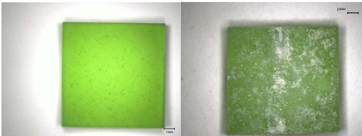
a) Glass square magnified 20X before VHT; b) Glass square magnified 20X after VHT
