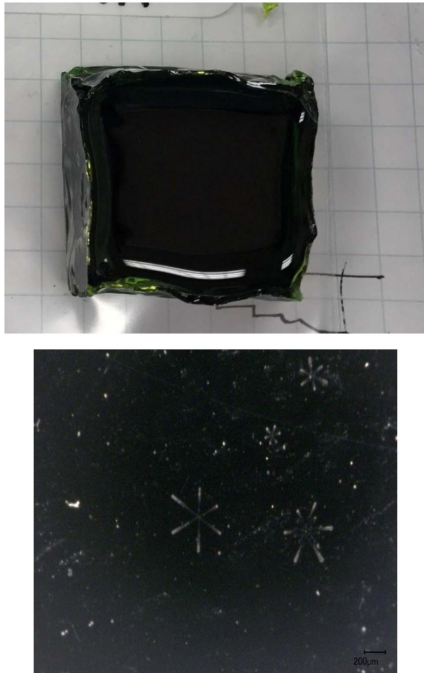
Figure G.9. Glass LP2-IL-09 after CCC Beginning at 1150 °C both Glass (top) and Magnified 100X (bottom)
