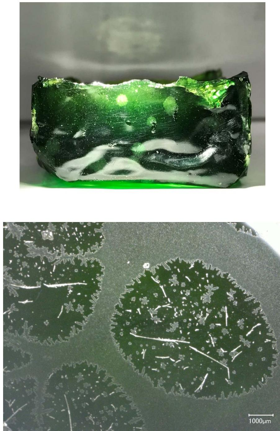
Figure G.10. Glass LP2-IL-10 CCC Beginning at 1150° C both Glass (top) and Magnified 30X (bottom)
