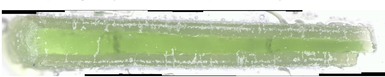
Figure I.83. CCC-Treated Glass LP2-IL-10 after VHT for 24 Days
