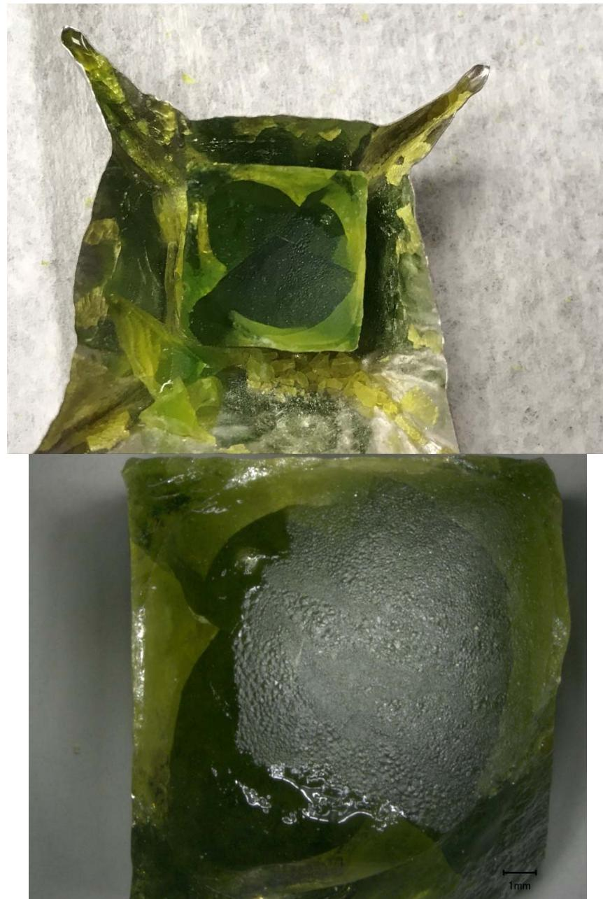
Figure E.21. Glass LP2-OL-05 after CF Heat Treatment at 950 °C for 24 h both in crucible (top) and magnified 20X (bottom)
