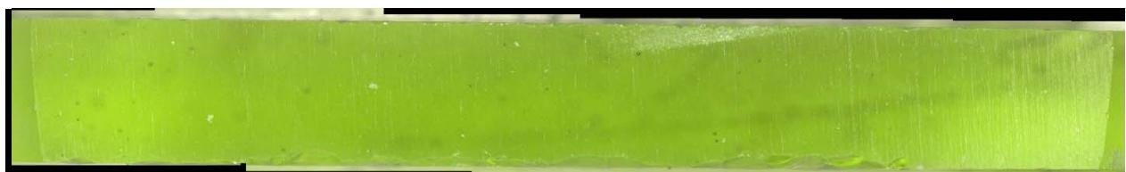
c) Glass cross section magnified after VHT
