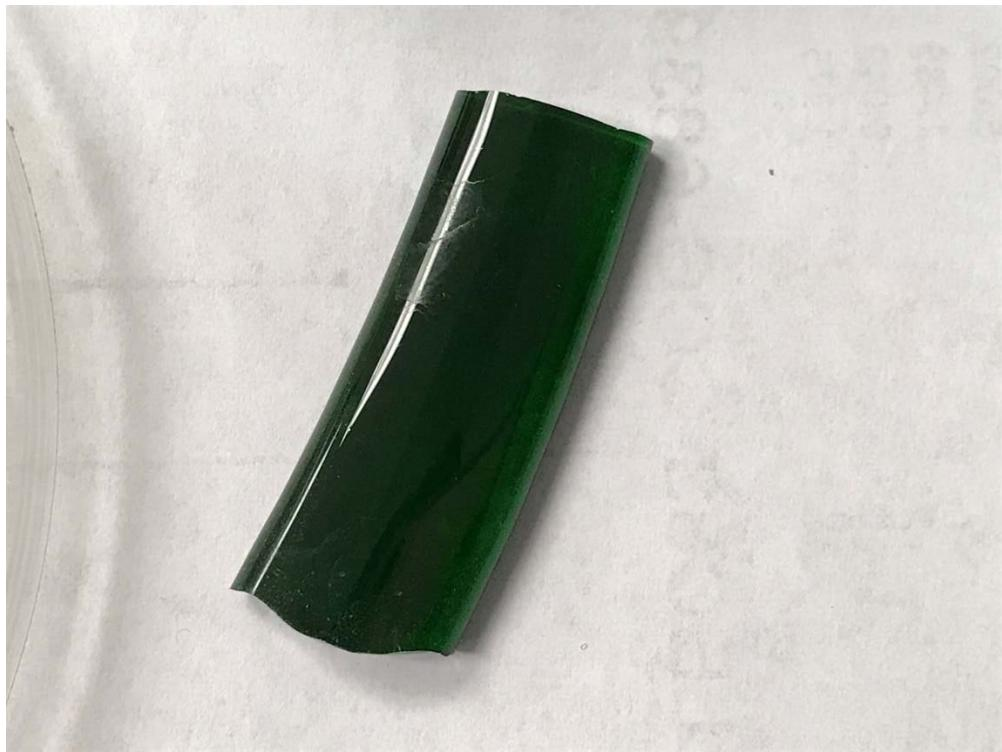
Figure A.13. Photo of Glass LP2-IL-13 Morphology of Second Melt at 1150 °C for 1.5 h
