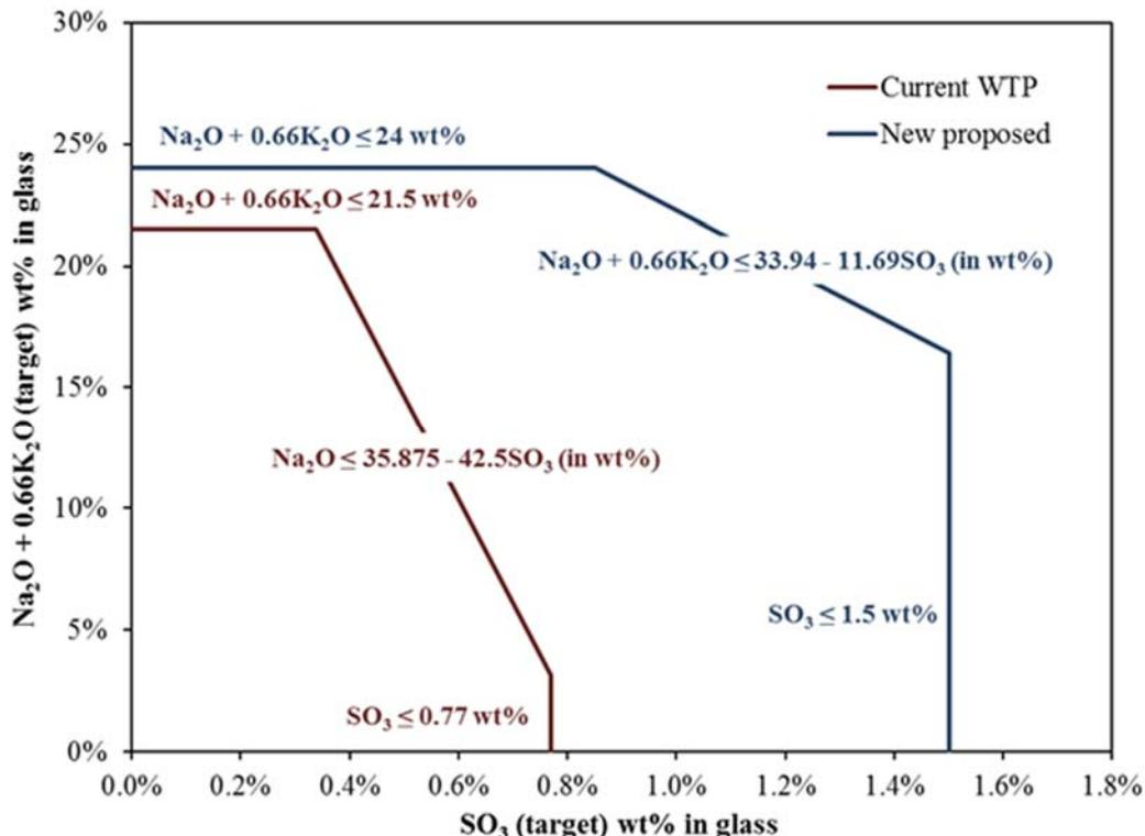
Figure 1.1. Plot of Glass Waste Loading Constraints for the Current WTP and Advanced ORP LAW Glasses as Projected Based on  $\text{Na}_2\text{O}+0.66\text{K}_2\text{O}$  Versus  $\text{SO}_3$  Concentrations in Glass (Vienna et al. 2016)
