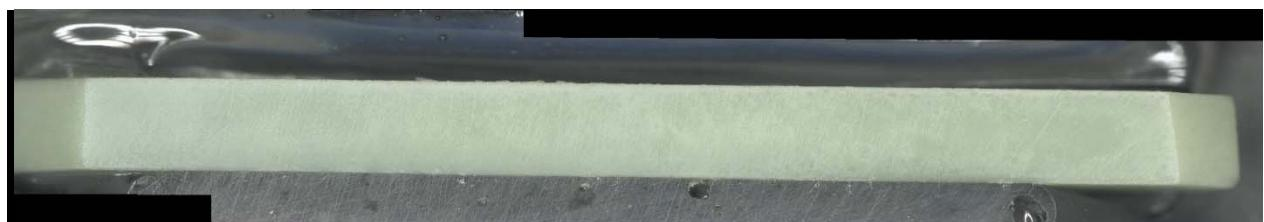
Figure I.98. CCC-Treated Glass LP2-OL-03 MOD2 after VHT for 7 Days
