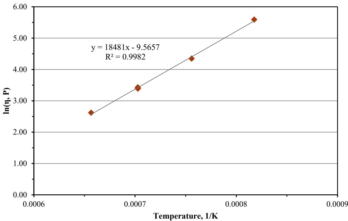
Figure C.23. Viscosity-Temperature Data and Arrhenius Equation Fit for Glass LP2-OL-07-1
