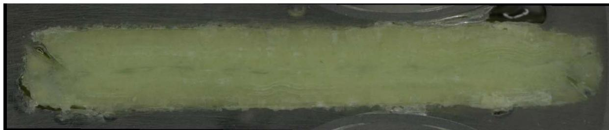
c) Glass cross section magnified after VHT
