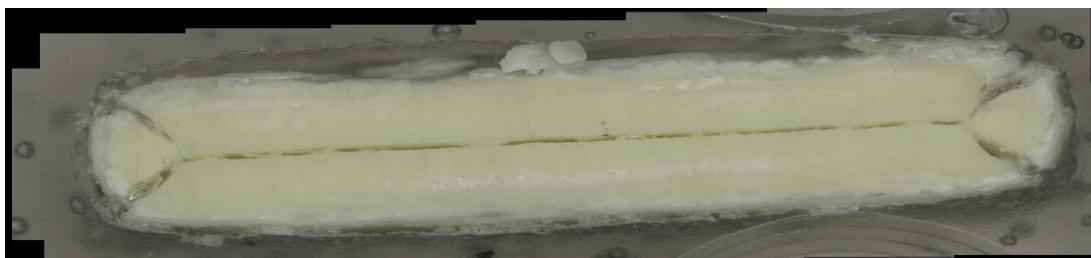
c) Glass cross section magnified after VHT
