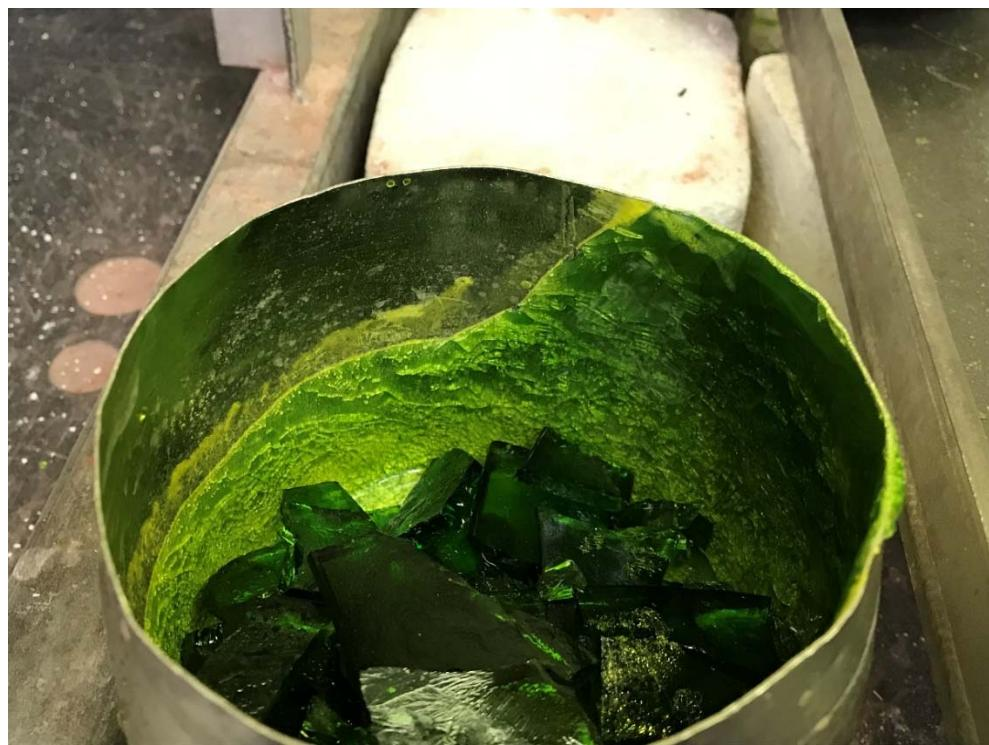
Figure 2.3. Glass LP2-OL-03 First Modified Composition after Third Melt
