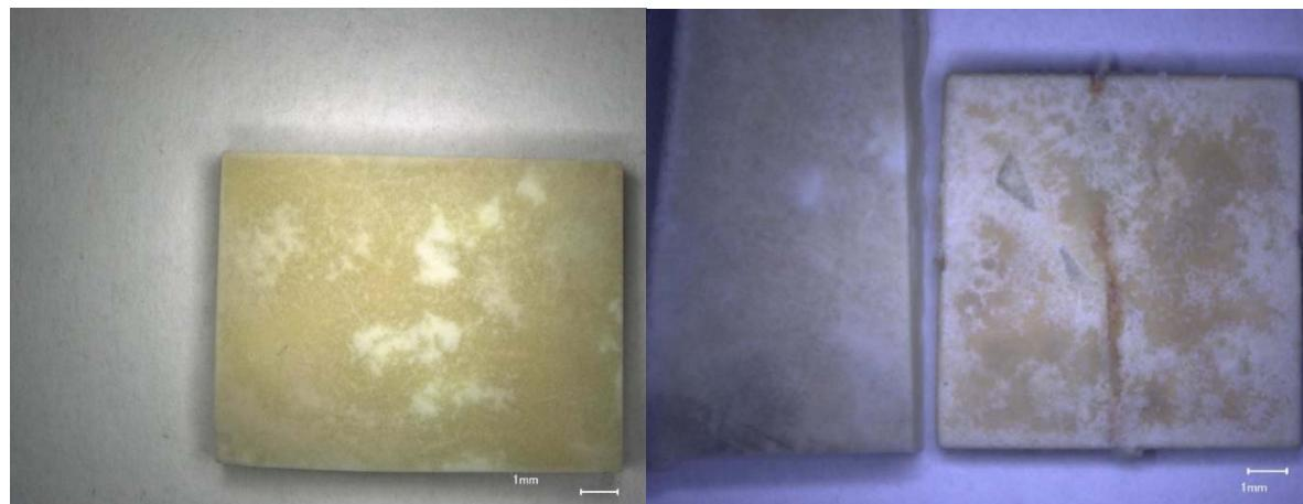
a) Glass square magnified 20X before VHT b) Glass square before (on left) and after (on right) VHT
