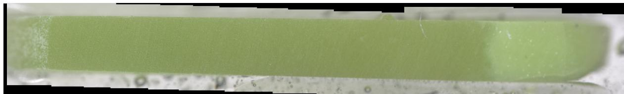
b) Glass cross section magnified after VHT
