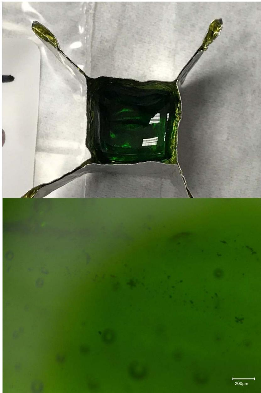
Figure E.12. Glass LP2-IL-13 after CF Heat Treatment at 950 °C for 24 h both in Crucible (top) and Magnified 150X (bottom)
