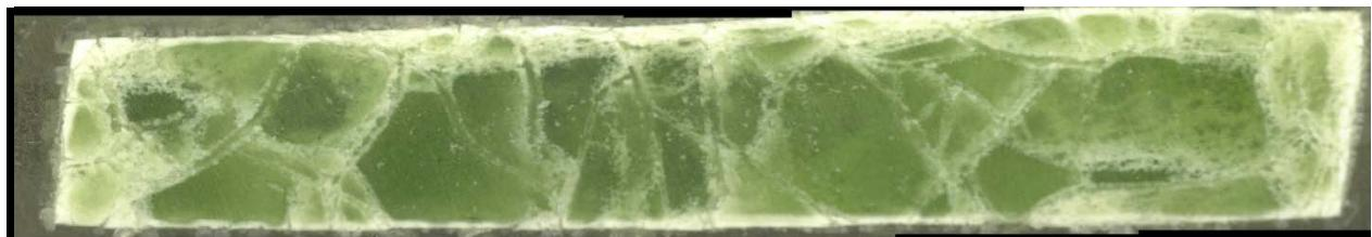
c) Glass cross section magnified after VHT
