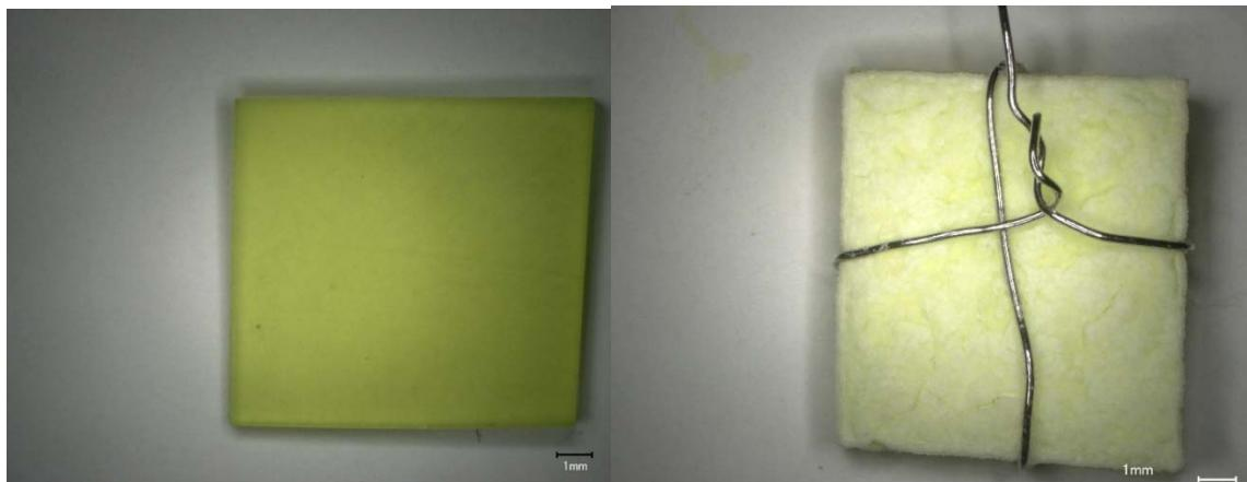
a) Glass square magnified 20X after VHT; b) Glass surface magnified after VHT
