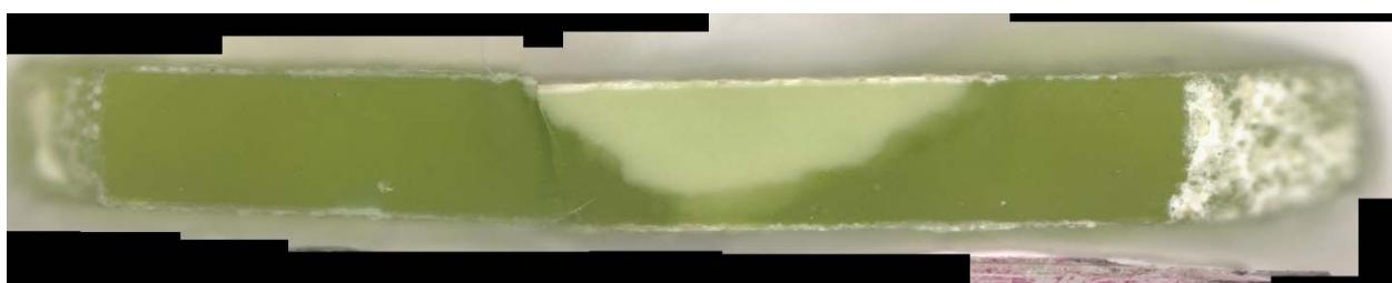
Figure I.102. CCC-Treated Glass LP2-OL-05 after VHT for 24 Days
