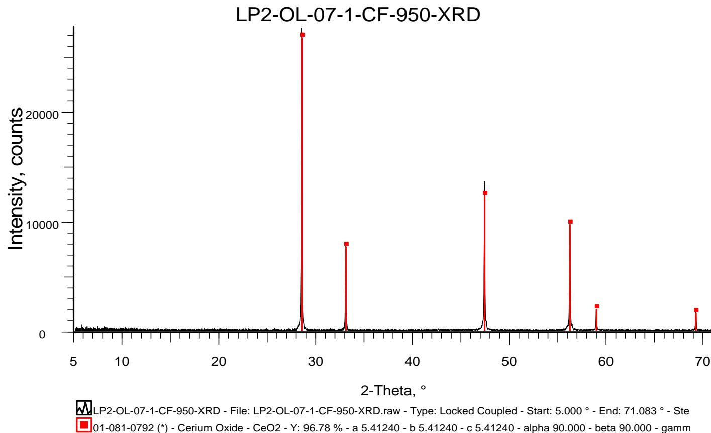
Figure F.14. XRD Spectrum of Heat-Treated Glass LP2-OL-07-1
