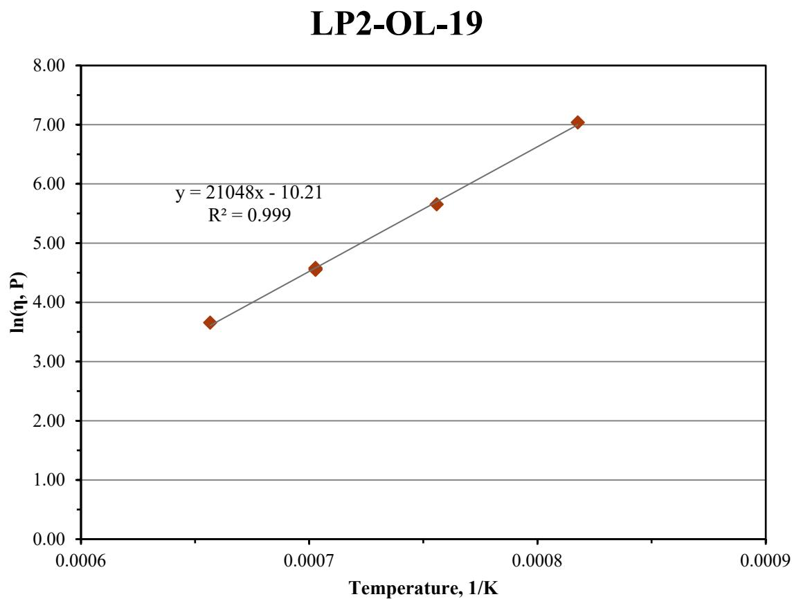
Figure C.35. Viscosity-Temperature Data and Arrhenius Equation Fit for Glass LP2-OL-19
