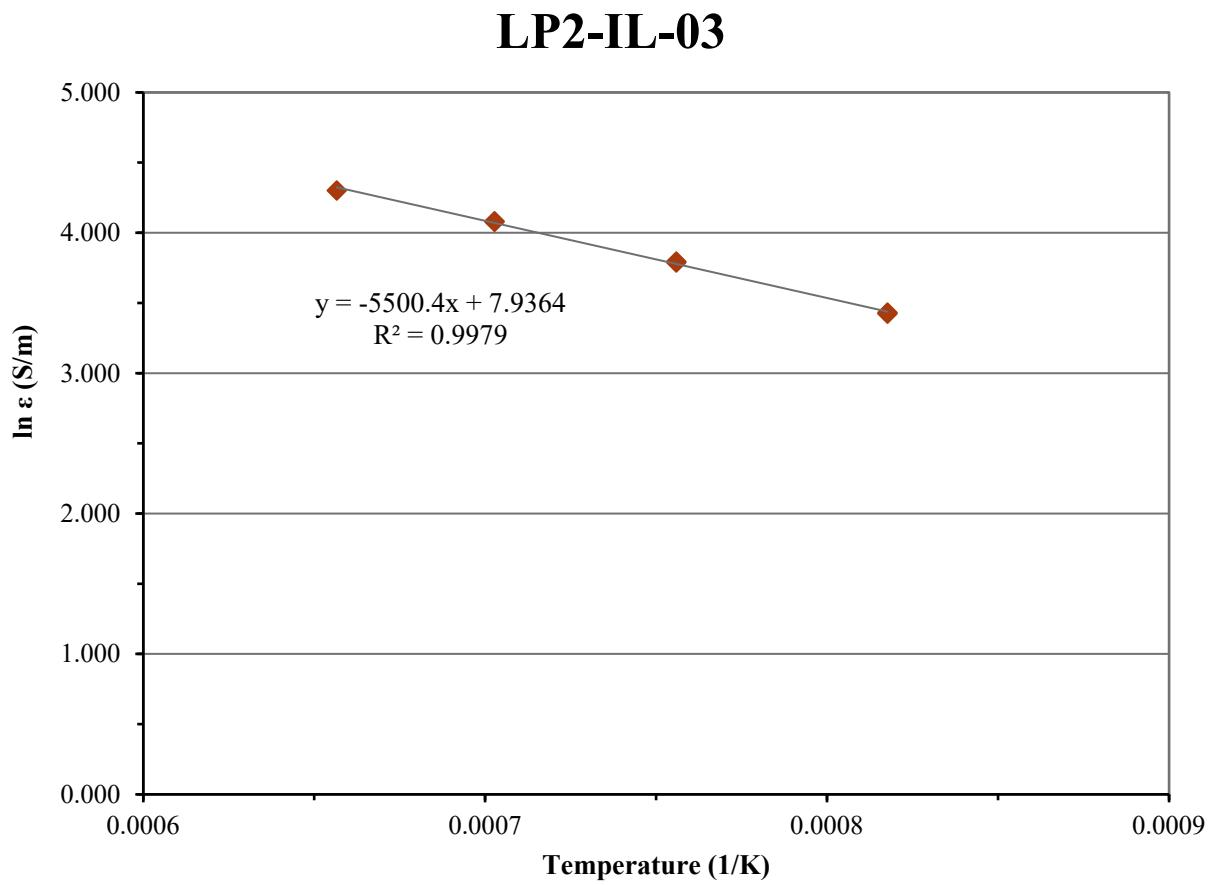
Figure D.3. Electrical Conductivity-Temperature Data and Arrhenius Equation Fit for Glass LP2-IL-03
