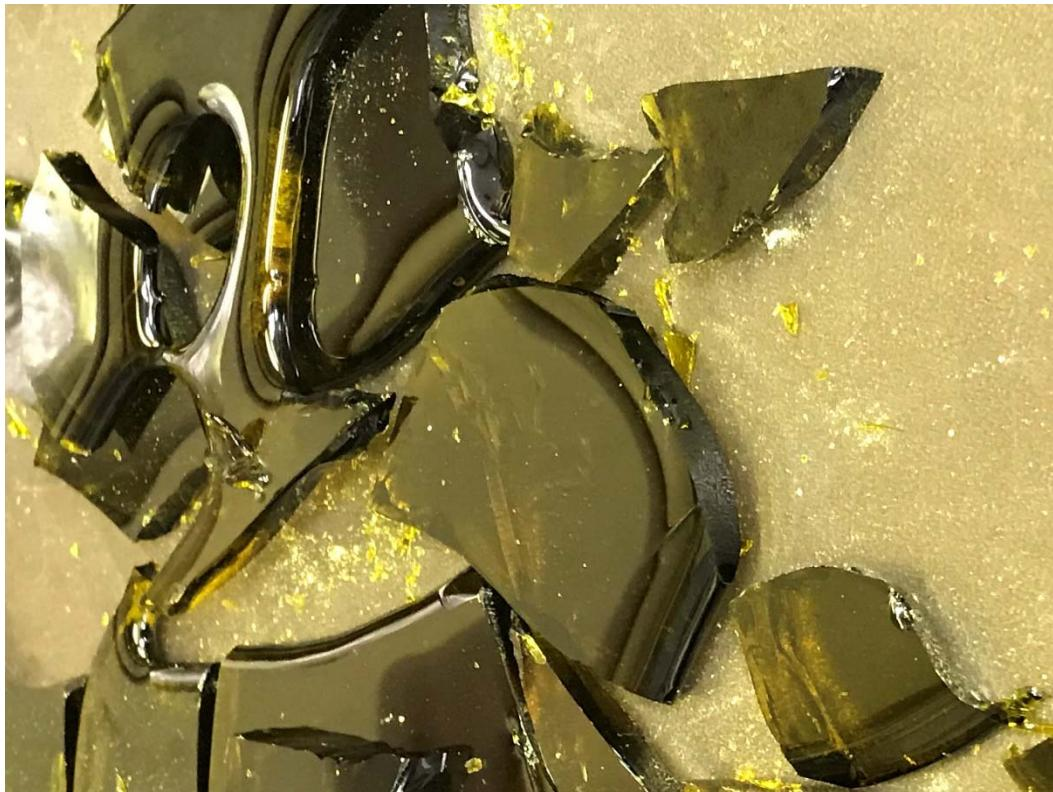
Figure A.24. Photo of Glass LP2-OL-08MOD Morphology of Second Melt at 1200 °C for 1.3 h
