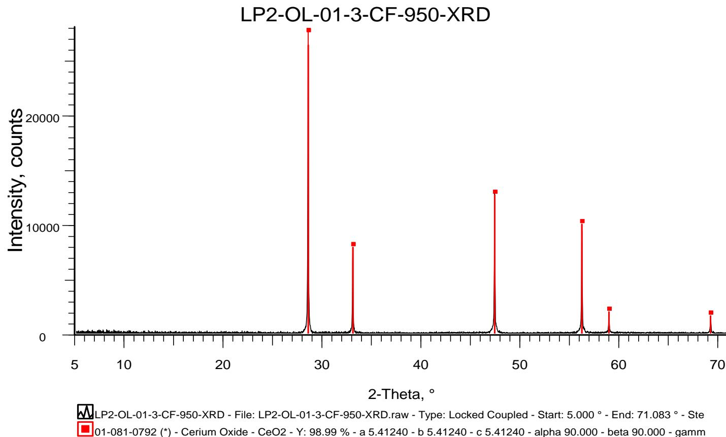
Figure F.10. XRD Spectrum of Heat-Treated Glass LP2-OL-01-3
