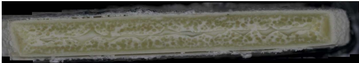
b) Glass cross section magnified after VHT
