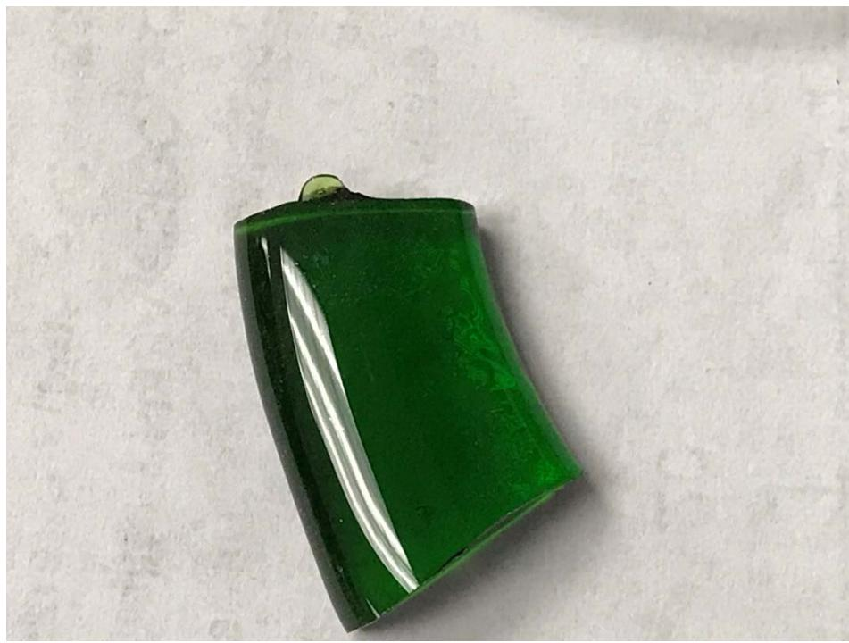
Figure A.16. Photo of Glass LP2-IL-16 Morphology of Second Melt at 1175 °C for 0.75 h
