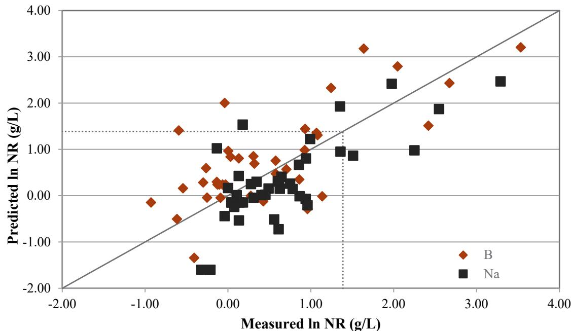
Figure 3.8. Predicted Versus Measured Natural Logarithms of Normalized Releases (g/L) of Boron and Sodium for Phase 2 Enhanced LAW Glasses. The predicted values were obtained using the model form in Equation (3.8) with coefficients listed in Tables 3.10 and 3.11.
