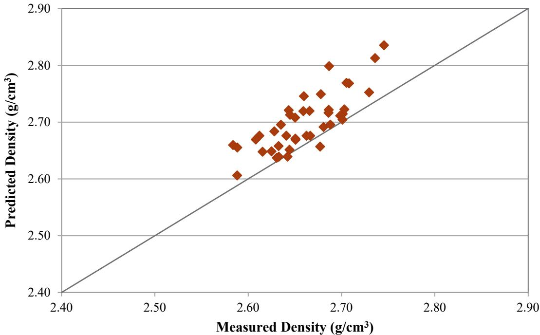
Figure 3.1. Predicted versus Measured Density for Phase 2 Enhanced LAW Glasses. The predicted values were obtained using the model in Equation (3.1).
