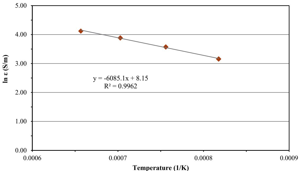
Figure D.27. Electrical Conductivity-Temperature Data and Arrhenius Equation Fit for Glass LP2-OL-11
