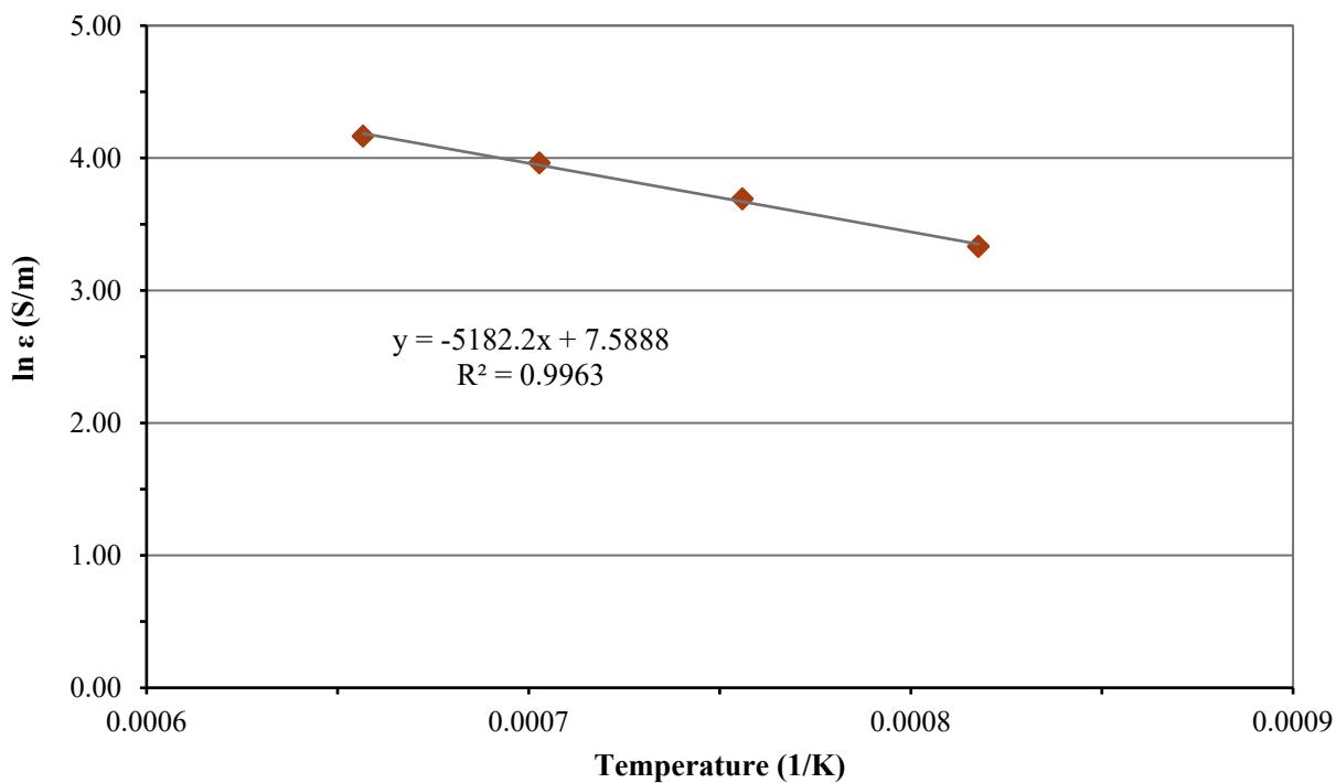
Figure D.40. Electrical Conductivity-Temperature Data and Arrhenius Equation Fit for Glass LP2-OL-24
