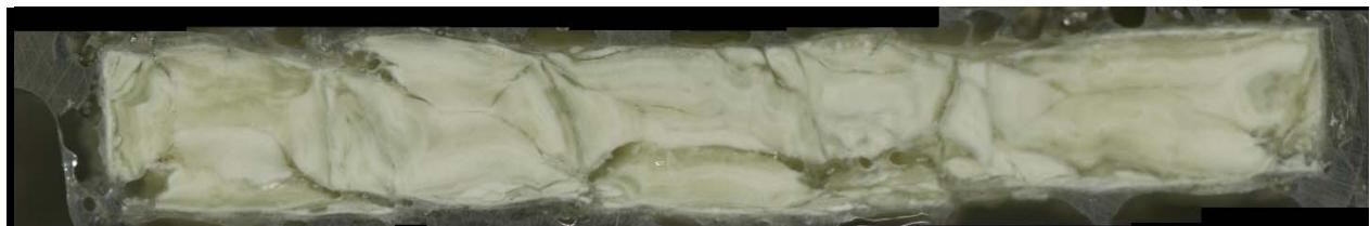
c) Glass cross section magnified after VHT
