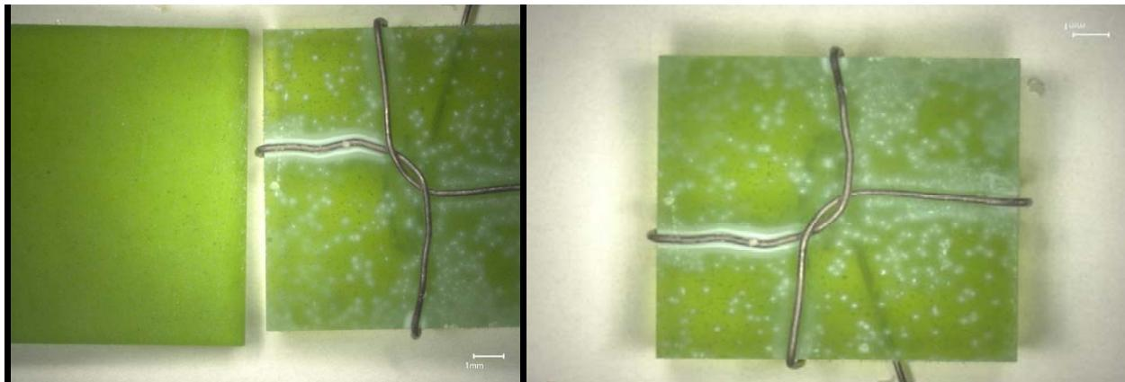
a) Glass square after (right) and before (left) VHT; b) Glass square after VHT
