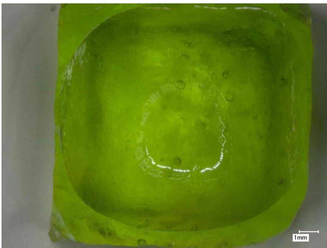
Figure E.35. Glass LP2-OL-20 after CF Heat Treatment at 950 °C for 24 h Magnified 20X
