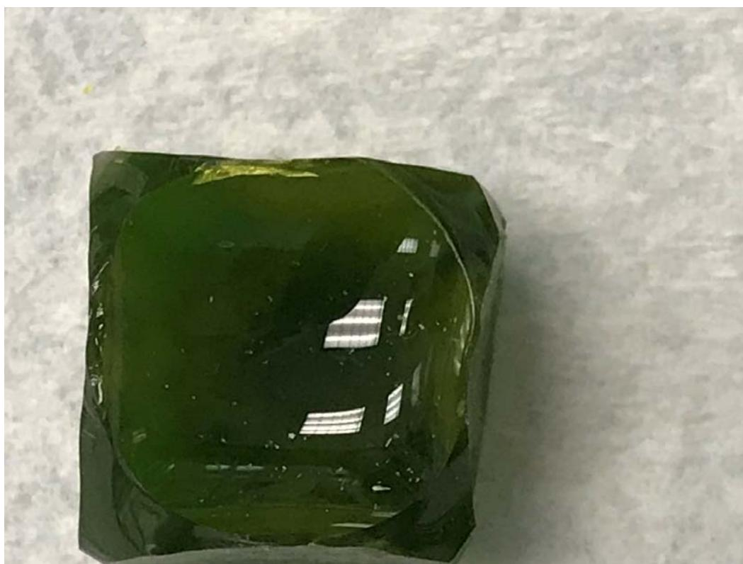
Figure E.31. Glass LP2-OL-16 MOD after CF Heat Treatment at 950 °C for 24 h
