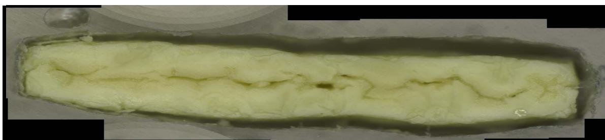
c) Glass cross section magnified after VHT
