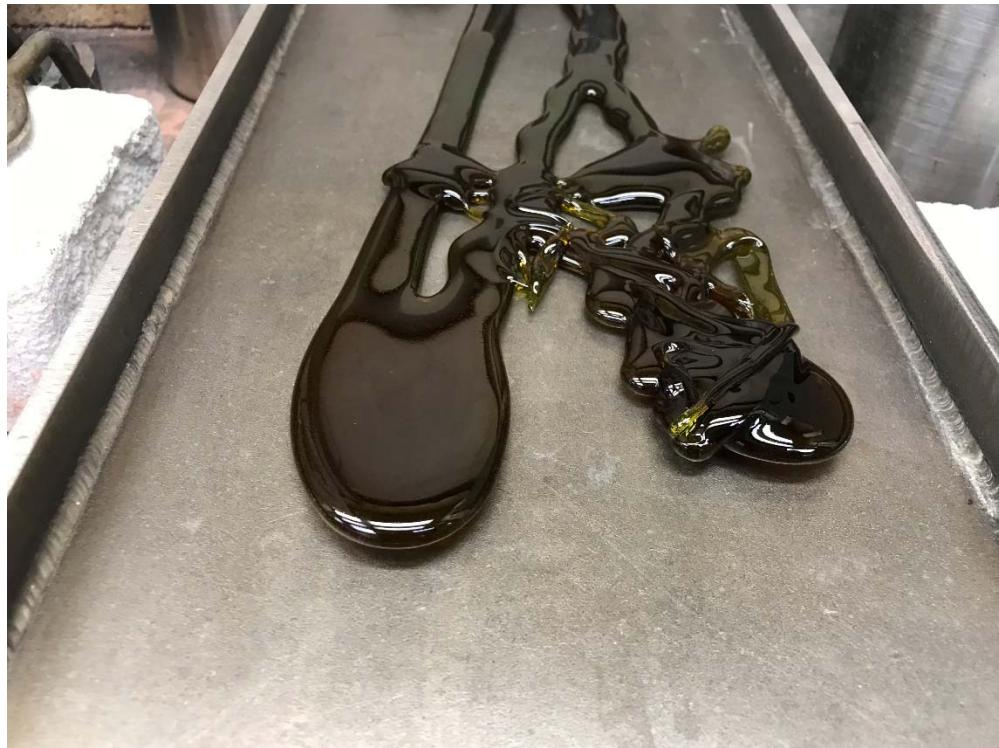
Figure A.26. Photo of Glass LP2-OL-10 MOD Morphology of Second Melt at 1150 °C for 1.5 h
