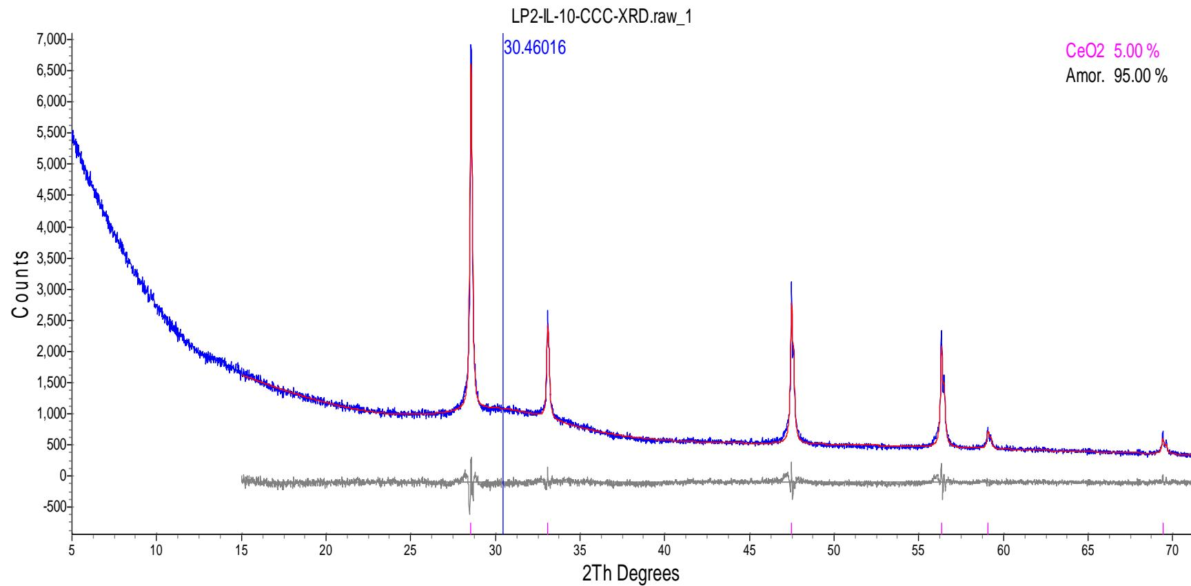
Figure H.4. XRD Spectrum of CCC-Treated Glass LP2-IL-10
