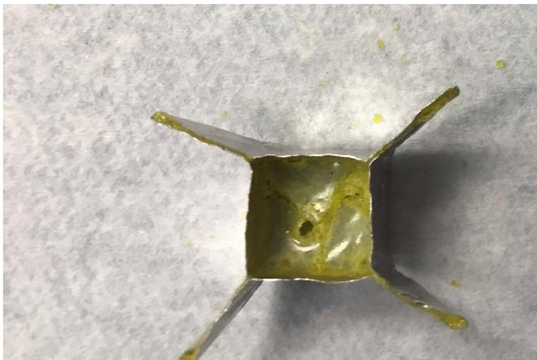
Figure E.23. Glass LP2-OL-08 MOD after CF Heat Treatment at 950 °C for 24 h
