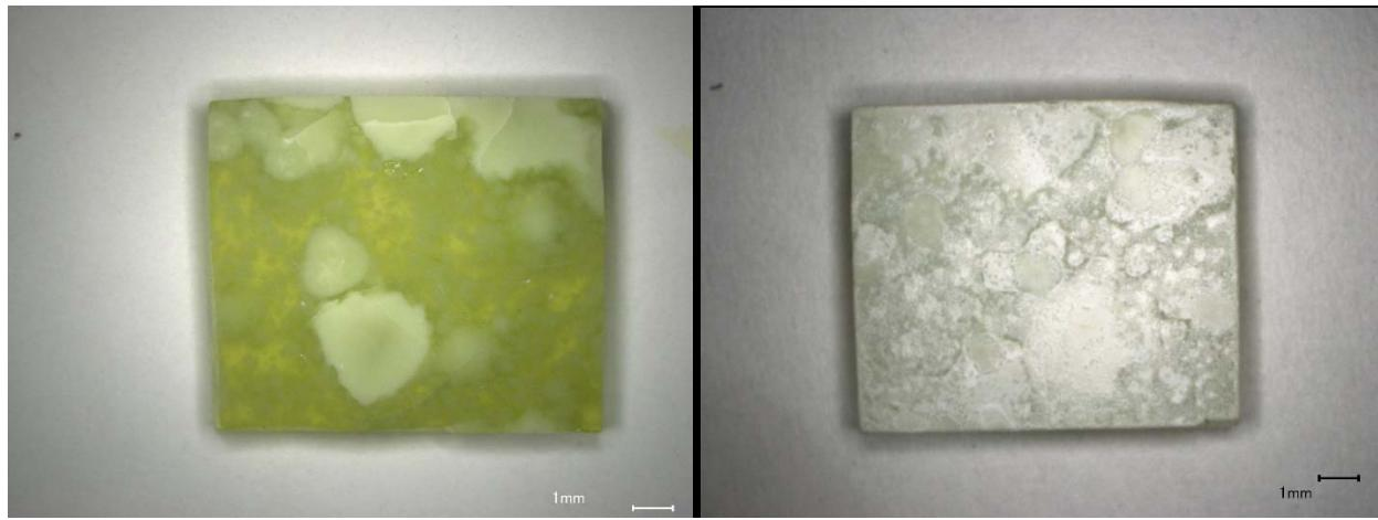
a) Glass square magnified 20X before VHT; b) Glass square magnified after VHT
