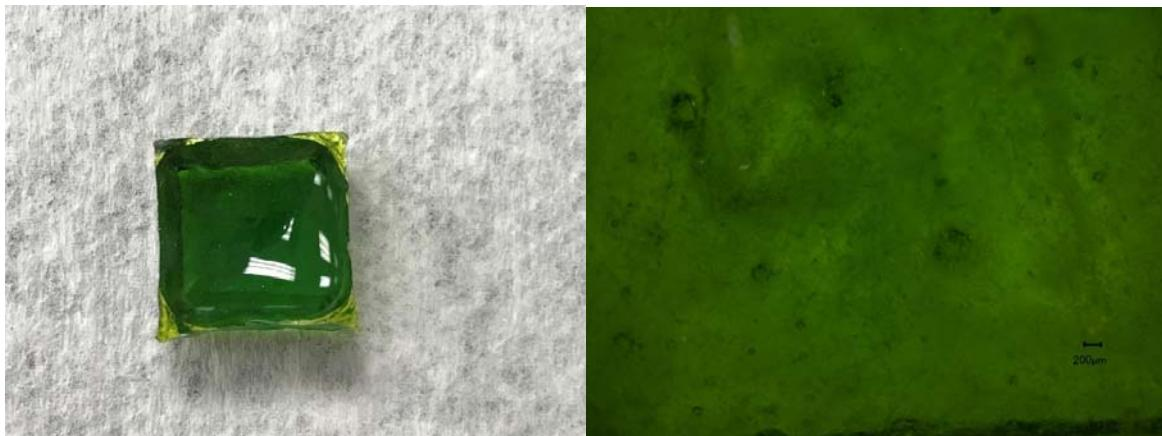
Figure E.17. Glass LP2-OL-01-3 after CF Heat Treatment at 950 °C for 24 h both Glass (left) and Magnified 50X (right)
