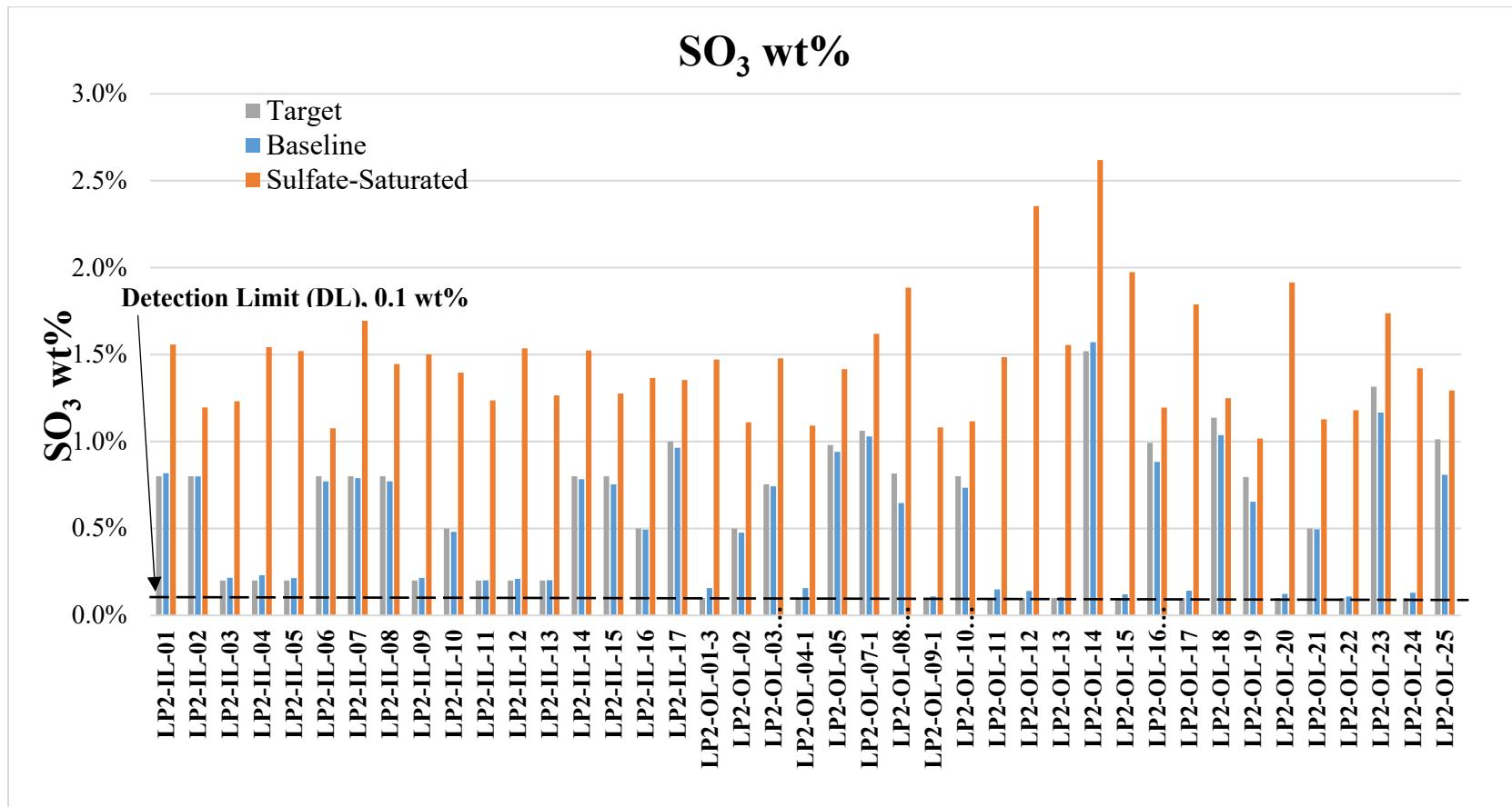
Figure 3.14. Analyzed Sulfur Concentration (wt%) in the Baseline and the Sulfur-Saturated Glasses
