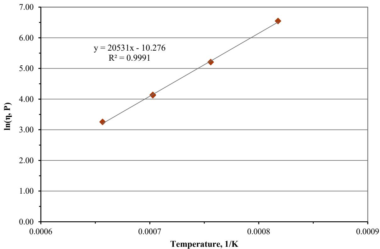
Figure C.12. Viscosity-Temperature Data and Arrhenius Equation Fit for Glass LP2-IL-12
