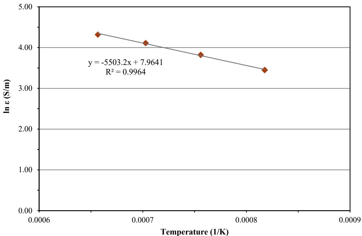
Figure D.20. Electrical Conductivity-Temperature Data and Arrhenius Equation Fit for Glass LP2-OL-03 MOD2
