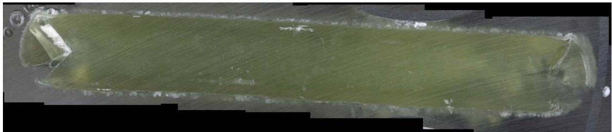
b) Glass cross section magnified after VHT
