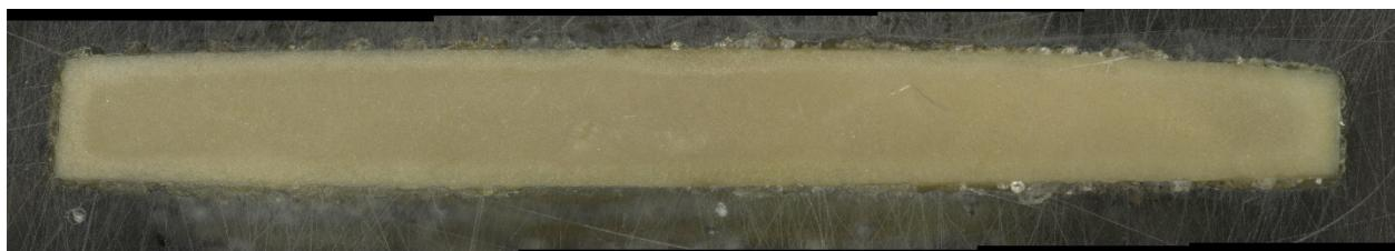
c) Glass cross section magnified after VHT
