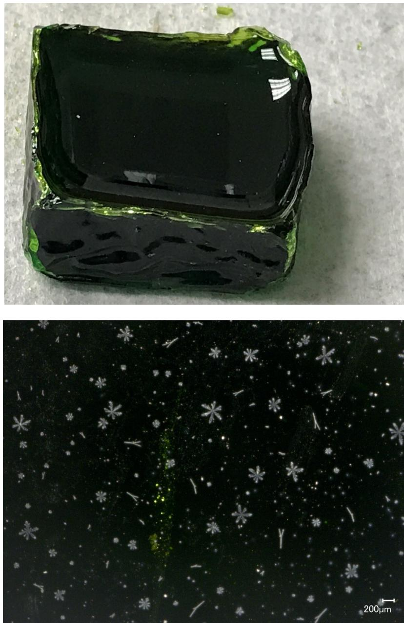
Figure G.13. Glass LP2-IL-13 after CCC Beginning at 1150°C both Glass (left) and Magnified 50X (right)
