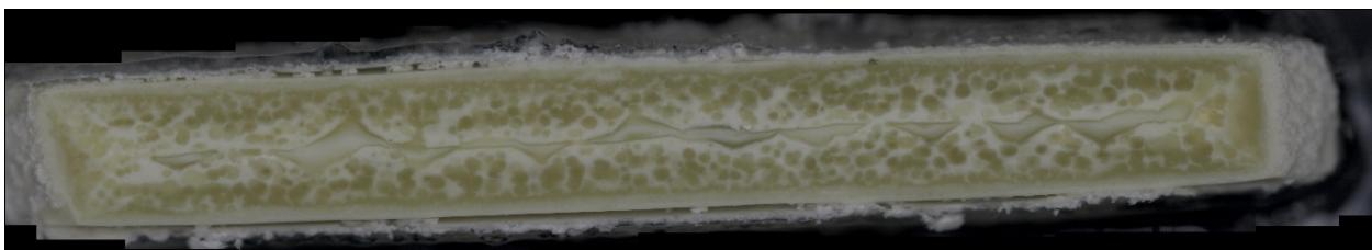
b) Glass cross section magnified after VHT
