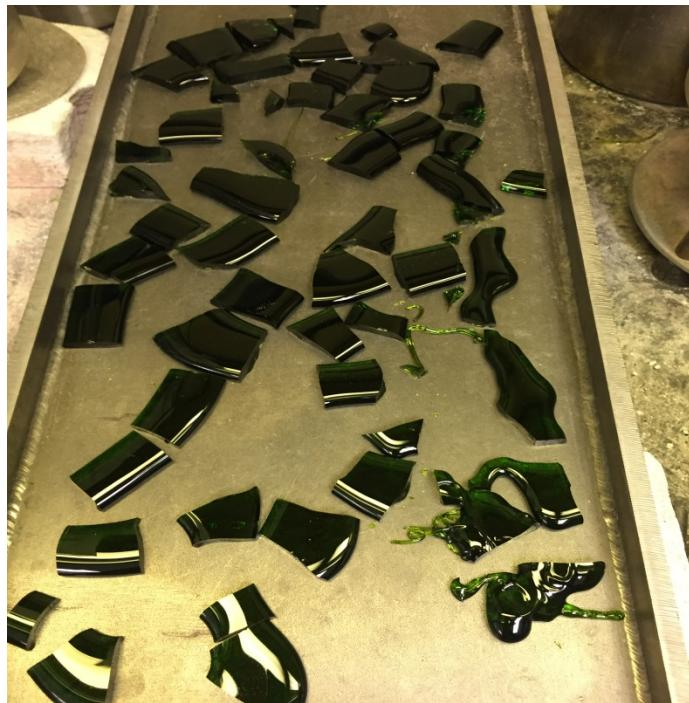
Figure A.25. Photo of Glass LP2-OL-09-1 Morphology of Second Melt at 1150°C for 1.5 h
