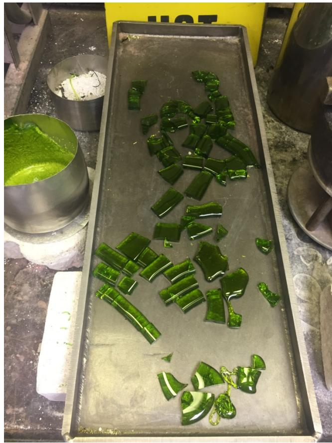
Figure A.36. Photo of Glass LP2-OL-20 Morphology of First Melt at 1150°C for 1.5 h
