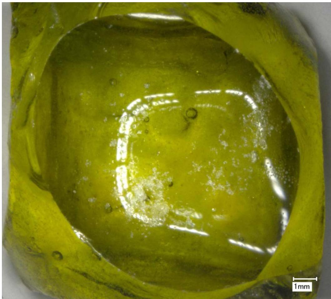
Figure E.40. Glass LP2-OL-25 after CF Heat Treatment at 950°C for 24 h
