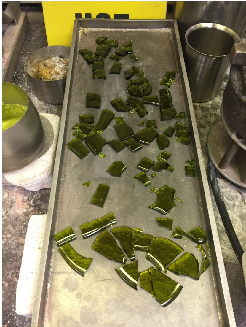
Figure A.41. Photo of Glass LP2-OL-25 Morphology of Second Melt at 1150°C for 1.6 h
