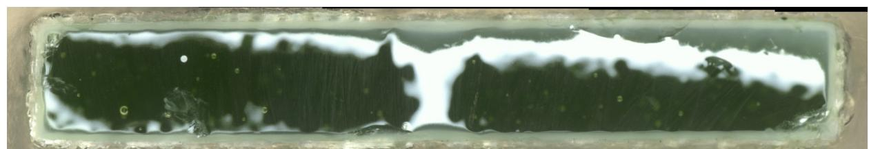
c) Glass cross section magnified after VHT
