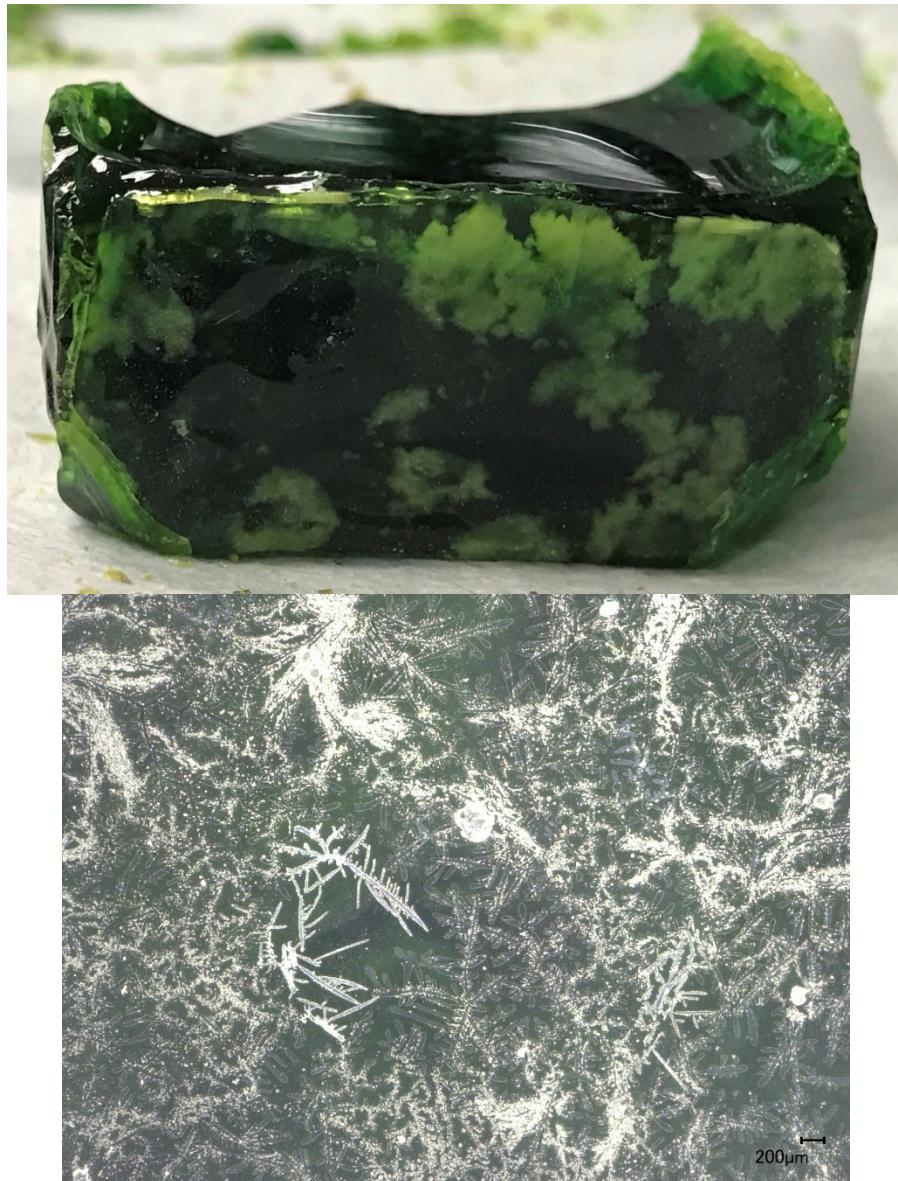
Figure G.1. Glass LP2-IL-01 after CCC Beginning at 1150°C both Glass (left) and Magnified 50X (right)
