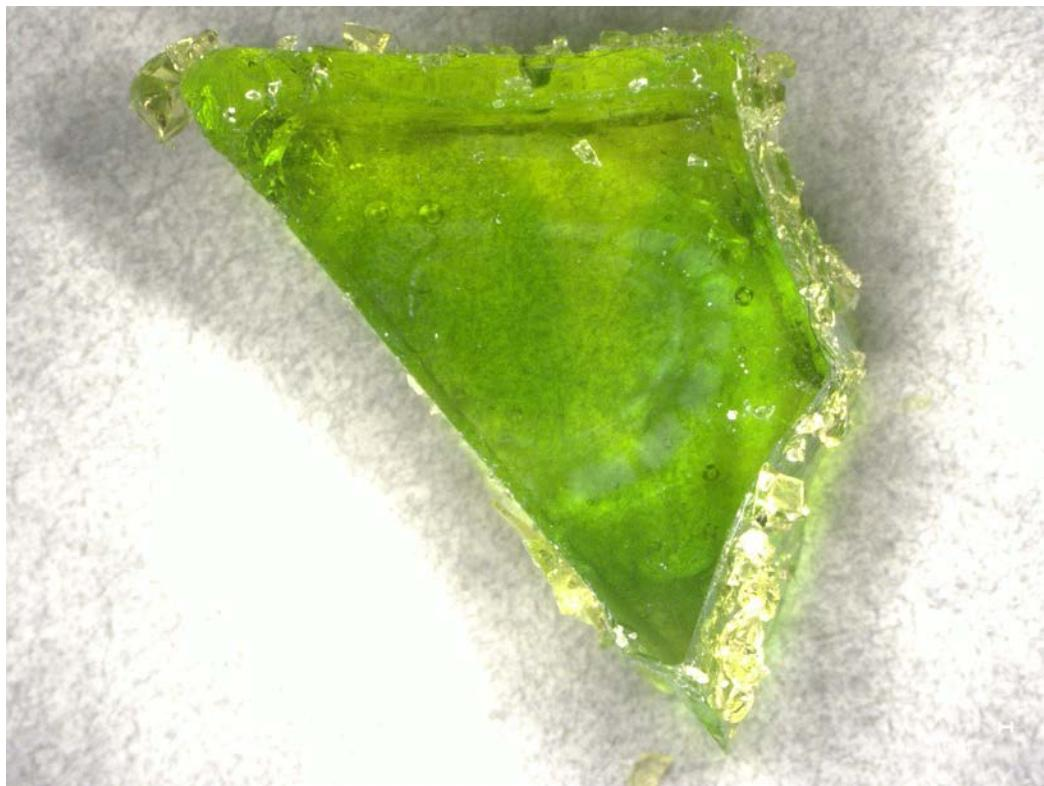
Figure E.6. Glass LP2-IL-07 after CF Heat Treatment at 950°C for 24 h Magnified 20X
