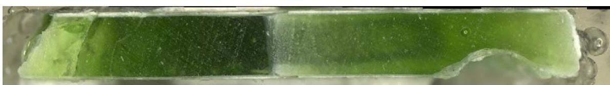
c) Glass cross section magnified after VHT
