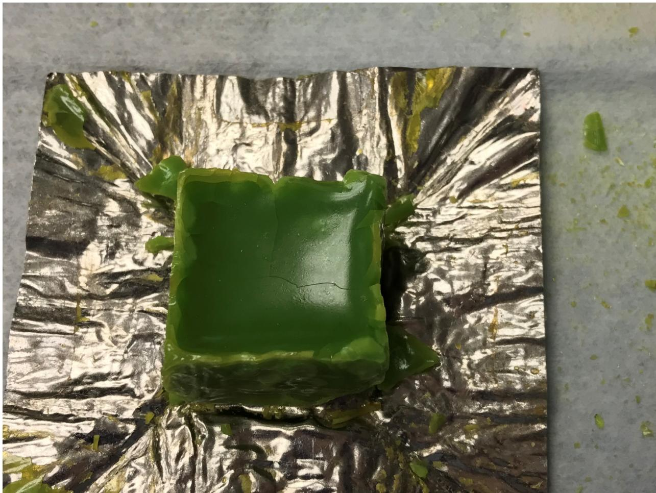
Figure G.34. Glass LP2-OL-18 after CCC Beginning at 1150°C
