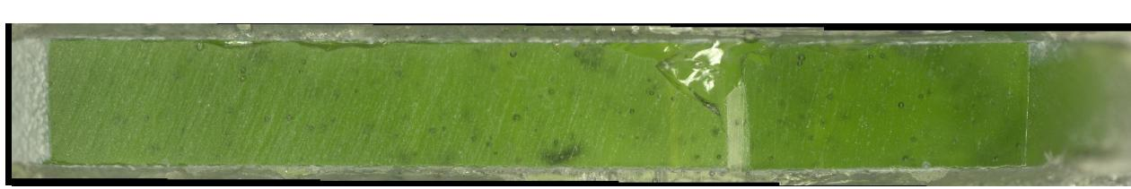
Figure I.5. Quenched Glass LP2-IL-04 after VHT for 7 Days
