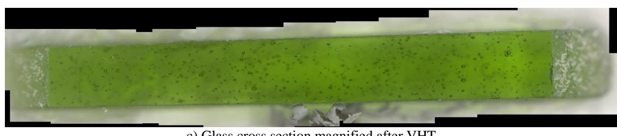
Figure I.25. Quenched Glass LP2-IL-15 after VHT for 24 Days
