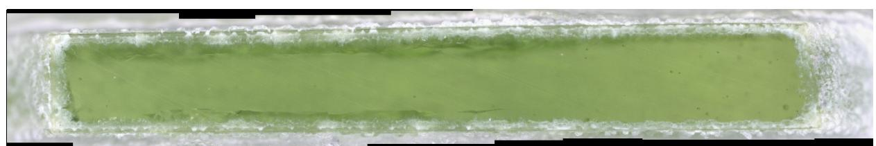
b) Glass cross section magnified after VHT
