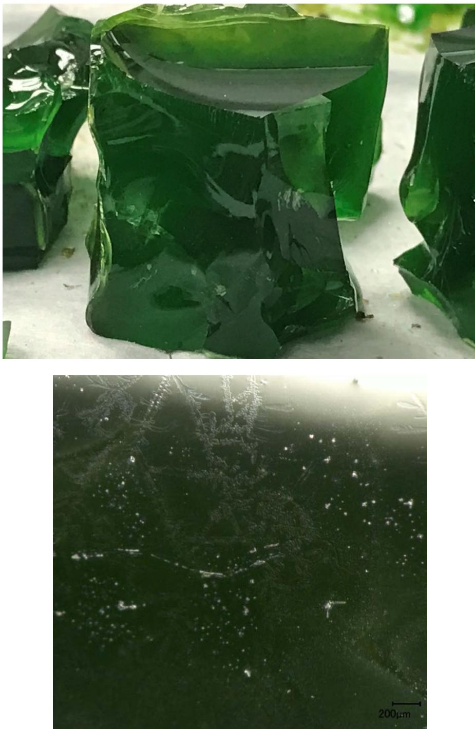
Figure G.2. Glass LP2-IL-02 after CCC Beginning at 1150°C both Glass (left) and Magnified 100X (right)
