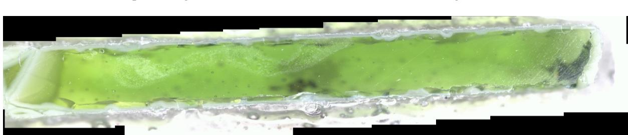
Figure I.91. ~~CCC~~-Treated Glass LP2-IL-15 after VHT for 24 Days
