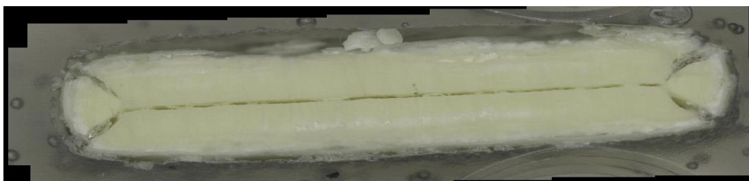
c) Glass cross section magnified after VHT
