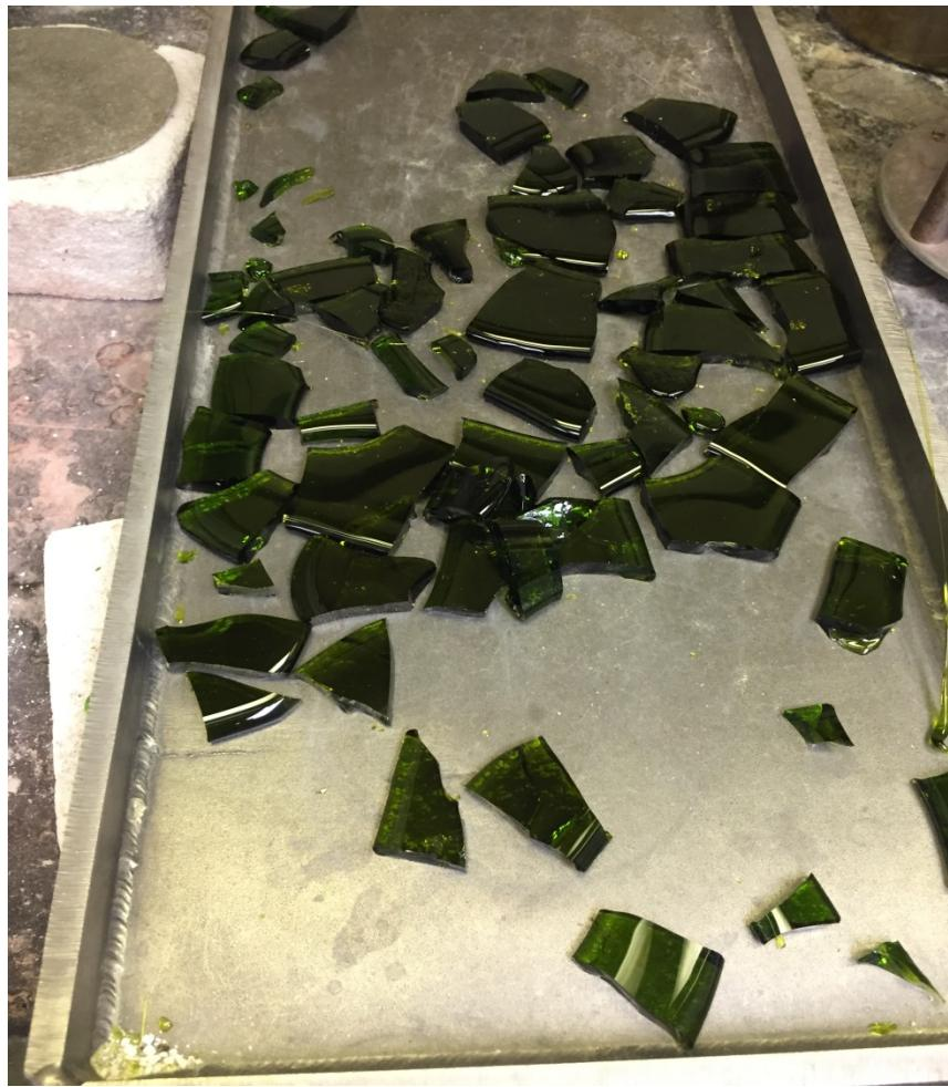
Figure A.28. Photo of Glass LP2-OL-12 Morphology of Second Melt at 1150°C for 1.5 h
