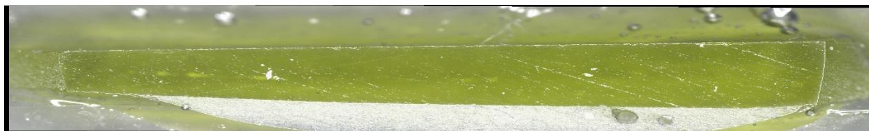
c) Glass cross section magnified after VHT
