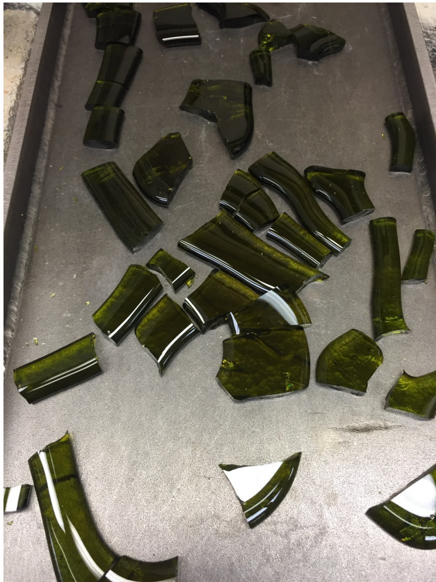
Figure A.40. Photo of Glass LP2-OL-24 Morphology of Third Melt at 1200°C for 1.5 h
