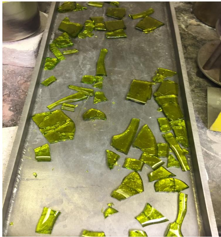
Figure A.29. Photo of Glass LP2-OL-13 of Morphology Third Melt at 1150°C for 1.7 h
