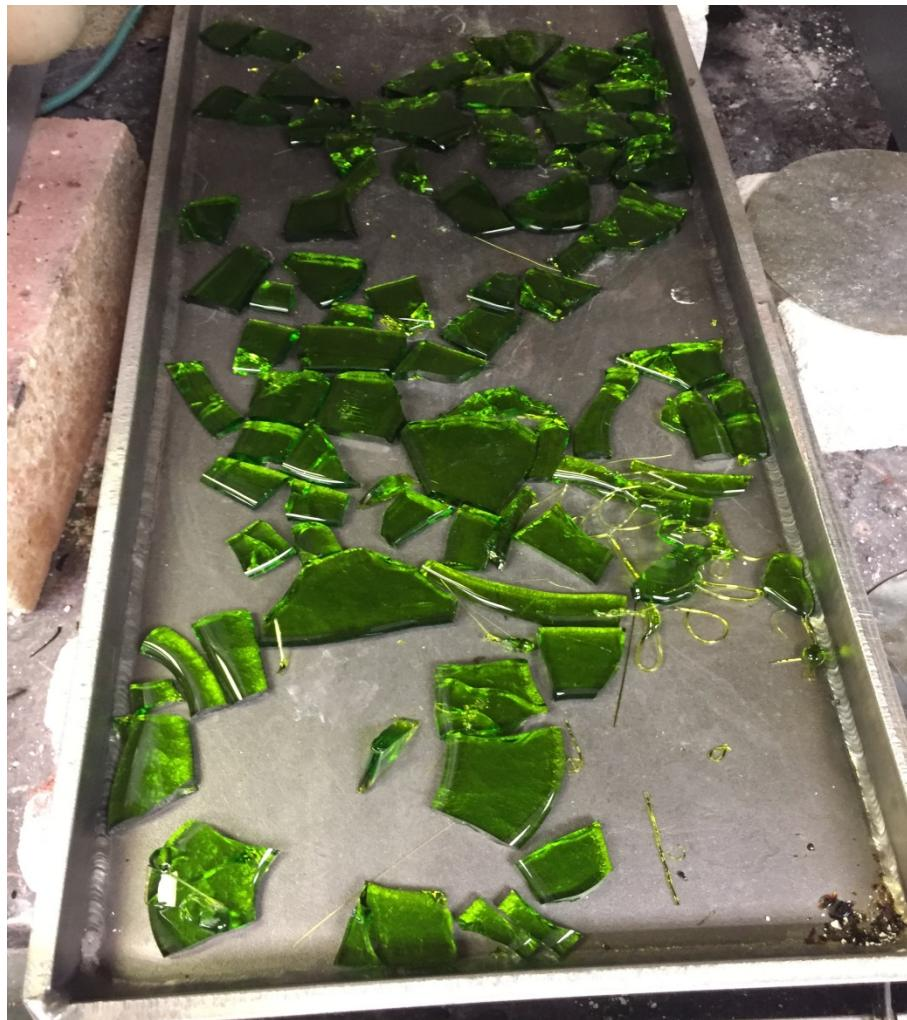
Figure A.30. Photo of Glass LP2-OL-14 Morphology of Second Melt at 1150°C for 1.5 h
