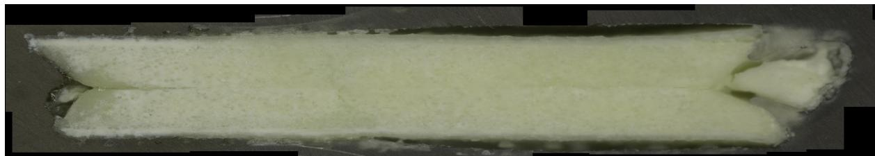
b) Glass cross section magnified after VHT
