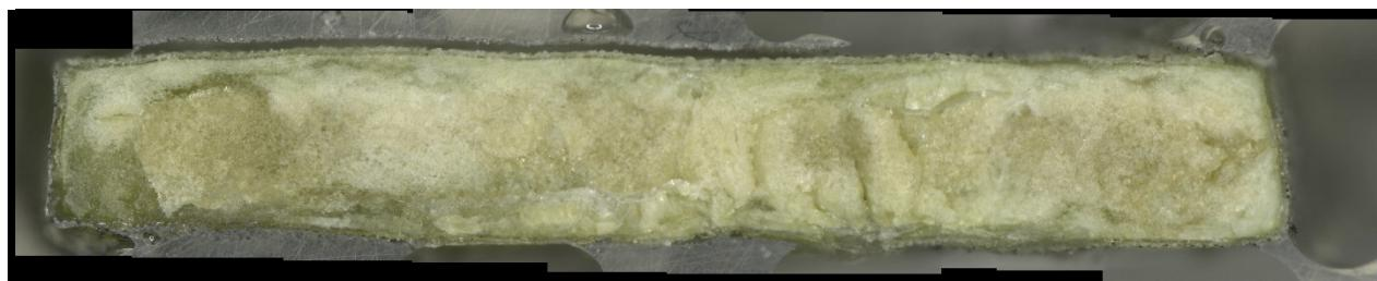
c) Glass cross section magnified after VHT
