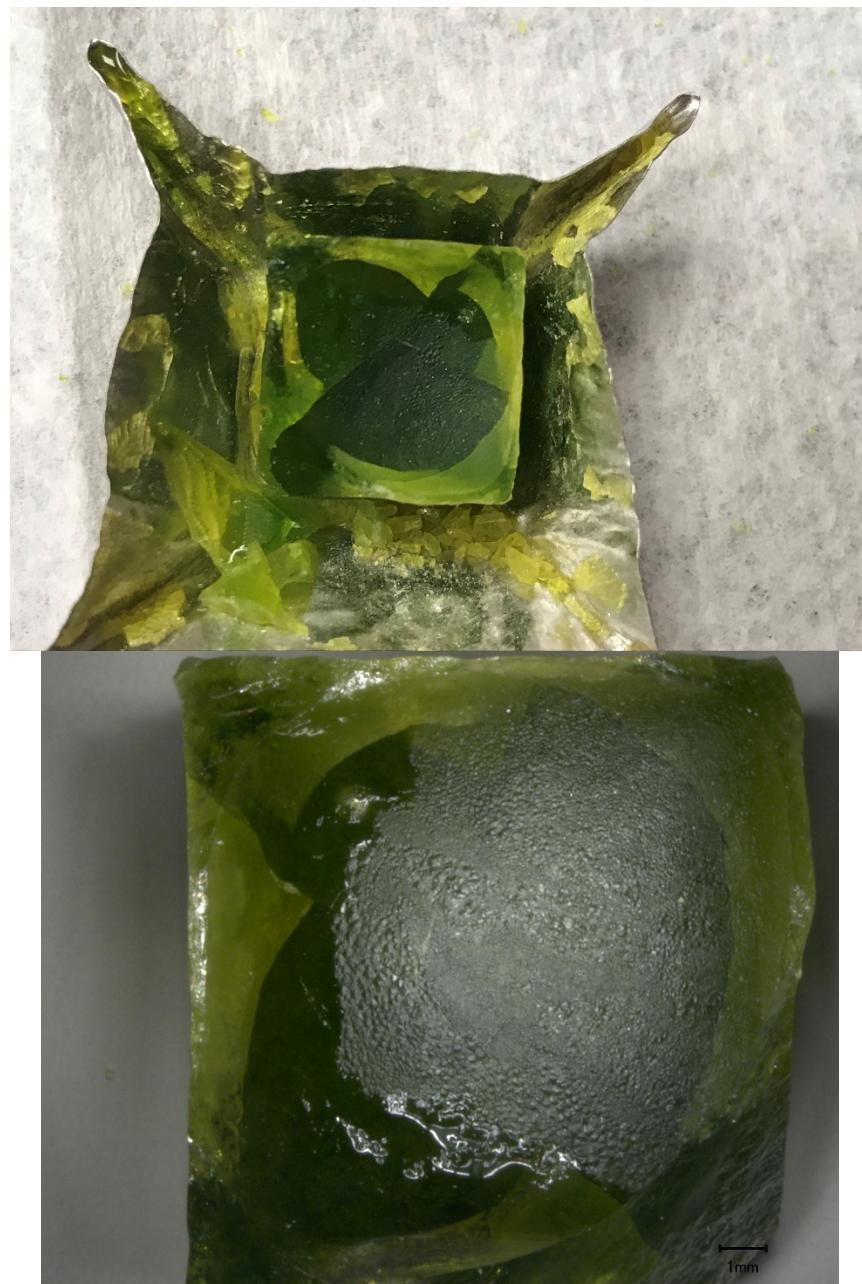
Figure E.21. Glass LP2-OL-05 after CF Heat Treatment at 950°C for 24 h both in crucible (left) and magnified 20X (right)
