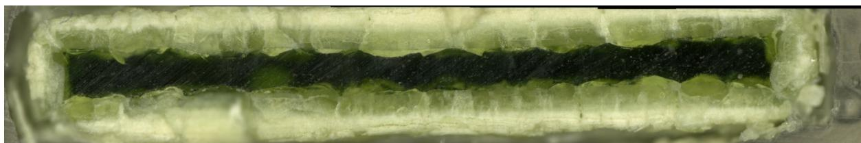
Figure I.4. Quenched Glass LP2-IL-03 after VHT for 7 Days
