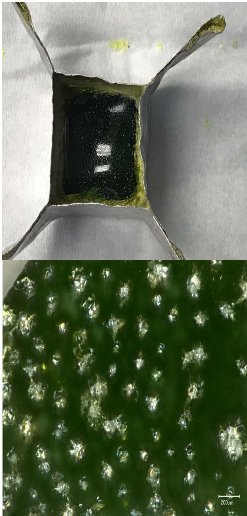
Figure E.7. Glass LP2-IL-08 after CF Heat Treatment at 950°C for 24 h both in Crucible (left) and Magnified 150X (right)
