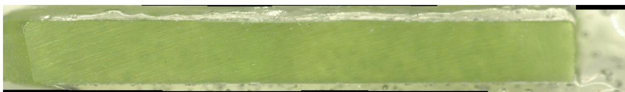
c) Glass cross section magnified after VHT
