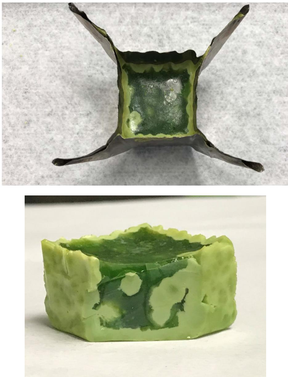
Figure G.22. Glass LP2-OL-05 after CCC Beginning at 1150°C both in Crucible (left) and Glass (right)
