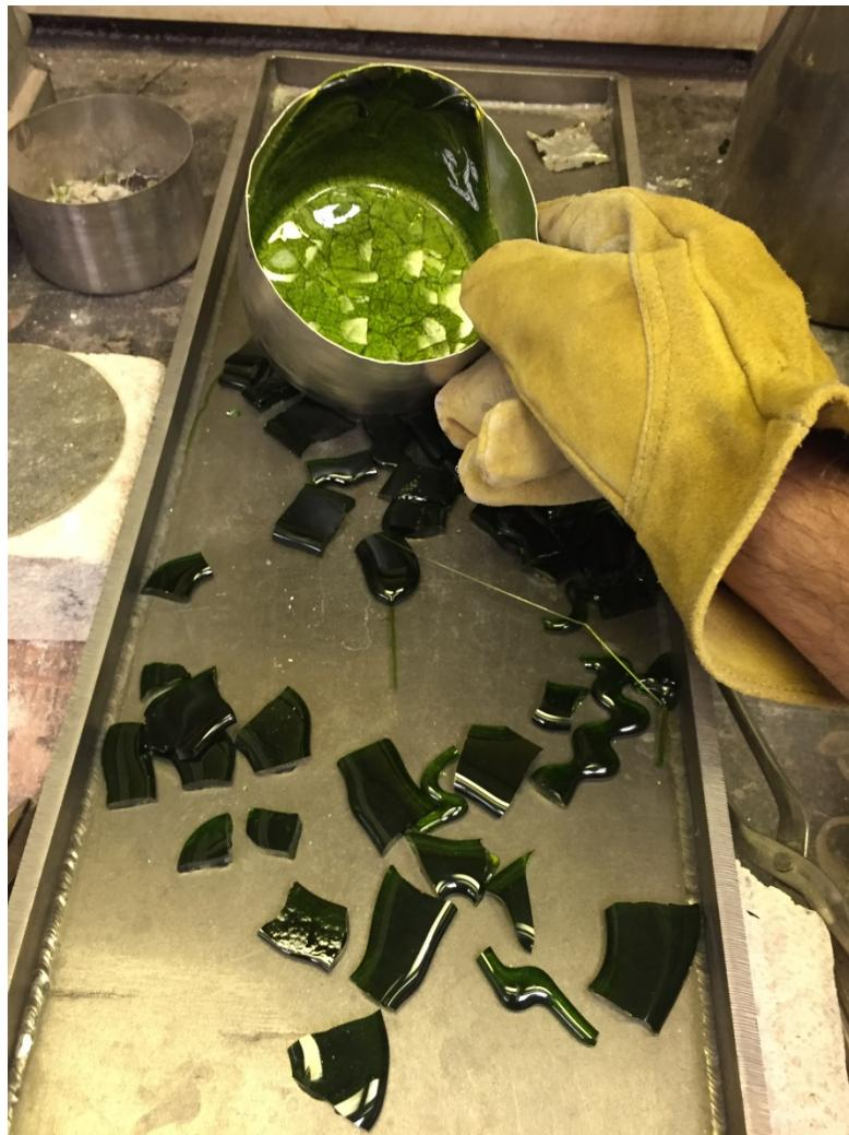
Figure A.22. Photo of Glass LP2-OL-05 Morphology of Third Melt at 1150°C for 1.5 h
