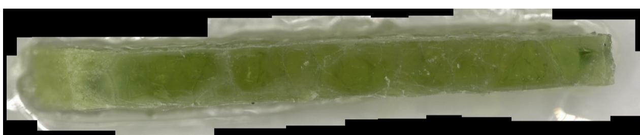
Figure I.12. Quenched Glass LP2-IL-08 after VHT after 24 Days
