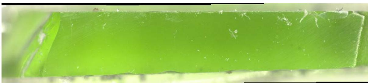
c) Glass cross section magnified after VHT
