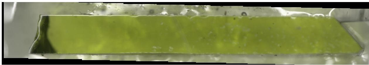
c) Glass cross section magnified after VHT
