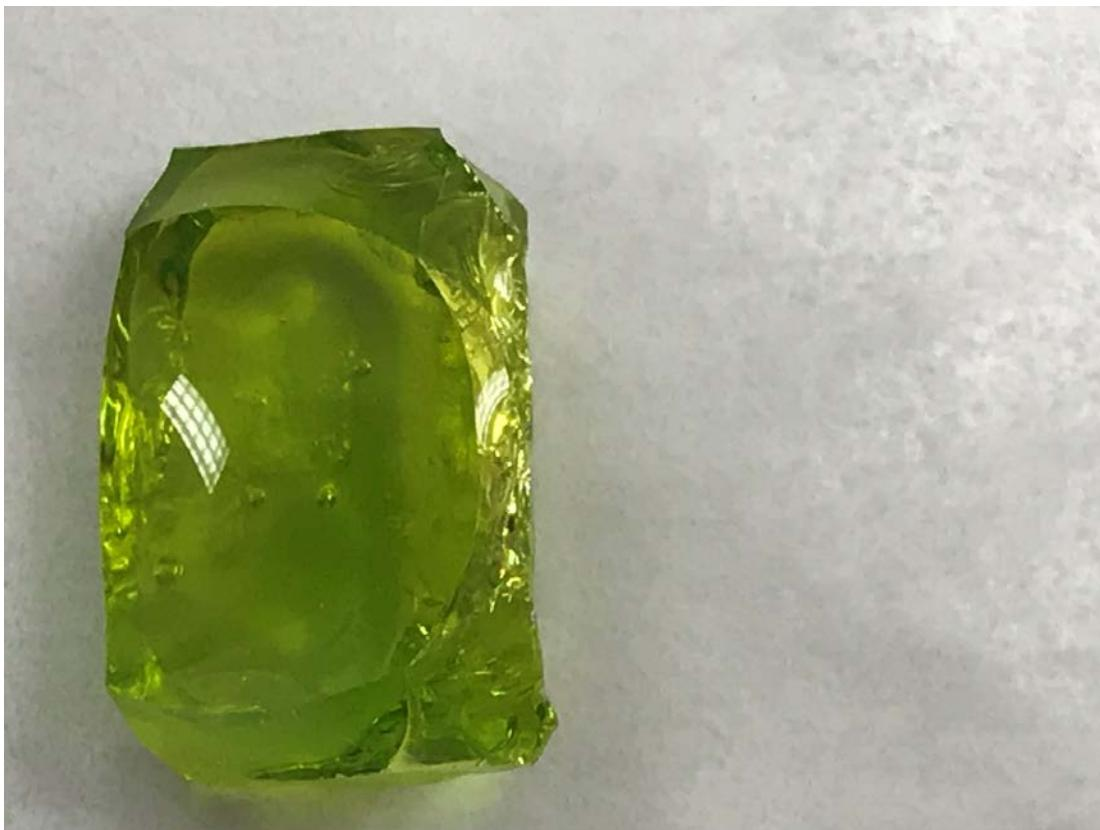
Figure E.29. Glass LP2-OL-14 after CF Heat Treatment at 950°C for 24 h
