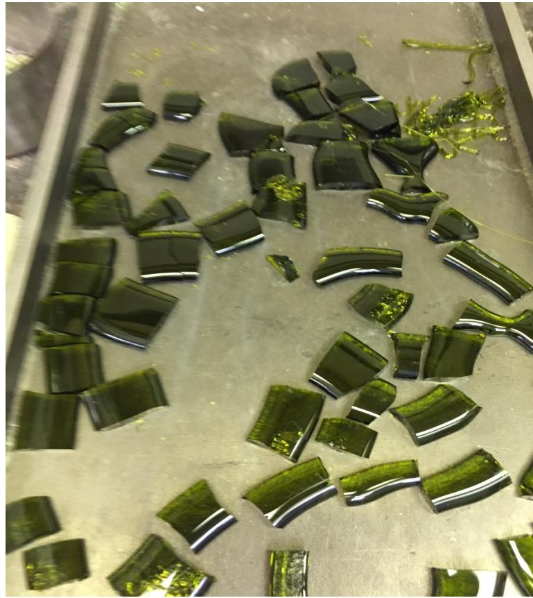
Figure A.21. Photo of Glass LP2-OL-04-1 Morphology of Second Melt at 1150°C for 1.5 h
