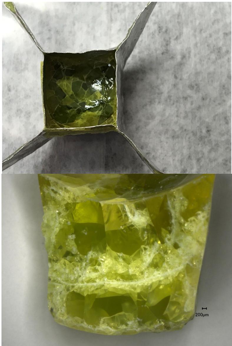
Figure E.20. Glass LP2-OL-04-1 after CF Heat Treatment at 950°C for 24 h both in Crucible (left) and Magnified 30X (right)
