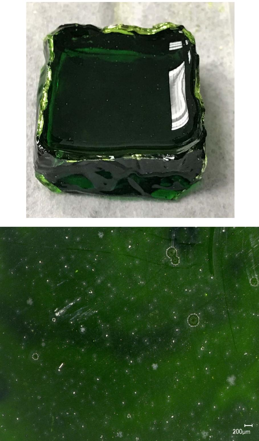
Figure G.12. Glass LP2-IL-12 after CCC Beginning at 1150°C both Glass (left) and Magnified 50X (right)
