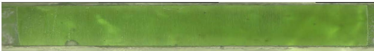
c) Glass cross section magnified after VHT
