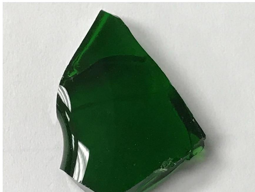
Figure A.10. Photo of Glass LP2-IL-10 Morphology of Third Melt at 1175°C for 1.5 h
