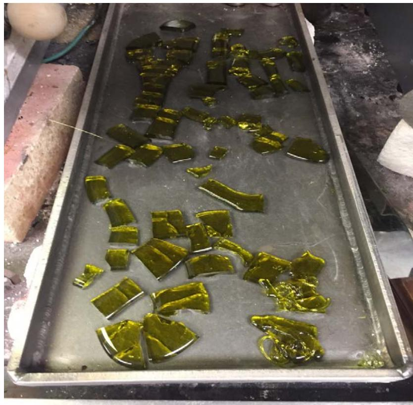
Figure A.33. Photo of Glass LP2-OL-17 Morphology of Second Melt at 1150°C for 1.5 h
