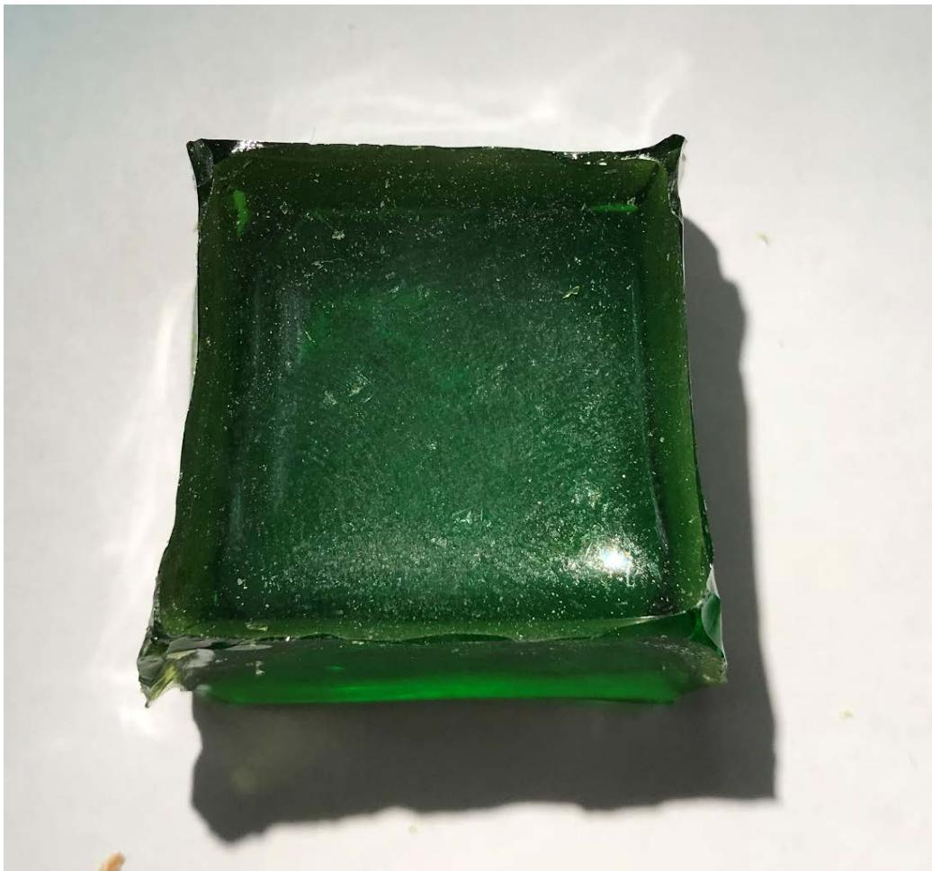
Figure G.39. Glass LP2-OL-23 after CCC Beginning at 1150°C
