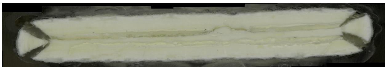
c) Glass cross section magnified after VHT
