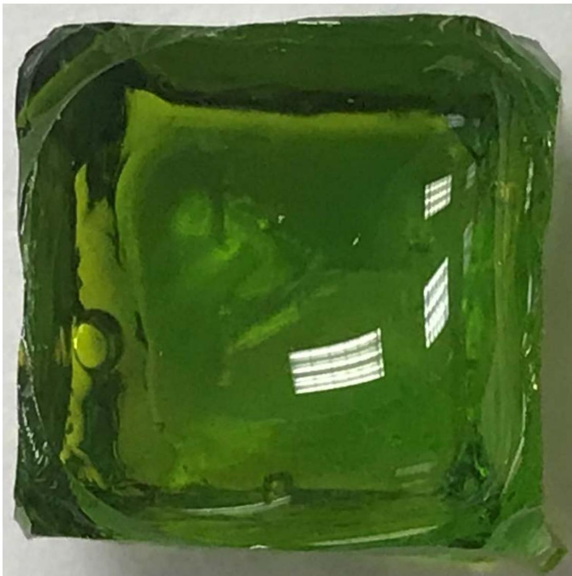
Figure E.36. Glass LP2-OL-21 after CF Heat Treatment at 950°C for 24 h
