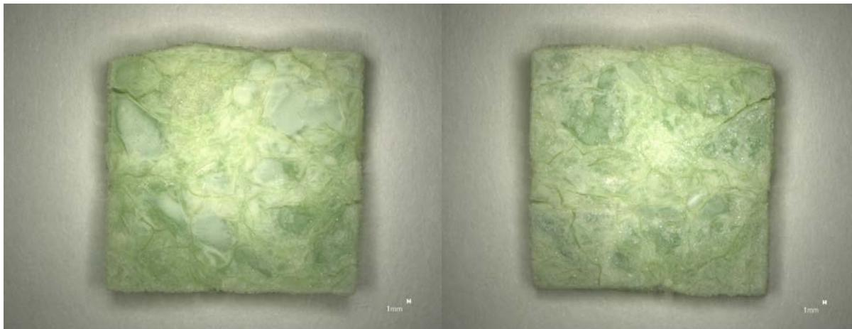
a) Glass square magnified after VHT; b) Glass square magnified after VHT
