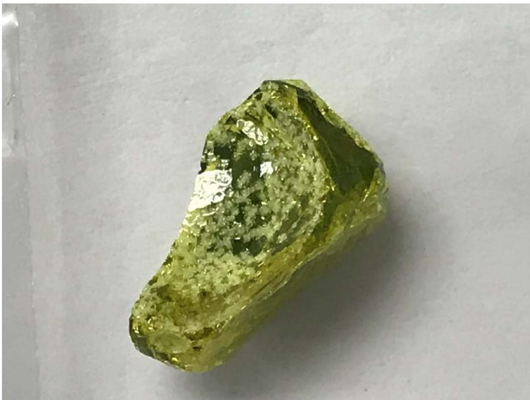
Figure E.37. Glass LP2-OL-22 after CF Heat Treatment at 950°C for 24 h
