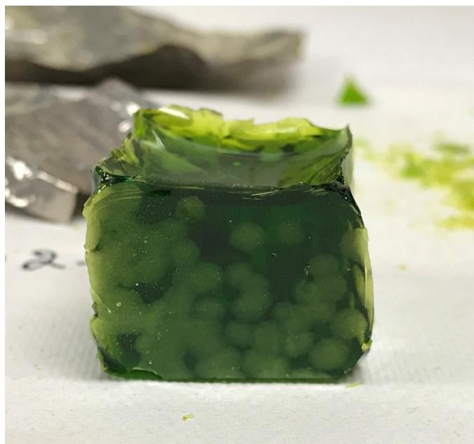
Figure G.19. Glass LP2-OL-02-1 after CCC Beginning at 1150°C both in Crucible (left) and Glass (right)
