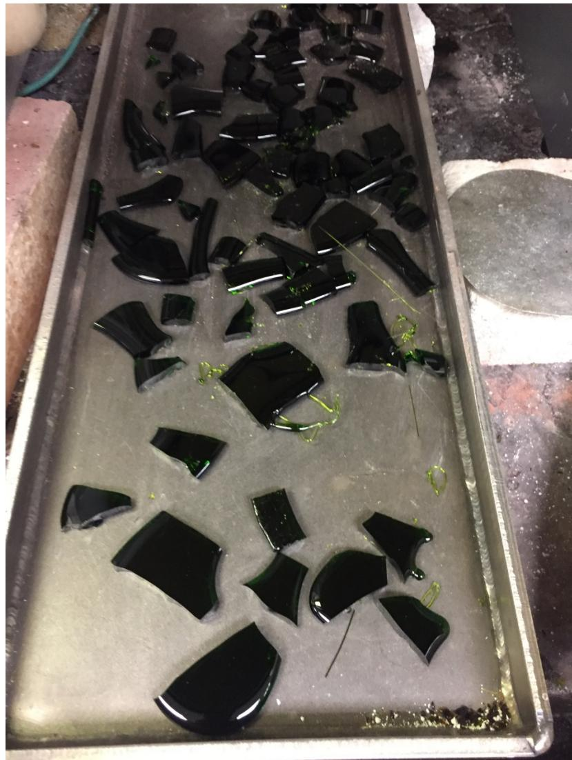
Figure A.31. Photo of Glass LP2-OL-15 Morphology of Third Melt at 1150°C for 1 h
