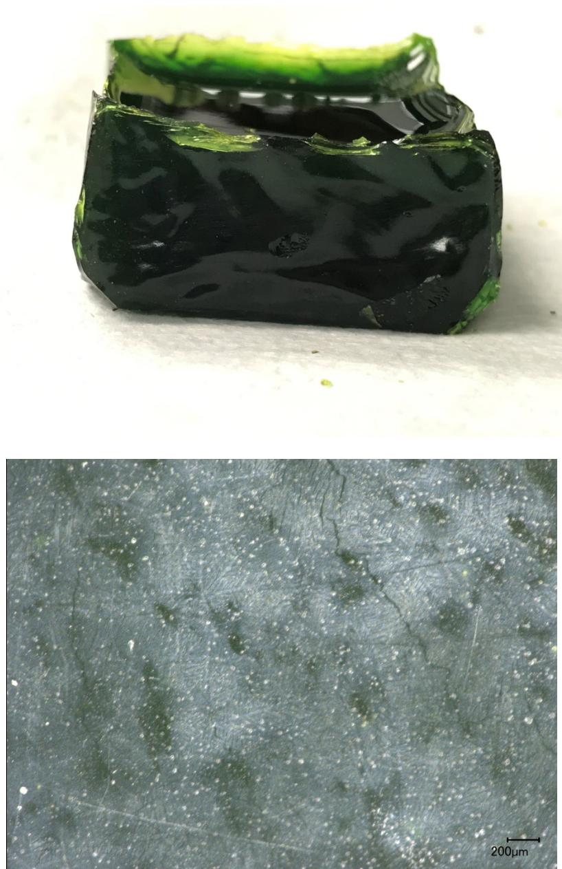
Figure G.3. Glass LP2-IL-03 after CCC Beginning at 1150°C both Glass (left) and Magnified 100X (right)
