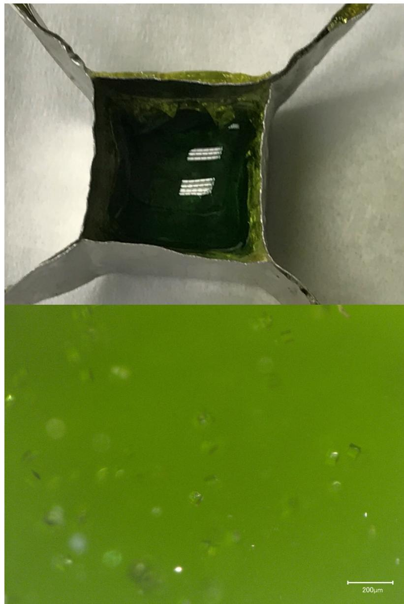
Figure E.10. Glass LP2-IL-11 after CF Heat Treatment at 950°C for 24 h both in Crucible (left) and Magnified 200X (right)
