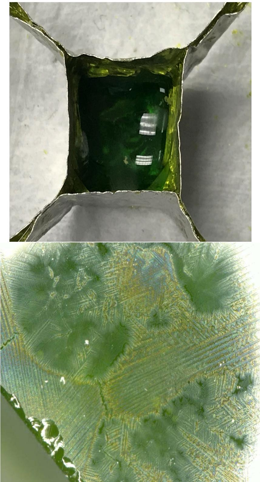
Figure E.5. Glass LP2-IL-06 after CF Heat Treatment at 950°C for 24 h both in Crucible (left) and Magnified 100X (right)
