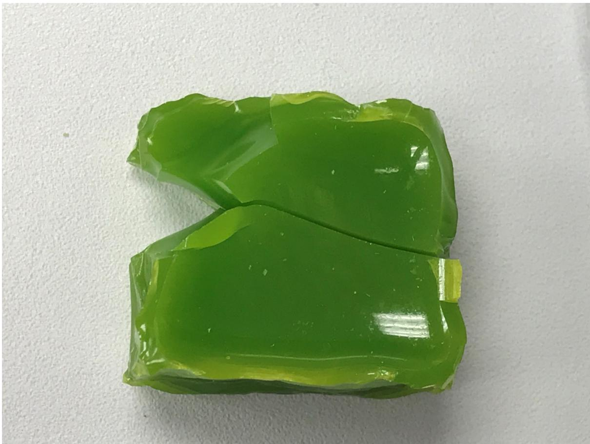
Figure G.30. Glass LP2-OL-14 after CCC Beginning at 1150°C
