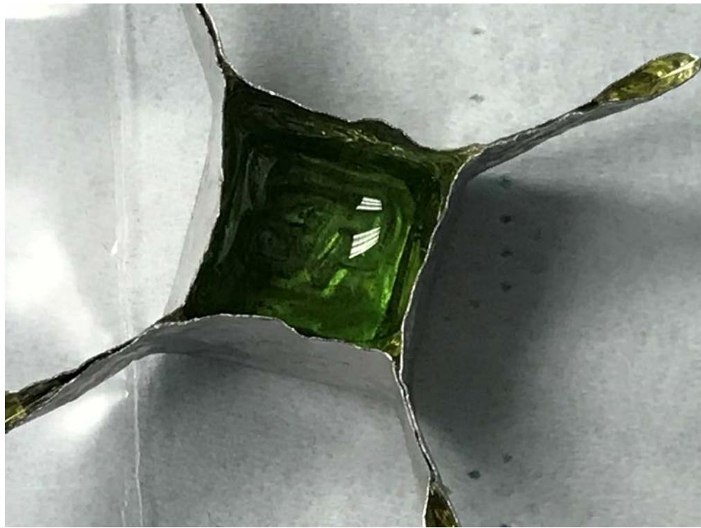
Figure E.16. Glass LP2-IL-17 after CF Heat Treatment at 950°C for 24 h
