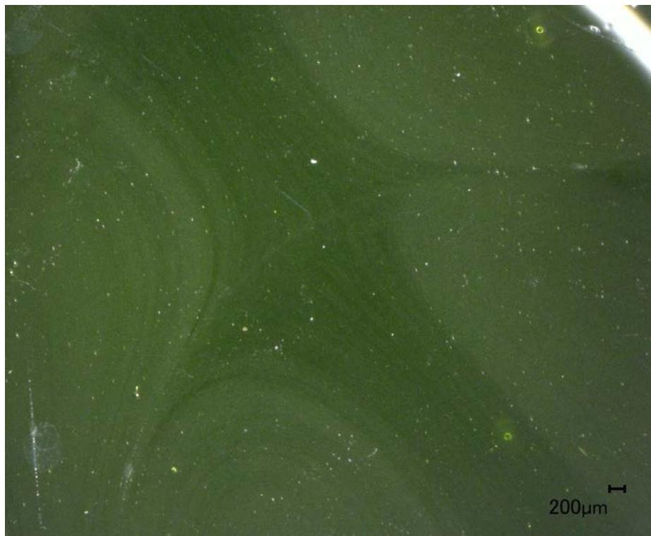
Figure A.8. Photo of Glass LP2-IL-08 Morphology of Third Melt at 1175°C for 1.1 h
