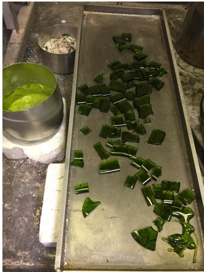
Figure A.37. Photo of Glass LP2-OL-21 Morphology of Second Melt at 1150°C for 1.4 h
