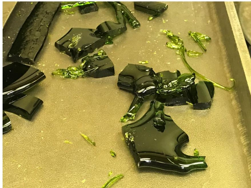
Figure A.32. Photo of Glass LP2-OL-16 MOD of Third Melt at 1200°C for 2 h
