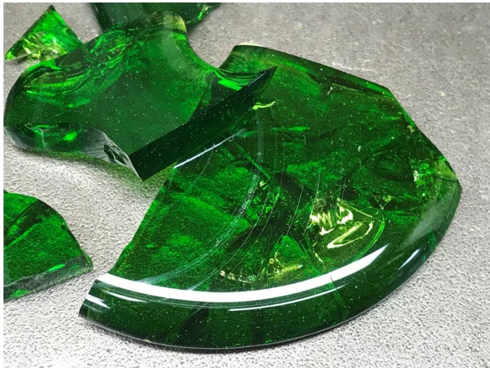
Figure 2.2. Glass LP2-OL-03 First Modified Composition after First Melt
