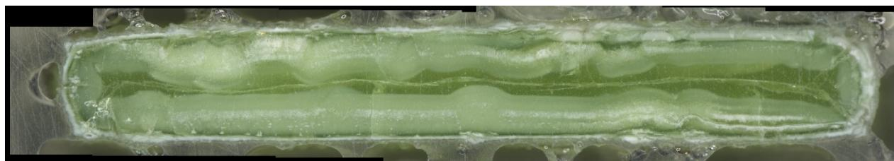
c) Glass cross section magnified after VHT
