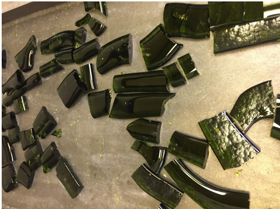
Figure A.23. Photo of Glass LP2-OL-07-1 Morphology of Second Melt at 1150°C for 1.5 h
