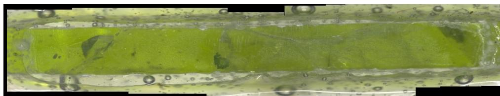
b) Glass cross section magnified after VHT
