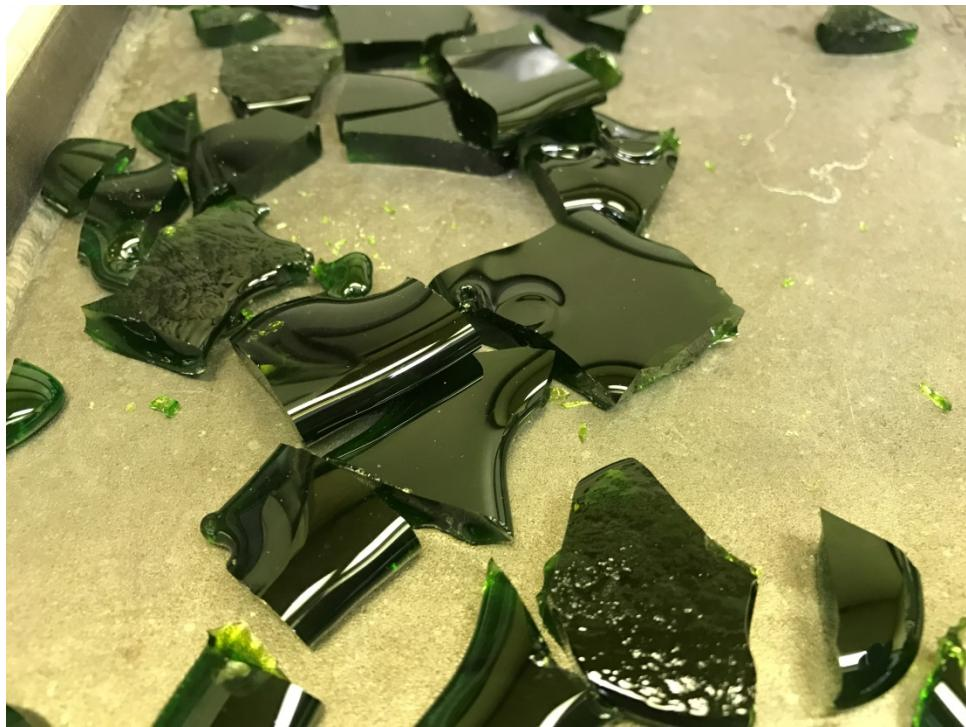
Figure A.6. Photo of Glass LP2-IL-06 Morphology of Fourth Melt at 1175°C for 1 h
