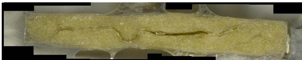
c) Glass cross section magnified after VHT
