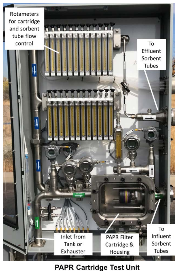
Figure 5. Photograph of the CT Rig
