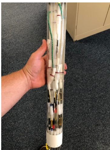
Figure 7. Photograph of a Routine HS Tube Bundle
