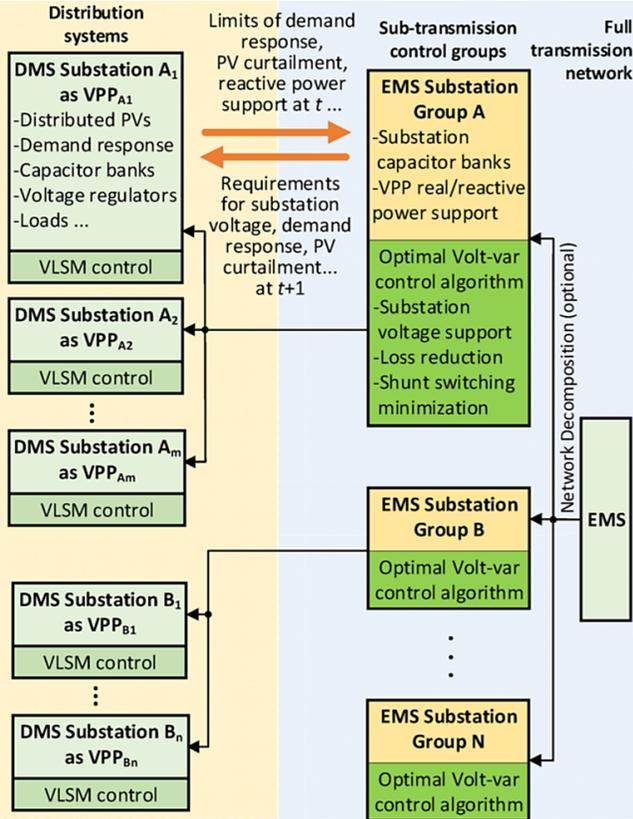
Operation of systems such as CReST-VCT depends on the communication network between the various elements. Successful real-time operation will depend on the ability of the algorithm to complete necessary analysis and the ability of the communication system to transfer data reliably and within necessary time constraints.
