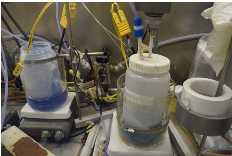
Figure 3 Experimental Set Up for a Reverse Strike Experiment (Run 16 Shown)
