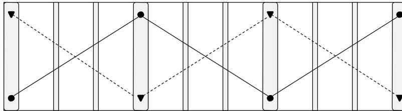
**Figure 2.2.** Front View Schematic of Hydrophone Deployments at Three Turbines Showing the Double-Detection Arrays. The circles denote the hydrophones of Array 1 and the triangles denote the hydrophones of Array 2.
