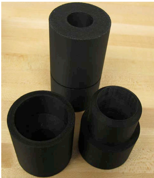
Figure 6: The jig used to center the beta cell on the PMT window for the gluing process. A weight is then placed on top of the jig to provide uniform pressure during the gluing process.
