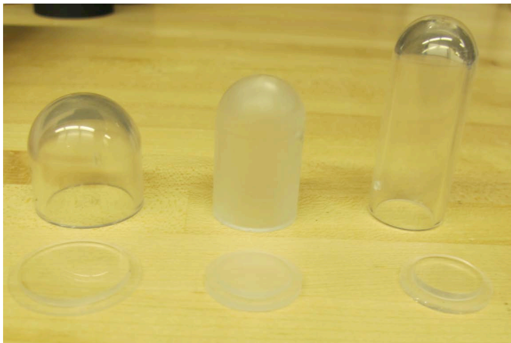
Figure 5: The dome and end-cap portions of the 6cc-wide (left), diffuse (center), and 6cc-long (right) cells. The end-cap is a top-hat design for a more secure connection.
