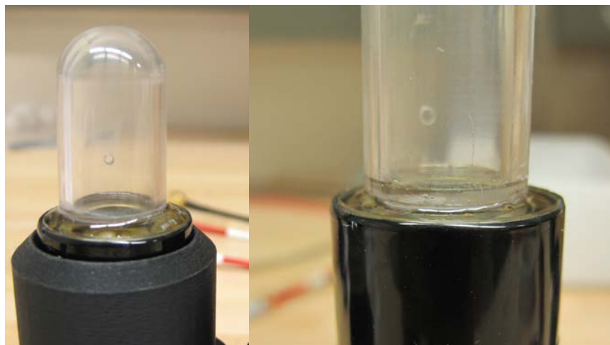
Figure 15: Cell used in the tests before (left) and after (right) the cell was removed and recemented.
