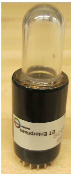
Figure 7: Completed 4cc cell glued to a 1-inch PMT.
