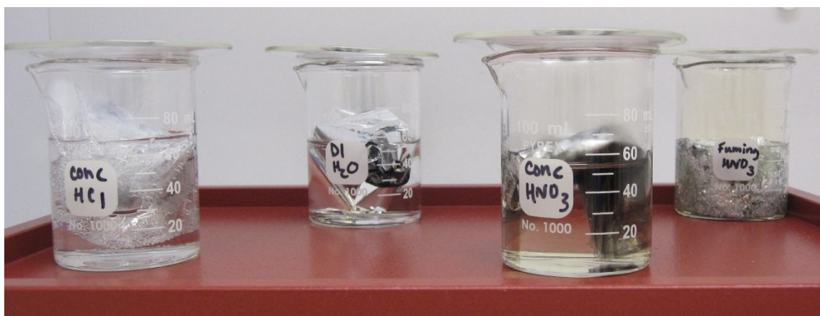
Figure A.3. Mylar Samples in Reagents after Heating at 150°C for 5 minutes
