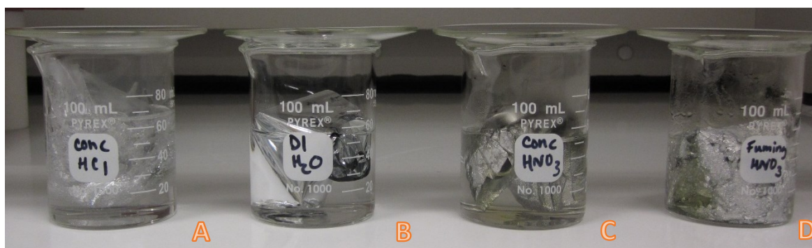
Figure A.2. Mylar Samples in Reagents after 1 Hour at Room Temperature
