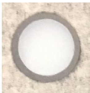
Figure 3. A silicon wafer coated with the zeolite sorbent thin film.
