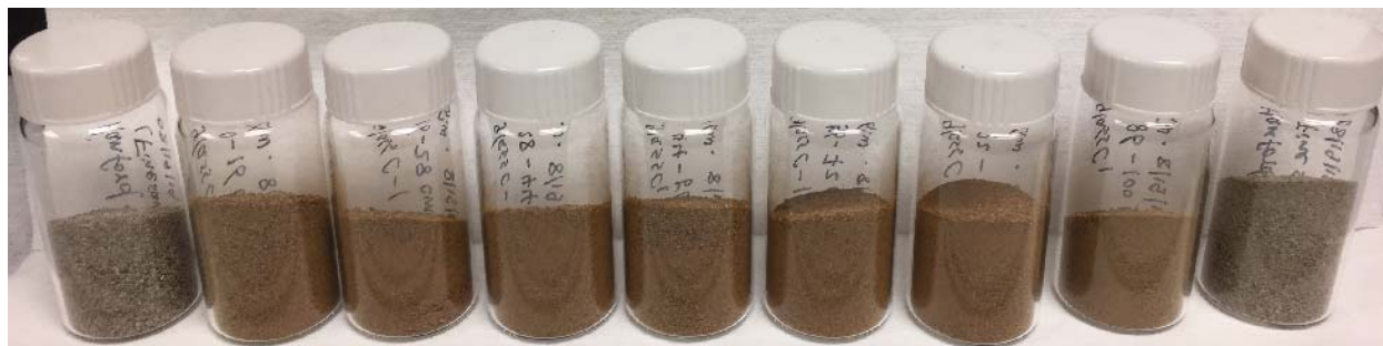
Figure 5.21. Color comparison between treated (brown) and untreated (gray) HF sediments. The seven brownish samples located in the middle are the reacted sediments from column 1mG-1 after in-situ HFO precipitation, which, from left to right, represented the samples collected following the column flow direction (0 to 100 cm); the two grayish samples at far left and right are the untreated HF sediments.
