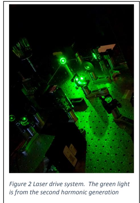
Figure 2 Laser drive system. The green light is from the second harmonic generation
