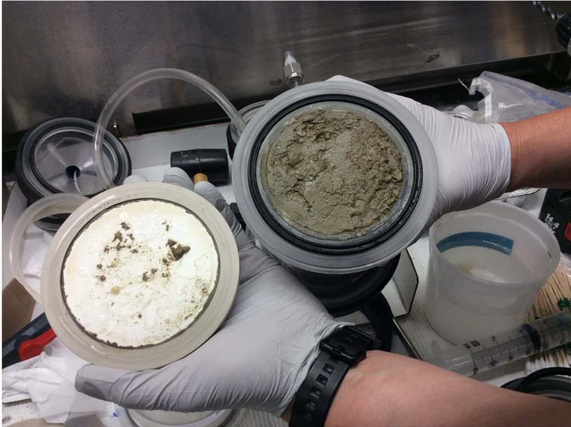
Figure 29. Photograph of the bottom of core B355M0, with end cap removed, after termination of the multistep outflow experiment.
