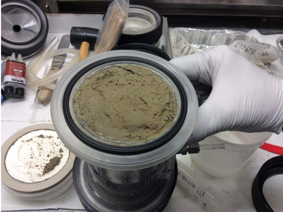
Figure 30. Photograph of the top of core B355M1, with end cap removed, after termination of the multistep outflow experiment.
