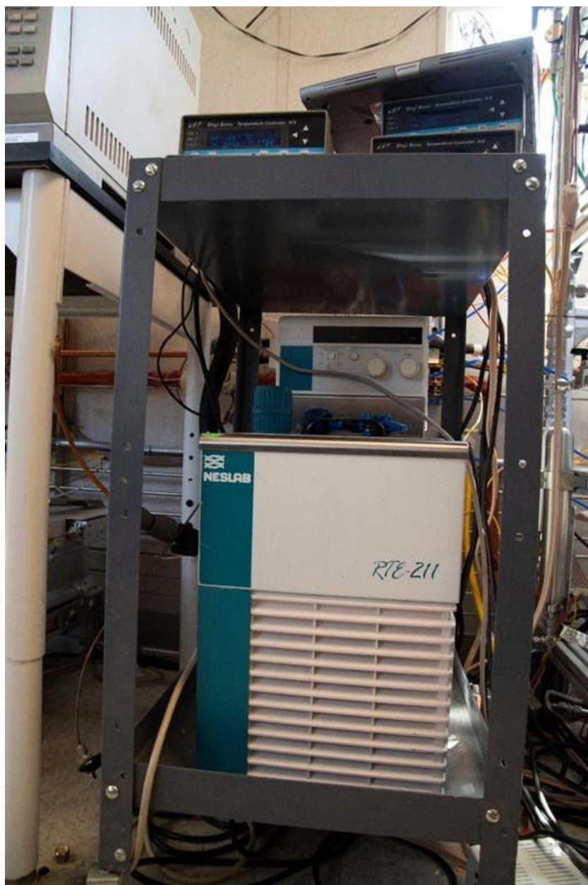
Figure B.5. The NESLAB RTE-211 was used to cool key sample lines as part of potential temperature controls along the exhaust sampling lines. It was used during shakedown and it was determined not to be necessary in later testing. The heat tape controllers on the top of the cart are part of the seven to ten tapes (depending on the test) that were operated at 120°C to 200°C during testing. They were on the primary analytical sample loop tubes and lines (as well as the intake sample lines) to limit moisture condensation as the exhaust cooled coming from the NUCON VAU. The orange insulation over the heat tape on the sampling header can be seen on the back wall.
