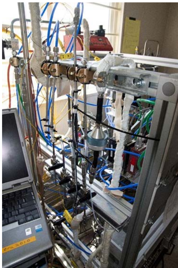
Figure B.19. The north side of the gas control rack included the sorption tube sample collection system.
