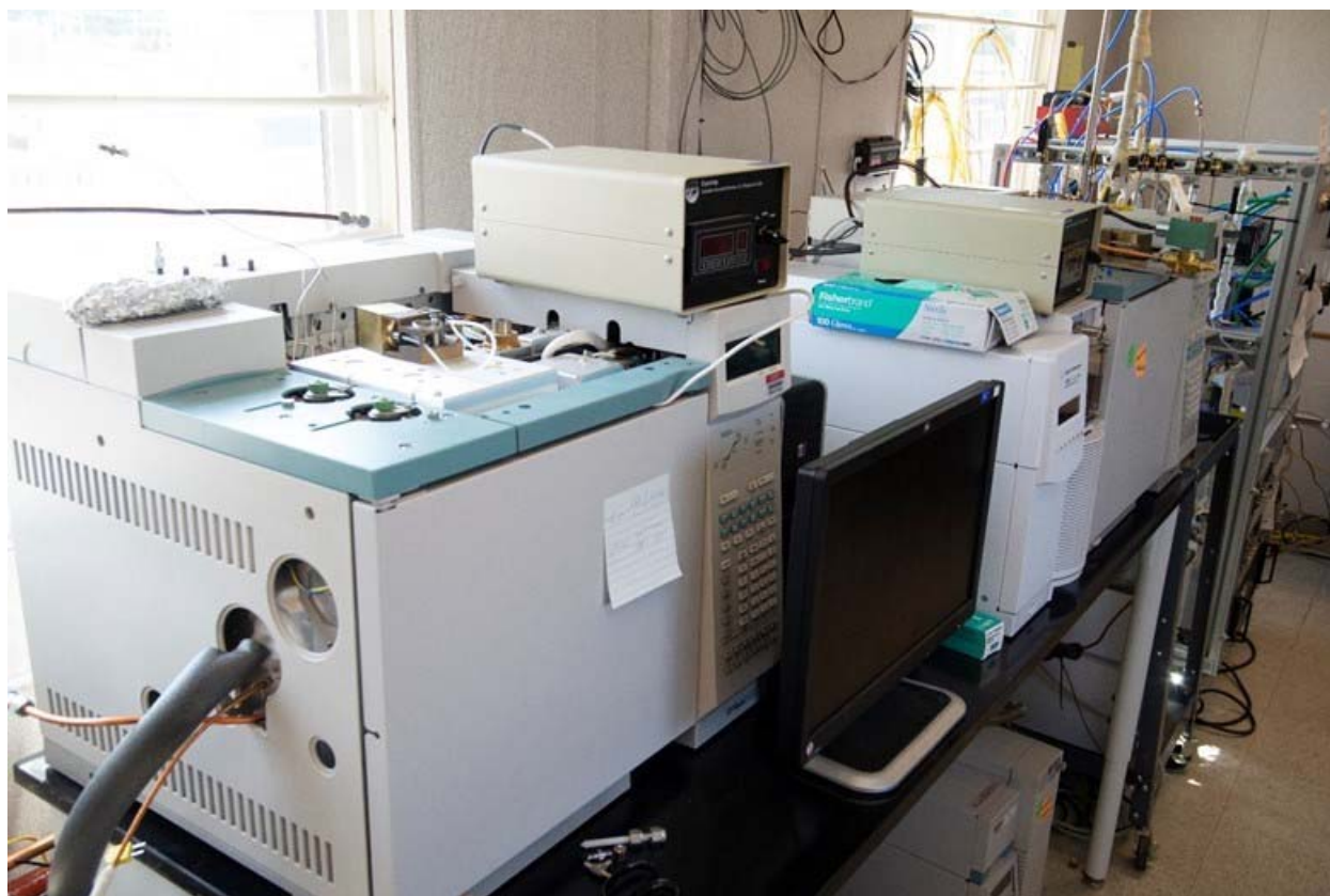
Figure B.4. The Agilent 6890N Gas Chromatograph set up as a pre-concentrator (left) for the PTR-MS. The second unit is the Agilent 6890N Gas Chromatograph with an Agilent 5973 Mass Selective Detector (right). Neither device was needed to support final testing.
