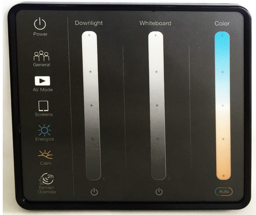
Figure 3. The Finelite LED lighting system control interface.
