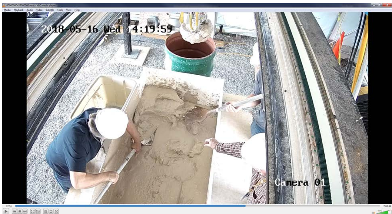
Figure TS31 – Removing simulant shelf in Simulant tank – Load 1
