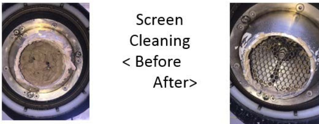
Figure 5.18. HWEE Screen Cleaning Demonstration of Kaolin Clay with 500 psi Internal Flush
