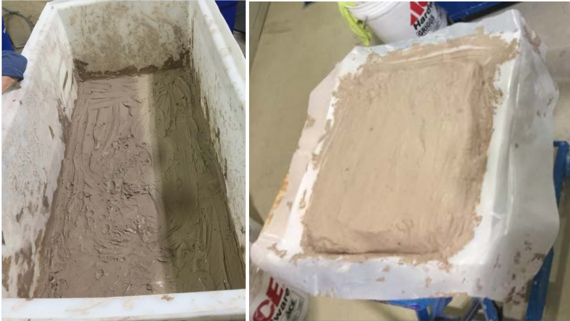
Figure 5.7. Layered Waste Profile (PNNL Layer Build—Thickness in Sections)
