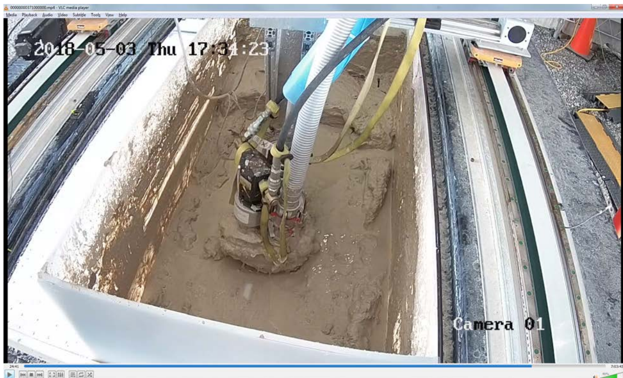
Figure LS33 - Pass 9 - Suction Clean – No flushing - Leg 3 – HWEE dragging along bottom of tank. See exposed tank bottom where scrapping occurred.
