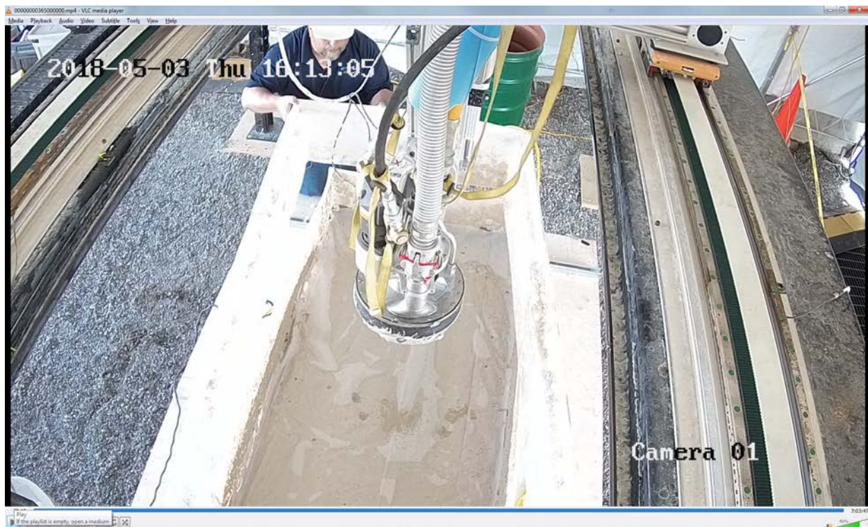
Figure LS6 - Simulant Tank Top Removal – Cut off 11 inches – Required to reduce interference from gantry/scanner moving down vertically to continue retrieval mining.
