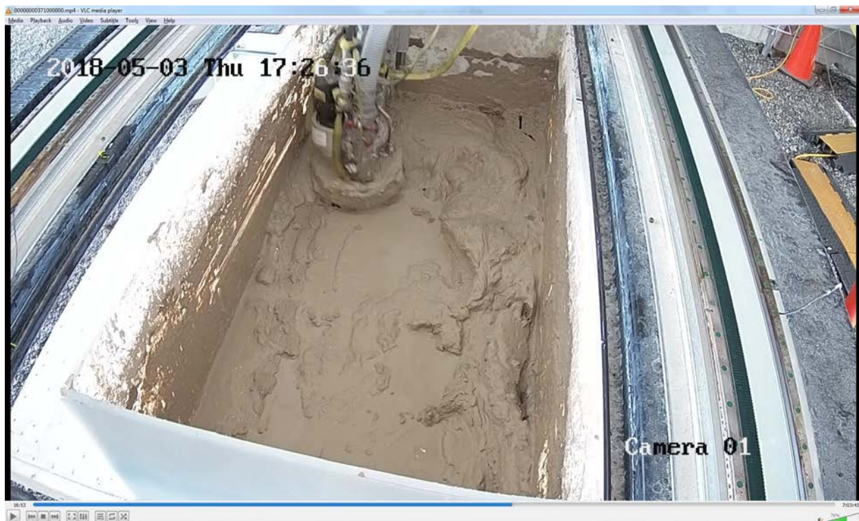
Figure LS29 - Pass 9 (Rerun) – Leg 1 – End - Tank lifting slightly again when simulant sludge at far end is impacted by HWEE.
