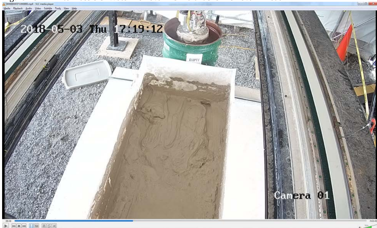
Figure LS23 - Setting HWEE pressure in Capture Tank prior to Pass 9. This operation is required whenever the high pressure pump has been shut down to set pressure of the HWEE rotating jet to 1,000 psi operating pressure (set with pressure reducing station gauge) for this kaolin simulant retrieval operation. Flush pressure is not set, only HWEE rotating jets with the HWEE jet pump operating
