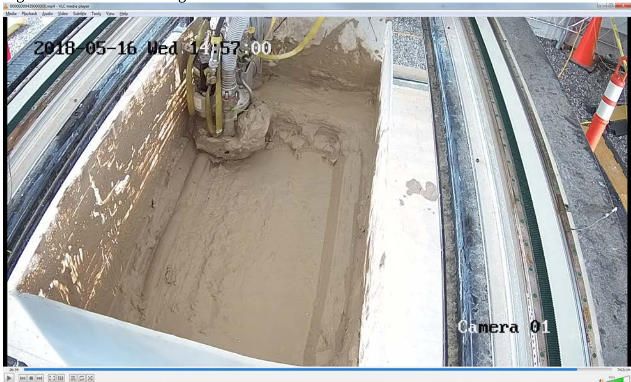
Figure TS68– Pass 13 – Leg 1 – End – Suction Clean – Flushing during Y-axis jogs.
