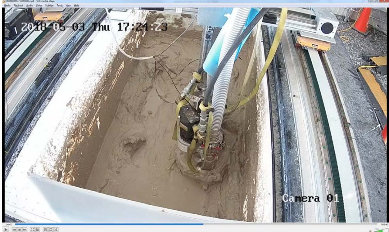
Figure LS28 - Pass 9 – Leg 5 - Stopped at this point (about ¼ into run length) - Test stopped because test personnel thought the HWEE was not rotating in error. After looking at data, HWEE rotation was operating properly and test did not need to be stopped. After test was stopped at this point, it was decided to rerun this Pass 9.
