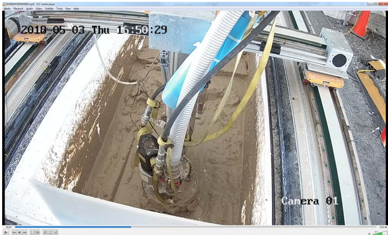
Figure LS20 - After Pass 8 – Water in simulant clean up using HWEE suction – End of suction
