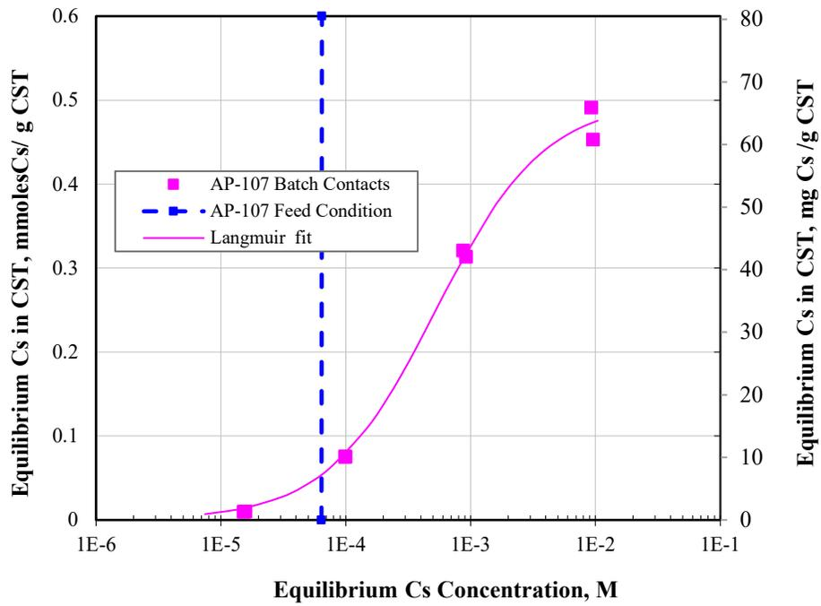
**Figure 3.3.** Isotherm for AP-107 Tank Waste with CST
