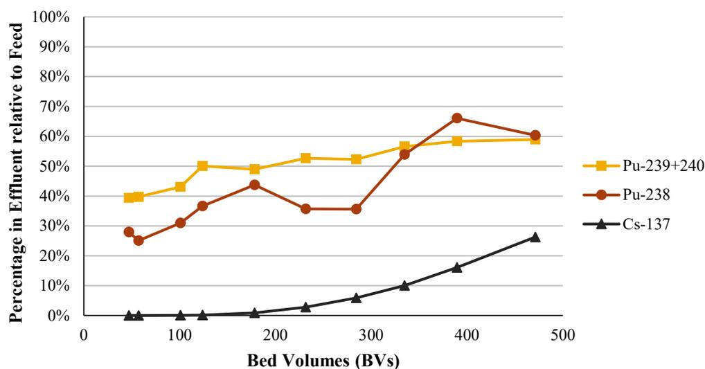
**Figure 5.1.** Increased Selected Radionuclide Percentage with Loading (Radiochemistry)
