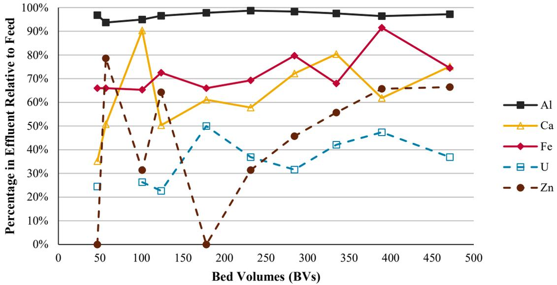
**Figure 5.3.** Increased or Erratic Selected Analyte Percentage with Loading (ICP-OES)
