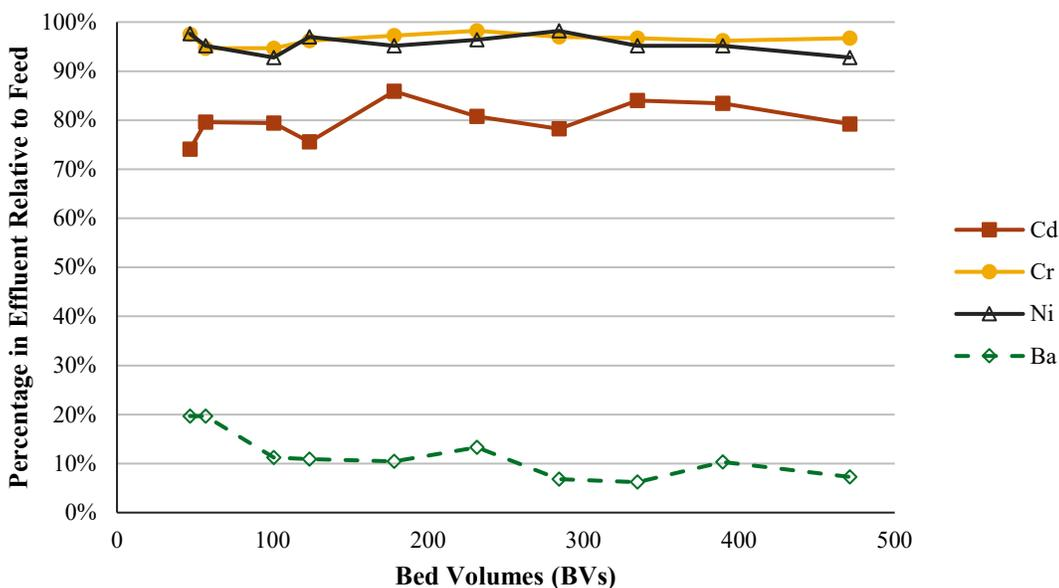
**Figure 5.4.** RCRA Element Percentages with Loading (ICP-OES)
