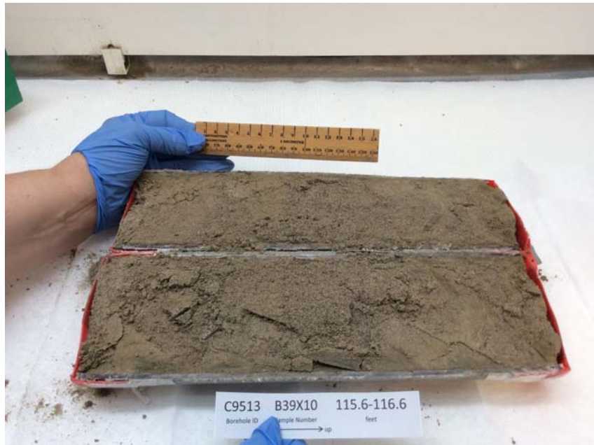
Figure 14. Core images of borehole S-13 (C9513) for sample B39X10 (Liner 18E, H2/CCUz sample).
