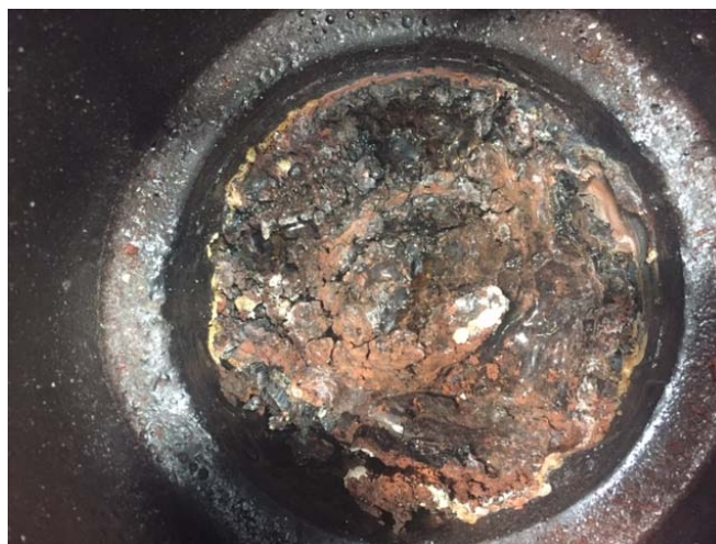
Figure 5.13. Top View of Melt Pool after Quenching (After Completion of the Test)
