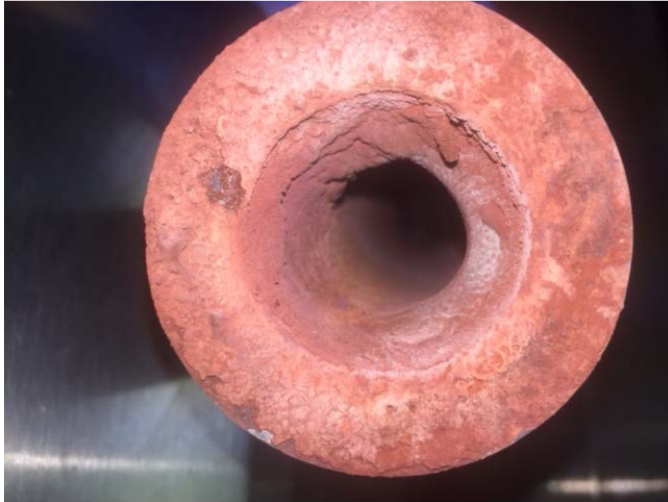
Figure 5.15. Off-Gas Deposits in the Film Cooler
