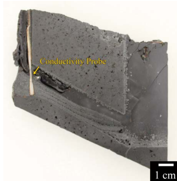
Figure 5.21. Polished Cross Section of the Other Half of the RSM Glass-Discharge Riser Section
