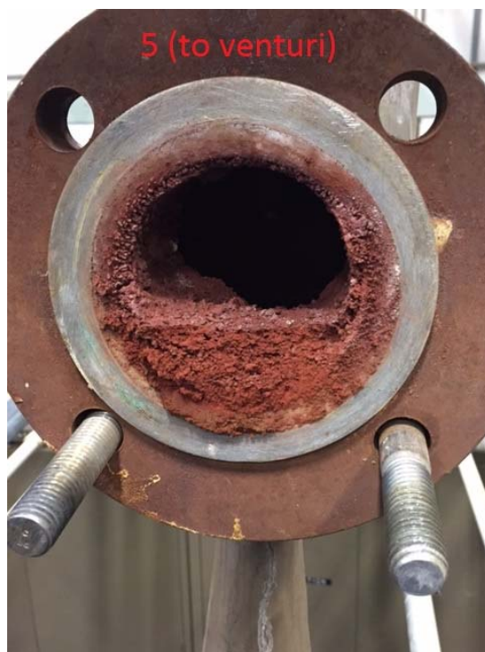
Figure 5.17. Off-Gas Deposits at the Entrance to the Ejector Venturi Scrubber (EVS) System
