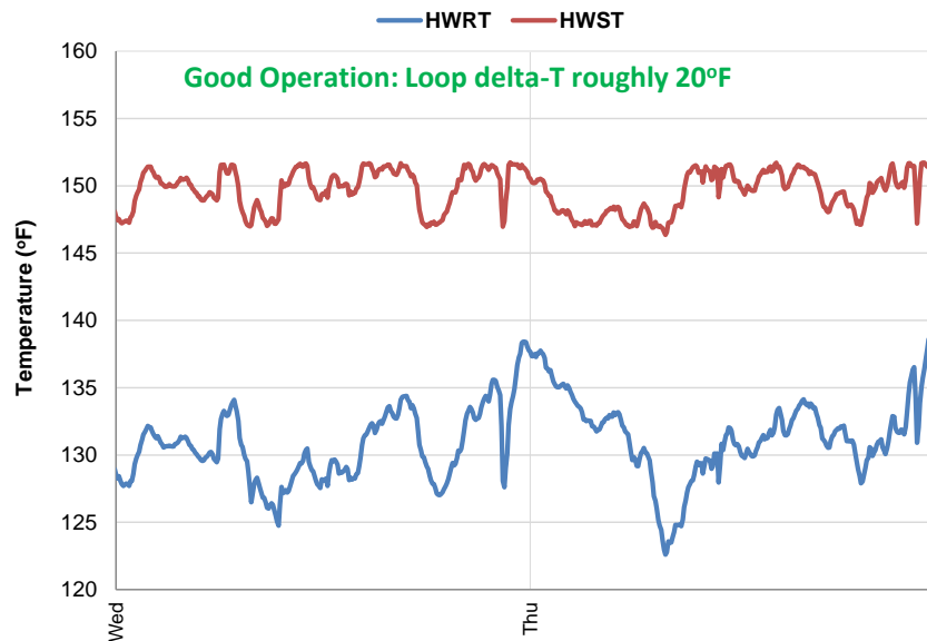
Figure 4.12. Example of Good Operations of HW System with Respect to Low Delta-T
