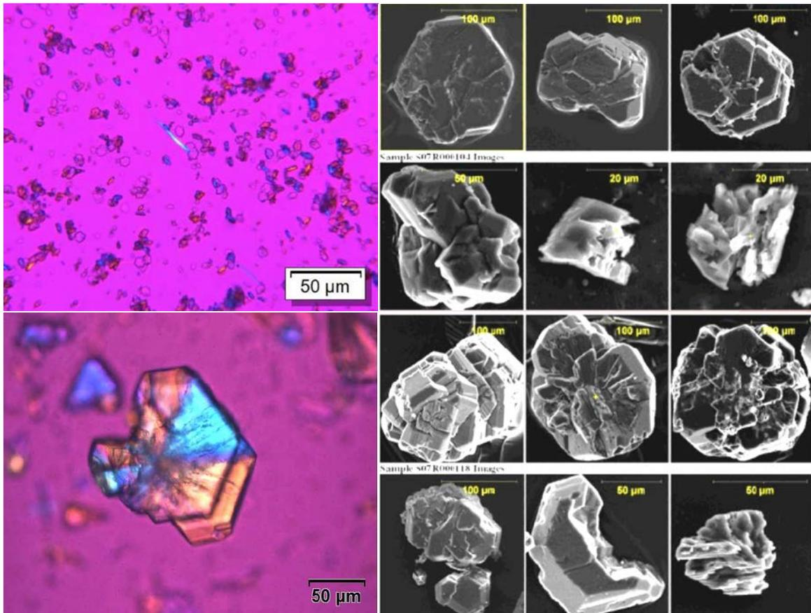
**Figure 1.** Microscope Images of Gibbsite from Hanford Tank Waste. Left: Polarized light microscope images of particles from Tanks 241-SX-101 (top) and -S-112 (bottom). Right: Scanning electron microscope images of particles from Tank 241-C-109. (Taken from Figures 3.1.2, 3.1.3, and 3.1.5, respectively, of Herting et al. 2015)
