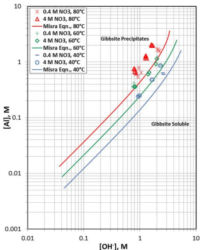
**Figure 4.** Gibbsite Solubility in the Presence of  $\text{NaNO}_3$  (Herting et al. 1986)
