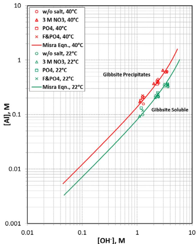
**Figure 5.** Gibbsite Solubility in the Absence/Presence of NaNO<sub>3</sub>, Na<sub>3</sub>PO<sub>4</sub>·12H<sub>2</sub>O, and Na<sub>7</sub>F(PO<sub>4</sub>)<sub>2</sub>·19H<sub>2</sub>O (Herting 2014)
