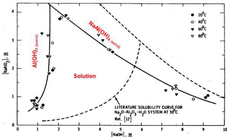
**Figure 7.** “Barney Diagram” for the Solubility of Gibbsite and Sodium Aluminate in Simulated Waste Solutions Saturated in Sodium Nitrate, Sodium Nitrite, Sodium Sulfate, and Sodium Carbonate (from Barney 1976; reference [12] in the figure is Volf and Kuznetsov 1955)
