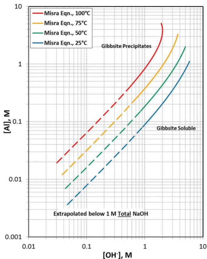
**Figure 2.** Gibbsite Solubility as Functions of NaOH Concentration and Temperature
