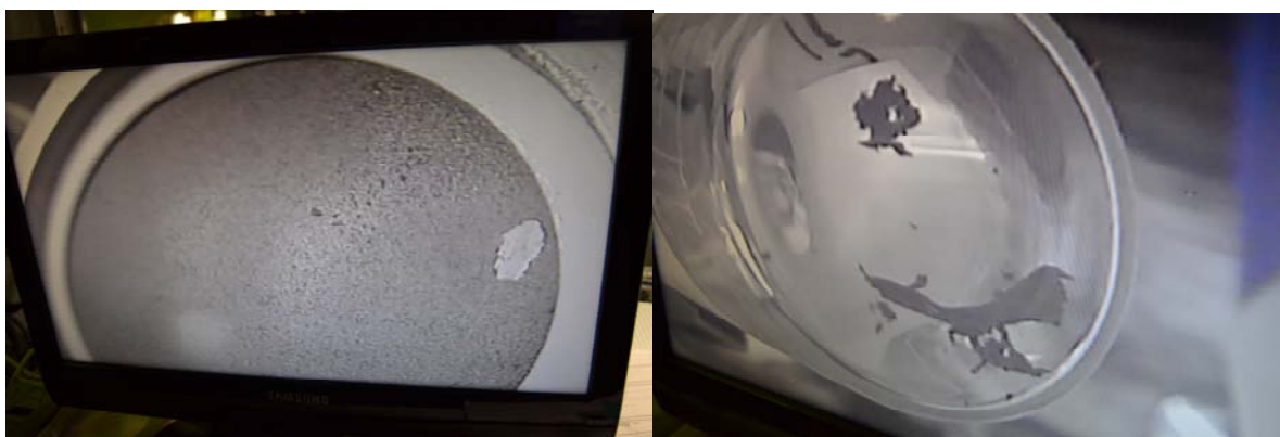
Figure 3.10. a) Picture of Solids on the Dead-end Filter, b) Picture of Solids in Vial after Collection
