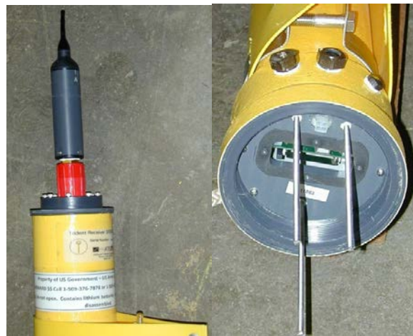
Figure 2.4. Outer (left) and Internal (right) Views of an Autonomous Node
