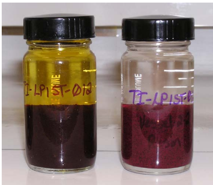
Figure 6.5. Test 2, resin color difference post-test: rad system (left), thermal system (right).
