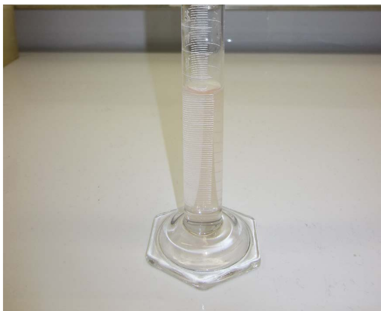
Figure 6.3. Pink-tinged liquid from Test 1 rad system water/resin after irradiation.
