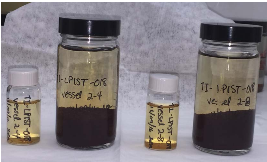
Figure 6.12. Test 4 thermal system post-test resin and simulant with HEDTA.
