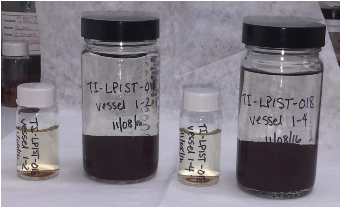
Figure 6.10. Test 4 rad system post-test water with resin.
