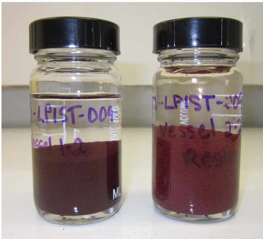
Figure 6.2. Color difference of resin from the rad system (left) and thermal system (right).
