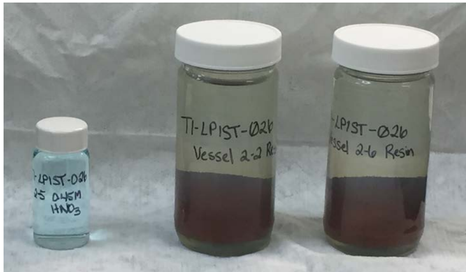
Figure 6.15. Nitric acid after exposure to the thermal vessel at 70 °C (left). Resin after exposure to nitric acid at 70 °C.
