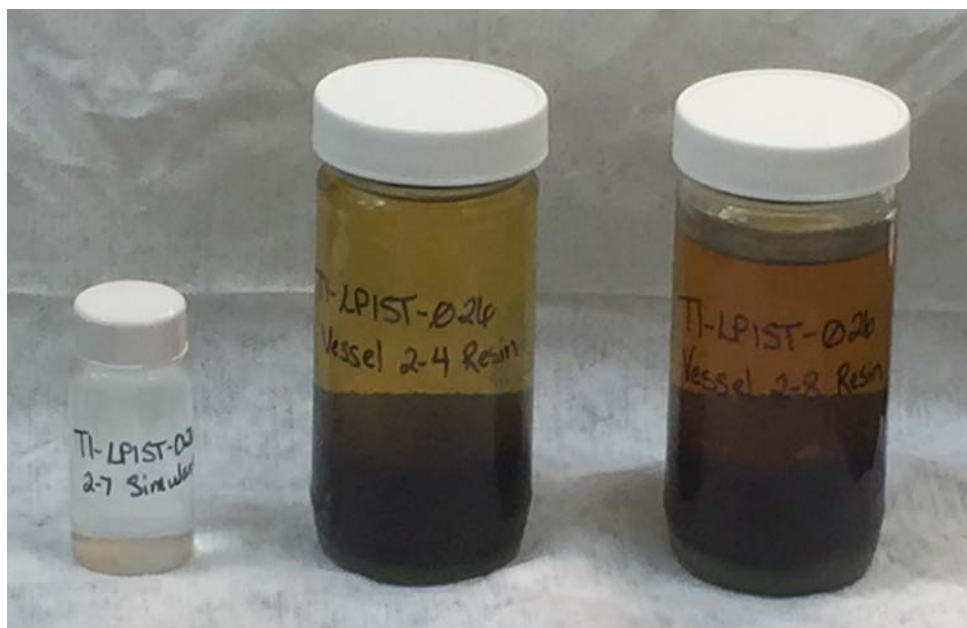
Figure 6.17. Test 5 post-test thermal system simulant and resin.
