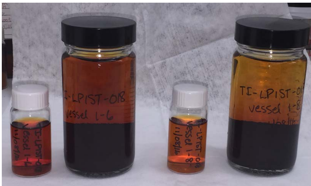
Figure 6.13. Test 4 rad system simulant with HEDTA and resin post-test.
