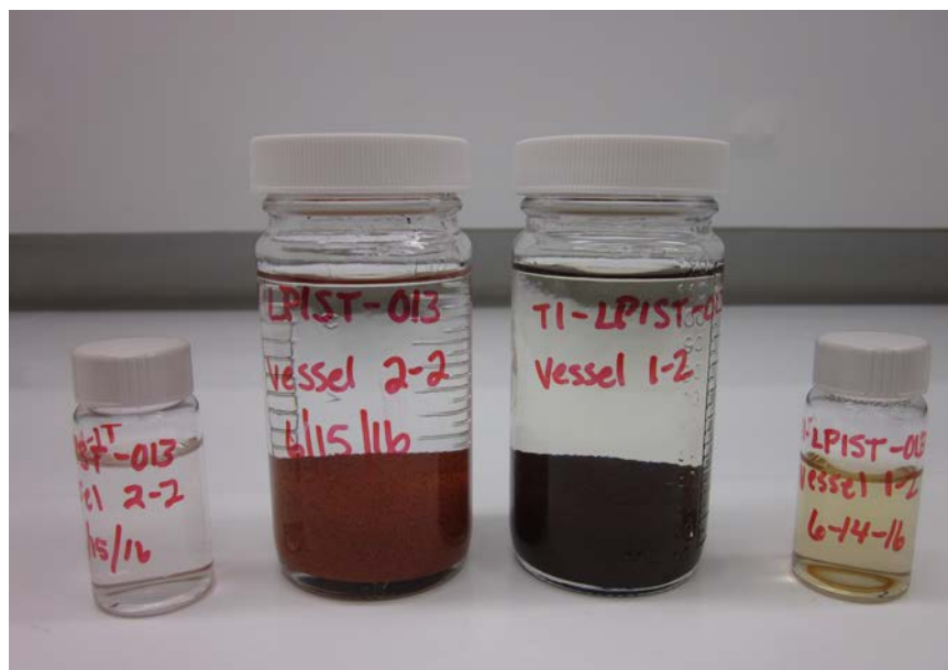
Figure 6.7. Comparison of Test 3 resin and liquids from the thermal system (left) and rad system (right).
