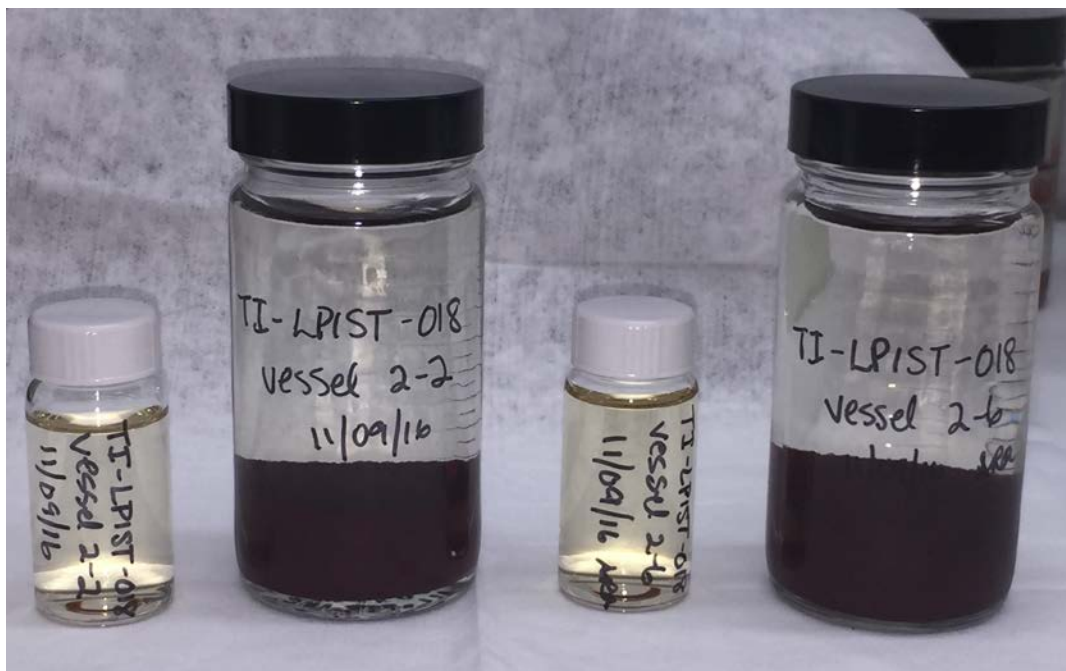
Figure 6.11. Test 4 thermal system post-test resin with water.
