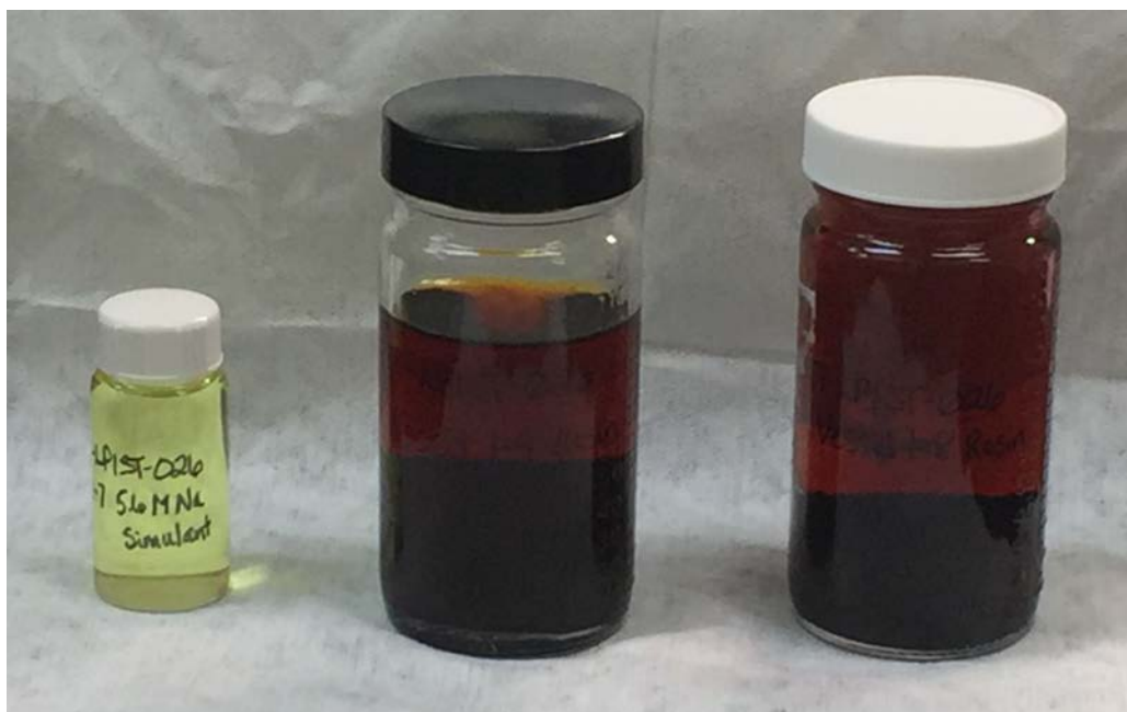
Figure 6.18. Test 5 post-test rad system simulant and resin.
