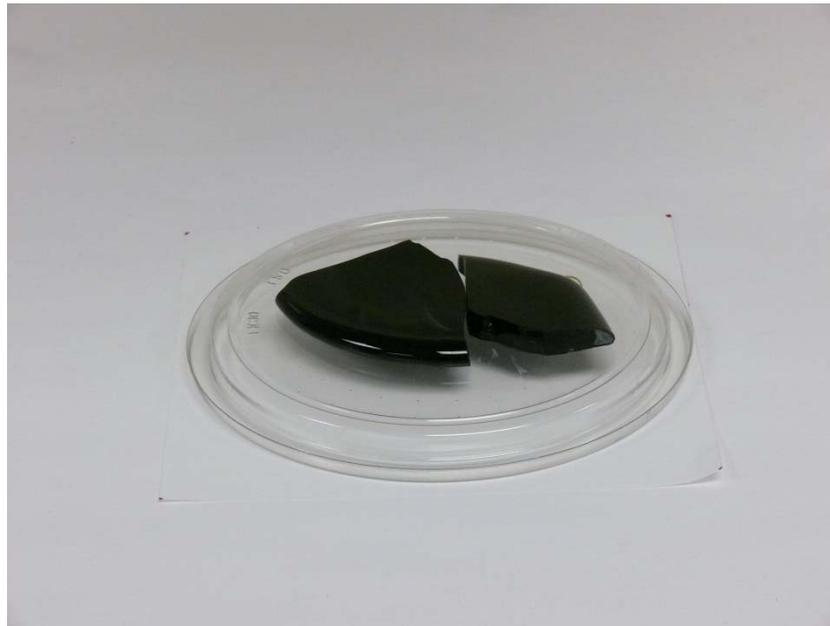
Figure 3.37. Photograph of Glass New-OL-65959 Second Modification Melted at 1250°C for 60 min (plastic disk is 12 cm diameter)
