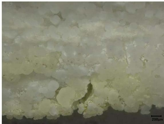
c) Micrograph of glass surface after VHT
