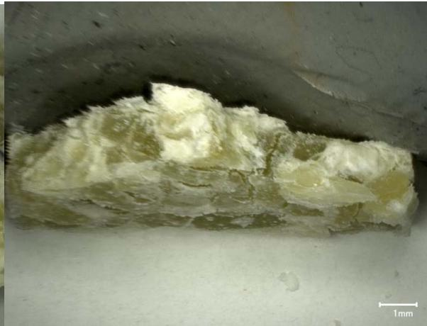
c) Micrograph of glass cross section after VHT
