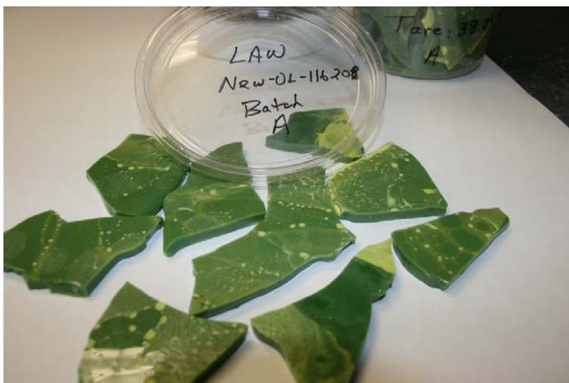
Figure 3.45. Photograph of Glass New-OL-116208 Original Composition Melted at 1200°C for 65 min (plastic disk is 12 cm diameter)
