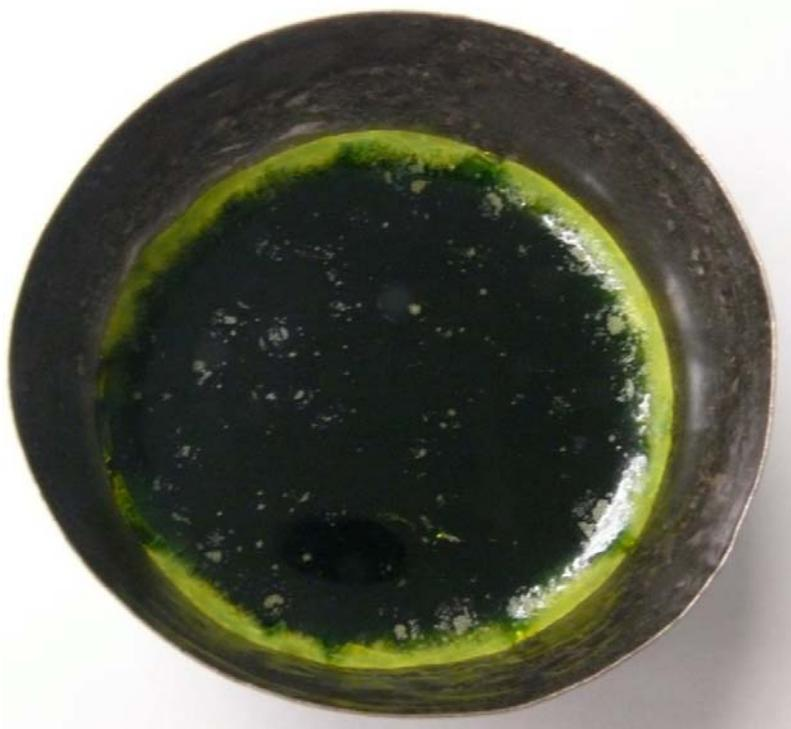
Figure 3.6. Photograph of Glass LAW-ORP-LD1(1) Cooled in a Pt Crucible with Crystals Along Edge
