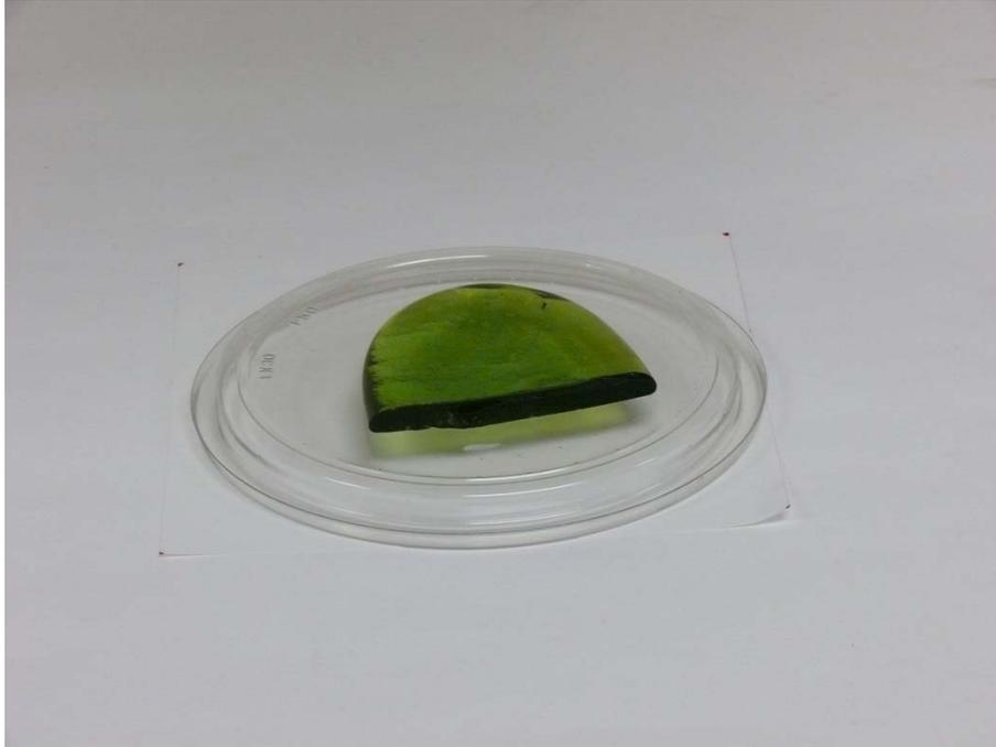
Figure 3.36. Photograph of Glass New-OL-65959 First Modification Melted at 1250°C for 60 min (plastic disk is 12 cm diameter)
