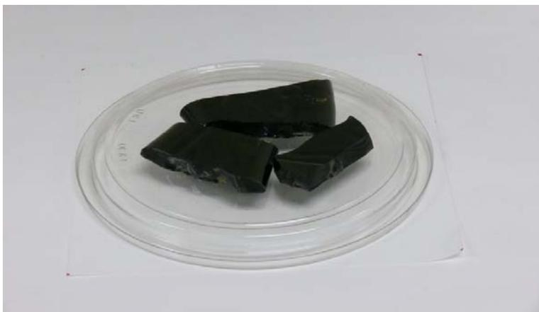
Figure 3.38. Photograph of Glass New-OL-65959 Final Modification Melted at 1250°C for 60 min (plastic disk is 12 cm diameter)
