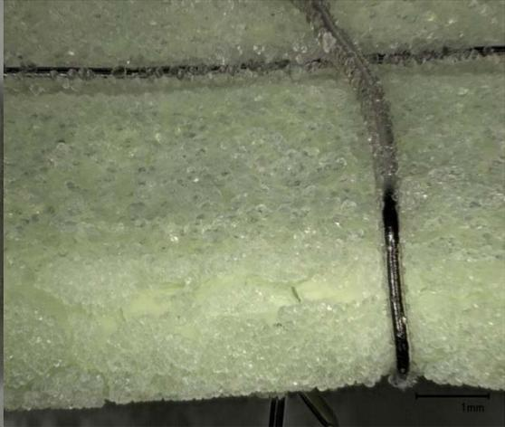
b) Micrograph of glass surface after VHT
