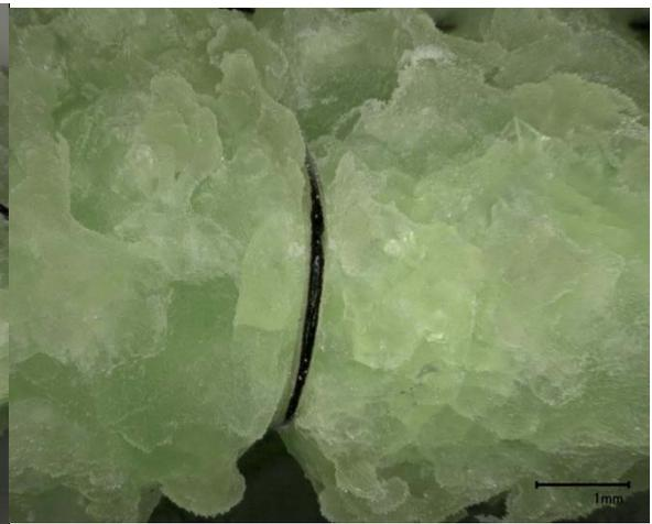
d) Micrograph of glass surface after VHT
