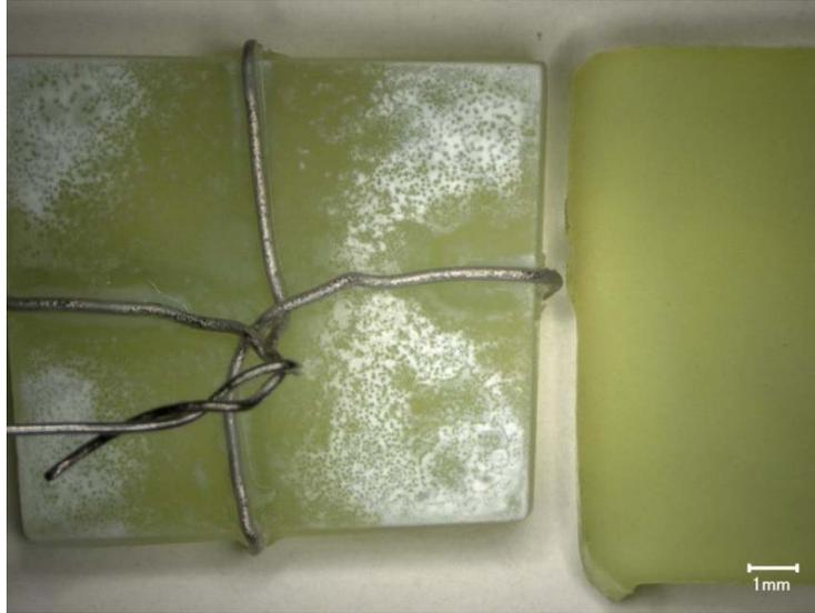
Figure F.2. Photo of Glass New-IL-456 after VHT for 7 Days (left) and before VHT (right) (1 cm square)
