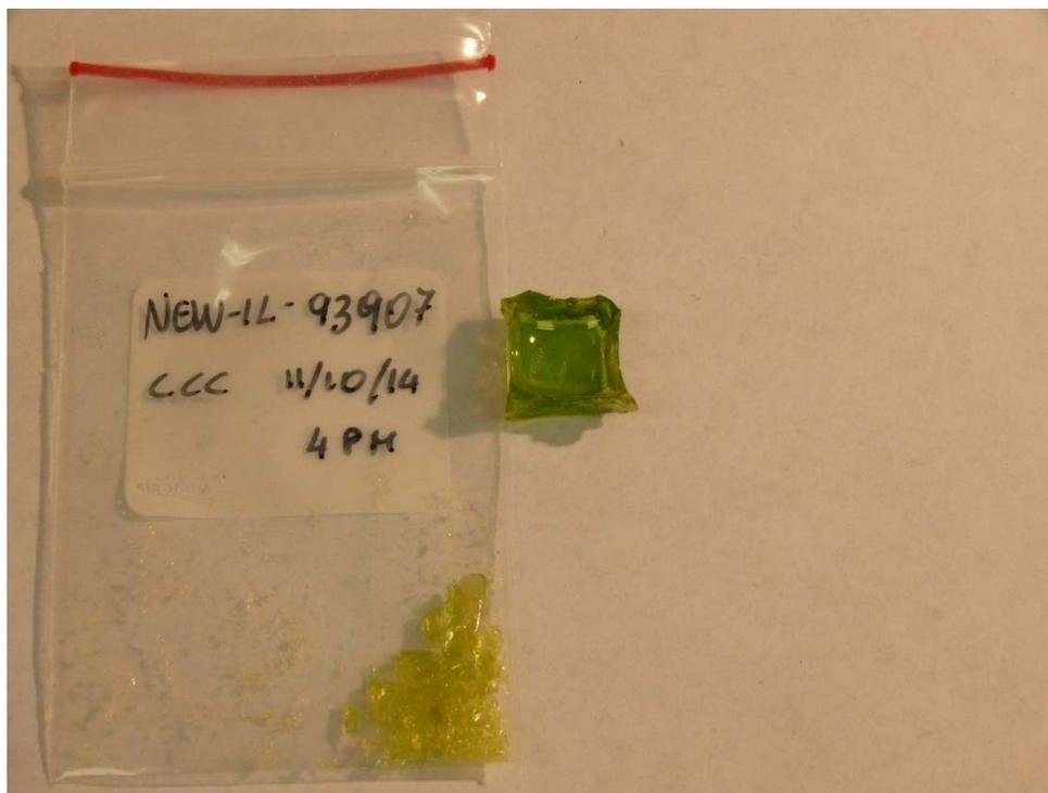
Figure D.6. Photograph of Glass New-IL-93907 after CCC Beginning at 1150°C (1 cm cube glass)
