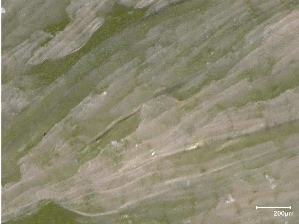
Figure D.2. Optical Micrograph of Glass New-IL-5253 Surface after CCC Beginning at 1150°C
