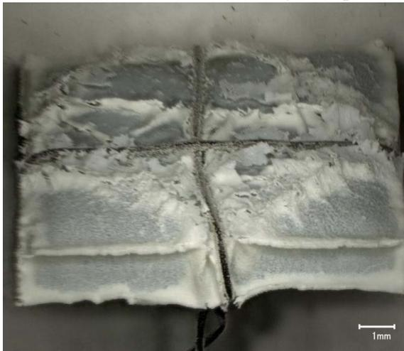
b) Micrograph of glass square after VHT
