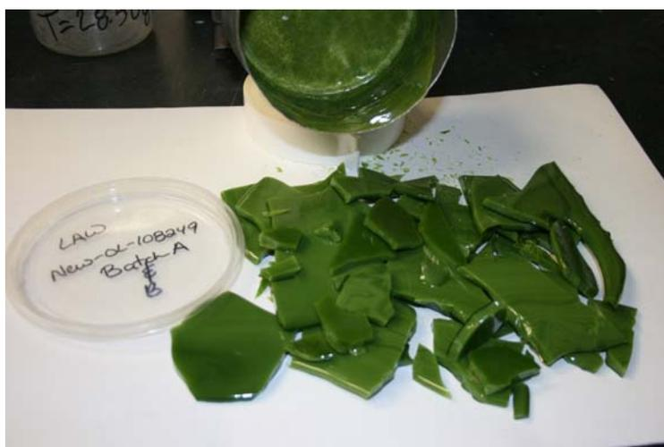
Figure 3.53. Photograph of Glass New-OL-108249 2<sup>nd</sup> Melt (1300°C for 60 min) after 2<sup>nd</sup> Sulfur Washing (plastic disk is 12 cm diameter)
