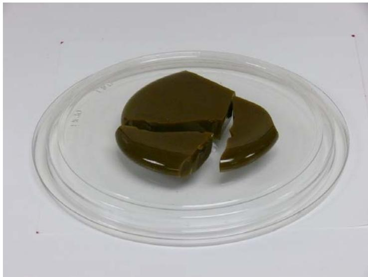
Figure 3.17. Photograph of First Compositional Modification of New-OL-8788 Glass Melted at 1350°C for 90 min (plastic disk is 12 cm diameter)
