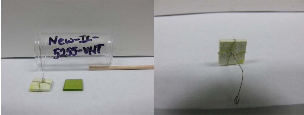
a) Photo of glass square (1 cm) after and before VHT      b) Photo of glass square (1 cm) after VHT
