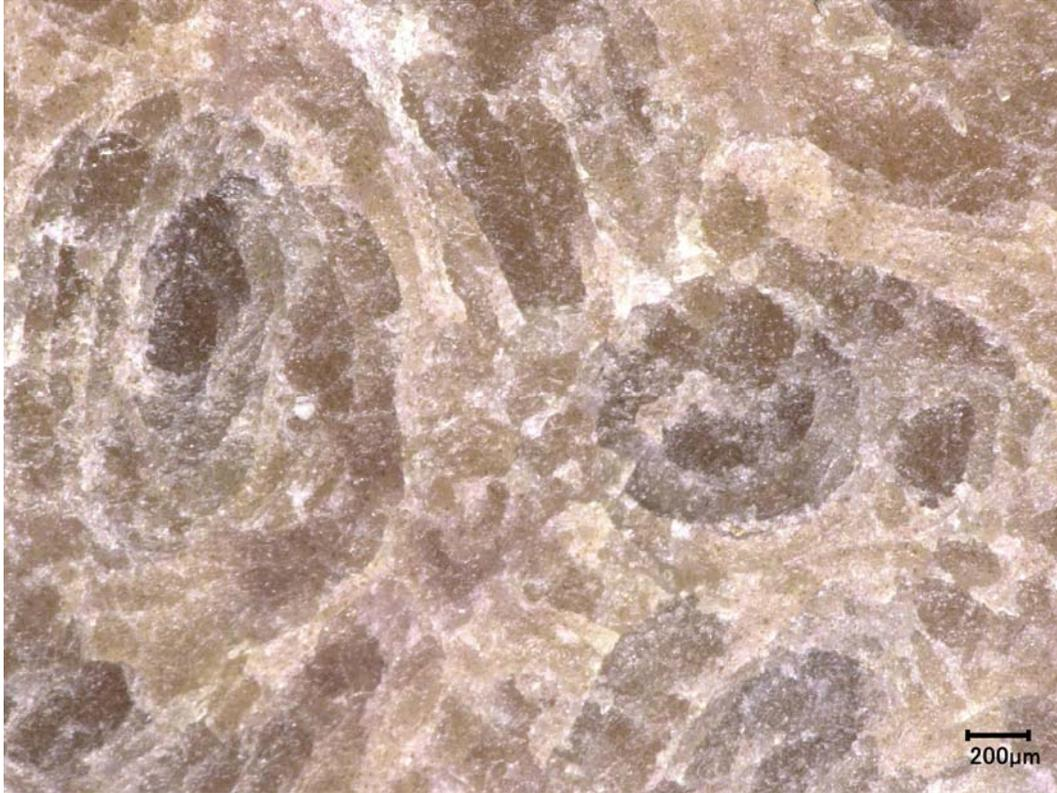
Figure D.16. Optical Micrograph of Glass New-OL-45748 (Sn Mod) after CCC Beginning at 1300°C
