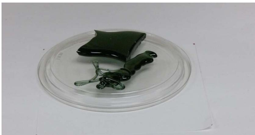
Figure 3.50. Photograph of Glass New-OL-127708 after 3<sup>rd</sup> Modification Melted at 1300°C for 60 min (plastic disk is 12 cm diameter)
