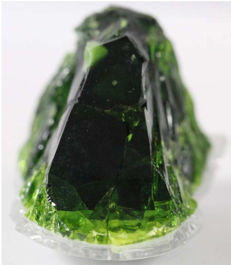
Figure D.29. Photograph of LAW-ORP-LD1-3 after CCC Beginning at 1300°C from Quartz Crucible
