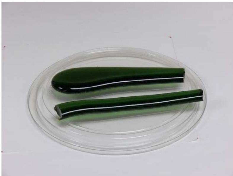
Figure 3.21. Photograph of Final Compositional Modification of New-OL-8788 Glass Melted at 1300°C for 60 min (plastic disk is 12 cm diameter)
