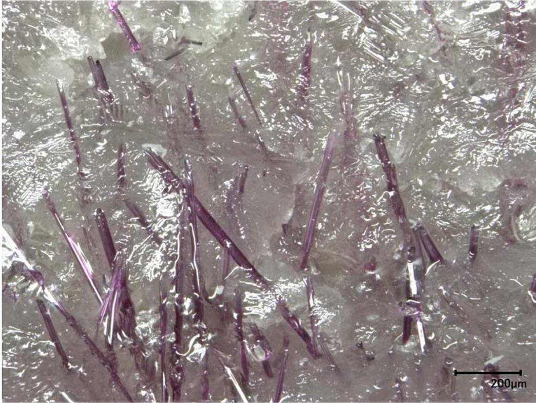
Figure D.20. Optical Micrograph of Glass New-OL-65959(Mod) after CCC Beginning at 1225°C
