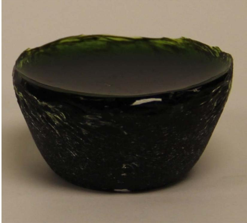
Figure 3.7. Photograph of Glass LAW-ORP-LD1(1) Cooled in a Quartz Crucible without Crystals along Edge
