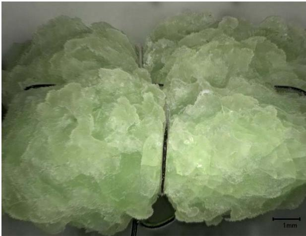
c) Micrograph of glass square after VHT
