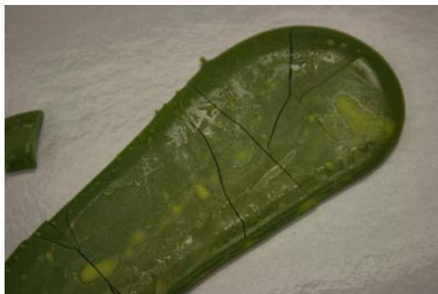
Figure 3.46. Photograph of Glass New-OL-116208 3<sup>rd</sup> Modification Melted at 1200°C for 65 min
