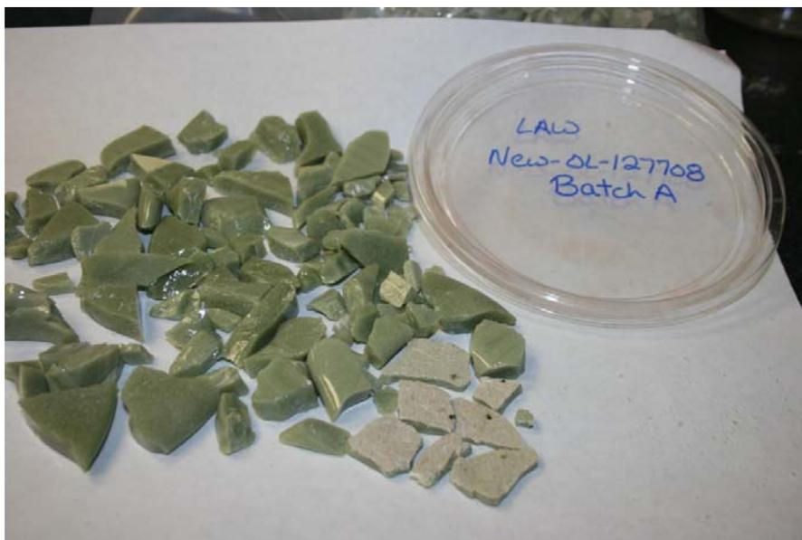
Figure 3.47. Photograph of Glass New-OL-127708 Original Composition Melted at 1350°C for 60 min (plastic disk is 12 cm diameter)
