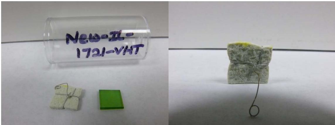
a) Photo of glass square (1 cm) after and before VHT    b) Photo of glass square (1 cm square) after VHT
