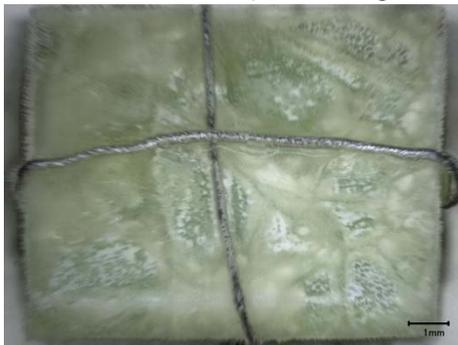
b) Micrograph of glass square after VHT
