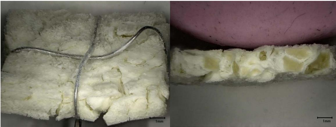
c) Micrograph of glass square after VHT
