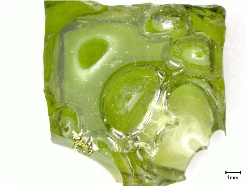
Figure D.1. Photograph of Glass New-IL-456 after CCC Beginning at 1200°C
