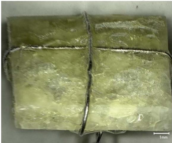
b) Micrograph of glass square after VHT
