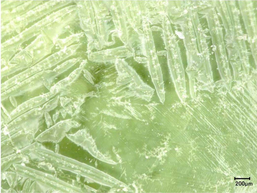
Figure D.22. Optical Micrograph of Glass New-OL-90780 after CCC Beginning at 1200°C
