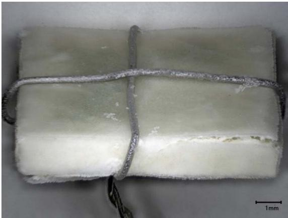
b) Micrograph of glass square after VHT
