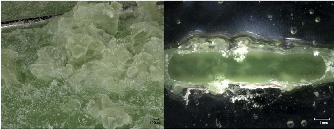
c) Micrograph of glass surface after VHT
