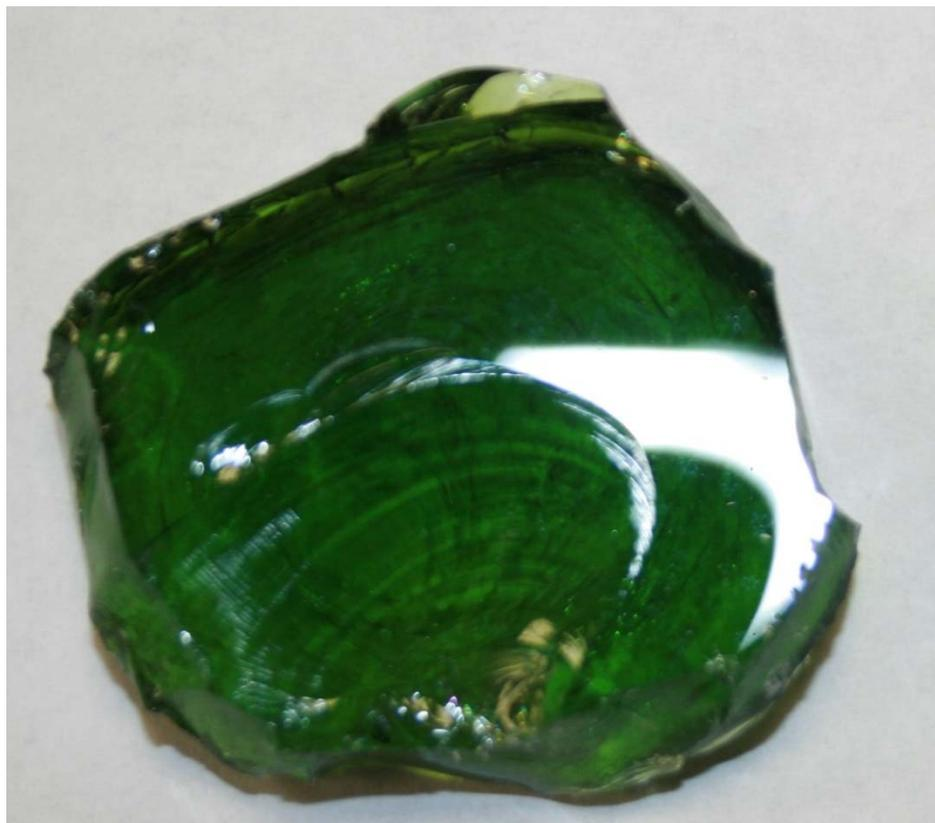
Figure D.7. Photograph of Glass New-IL-94020 after CCC Beginning at 1300°C
