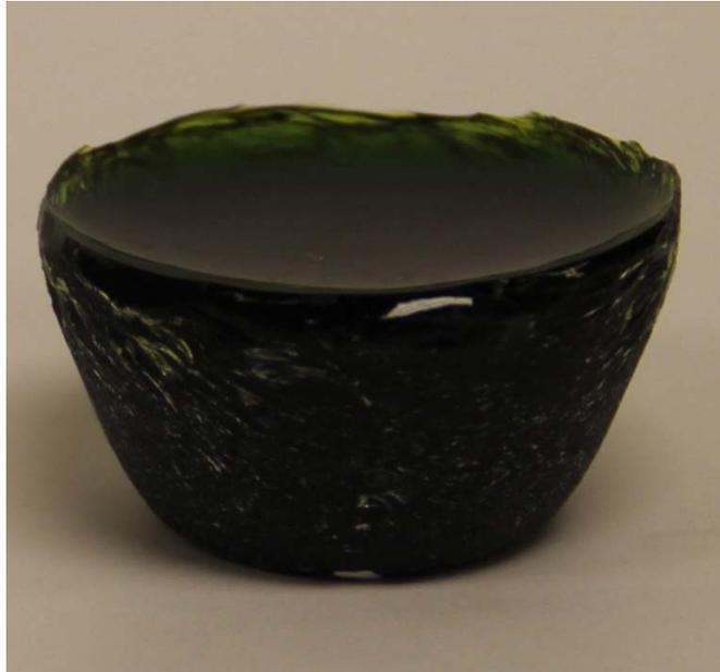
Figure D.27. Photograph of LAW-ORP-LD1-1 after CCC Beginning at 1300°C from 1 cm cube Pt Crucible (top) and Quartz Crucible (bottom)
