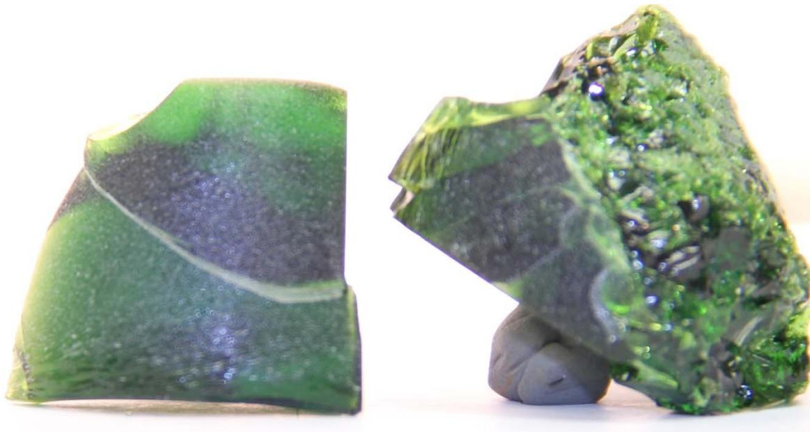
Figure D.28. Photograph of LAW-ORP-LD1-2 after CCC Beginning at 1300°C from Quartz Crucible
