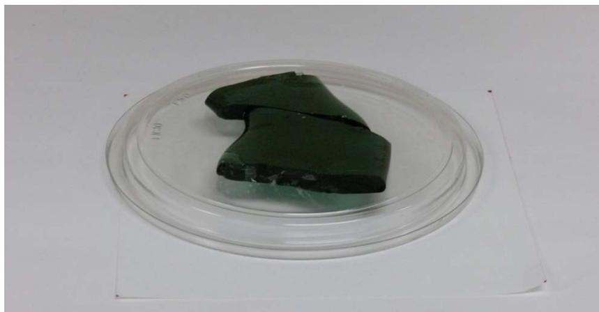
Figure 3.51. Photograph of Glass New-OL-127708 Final Composition Melted at 1300°C for 60 min (plastic disk is 12 cm diameter)
