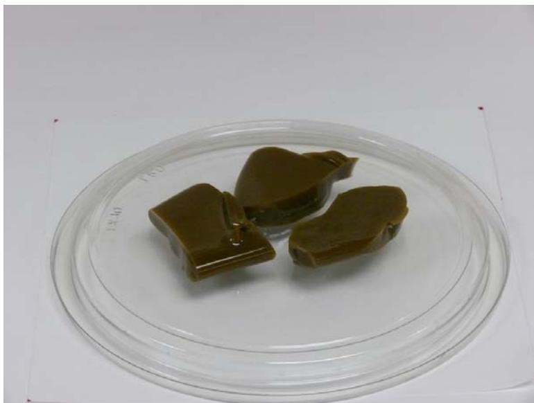
Figure 3.18. Photograph of Second Compositional Modification of New-OL-8788 Glass Melted at 1325°C for 60 min (plastic disk is 12 cm diameter)
