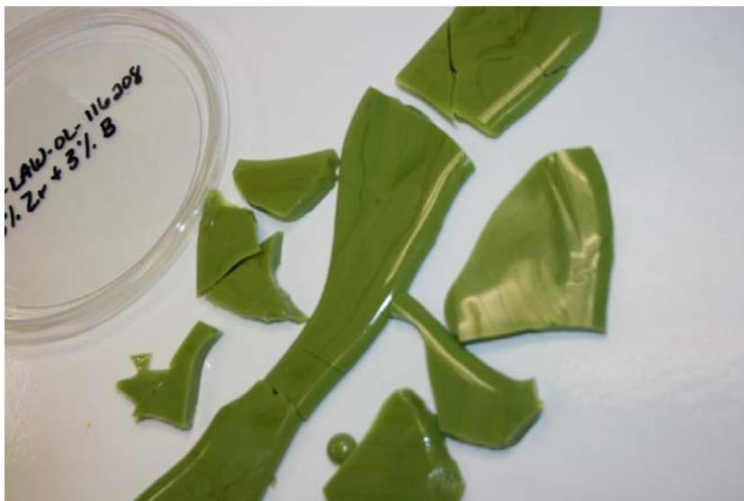
Figure 3.44. Photograph of Glass New-OL-116208 2<sup>nd</sup> Modification Melted at 1200°C for 60 min (plastic disk is 12 cm diameter)
