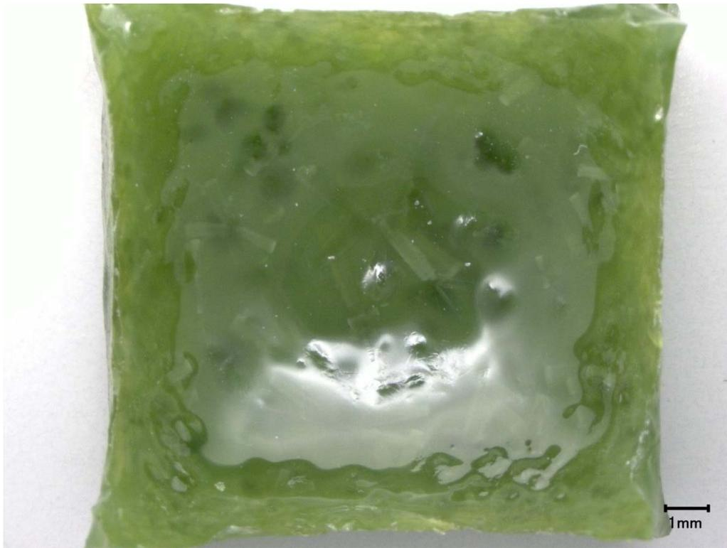
Figure D.18. Photograph of Glass New-OL-57284 after CCC Beginning at 1225°C
