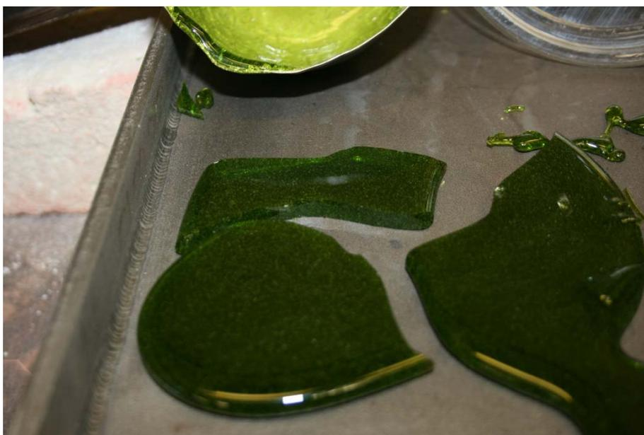
Figure 3.40. Photograph of Glass New-OL-108249 4<sup>th</sup> Modification Melted at 1150°C for 60 min
