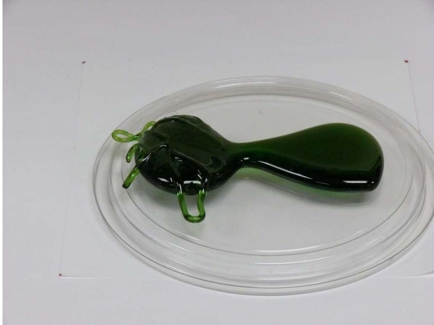
Figure 3.19. Photograph of Third Modification of New-OL-8788 Glass Melted at 1300°C for 60 min (plastic disk is 12 cm diameter)
