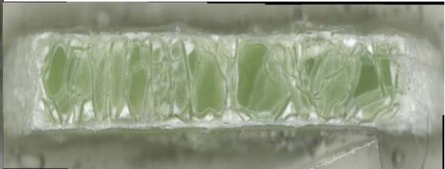
c) Micrograph of glass cross section after VHT
