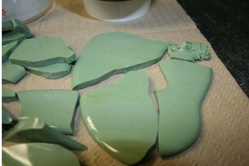
Figure 3.28. Photograph of Glass New-OL-62909 Original Composition Melted at 1300°C for 60 min
