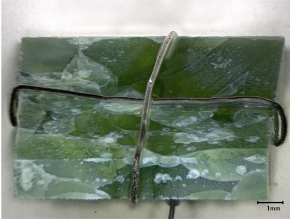
b) Micrograph of glass square after VHT
