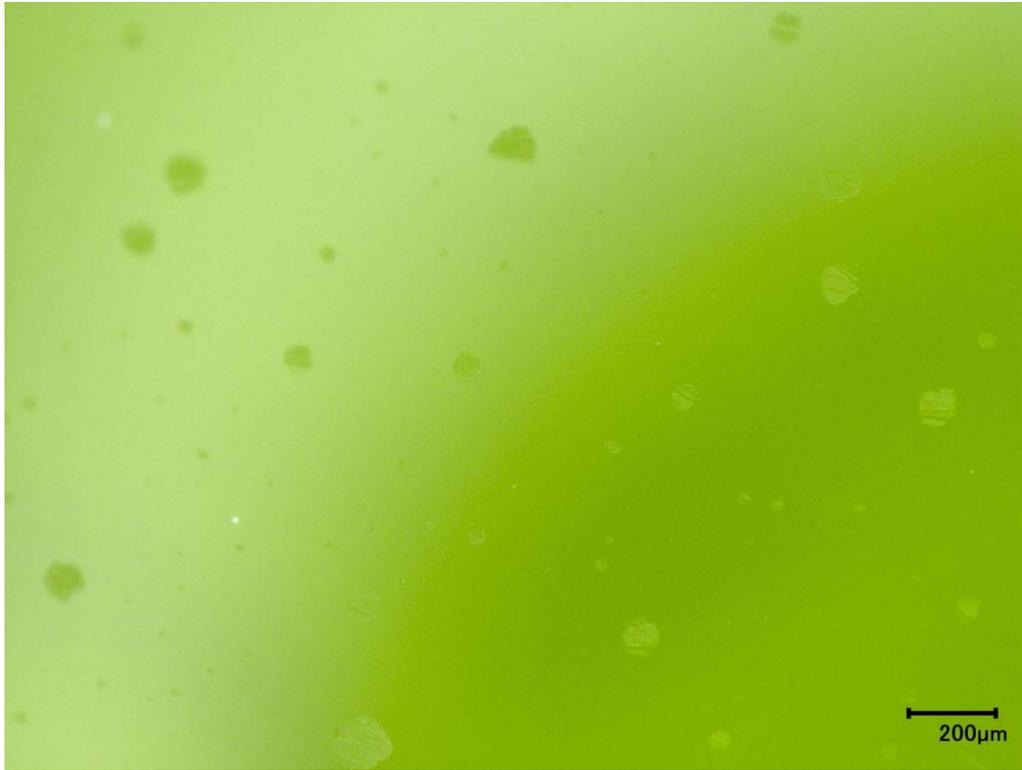
Figure D.24. Optical Micrograph of Glass New-OL-122817 after CCC Beginning at 1200°C
