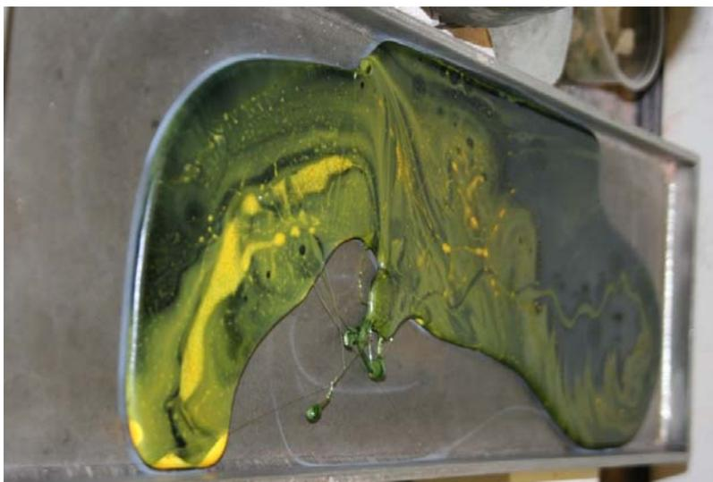
Figure 3.39. Photograph of Glass New-OL-108249 Original Composition Melted at 1200°C for 65 min
