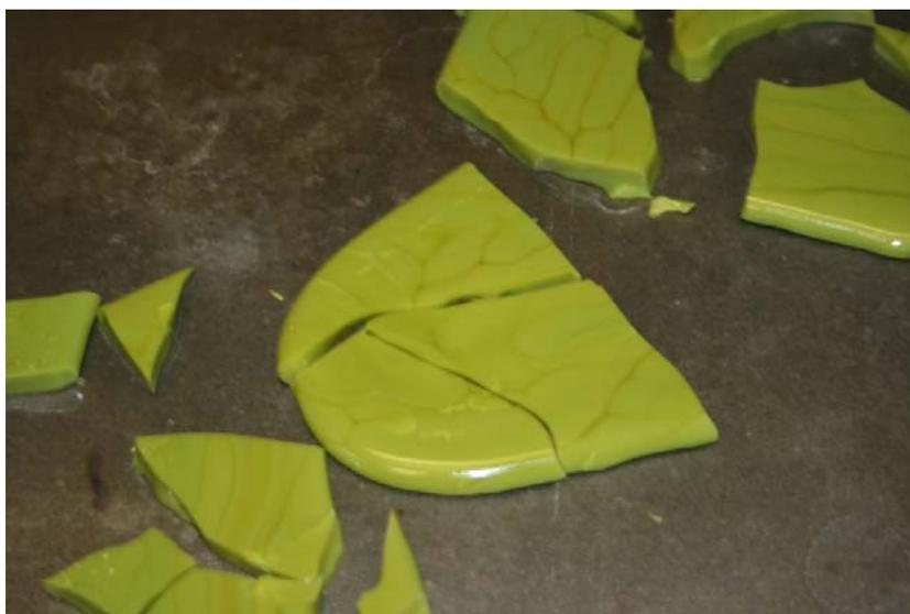
Figure 3.43. Photograph of Glass New-OL-116208 1<sup>st</sup> Modification Melted at 1200°C for 60 min
