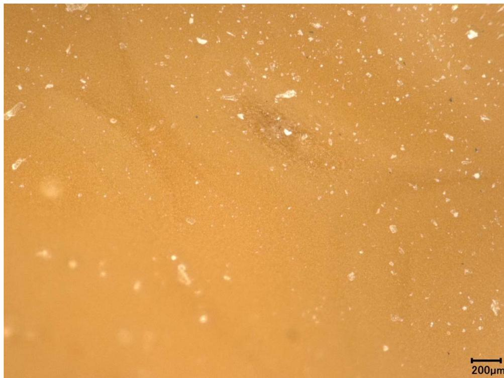
Figure D.13. Optical Micrograph of Glass New-OL-8788(Mod) after CCC Beginning at 1150°C
