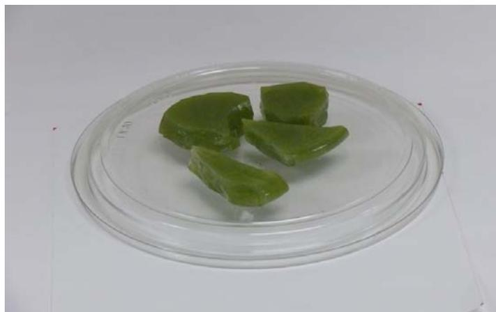
Figure 3.49. Photograph of Glass New-OL-127708 after 1<sup>st</sup> Modification Melted at 1300°C for 90 min (plastic disk is 12 cm diameter)
