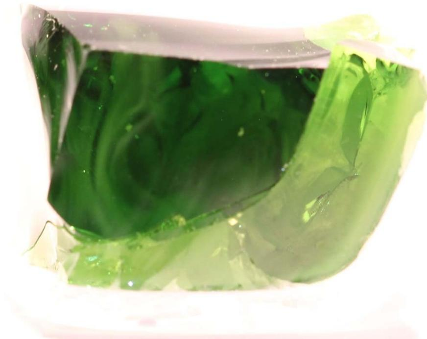
Figure D.10. Photograph of Glass New-IL-166697 after CCC Beginning at 1250°C from Pt Crucible 1 cm Cube (top) and Quartz Crucible (bottom)
