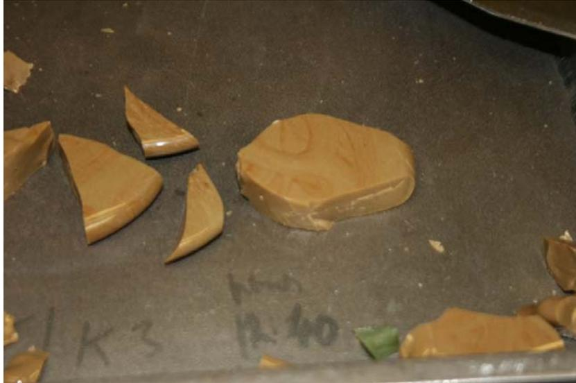
Figure 3.16. Photograph of First Melt of New-OL-8788 Glass with Increased Melt Temperature to 1325°C for 90 min
