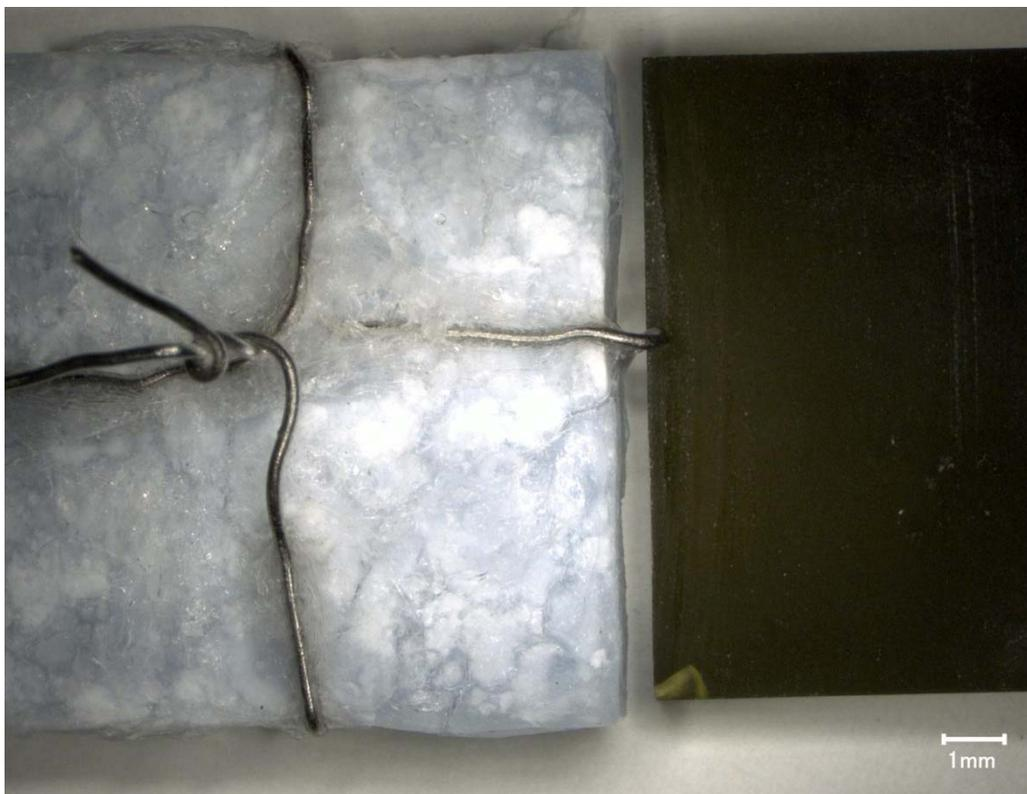
Figure 3.13. Photograph of Glass New-OL-65959(Mod) Before (Right) and After (Left) VHT
