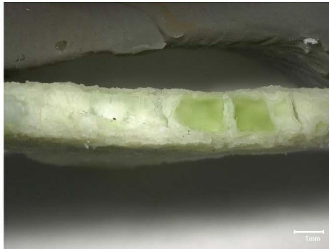
c) Micrograph of glass cross section after VHT
