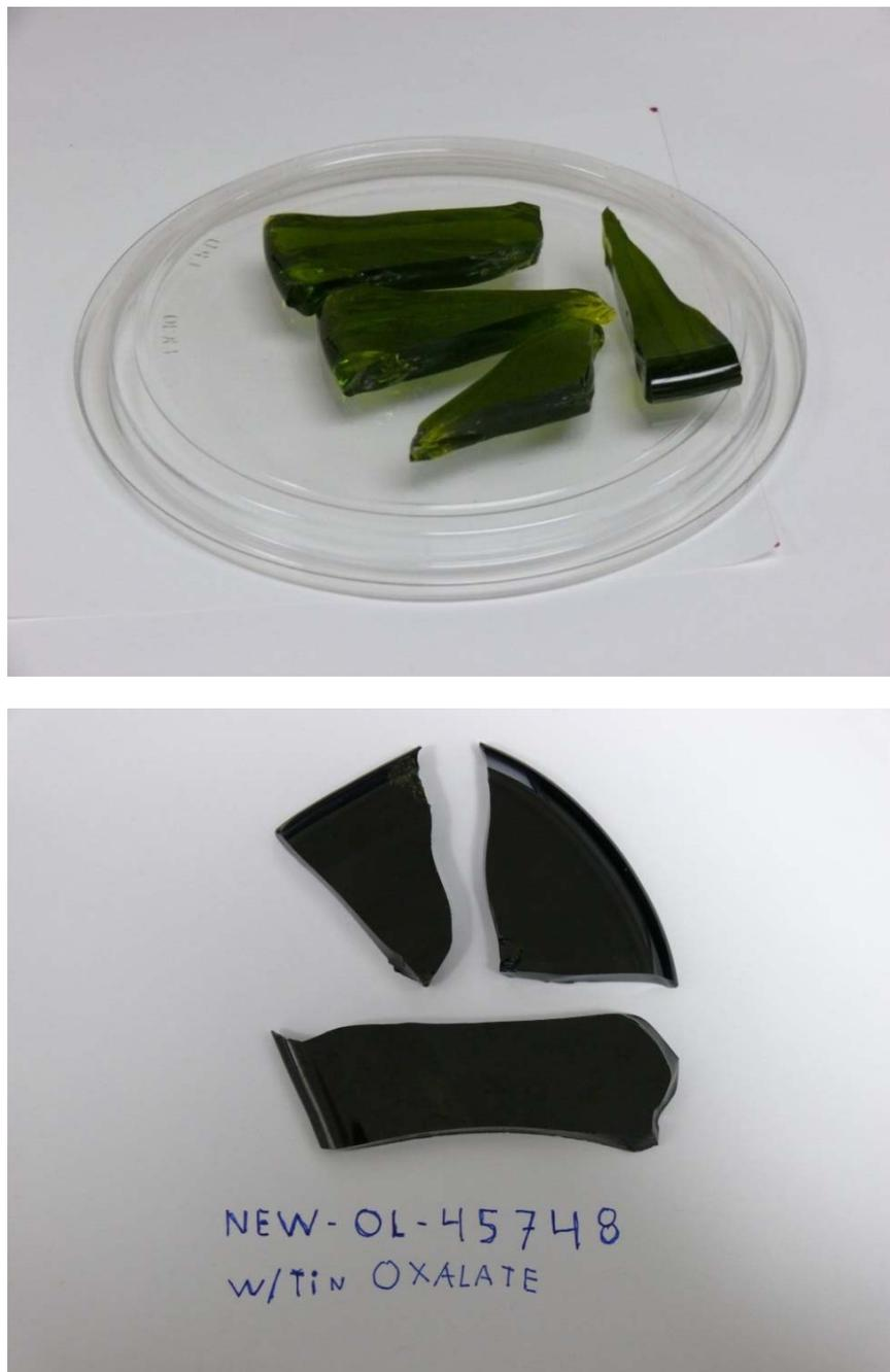
Figure 3.23. Photographs of Glass New-OL-45748 Color Comparison with Oxidizing Conditions (top) and Reducing Conditions (bottom) (plastic disk is 12 cm diameter)
