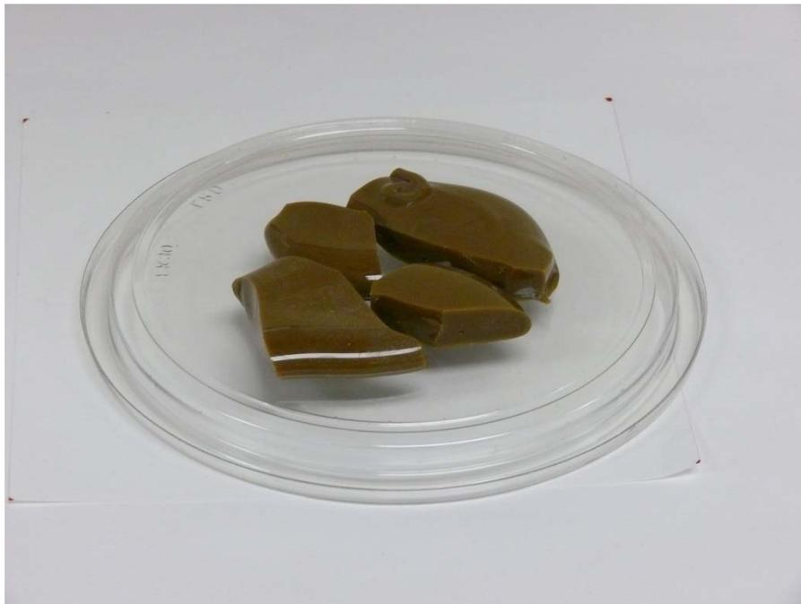
Figure 3.20. Photograph of Fourth Modification of New-OL-8788 Glass Melted at 1300°C for 60 min (plastic disk is 12 cm diameter)
