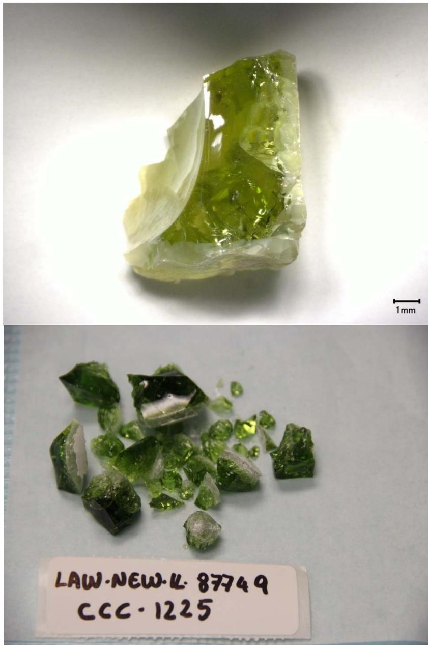
Figure D.5. Photograph of Glass New-IL-87749 after CCC Beginning at 1225°C from Pt Crucible (bottom) and Quartz Crucible (top)
