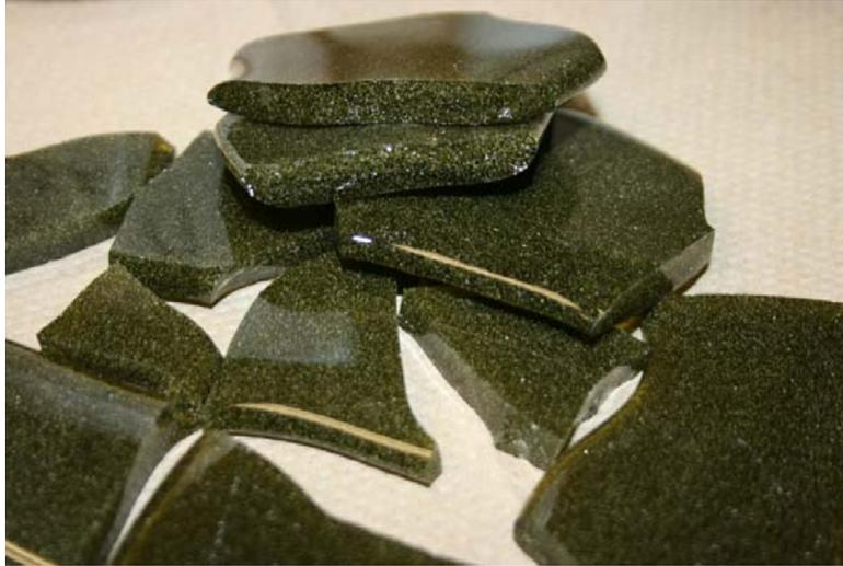
Figure 3.25. Photograph of Glass New-OL-54017 Original Composition Melted at 1200°C for 85 min
