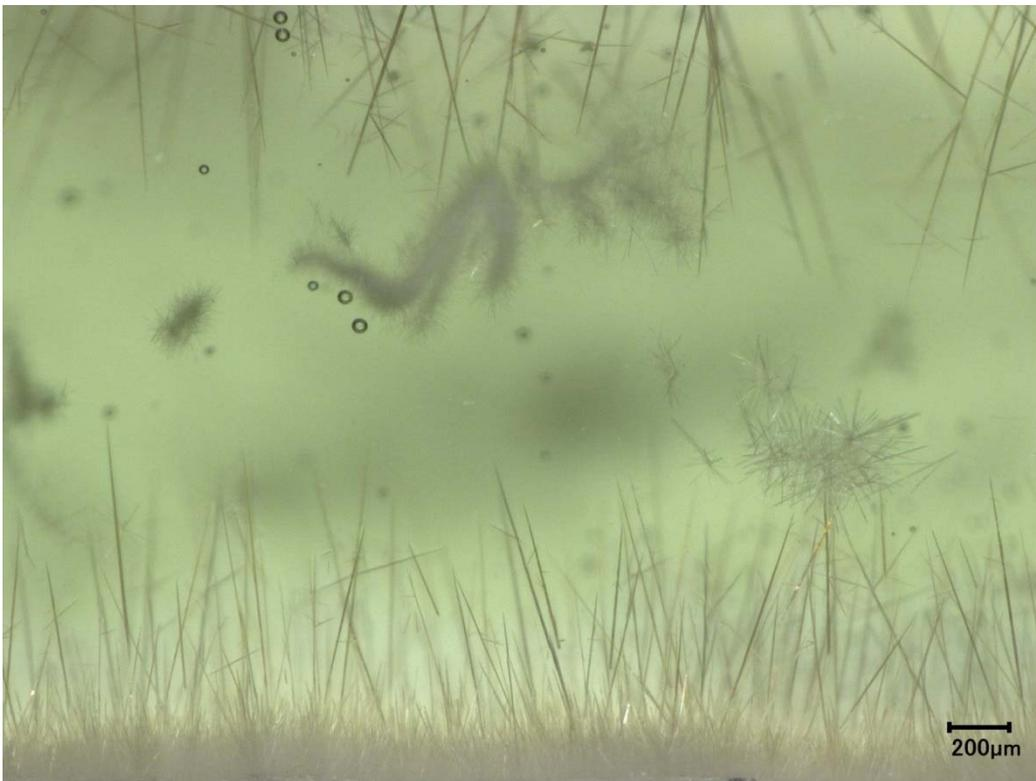
Figure D.25. Optical Micrograph of Glass New-OL-127708(Mod) after CCC Beginning at 1150°C
