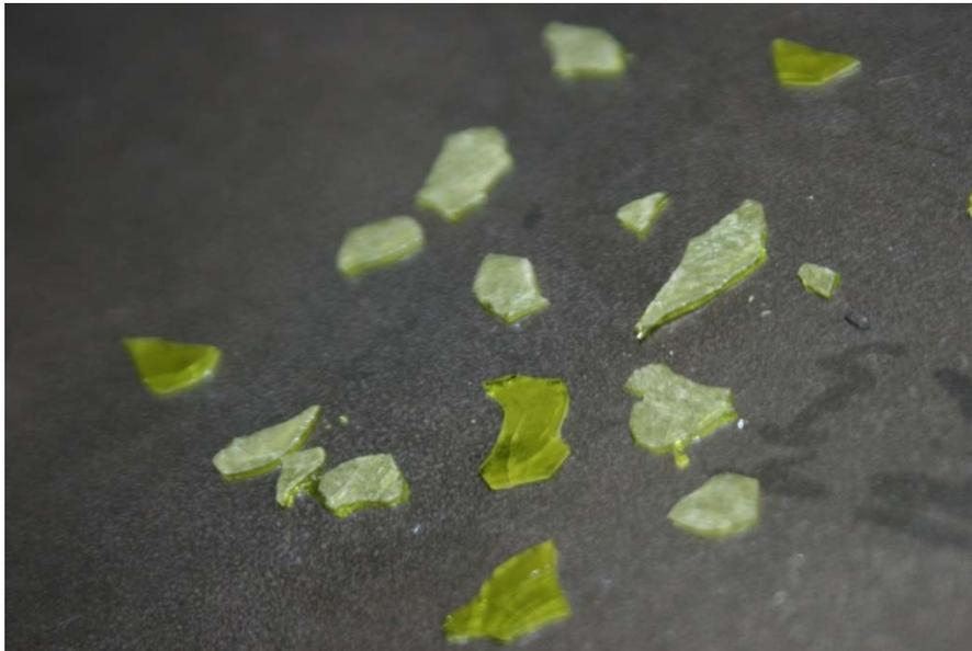
Figure 3.22. Photograph of New-OL-45748 Glass from Bottom of Crucible after First Modification Melted at 1300°C for 90 min
