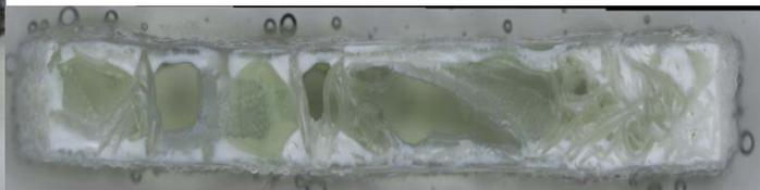
c) Micrograph of glass cross section after VHT
