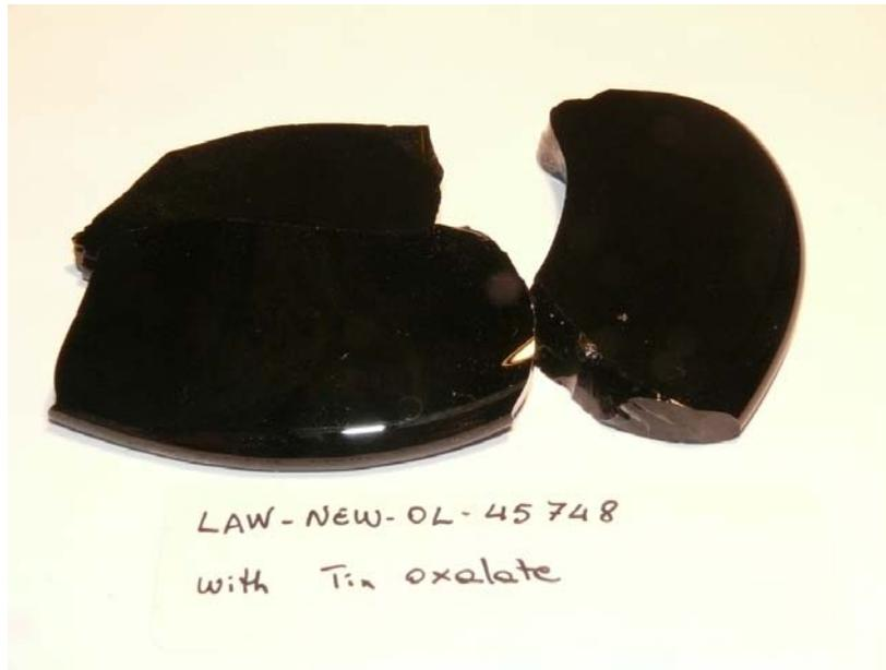
Figure 3.24. Photograph of Melt of New-OL-45748 with Tin Oxalate Substituted for Tin Oxide in Original Composition Melted at 1300°C for 60 min
