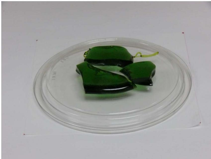
Figure 3.31. Photograph of First Modification of Glass New-OL-62909 Melted at  $1300^\circ\text{C}$  for 60 min (plastic disk is 12 cm diameter)
