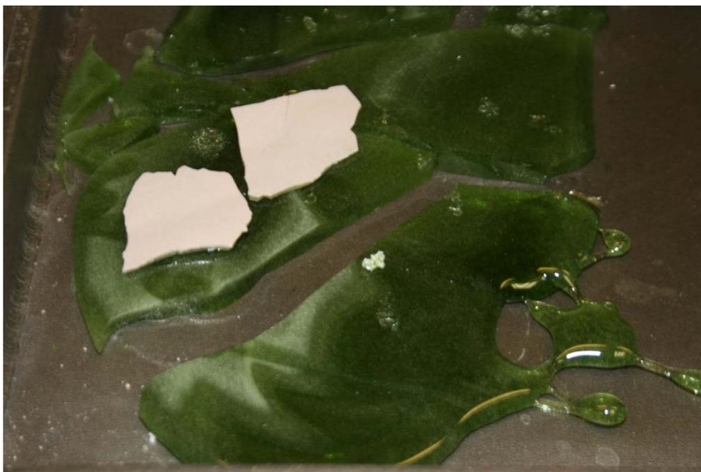
Figure 3.34. Photograph of Glass New-OL-65959 Original Composition with Large Ceramic Pieces Melted at 1275°C for 75 min
