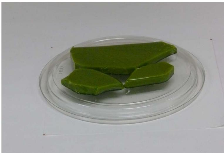
Figure 3.56. Photograph of Glass New-OL-116208 Final Composition after Final Pour Melted at 1300°C for 60 min (plastic disk is 12 cm diameter)
