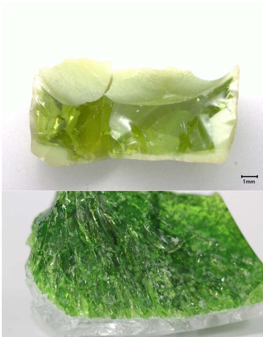
Figure D.11. Photograph of New-IL-166731 after CCC Beginning at 1225°C from Pt Crucible (top) and Quartz Crucible (bottom)
