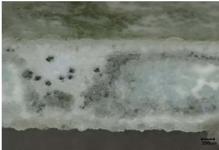
c) Micrograph of glass surface after VHT
