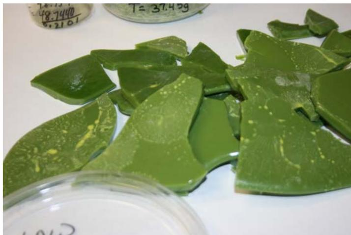
Figure 3.52. Photograph of Glass New-OL-108249 1<sup>st</sup> Melt after 1<sup>st</sup> Sulfur Washing Melted at 1150°C for 60 min
