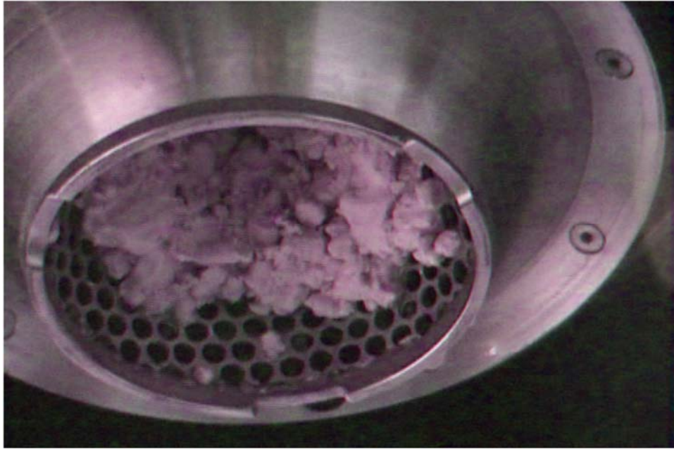
Figure 2.2. Screen Clogging during Prior Tests
