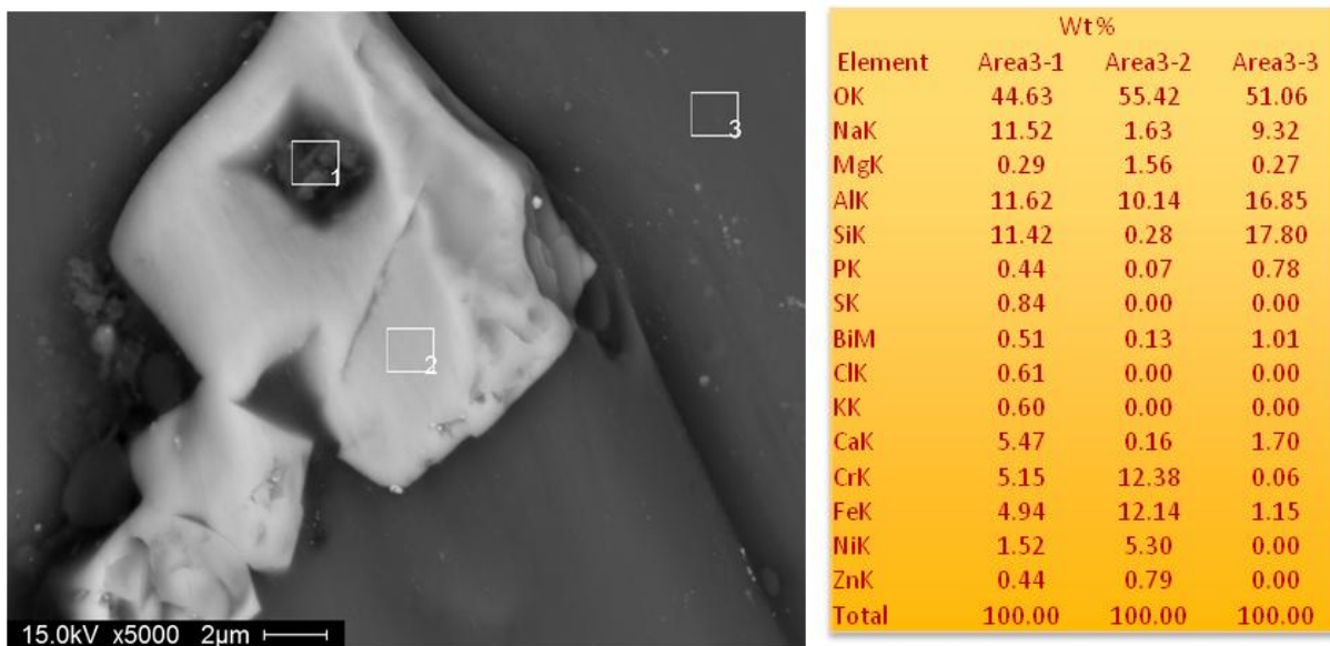
Figure 7.3. Micrograph and EDS of a Large Crystal in the RSM-6 Melt
