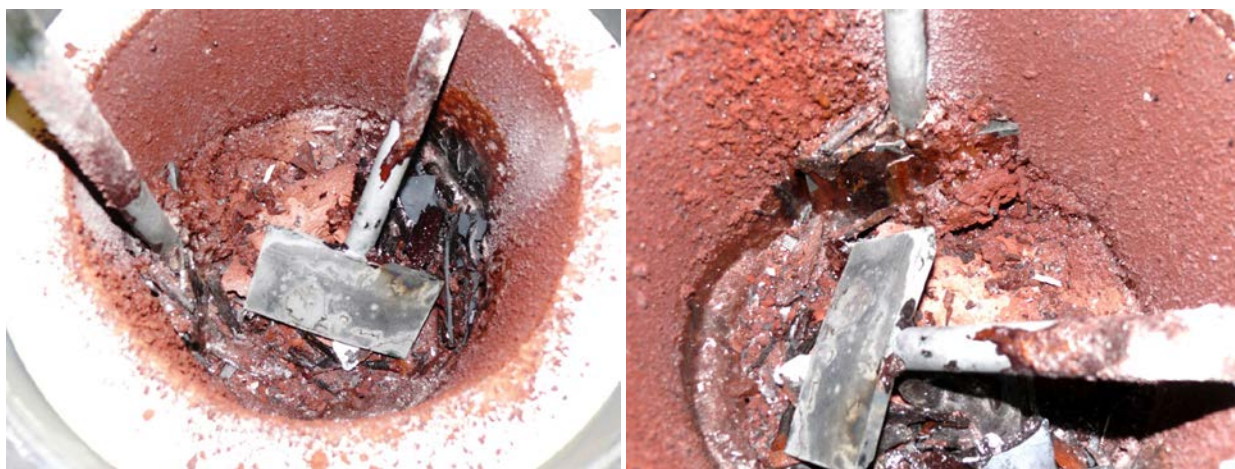
Figure 5.9. RSM-10 Melter Electrodes Pulled From the Glass Melt
