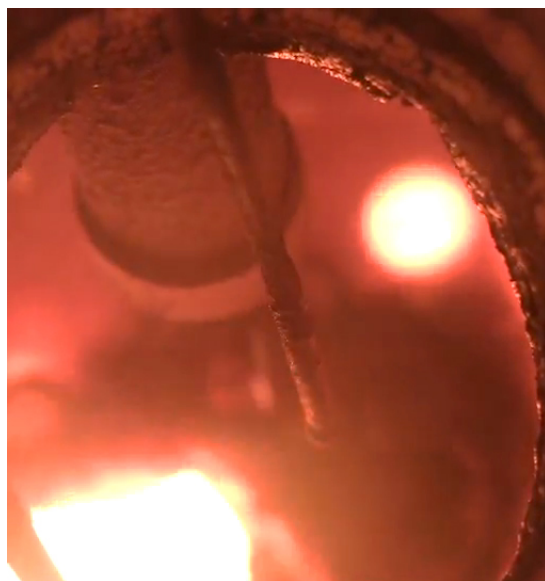
Figure 5.3. Photograph of the Cold Cap in RSM-6 Test Segment 1
