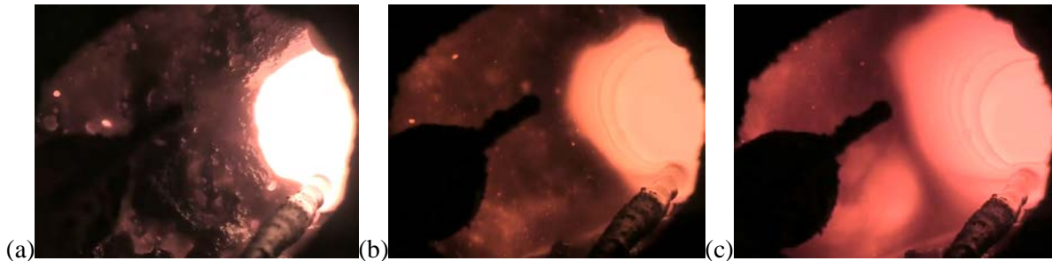
Figure 5.4. Frames Captured from a Video Taken during RSM-6 Test Segment 2 at 2.5-Minute Intervals (a) Before and (b & c) After a Glass Pour
