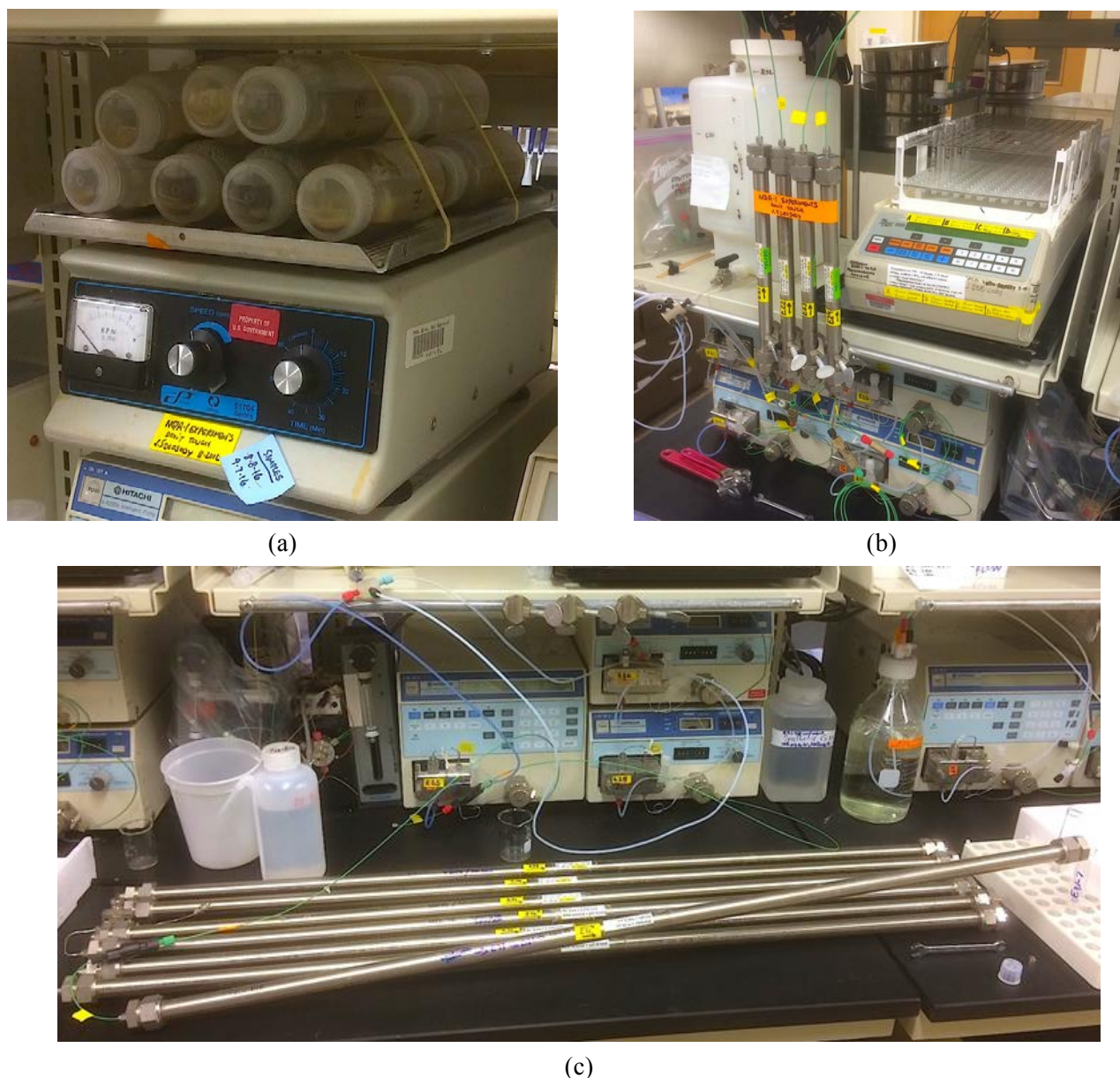
Figure 3.2. Images of (a) batch water leach experiments, (b) 1-D column water leaching experiments with continuous flow, and (c) no-flow column reduction rate and capacity experiments.
