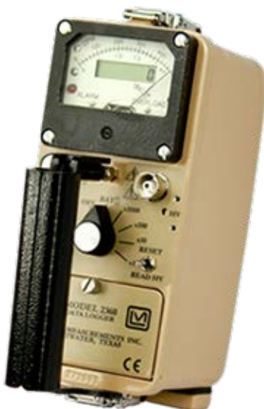
Figure 4. General purpose Ludlum 2360 meter generally paired with alpha/beta probe for contamination surveys
