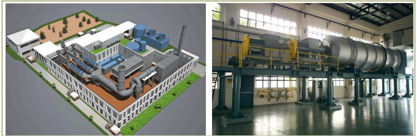
Fig. 6. Left) Three reactor rotary kiln system with waste dryers and a slagging kiln for conversion of high moisture MSW to energy; Right) Rotary kiln gasification reactor installation (flue gas clean up systems are exterior to the building).
