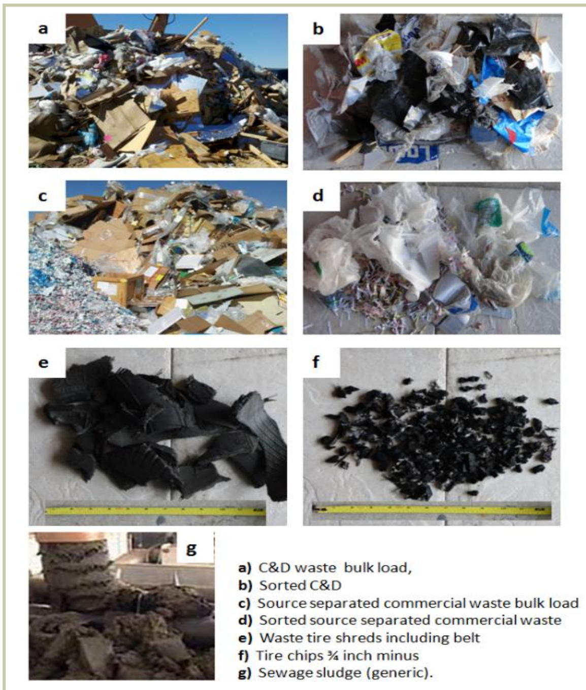
Fig. 14 (a, b, c, d, e, f, g) Various components of RDF for an air fed gasifier
