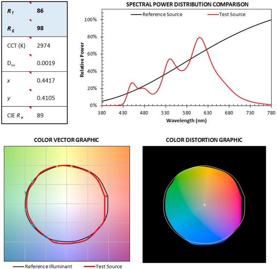
**Figure 10.** SPD, color metrics, and color rendering graphics for the 3000 K OLED panels.
