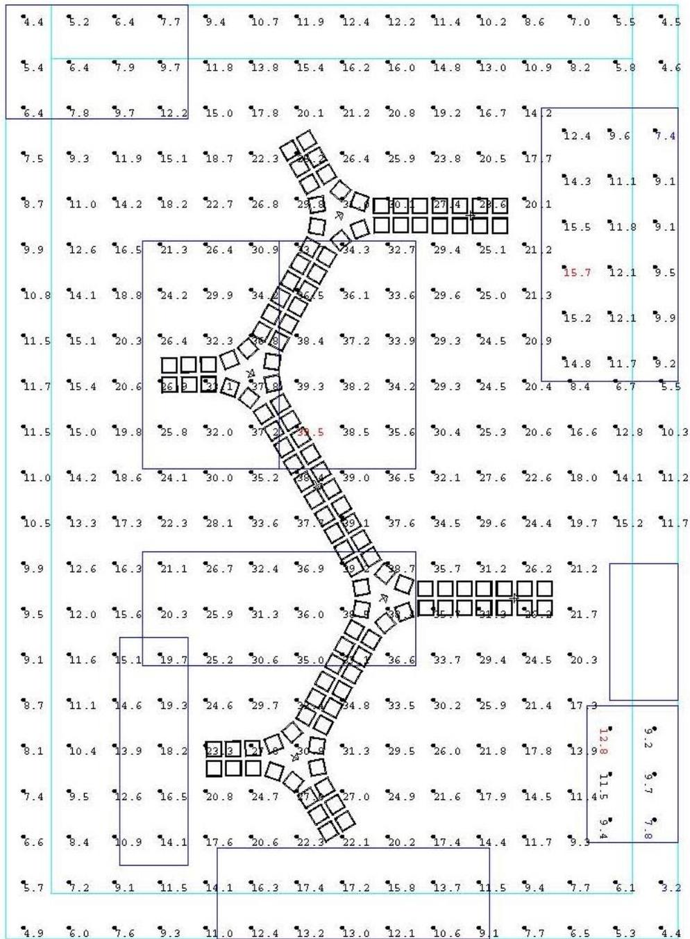
**Figure 3.** OLED system layout showing the calculated 30-in. workplane illuminances, using AGI32 software. Furniture locations are shown as rectangles and are approximate. Values are in footcandles. (Multiply by 10.76 for lux.) Calculation points are 1 ft on center. The light loss factor applied in the calculation was 0.85. The two areas with offset grids are calculated at a 3 ft 0 in. drafting table height. (Calculation: Aurora Lighting Design, Inc.)
