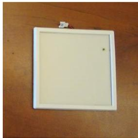
**Figure 8.** Failed OLED panel, showing dark spot in upper right corner that indicates a shorting defect in the OLED material. (Photo: Leslie North.)
