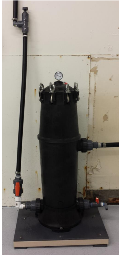
Figure 1. Big Bubba Filter System for Gross Filtration of Large Debris from Ambient Seawater. The unfiltered seawater was filtered through a 150 µm filter and delivered to a head tank for temperature control.
