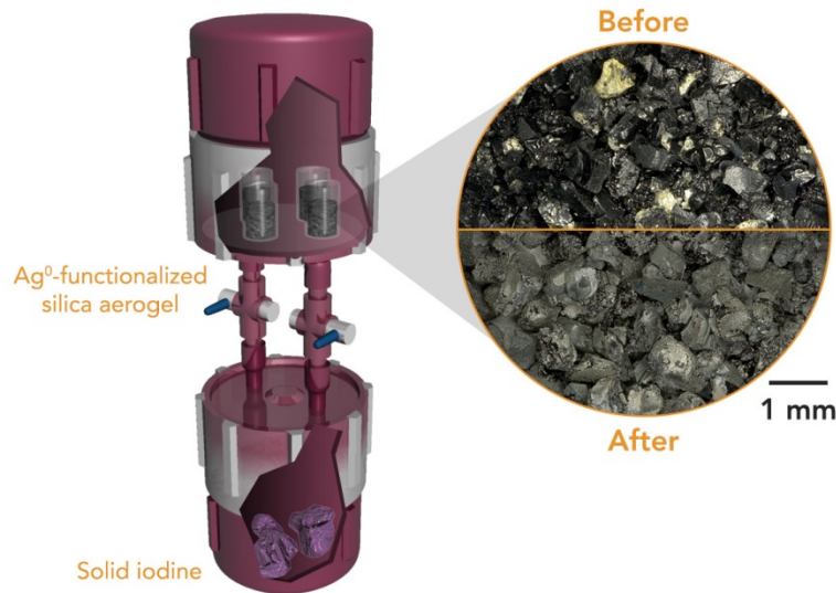
Figure 1. Assembly to produce iodine-loaded Ag 0 -aerogel; iodine vapors at 150°C for 24 h.
