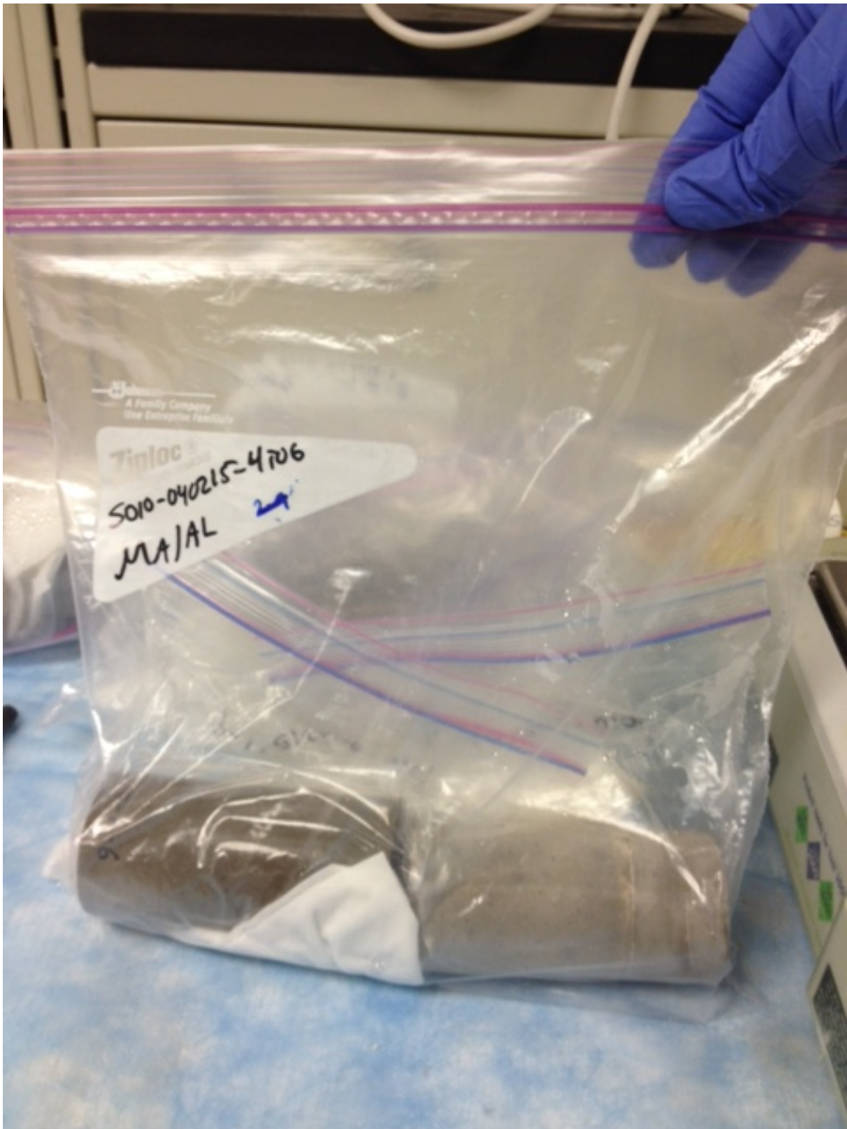
Figure 2.6. Storage Method-Monoliths in Double Lined Bags with Wet Paper Towel
