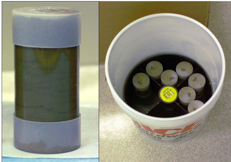
Figure 2.5. Curing Molds Filled with Cast Stone Slurry & Placement in Curing Containers
