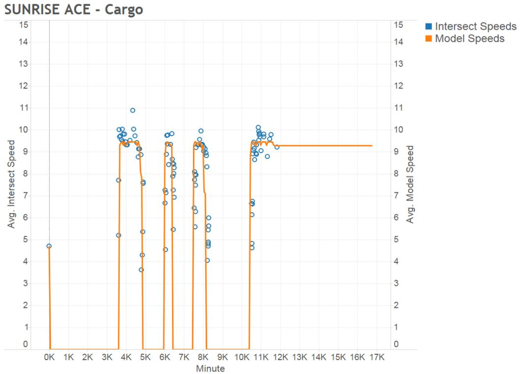
Figure E - 4: Example of speed checks against time to view correlation of model and original intersection files. The Sunrise Ace, a cargo vessel, had a very good correlation with the above scaling factors.
