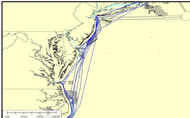
Figure E - 3: Towing model validation tracks overlaid onto original AIS tracks. The darker orange represent lines the model run, and the lighter color are the AIS tracks.
