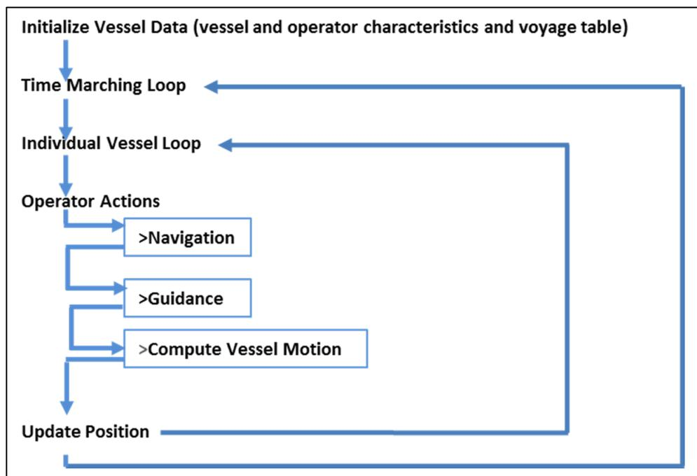
Figure D - 1: General computer code structure of MVT model for the solution navigation, guidance, and motion of marine vessels. Results from model computations are output at the end of each turn through the time marching loop.
