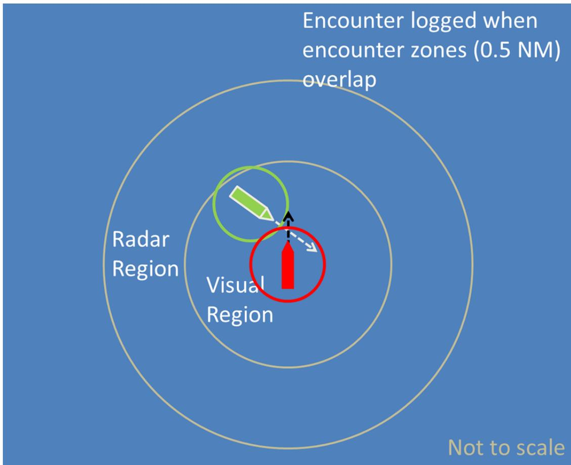
Figure D - 8: Schematic of the Method used to log when two vessels have an encounter.
