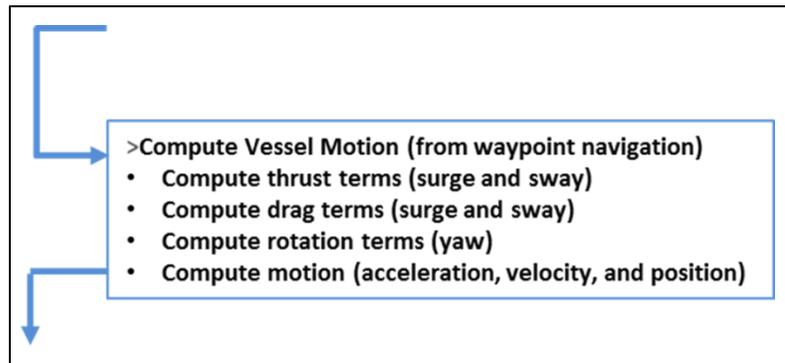
Figure D - 4: Vessel motion functionality in the MVT model computer code.
