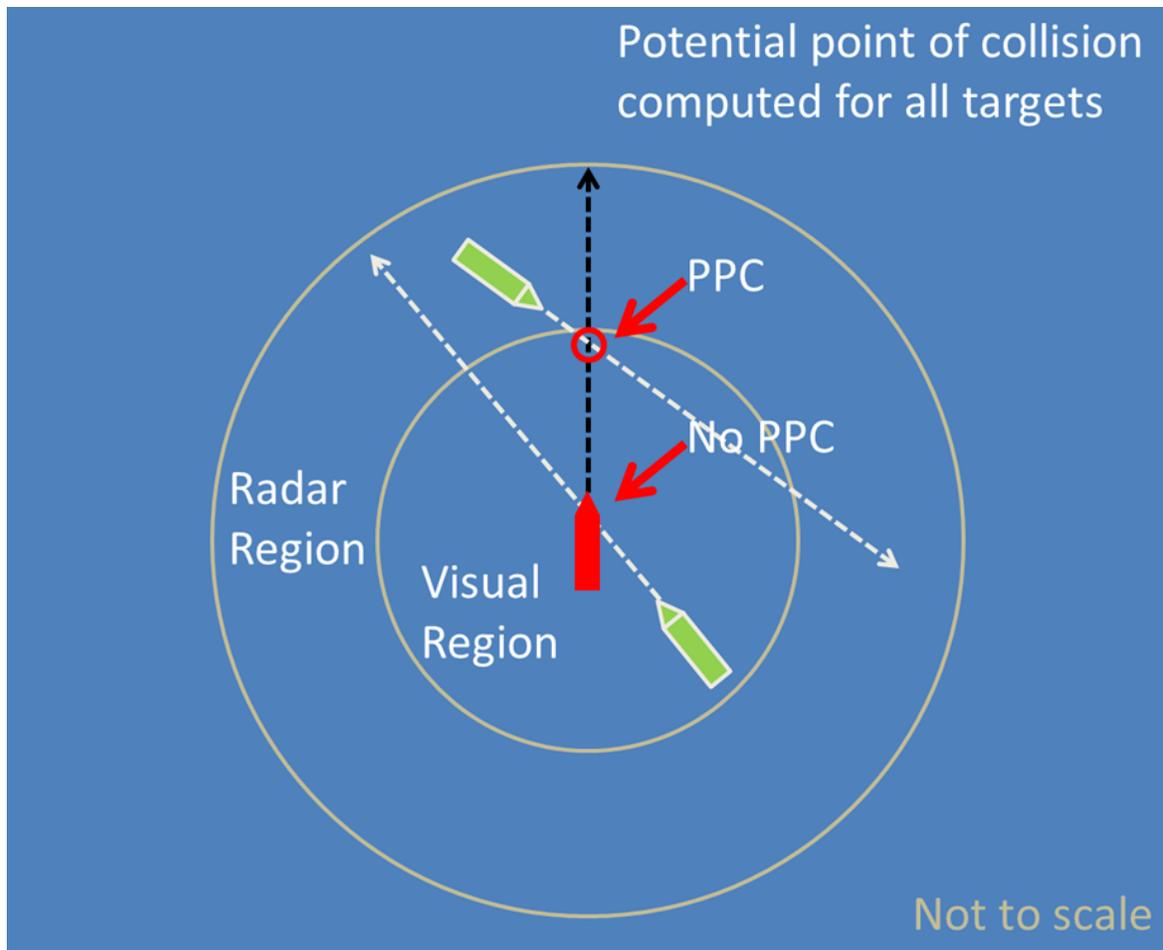
Figure D - 7: Schematic of the Method used to compute Potential Points of Collision (PPC).
