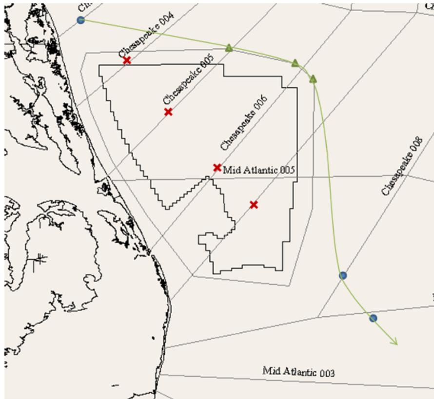
Figure D - 11: Generated Waypoints (green triangles) and estimated path (green line) to guide vessel around a windfarm. The input file waypoints are also shown, with eliminated waypoints in red and kept waypoints in blue.
