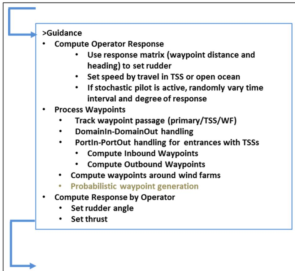
Figure D - 3: Guidance functionality in the MVT model computer code. The greyed text is functionality not yet fully implemented at the time of writing.
