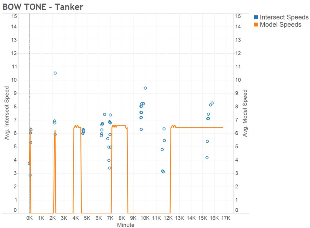
Figure E - 5: Example of speed checks against time to view correlation of model and original intersection files. The Bow Tone, a tanker vessel did not have a perfect correlation with the model scaling factors.
