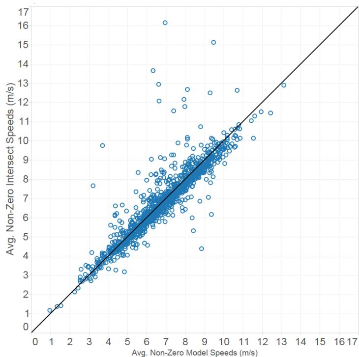
Figure E - 6: Plot of model average speed versus intersection file average speed. A perfect model would have a 1:1 ratio and the scaling factors come near to achieving this, with an R<sup>2</sup> value of 0.9819 and slope of 0.9993.
