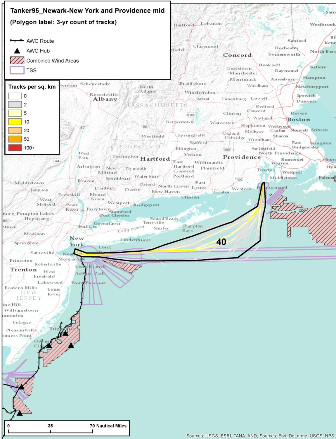
Figure B - 6: Port-to-port polygon showing the 95% boundary of cargo traffic between Newark-NY and Providence from 2010-2012.
