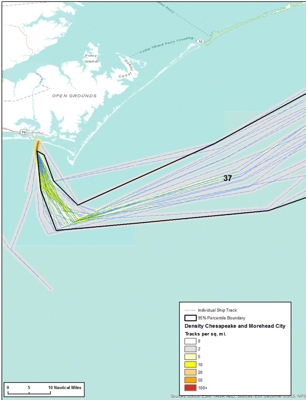
Figure B - 2: Example of the three GIS representations of port-to-port route polygons: lines, density raster and resulting polygon.
