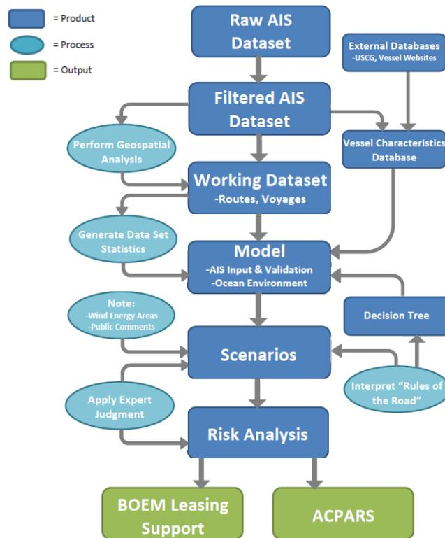
Figure 1: Process for acquiring, processing and applying AIS data for numerical modeling of navigation risk from offshore wind farms. The modeling critical path follows the center darker blue rectangles. Inputs processes provide further inputs (lighter blue ovals) and products (other dark blue rectangles) that build in a stepwise fashion. The green output rectangles represent to decision processes that the analyses will support.
