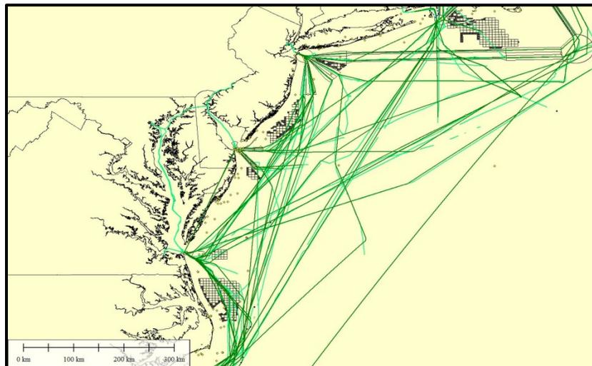
Figure E - 1: Cargo model validation tracks overlaid onto original AIS tracks. The darker green lines represent the model run, and the lighter color lines are the AIS tracks.
