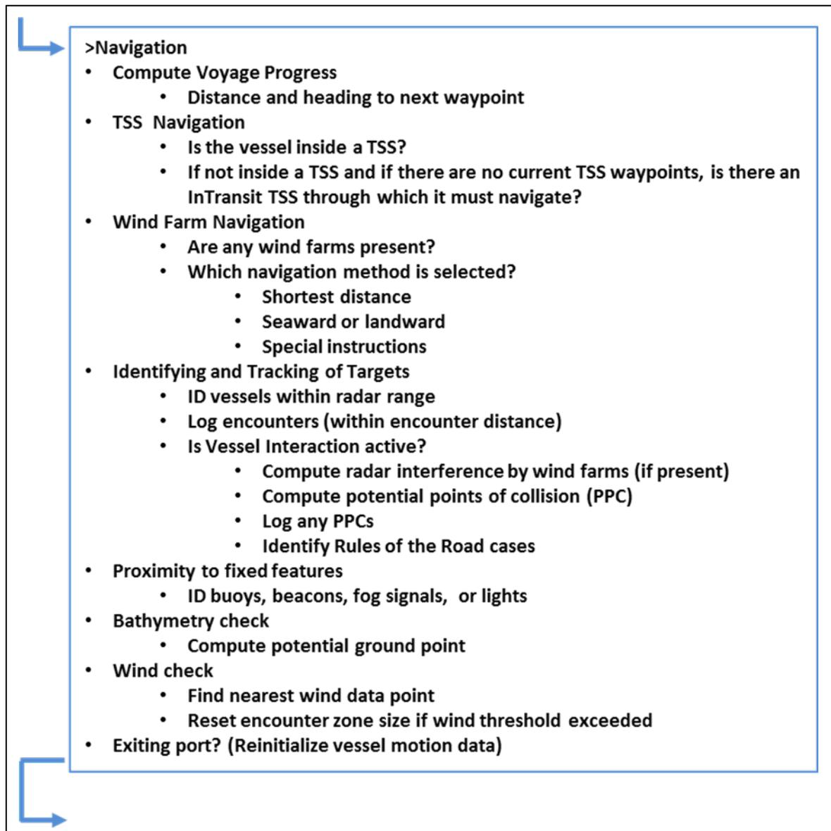
Figure D - 2: Navigation functionality in the MVT model computer code. Arrows indicate the navigational functionality is connected to a sequence of operations implemented to carry out vessel voyages.
